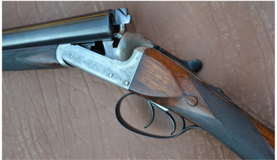
The venerable boxlock, in this case a 12-bore by William Evans, made on what is known as a Webley screw-grip action because of the unique rib extension.
