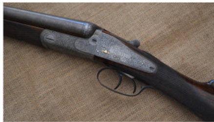
This is lovely Blanche 16-bore back-action sidelock shotgun. Because the mainspring is situated behind the tumbler in this design, the locks have a different shape compared to that of a bar-action sidelock.
