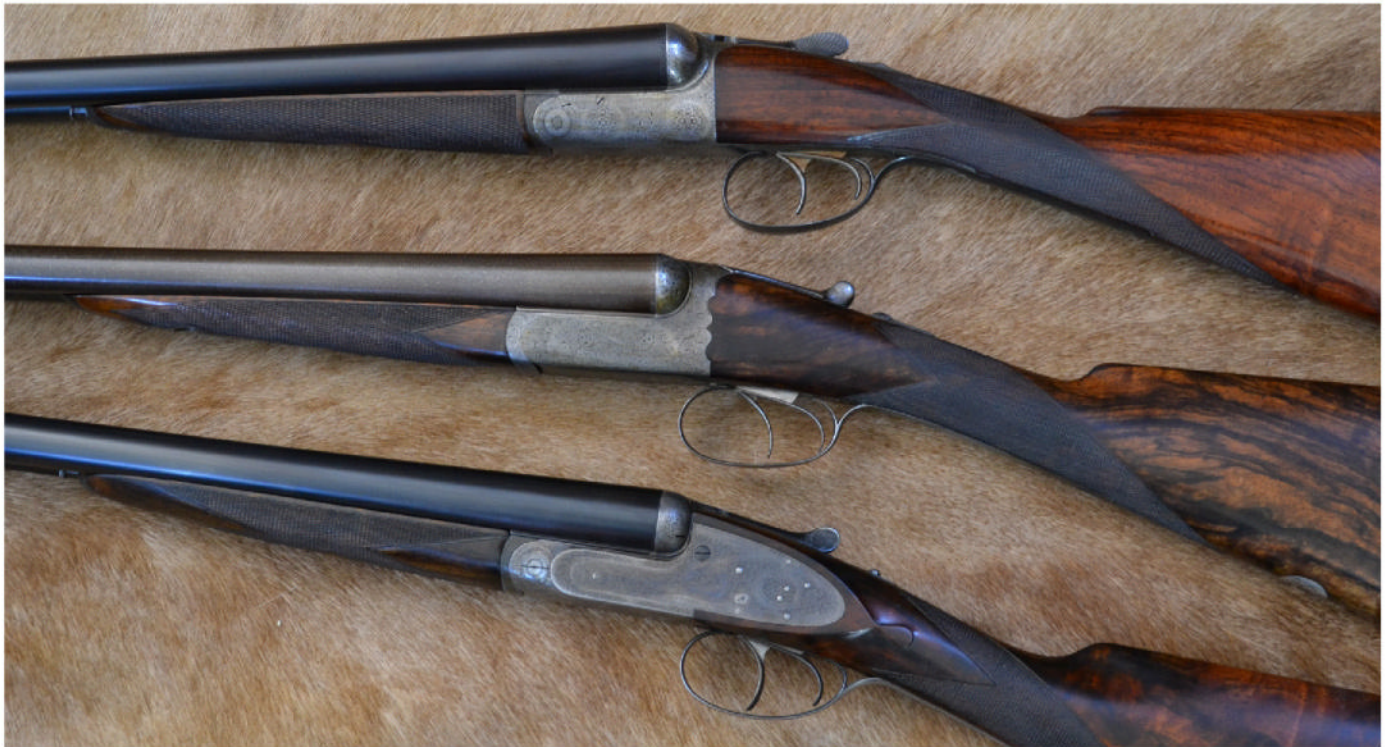
Three different British designs compared. At the top, we have a rare John Dickson 12-bore on their trigger-plate action. In the centre is a Westley Richards hand-detachable lock (or 'droplock') gun dating from 1897. At the bottom is a classic James Purdey Beesley-patent sidelock ejector gun. All three are in 12-bore.
