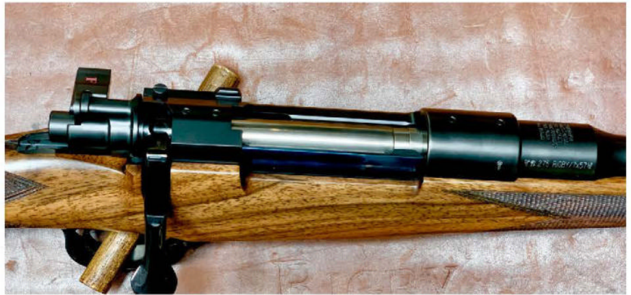
A .275 Rigby Mauser in the John Rigby & Co. London shop, with a three-position safety that rotates over the bolt axis as Bell would have used.
