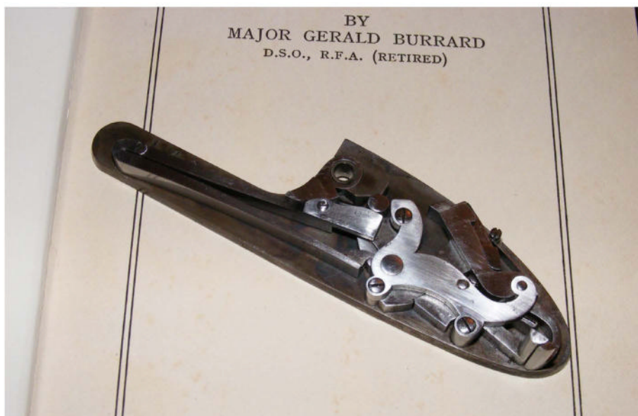
The lock of a classic Purdey sidelock ejector shotgun. The mainspring of the lock is clearly visible, as are the other moving parts. If such a mainspring breaks, it can be quite a headache to have a replacement made by a skilled pair of hands.
