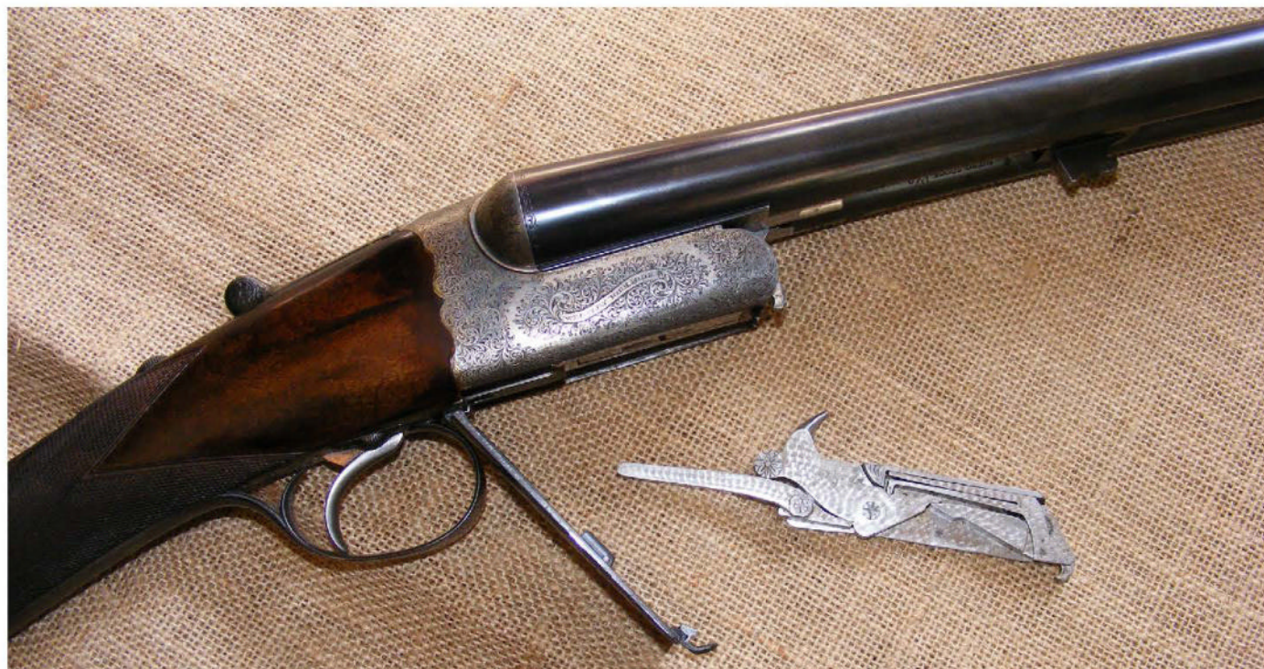
A Westley Richards hand-detachable lock boxlock-actioned shotgun with the left lock removed from the action. Note that the firing-pin protrusion is integral with the hammer...
