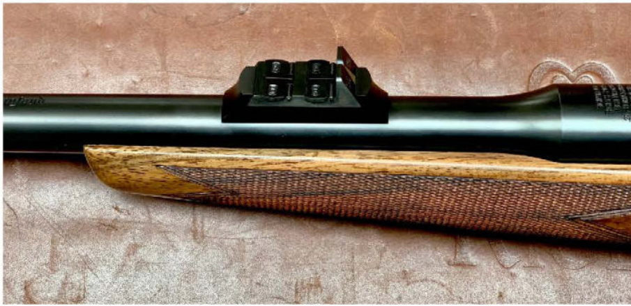
The three-leaf rear sight on a .275 Rigby set for 100, 300, and 400 yards. The leaf pack can also be ordered in a traditional 65-, 150-, and 250-yard setting, which seems practical when running the rifle without a scope.
