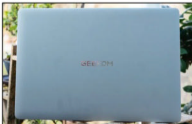
The magnesium alloy body is warm to the touch, rather than the cold feel of aluminium.
