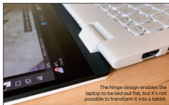
The selection of ports on the left- and right-hand side include HDMI, an audio jack, and USB Types A and C.
