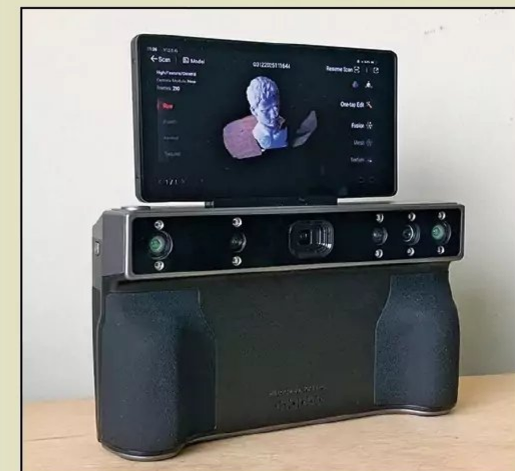
The screen flips out on a top-mounted hinge, making it easier to work with.
