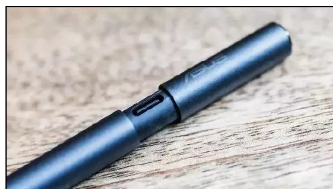
Open the clever pop-up port to reveal the ASUS Pen 2.0's hidden USB-C charging port.
