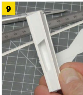
9 The corner pillars were constructed from 0.2mm plasticard.
