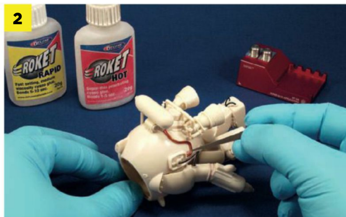
2 Scratchbuilt details are glued into place with the help of Rocket Rapid and Rocket Hot glues.
