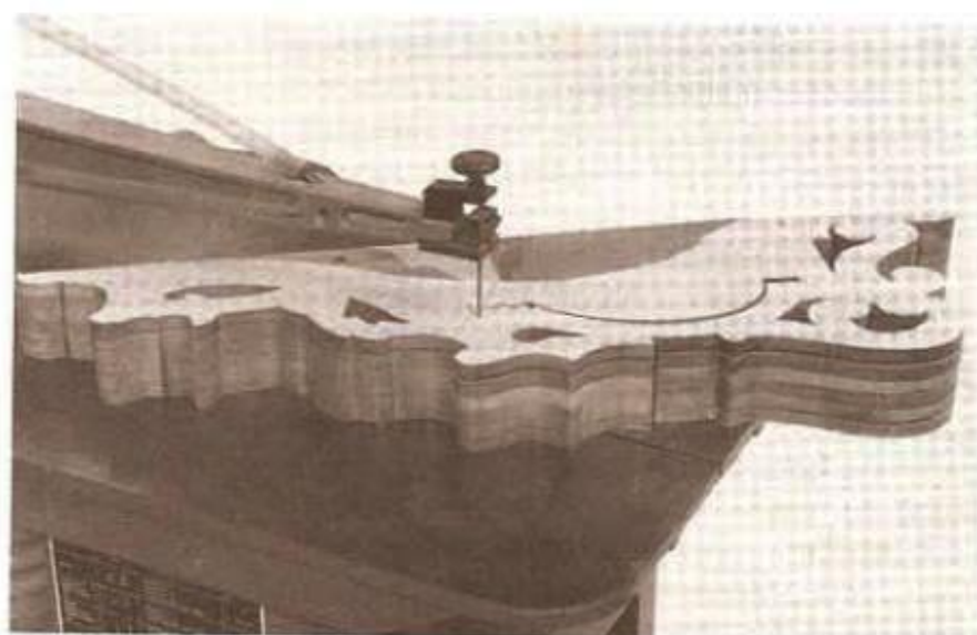
Illus. 2. The plant hanger project (pages 149–153) requires six identical pieces. Saw all from 1/4-inch-thick material. They can all be stacked and cut at once as shown with one of the many new precision-cutting scroll saws now available.
