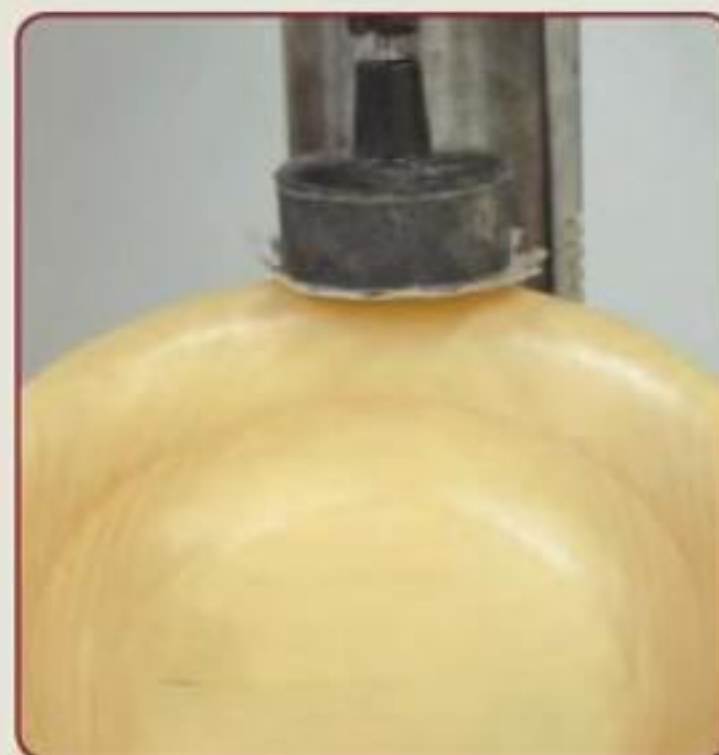
Use inside-to-outside strokes to shape the lip's outward flare.
