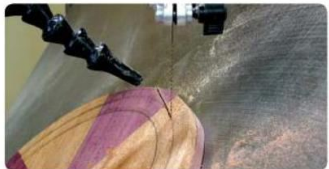
Cutting a ring in a clockwise direction means that the wood is moving counterclockwise. The cut will be wider on the upper face than on the lower one.
