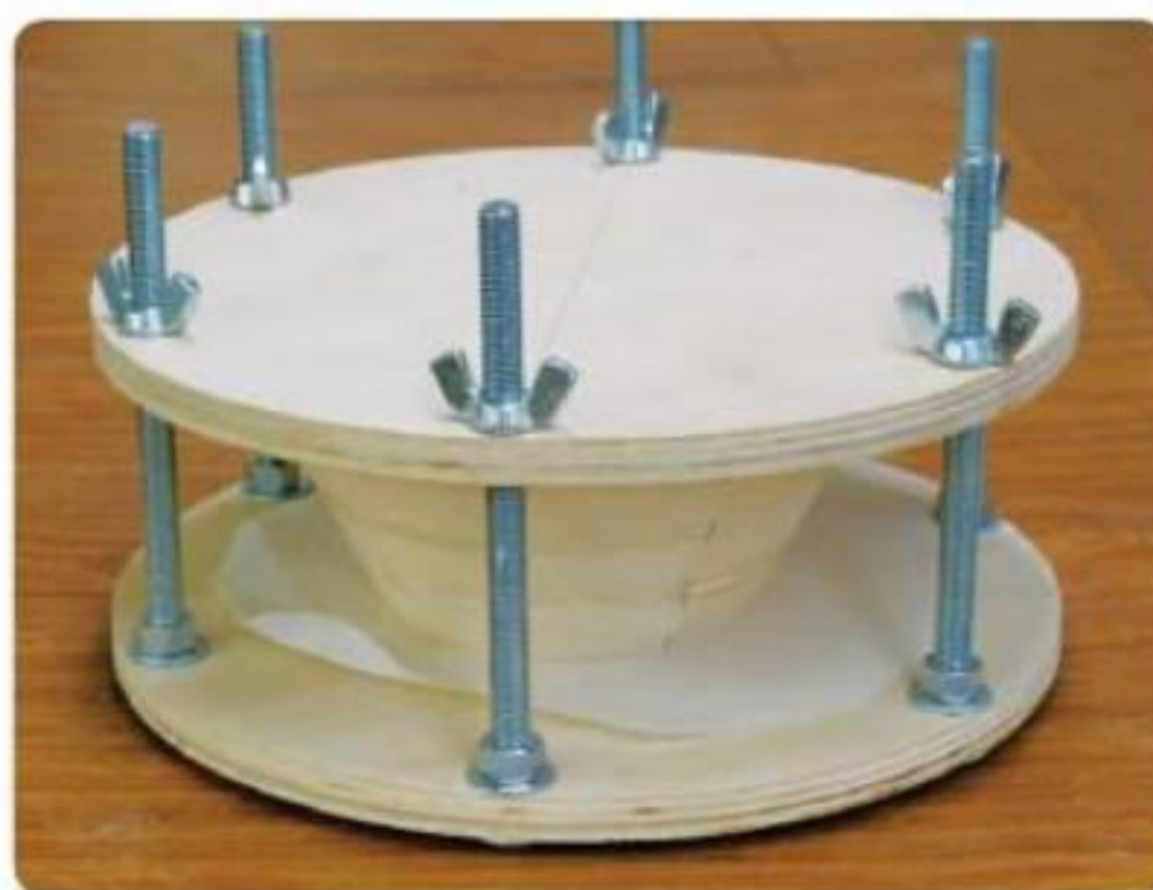
Evenly distributed downward pressure is essential for gluing up rings properly.
