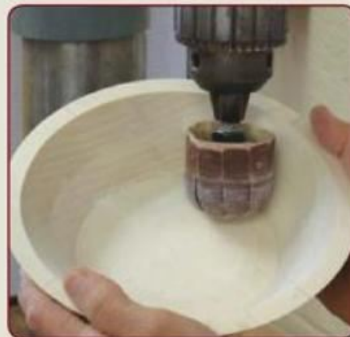
Use inflatable ball sanders to sand interiors.
