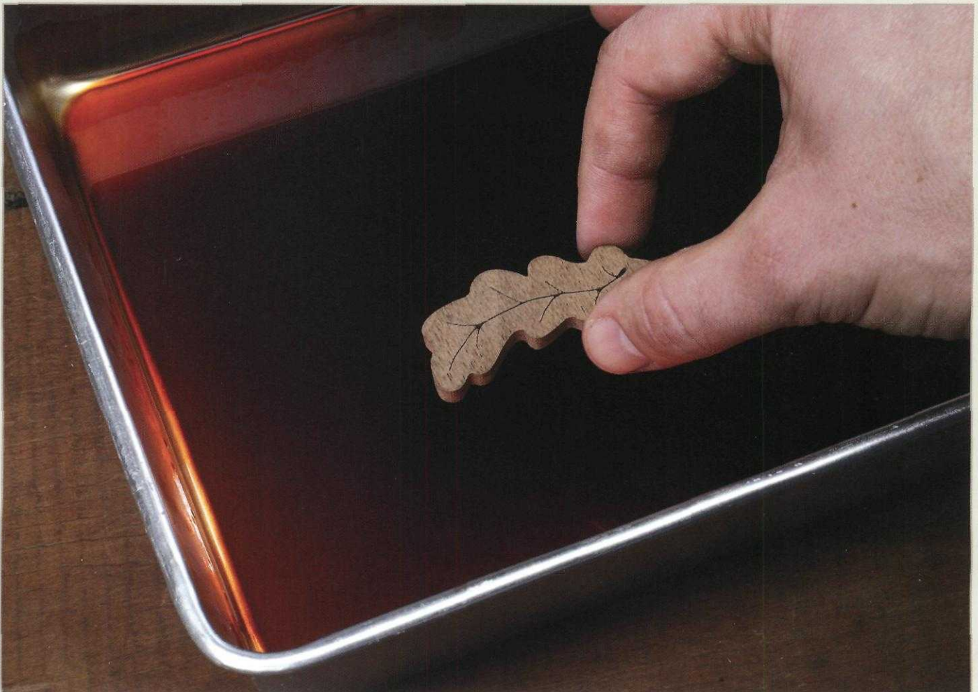
Figure 11. If you have used hardwood for your project, an easy method of finishing is to dip it in a dishpan or a similar container filled with a penetrating oil.
