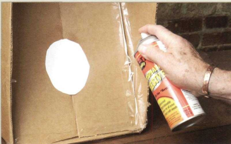
Figure 2. Use “repositionable” spray adhesive to adhere your patterns to the wood. A simple glue box, made from a common cardboard box, helps to confine the adhesive.
