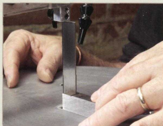
Figure 5. One way to check if your table is square to your blade is to use a small square. Place the square next to the blade and adjust the table as necessary until the blade and the square are parallel.
