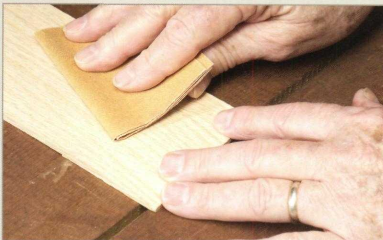
Figure 1. Be sure to sand the workpiece before applying the pattern. You may also want to sand the wood lightly once you have cut the design and removed the pattern to eliminate any “fuzz” and to get rid of any glue residue.
