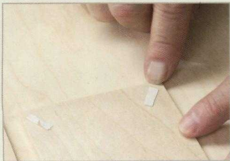
Figure 9. Masking tape or painter's tape (shown) placed around the edges can be used to hold a stack together. Some scrollers also like to cover the surface of the wood with tape before adhering the pattern to help lubricate the blade as it cuts. Double-sided tape placed in the corners of the workpieces can also be an effective method of holding the stack together.
