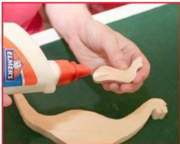
7. Applying glue to parts before clamping.
