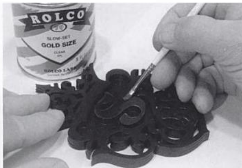
24-24. ▶ Applying the "size" (the gold-leaf adhesive) with an artist's brush.
