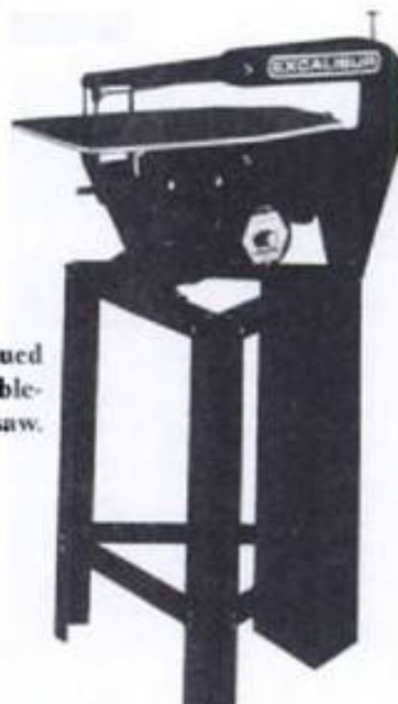
1-48. ► The RBI Eagle—a C-arm scroll saw with a 16-inch throat, 1½-inch stroke, two-speed belt drive, 2-inch maximum-cutting thickness, and tilting table—was discontinued in 1986 due to the success of the company's other parallel-arm machines.
