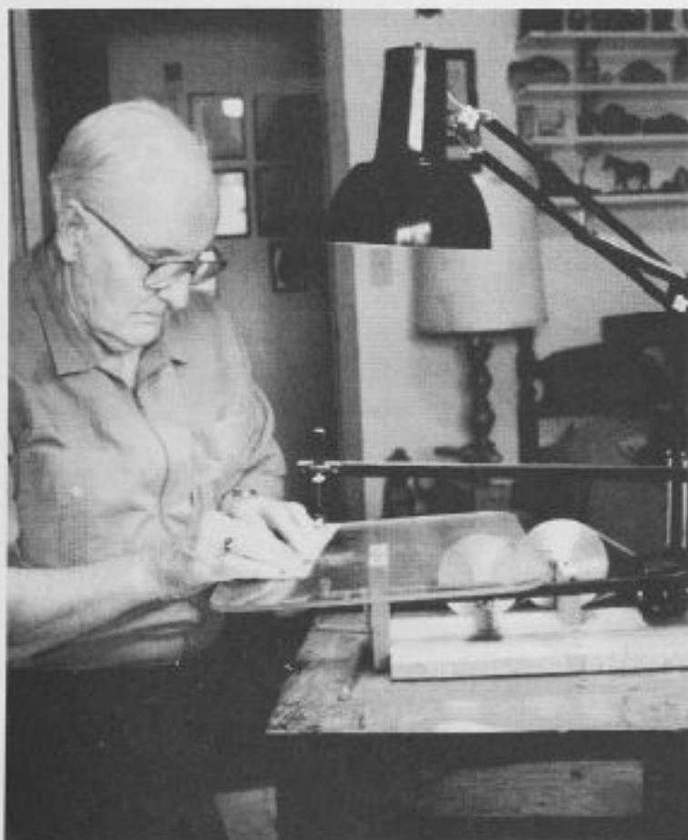
14-26. ► Marquetrarian Willard Bondhus at work on his current shop-made scroll saw designed exclusively for marquetry.
