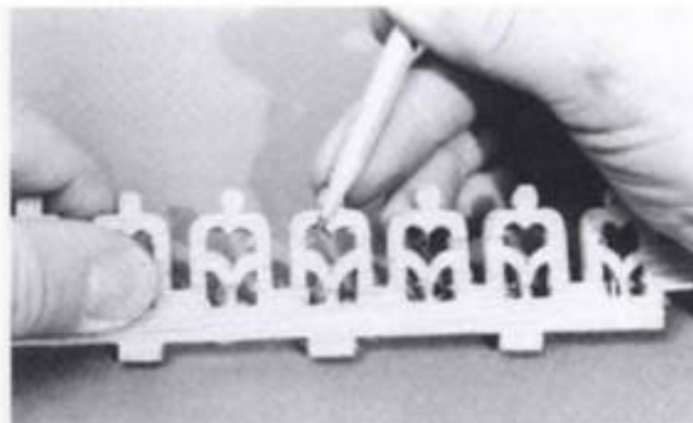
16-13. ▶ Examples of fretwork cutting problems primarily related to poor material choice. Weak fibers and poorly glued face veneer cause splintering and separation. Using a blade that is too coarse and an excessive feed can cause similar results.
