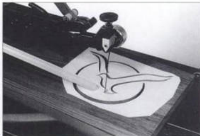
8-30. ▶ Sawing narrow inside openings.
