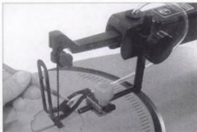
2-15. ▶ View showing how the airflow is obstructed with the open end of the hose fitted onto a "finger" of the hold-down.
