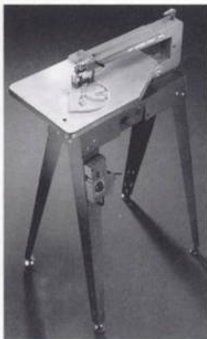
2-127. ▶ The Shopsmith 20-inch variable-speed scroll saw features new blade clamps and a speed range between 500 and 1,450 strokes per minute. Notice the switch-and-speed-control box mounted on the right front leg.
