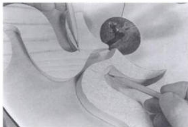
12-9. ► Here are the overcuts as seen from the back of the workpiece at the left and from the front at the right.
