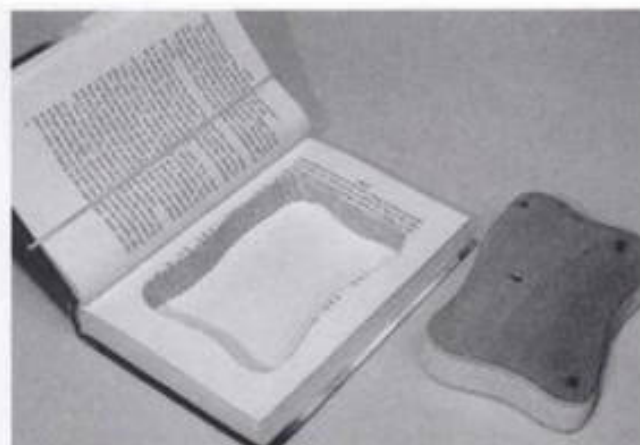
21-6. ▶ The completed sawn opening and the stack of waste.
