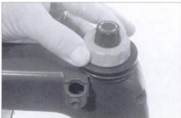
2-12. ▶ Craftsman's unique dual-control system for blade-tensioning. The outside is rotated to quickly engage or release the tension as shown. The smaller, inside knob is rotated to adjust the tension level. Notice the cast boss on the side provided for mounting an accessory light.
