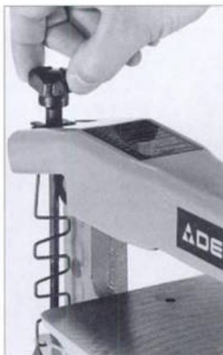
8-1. ► With the best blade installed, tension it with the appropriate control.
