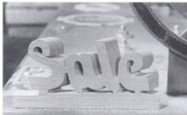
12-10. ► This cutout, sawn with a spiral blade capable of cutting in all directions without rotating the workpiece, has all of its edges slanted to the right. Notice the roughness of cut produced by the spiral blade.
