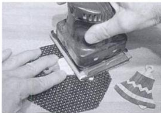
22-18. ▶ The surfaces are sanded flush and finished. The nonslip pad eliminates clamping.
