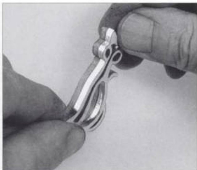
20-7. ▶ This shows the very smooth cut on 1/8-inch brass sawn while temporarily bonded to a plywood waste backer.
