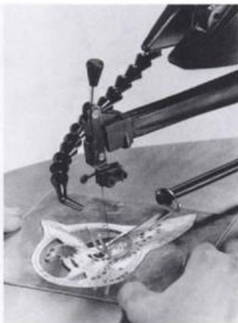
2-38. ▶ This excellent dust blower directs fine dust away from the operator.
