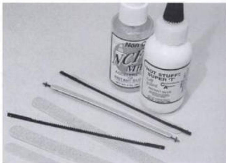
3-27. ► Glue emery boards to dull saw blades to make your own scroll-saw sanders.
