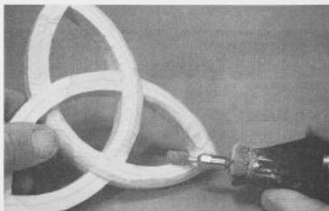
12-34. ▶ Shaping and rounding over the bevel-sawn edges. The pencil line made freehand along the center of the design aids the shaping.
