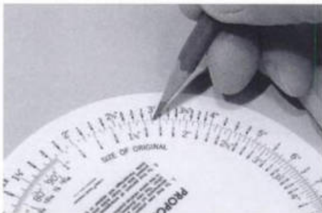
7-17. ▶ Step 1: Align the dimension of the small original pattern on the inner disc with the dimension you want (3 inches) on the outer disc, as shown.
