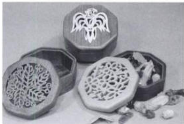
16-24. ▶ Router and fretsaw techniques were employed to make these boxes without requiring usual joinery.
