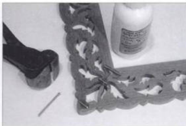
18-30. ► Epoxy or glued nails applied to the back surface of this fretwork mitered frame strengthen the joint without worry of splitting the thin, delicate joint with conventional nailing practices.
