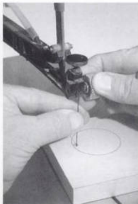
8-29. ▶ Threading the blade to saw an inside opening. Notice the location of the blade-entry hole. A layout made with red pencil is easier to follow than a black line.
