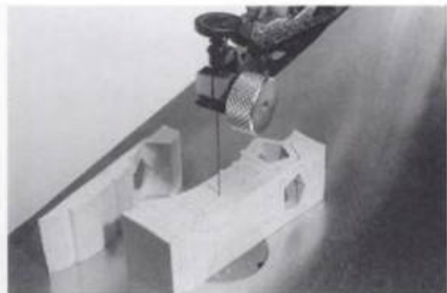
11-7. ▶ Completing the second cut of a chess piece.
