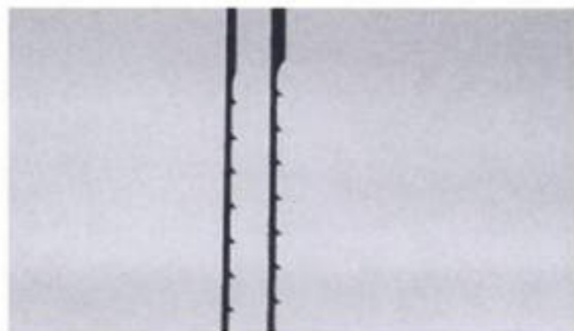
5-24. ► Unmodified blade on the left. The same modified blade on the right permits drilling smaller-size blade-entry holes.
