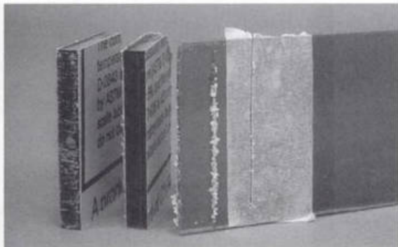
19-10. ▶ Left: Undesirable cut on \frac{1}{4} -inch-thick extruded acrylic plastic made with a No. 5 crown-tooth blade at 400 strokes per minute and with a slow feed. Center: Same extruded acrylic plastic, but cut with a No. 9 crown-tooth blade, at the same speed and approximately the same rate of feed. Right: Piece of \frac{1}{8} -inch extruded acrylic (covered with transparent film) with a fused cut that is shown alongside a clean kerf made when masking tape was applied to the surface. A No. 5 crown-tooth blade was used for both cuts at approximately 350 strokes per minute and a slow rate of feed.
