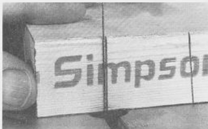
8-7. ▶ Rotate the test piece, keeping the same surface on the saw, and bring it and the test kerf to the back of the blade as shown. The table is square when the blade
