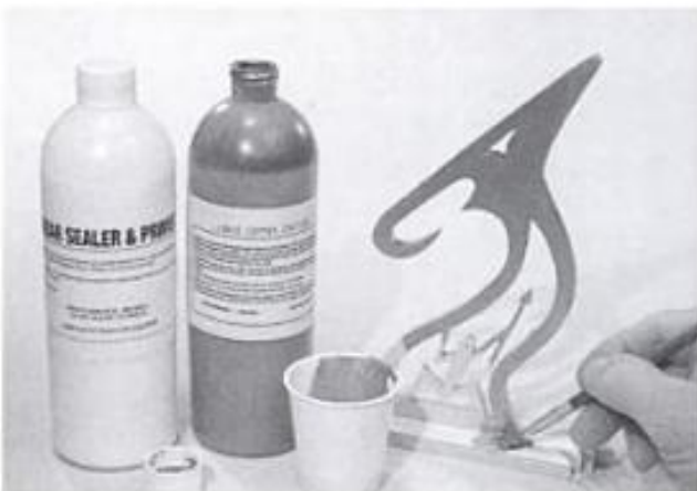
24-19. ► To apply a patina finish to wood, the wood is given a special coating, which is a blend of finely ground metallic (copper) solids suspended in a water-based air-drying emulsion.
