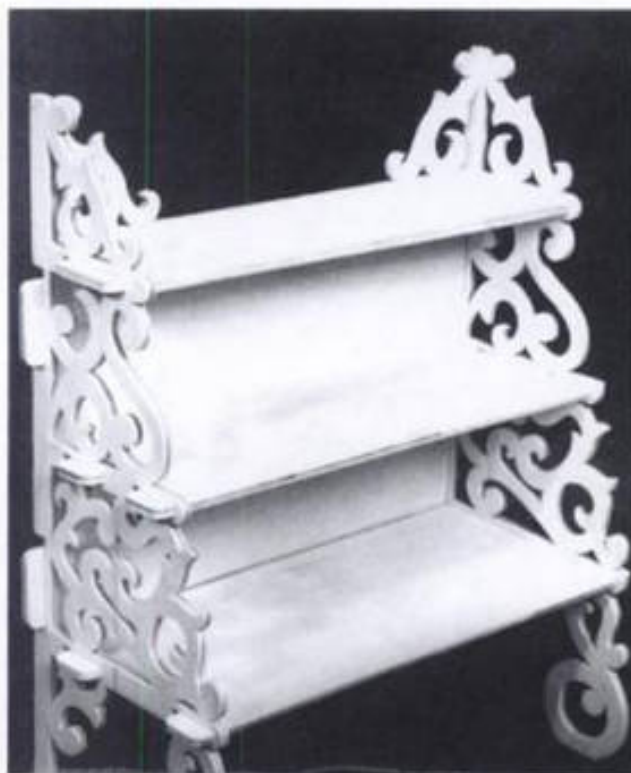
18-6. ▶ A locking tab-and-slot joint was used to assemble this entire project.
