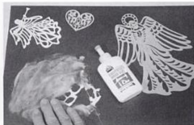
17-14. ► Thin \frac{1}{32} -inch plywood overlays ready for gluing. Glue is being spread on a flat laminate countertop in preparation for transferring it to the backs of the overlays.
