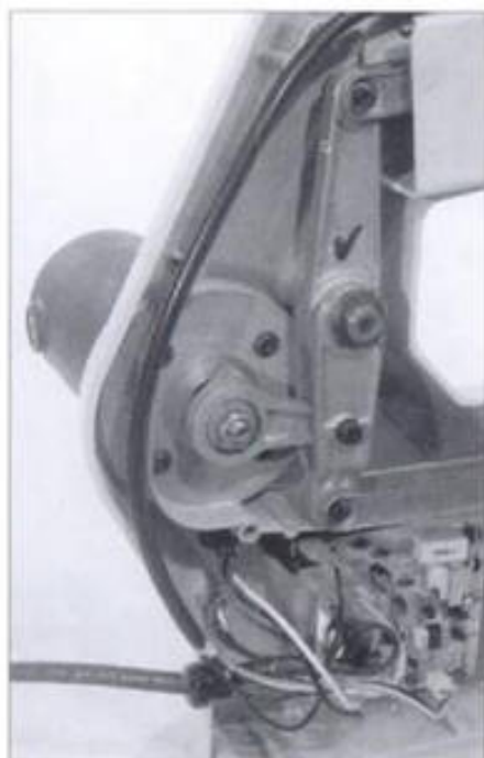
2-46. ► This close-up of the drive system shows the main rocker and connector, which create the back-and-forth movement of the upper and lower drive links.
