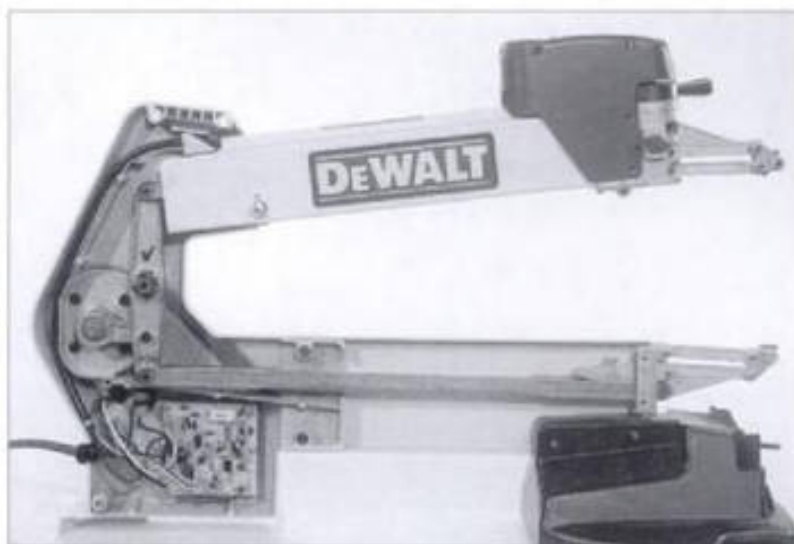
2-45. ► Removing the side panels of the DeWalt saw clearly shows the interior workings of the double parallel-link drive system that creates the vertical reciprocating blade action.
