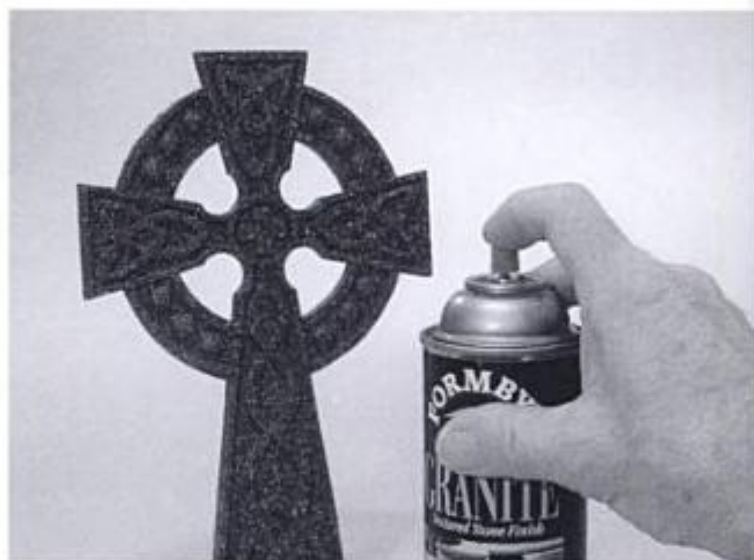
24-11. ▶ Applying a textured, stone-fleck aerosol finish.
