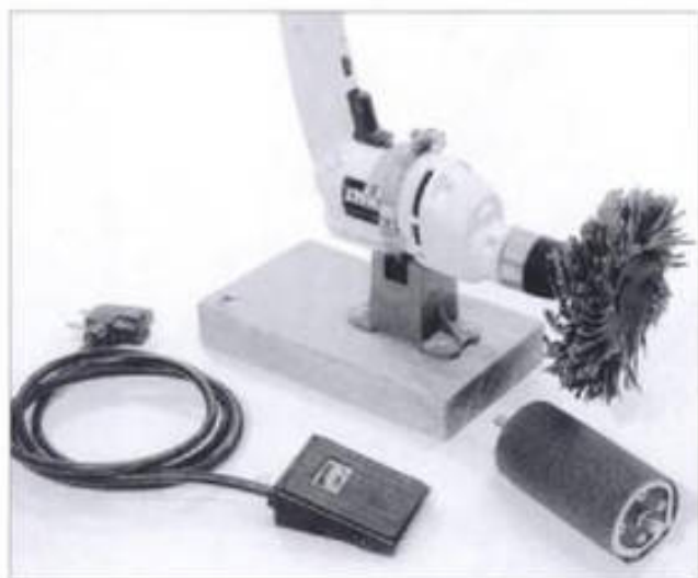
3-1. ▶ Lower left: Foot switch. Center: Hand drill with a flutter sanding wheel mounted on a stand. Lower right: Small air-inflated sanding drum that will fit the drill.
