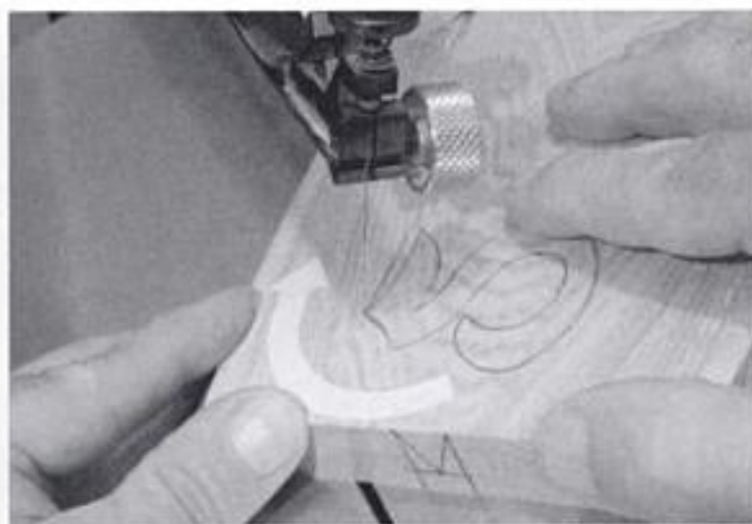
15-15. ► Here the table is tilted left and the workpiece is being rotated clockwise around the blade, making a complete 360-degree on-the-spot turn at this point before the cut is continued.
