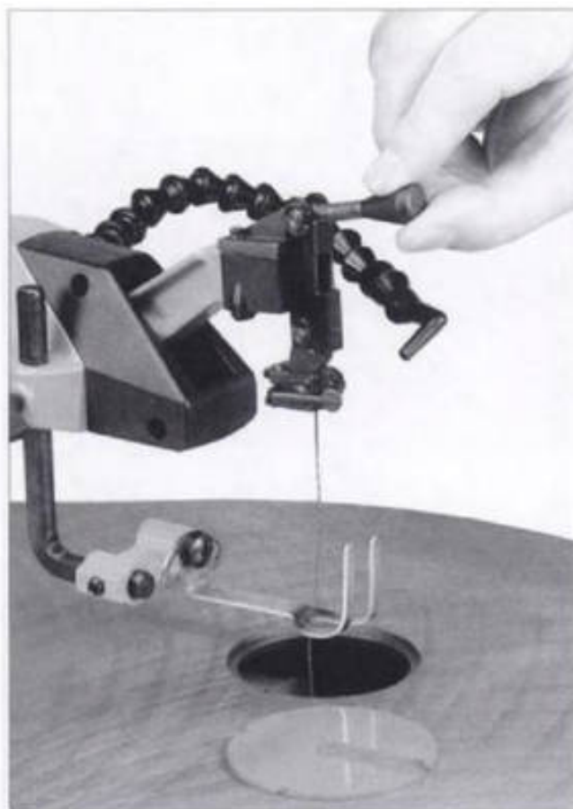
2-27. ▶ Delta's new blade-tension lever is pivoted toward the rear to apply tension or toward the operator to release the tension.
