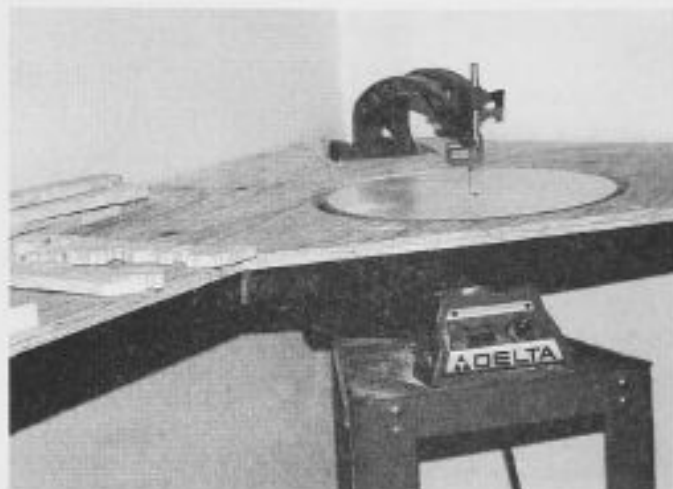
16-44. ▶ One of Robin's earlier scroll saw set-ups shown during construction. The entire tabletop will be covered with plastic laminate.
