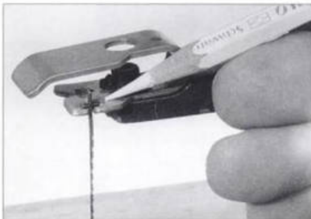
I-14. ▶ Pin-end blades are easy to install and some scroll saws have holders that allow their teeth to face in any of four directions: front, back, to the left, or to the right, as shown.
