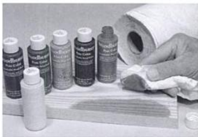
24-15. ▶ Direct from the bottle, "color stain" is an oil-based product applied with paper towels.
