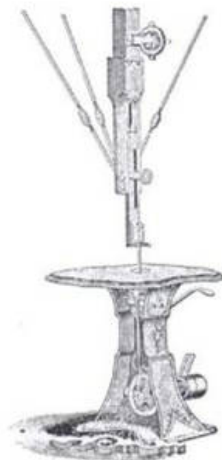
1-37. ▶ Fay's early-industrial scroll saw was driven by line shafts from water or steam power. The overhead straining mechanism provided unlimited throat capacity. Reciprocation was provided by the wheel-and-pitman (page 15) action, which moved the blade in vertical guides.
