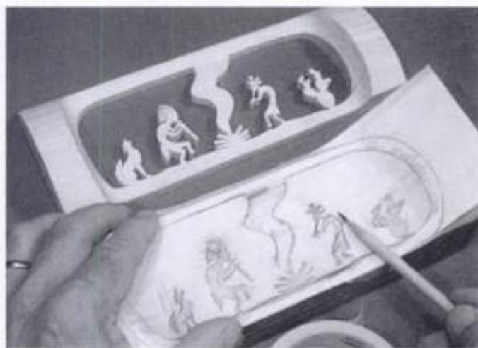
7-49. ► Copying an existing piece of scroll-saw work by making a "rubbing" using paper and a soft lead pencil.
