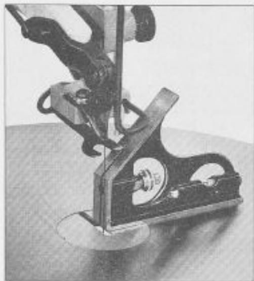
8-5. ▶ Check ing the table adjustment with a square.
