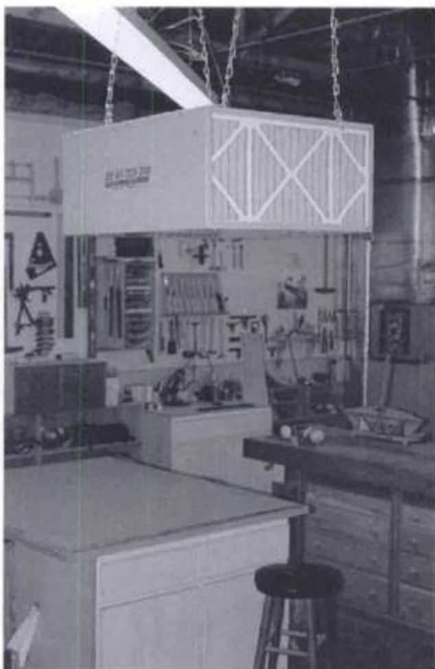
6-12. ▶ This ceiling-mounted air-filtration system quietly filters the shop air several times per hour, removing invisible and dangerous dust particles.
