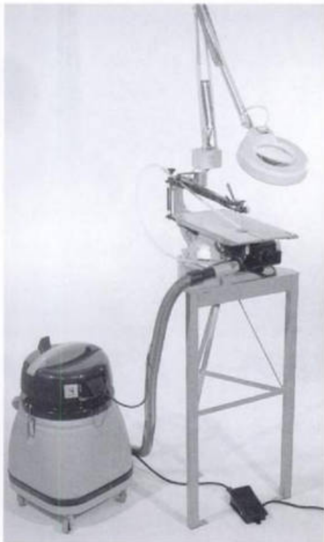
6-15. ▶ A Hegner saw equipped with its dust-removal system, and a Fein shop vacuum with a 5.0 micron-filtration capability.
