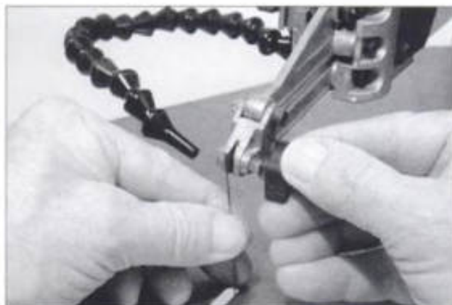
2-43. ▶ Blade installation is quick and easy with DeWalt's simple, toolless blade clamps.
