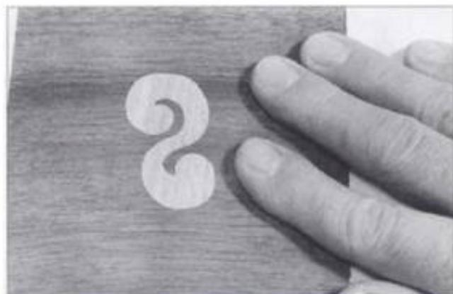
14-23. ► The back surface exhibits a perfect fit without any visible saw-kerf spaces.
