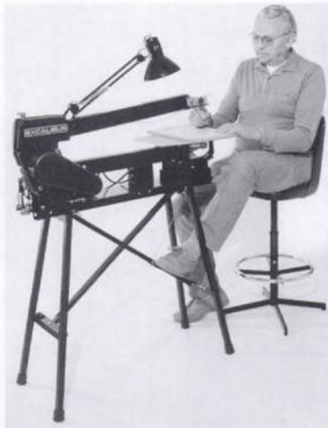
2-66. ▶ The setup for the Excalibur 30-inch saw, operated here by master scroll-sawer Carl Weckhorst, utilizes a stool, lamp, and Seyco's "top arm-lift pedal." (Photo courtesy of Seyco Sales.)
