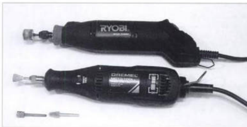
3-31. ▶ Ryobi, Dremel, and similar brands of rotary tool carry an endless variety of cutting, shaping, and drilling tools. They have collets from \frac{1}{32} to \frac{3}{16} inch in diameter and rotate at speeds up to 30,000 rpm.
