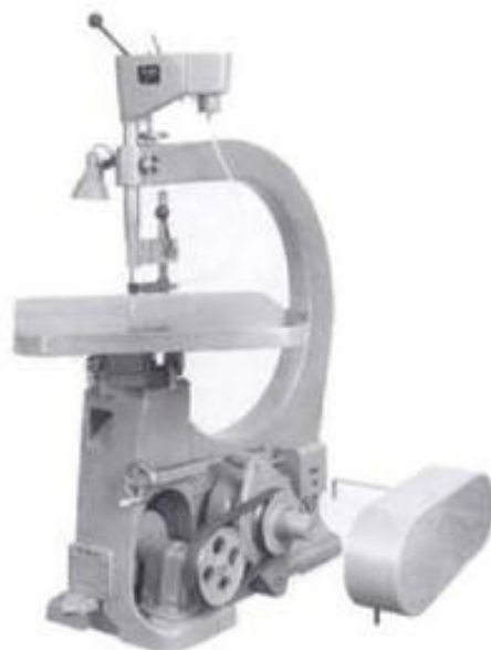
1-39. ▶ An Oliver 36-inch industrial, variable-speed scroll saw. This machine weighs 1,600 pounds, stands 6 feet high, carries blades up to 18 inches in length, and cuts stock up to 10 inches thick with a 2\frac{1}{2} -inch stroke.
