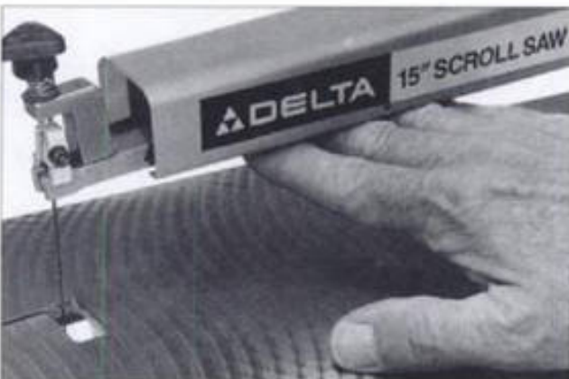
6-8. ► Some saws have guards or enclosures that protect the operator from contact with a moving upper arm.
