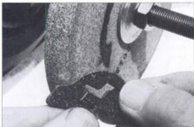
19-24. ► The Wonder Wheel (nylon impregnated with abrasive) is available from Judy Gale Roberts's studio. It is ideal for polishing metal and shaping Corian, as well as for detailing intarsia pieces.
