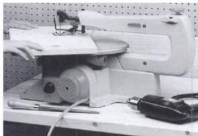
2-123. ▶ The Ridgid scroll saw in use. Notice the vacuum port visible under the rear right of the table and the non-adjustable blower hose connected to the hold-down.
