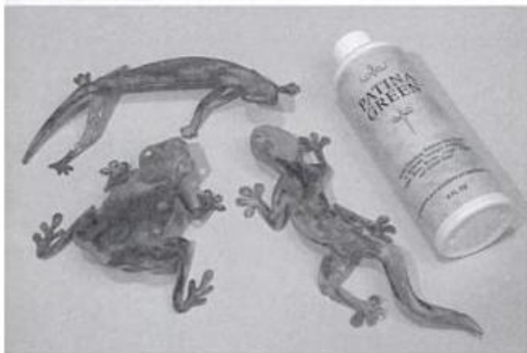
24-18. ► Scroll-sawn critters cut from sheet copper, bent, and then coated with a patina solution, which gives them a popular “aged” look.
