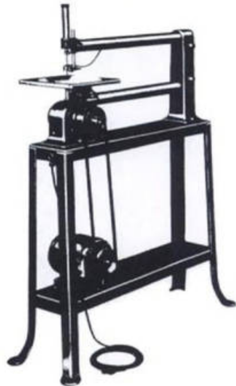
1-42. ➤ A 1930 version of Delta's popular 24-inch rigid-arm jigsaw. Manufacturer's claim: "5 years in development...opens new era in scroll sawing."
