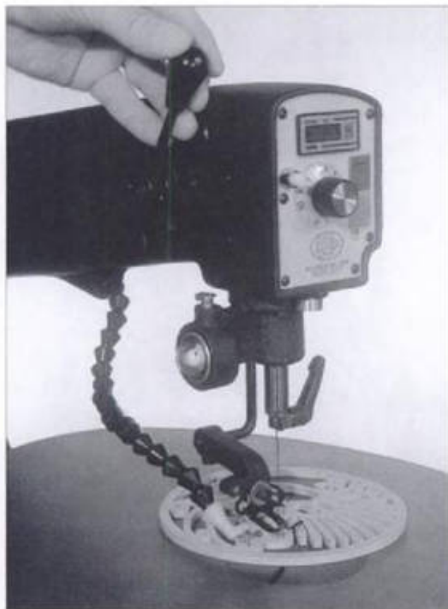
2-63. ▶ The up-front blade-tension lever is easy to reach and of a large size that is easy to use.
