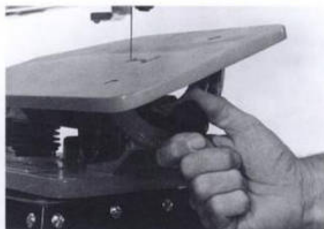
8-4. ► Use the table-tilt control knob to clamp the table square to the blade.
