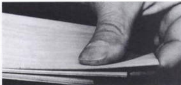
16-12. ▶ Light-colored \frac{1}{32} -, \frac{1}{16} -, and \frac{1}{8} -inch Finnish plywood with void-free edges. Baltic birch with similar characteristics is available.
