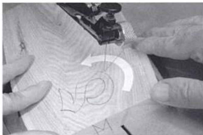
15-14. ► A practice bevel cut, in which the work is fed counterclockwise into the blade.
