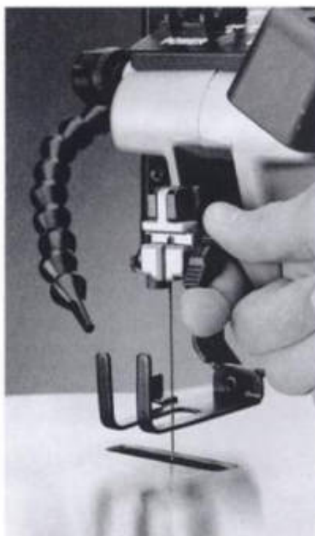
2-53. ► A good view of the improved upper blade-clamp design shows the reflective, zinc-oxide-coated surfaces that visually make blade installation much easier.
