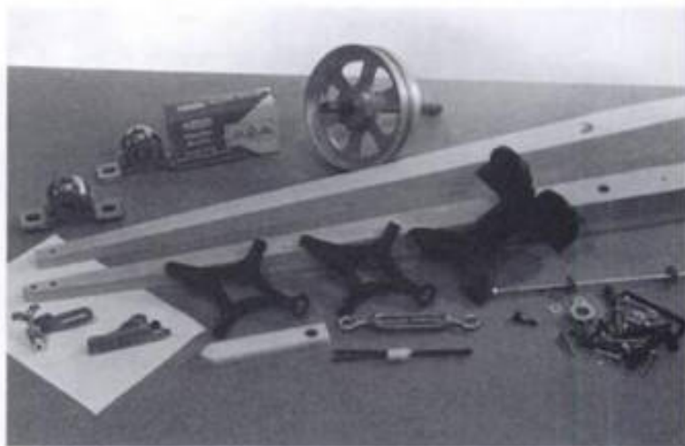
2-131. ► Components of The Tool Company's saw kit. The motor, motor pulley, belt, electrical switches, and wood for the stand must be obtained by the builder.
