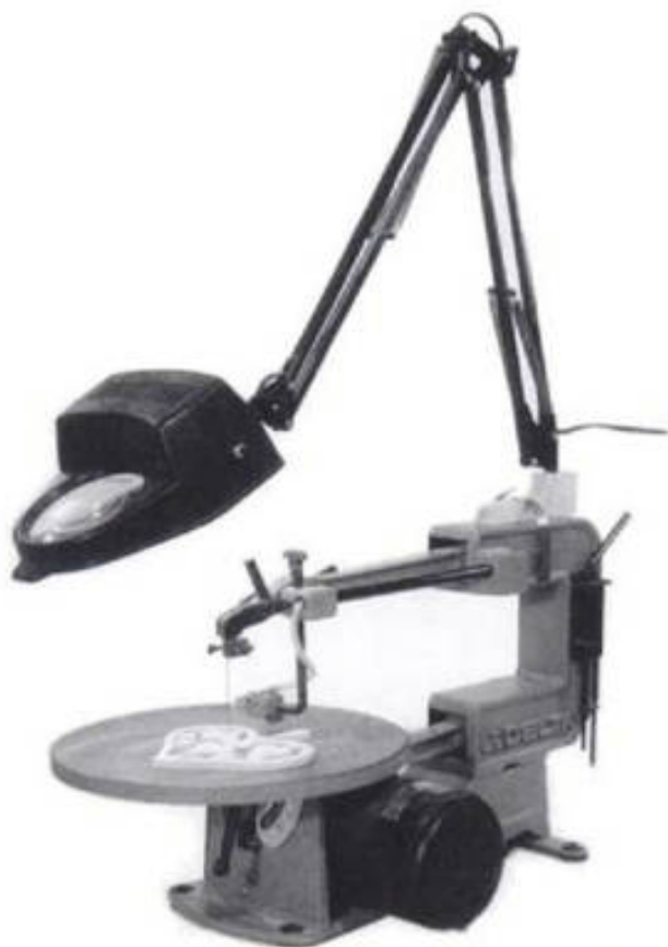
3-4. ▶ An inexpensive magnifier light on a small saw attached with a shop-made wooden mounting block and a large hose clamp.
