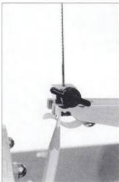
2-114. ▶ Close-up of the lower arm showing the two-position "notch" for the blade holder that offers a choice of cutting actions. Positioning the blade clamp into the rear "notch" is recommended for more aggressive sawing and square-cutting in thick stock. The front notch is recommended for normal cutting.
