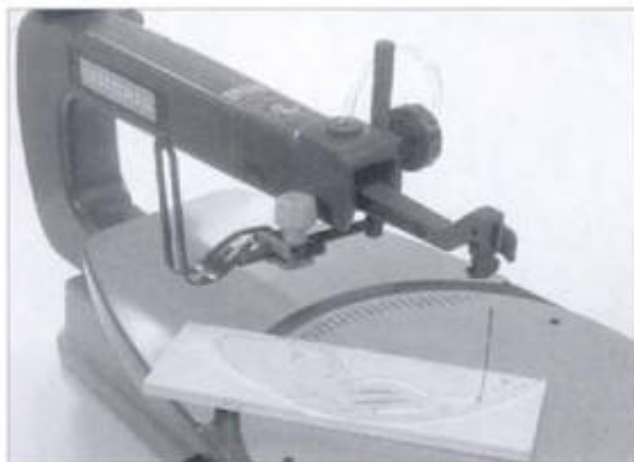
2-11. ▶ Making room for threading the blade through the workpiece requires raising the hold-down/guard and swinging it to the side.
