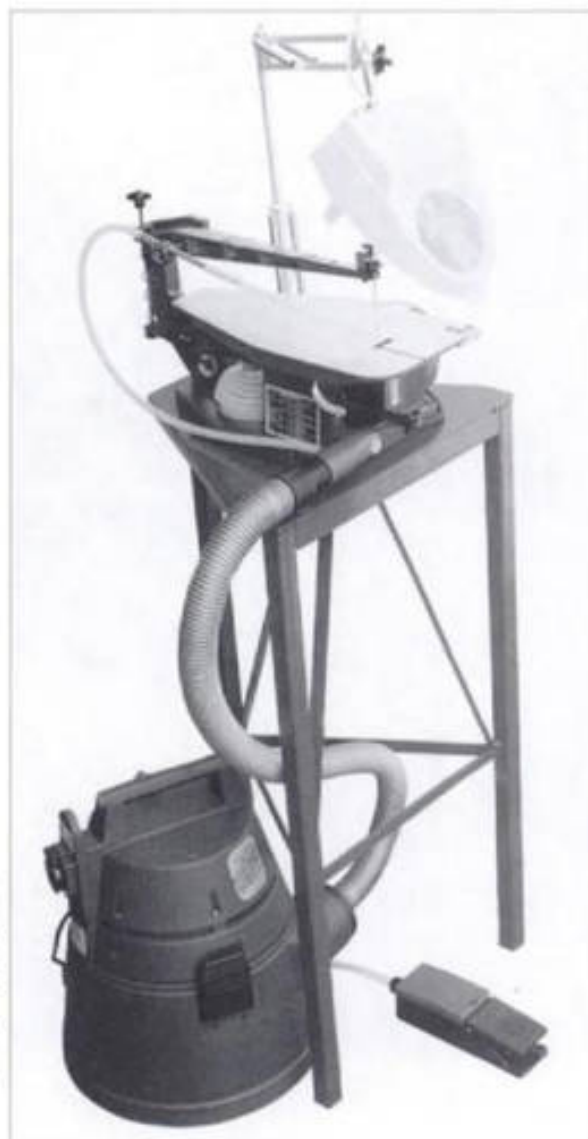
2-85. ► A Hegner saw on the company's typical floor stand. This saw is shown with Hegner's dust-extraction accessory, which pulls sawdust from the top of the workpiece and from under the table. A single-action foot switch controls the vacuum and machine.
