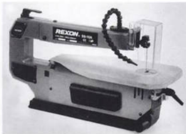
2-120. ► Rexon's single-speed 16-inch scroll saw cuts at 1,450 strokes per minute, has a 2-inch thickness-cutting capacity, and will accept both pin- and plain-end blades.
