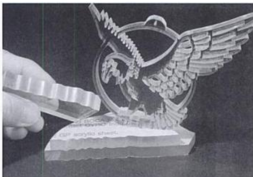
19-1. ▶ Cuts in acrylic plastic. Shown are a \frac{3}{8} -inch-thick eagle sawn by Bill Pickens, test cuts on a single \frac{1}{2} -inch-thick piece, and two \frac{3}{8} -inch stack-cut pieces. Notice that all sawn edges have near-polished surfaces.
