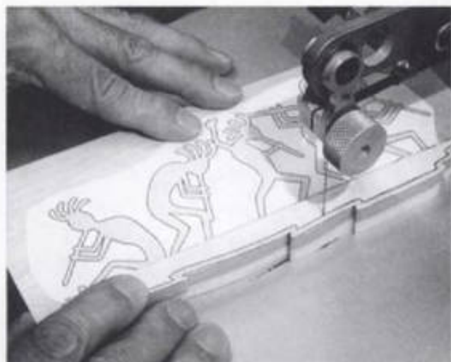
13-25. ▶ With the workpiece rotated end-for-end, the second bevel on the inlay and the background edges are cut simultaneously.
