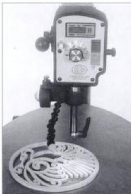
2-58. ▶ The up-front control panel includes a timer that starts and stops as the saw is turned on and off. Also included on the control panel are a light switch (left), the variable-speed control (center), and the power switches (right).
