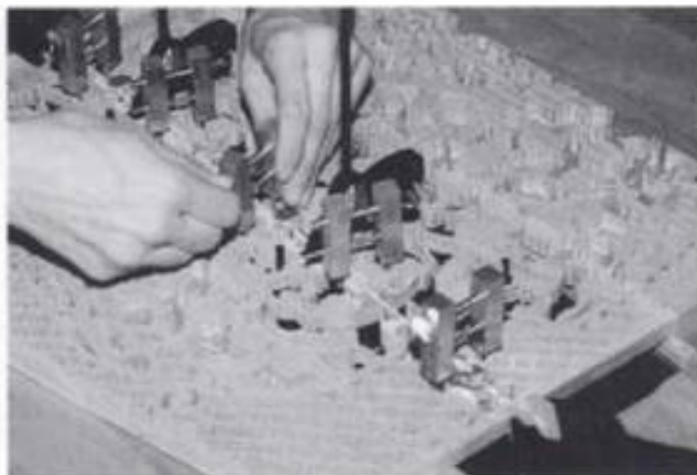
16-49. ▶ Clamping is done on a piece of plywood over an opening to provide access for the clamps and allow inspection from both sides. Specially made clamps are used to produce pinpoint pressure where needed.
