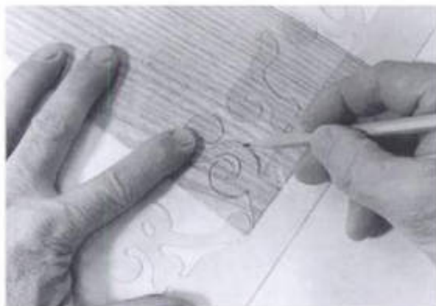
14-16. ▶ The inlay design is laid out on the selected veneer.
