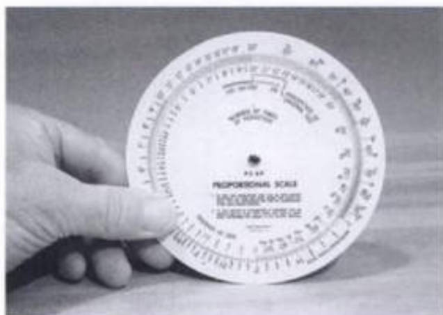
7-15. ▶ A proportional scale consists of two discs with a common pivot. Scaled divisions are marked around the outside of each disc.
