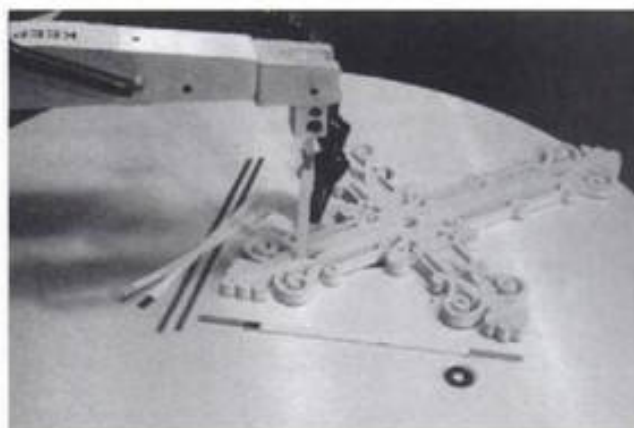
3-23. ▶ Super Sanders from Jim Dandy Products are available in \frac{1}{8} -, \frac{1}{4} -, and \frac{3}{8} -inch widths and grits between 100 and 300. They mount into the blade clamps of scroll saws like plain-end blades.
