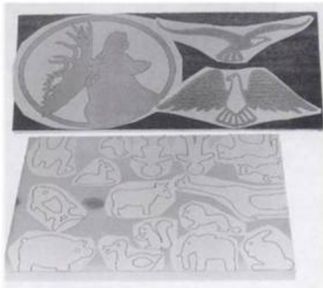
7-46. ▶ Work ready for sawing. Above: Patterns arranged so the longest dimension runs with the grain. Below: Small cutouts arranged around knots and positioned so that the bottom edges of the pattern are aligned to the straight edges of the board.
