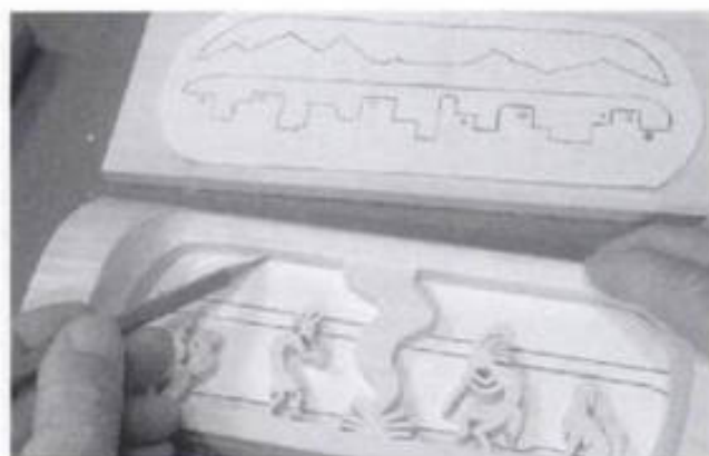
23-32. ► The window silhouette is used as a pattern to make the perimeter cut of the second silhouette layer.
