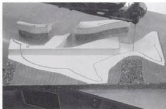
19-22. ▶ The double-thickness inlay areas are cut before the outside profile.
