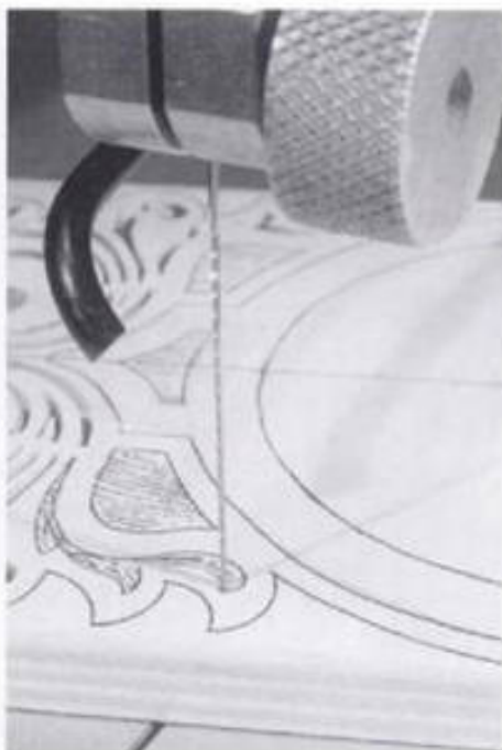
5-32. ▶ Scroll-saw blades spray-painted bright, fluorescent colors are easier to see and help you cut more accurately.
