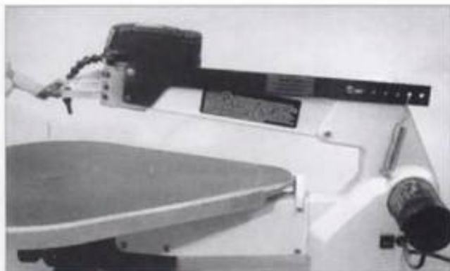
3-10. ▶ The Easy Lift arm lift by Jim Dandy Products works with a spring (shown at the rear).
