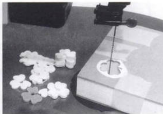
21-7. ▶ Pierced design completed with a No. 4 skip-tooth blade. Notice the smooth walls of the cut.
