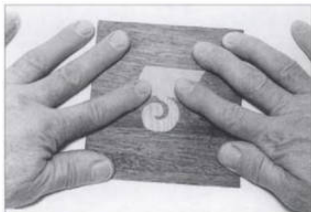
14-22. ► The inlay is set into the background and secured with veneer tape applied to the front surfaces.
