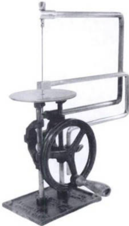
1-40. ➤ Shown here is the first scroll saw manufactured by Herbert Tautz in Milwaukee, Wisconsin, who eventually expanded the company to create the Delta Power Tool Company. The frame carrying the blade moves up and down with the operation of the hand crank. The lower frame is a hold-down that is adjustable to stock thickness.
