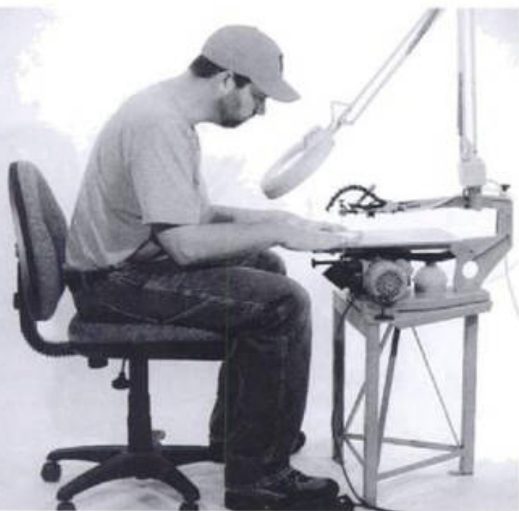
3-2. ▶ General accessories shown in use include a round, fluorescent magnifier light and foot switch; Hegner's chair-height (20-inch) floor stand and lamp bracket; and an aftermarket adjustable sawdust blower from another manufacturer.
