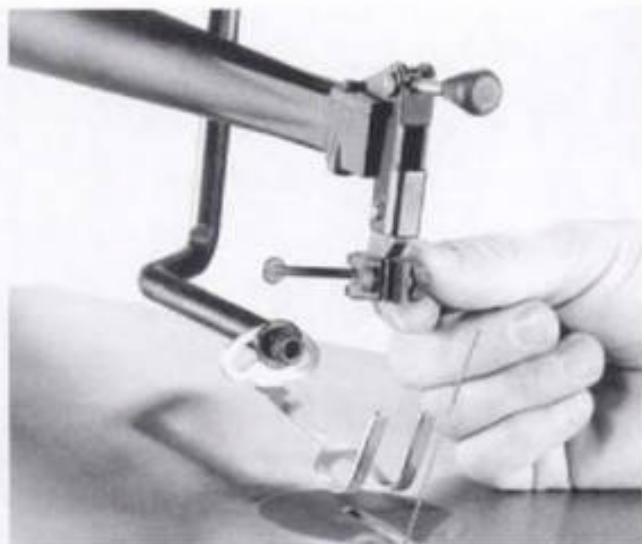
2-37. ▶ The finger-operated locknut changes the blade-clamp opening to accommodate blades of various thicknesses.
