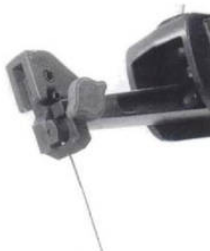
2-9. ▶ The blade clamps on the Sears saws feature toolless, side-by-side pin- and plain-end blade-mounting provisions.
