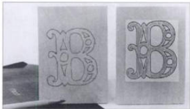
7-35. ▶ The pattern traced freehand with graphite paper at left is not as true or perfect a cutting guide as is a photocopy applied directly to the wood with spray adhesive, as shown at the right.
