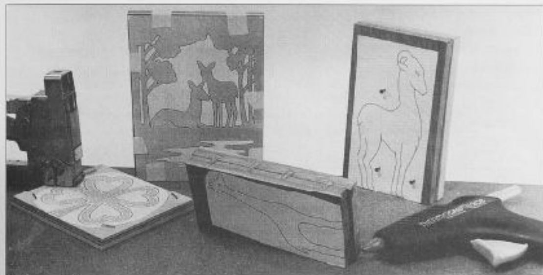
9-7. ▶ Some ways to hold layers of wood together for stack-cutting. From left to right: staples, tape, beads of hot-melt glue on the edges, and brads or nails.
