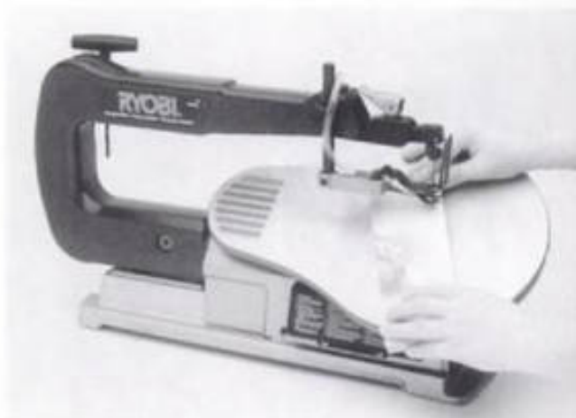
2-126. ▶ Bevel-cutting on a Ryobi saw. Adjusting the hold-down and guard for this type of work can be troublesome.
