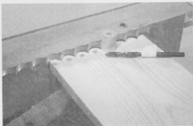
18-50. ▶ Setup for drilling the pin holes. A center-drilled \frac{3}{4} -inch-diameter dowel held cradled against the template locates each hole, and the tape on the bit gauges the hole depth.
