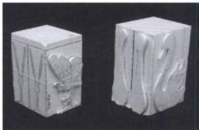
11-14. ▶ Material prepared for stack-cutting three-dimensional shapes. Notice the double pattern applied to one surface.
