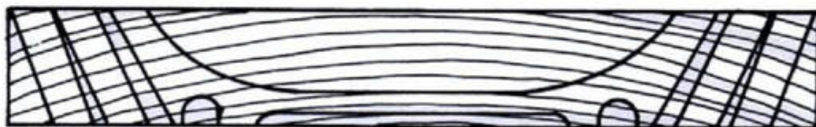
12-44. ▶ The edge-view cutting plan for the bowl shown in 12-43.
