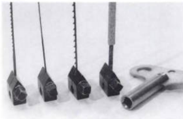
5-36. ▶ In some cases, it saves time and is convenient to have extra blade clamps "preloaded" with frequently used blades to speed blade changes.
