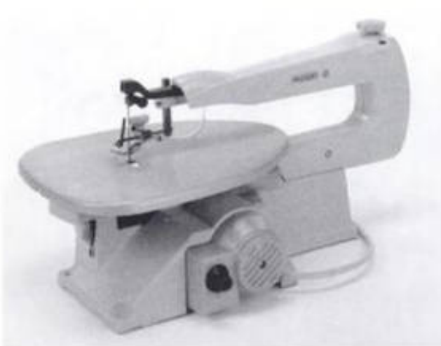
2-121. ► This variable-speed Ridgid machine is one of the few 16-inch bench-top scroll saws made in the United States.
