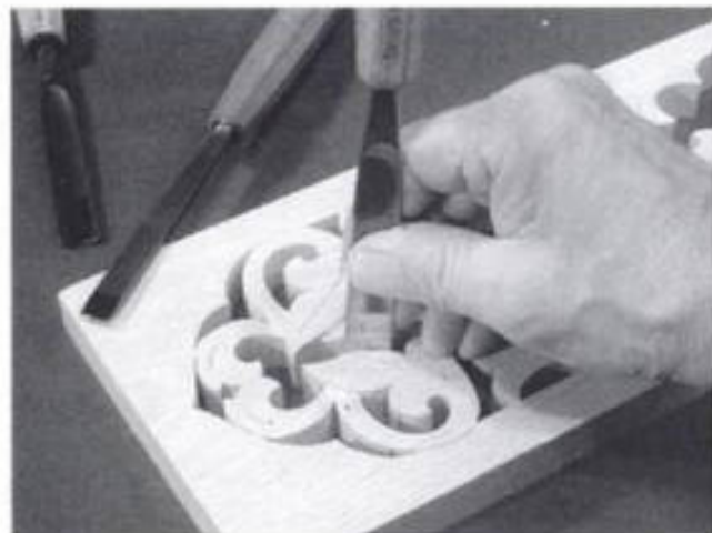
16-29. ▶ First, make vertical stopped cuts to sever the grain fibers.
