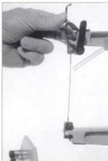
2-101. ▶ The blade-suspension system shown with the table removed for visual clarity. The blade-tension lever, which looks like an Allen wrench, is partially visible above the upper blade clamp.
