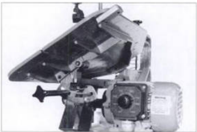
2-77. ▶ View showing the Hegner table tilted left and the combination switch and variable-speed control at the right.
