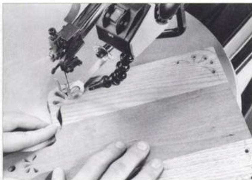
2-32. ► Making inside cuts on Delta's Q-3 saw. Notice the up-front controls.
