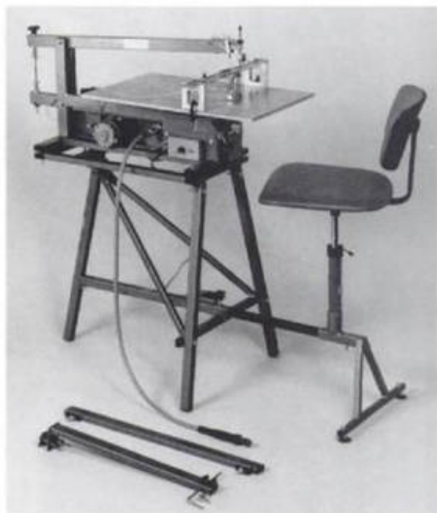
2-49. ▶ The Diamond 24-inch heavy-duty, variable-speed scroll saw, made in England, has a 3-inch cutting capacity and many unusual features and uncommon accessories such as the "tool bridge" shown attached to the table. This "bridge" acts as a hold-down and also ensures perfect blade alignment.
