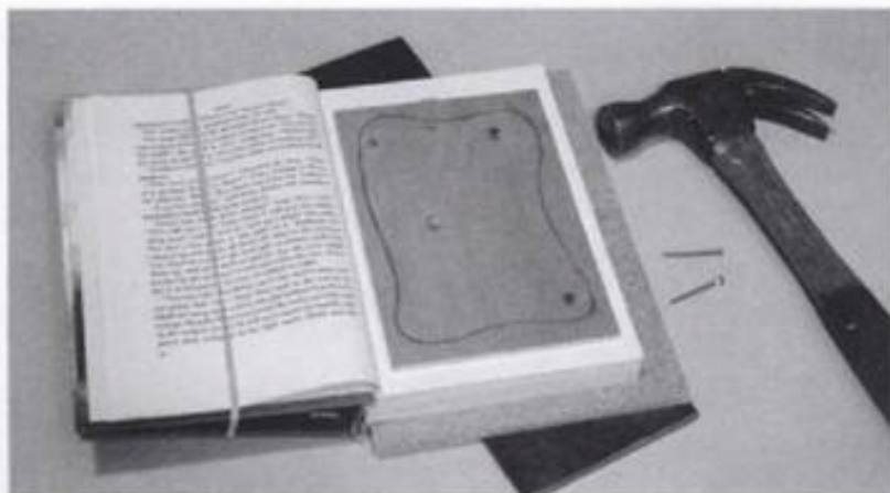
21-4. ▶ Two pieces of thin waste plywood are nailed together (over a metal plate) with the book pages sandwiched in between.
