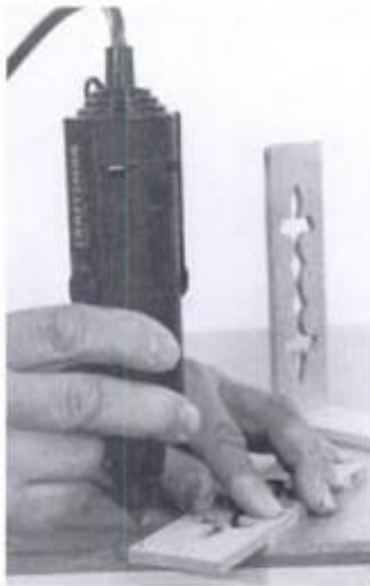
16-16. ▶ Using a high-speed rotary tool to drill pilot holes in hardwood for a butt-joint assembly nailed together with brads.
