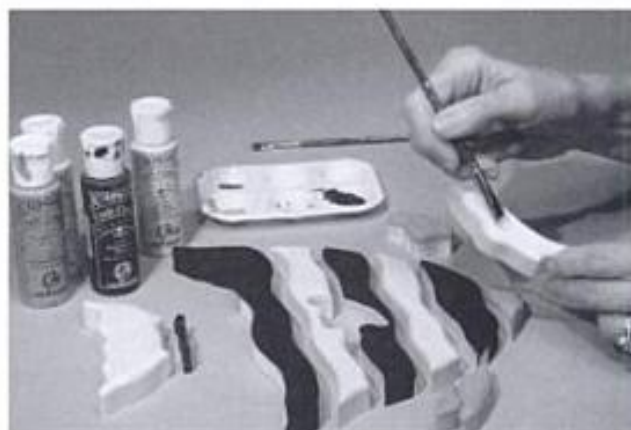
22-11. ▶ Acrylic paint is applied to all visible and non-gluing surfaces of the individual pieces.
