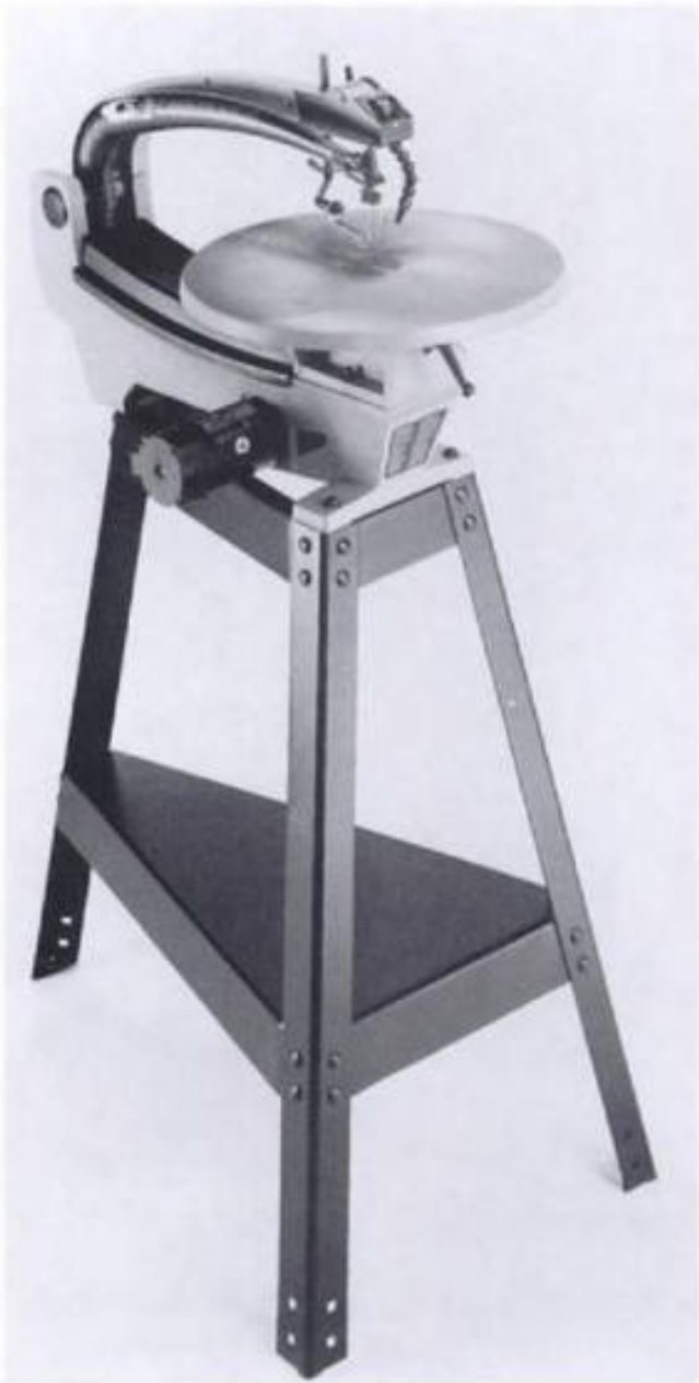
2-31. ▶ Delta's 18-inch, C-arm, variable-speed scroll saw has a more aggressive cutting action than Delta's other parallel-arm saws.
