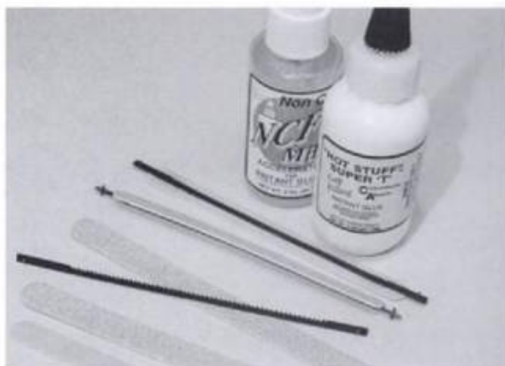
3-27. ► Glue emery boards to dull saw blades to make your own scroll-saw sanders.
