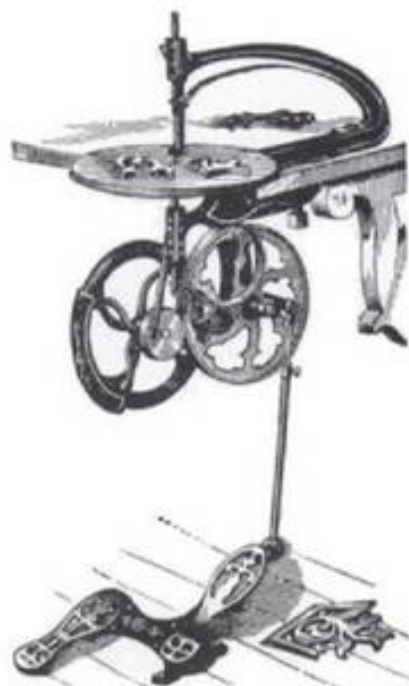
1-19. ▶ The bench-mounted, foot-powered Fleetwood scroll saw, patented in 1872, was claimed to be the best for delicate and accurate fret-sawing. It had unique, guided blade clamps, a 14½-inch throat, and could cut stock ¾ inch and under rapidly.
