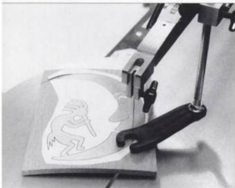
I-18. ▶ RBI's hold-down is made of a plastic that flexes with changing material thickness such as when cutting warped material as shown.
