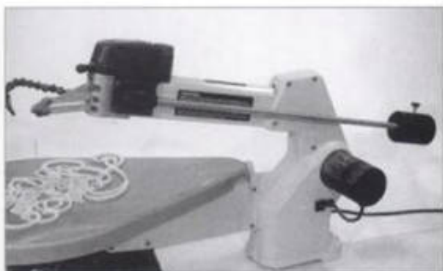
3-11. ▶ The Scroll Buddy arm-lift system by Best Wood Tools Corp. uses a heavy counterweight.
