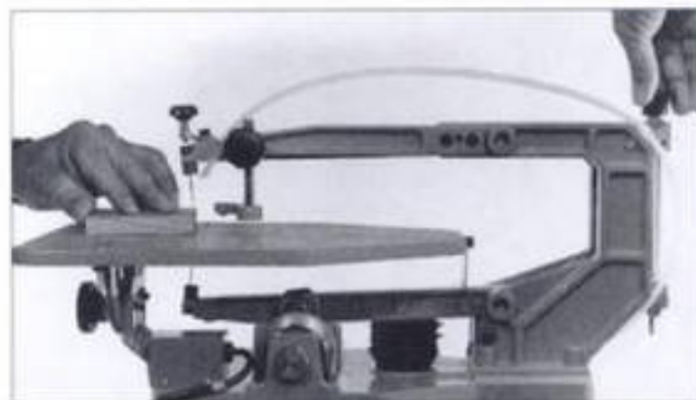
8-3. ► Checking blade tension (with the power off) by exerting moderate pressure against the front of the blade. Medium-to-large blades should deflect \frac{1}{8} to \frac{1}{16} inch.
