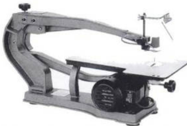
2-74. ▶ The Grizzly model G1060 scroll saw is a 22-inch, C-arm saw and has a table that tilts only up to 30 degrees.
