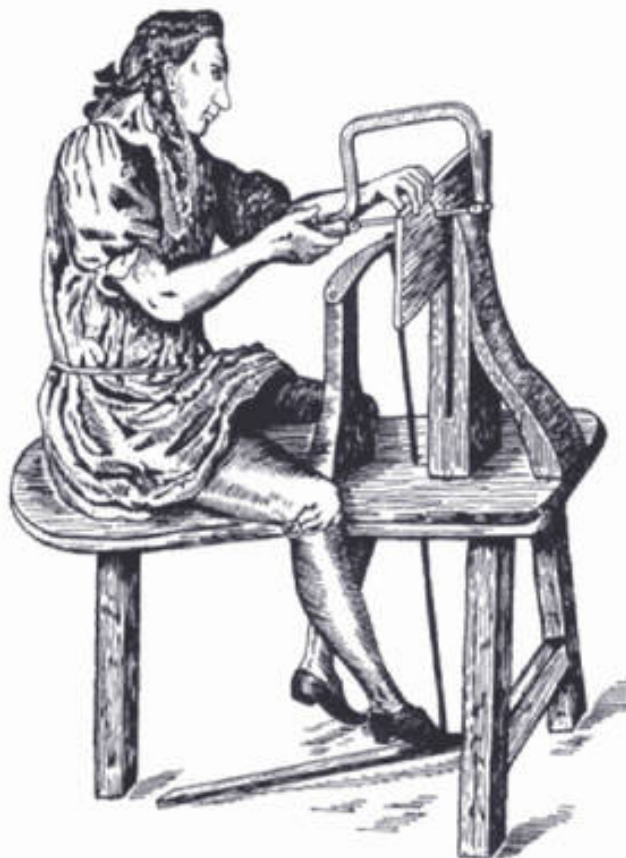
1-4. ▶ Buhl sawing circa 1775. The work is held vertically with the foot-operated clamp of this "Buhl Horse." Sawing was done with a push stroke.
