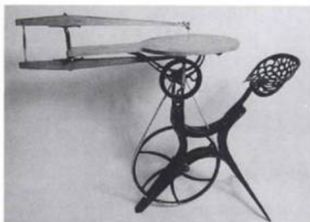
2-133. ▶ Cast-aluminum reproduction of the Barnes No. 2 Velocipede scroll saw manufactured by The Tool Company.
