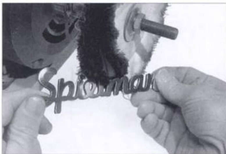
20-16. ► Buffing polishes surfaces and softens sharp edges.
