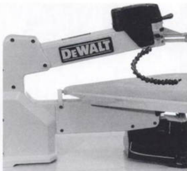
2-42. ▶ The upper arm lifts, which makes blade threading easy. It can be done by inserting the blade through the workpiece either from the bottom up or top down as desired.
