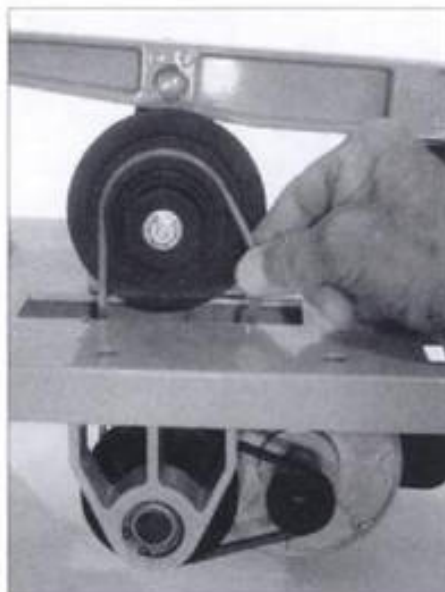
2-98. ▶ Speed change is made by shifting the flexible round belt to a new combination of pulley sizes.
