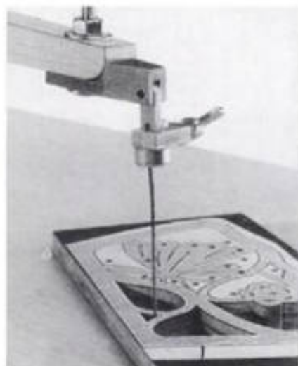
2-132. ▶ The time tested, toolless blade clamp is standard on The Tool Company's motorized scroll kit and its Velocipede Reproduction saw, shown in 2-133.
