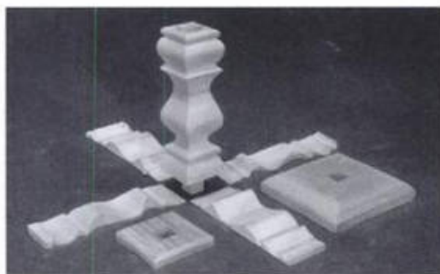
11-11. ▶ Sawing completed for the candlestick spindle. Also shown is the waste cut from each surface and the two extra square pieces prepared for the base.
