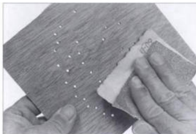
8-33. ► Removing exit-side grain tear-out or splintering to ensure the workpiece will rest flat on the saw table.
