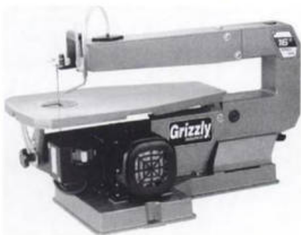
2-71. ▶ The Grizzly model G7949 saw carries only pin-end blades and is one of the lowest-priced 16-inch saws available.
