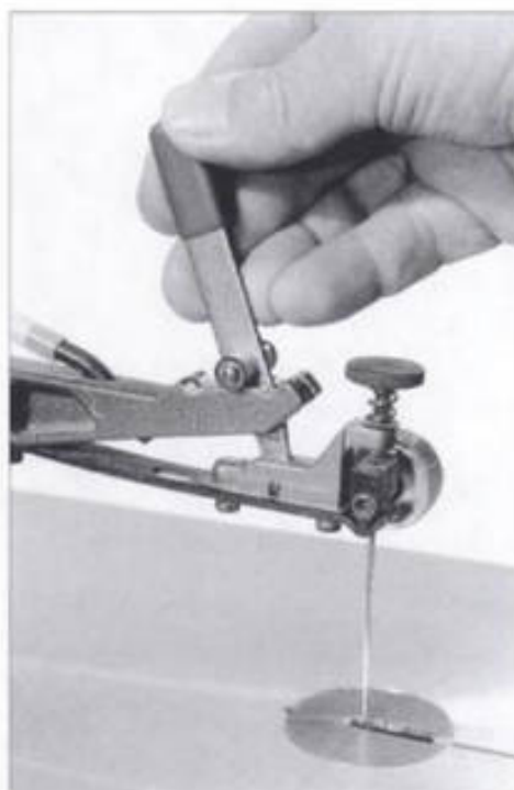
2-87. ► The Hegner 18- and 22-inch saws come with this up-front tension-release lever. Notice the knife-edge blade clamps and the finger-controlled knob visible on the right of the upper blade clamp (an optional accessory for all saws).
