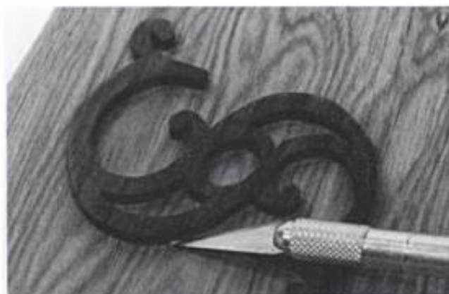
17-13. ► Carefully remove any glue “squeeze-out” after it sets, but before it cures hard.
