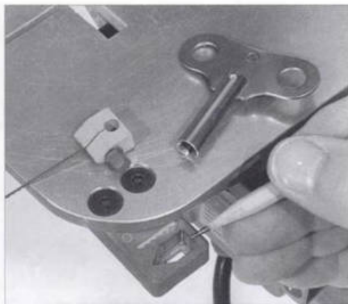
2-88. ► Installing a blade in the lower blade clamp is done in the fixture attached to the saw table.
