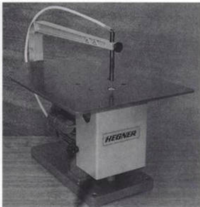
2-81. ► Hegner UniMax with upper arm installed for maximum blade support.
