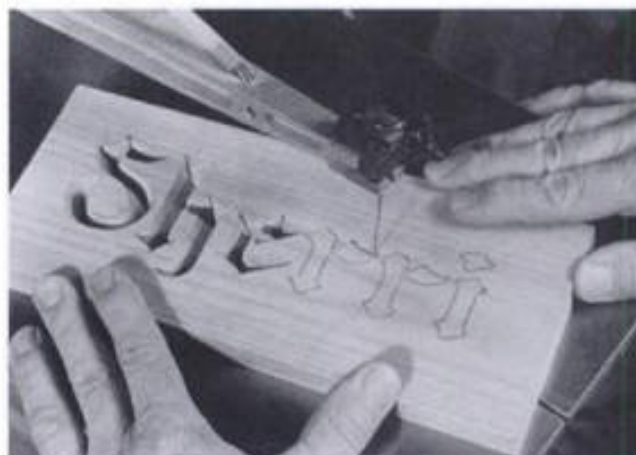
15-17. ▶ Another example showing the counterclockwise feed for cutting a letter "r." At this outside corner, a near full 360-degree on-the-spot, clockwise turn will be made before continuing.
