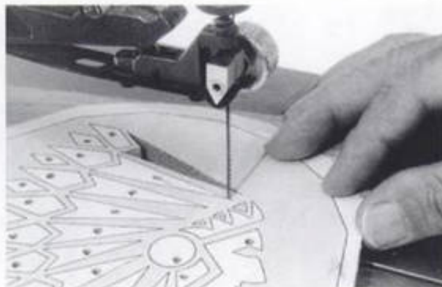
8-44. ▶ Saw along one “leg” of the angle, all the way to the point or corner.
