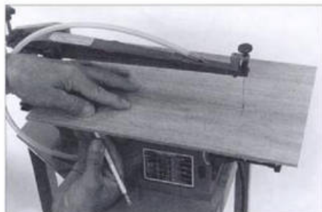
10-8. ► Making a reusable zero-clearance auxiliary table that can be quickly put on or removed. Using \frac{1}{8} -inch or thicker oversized plywood, saw inward; then stop and mark the table shape all around the underside, as shown here.
