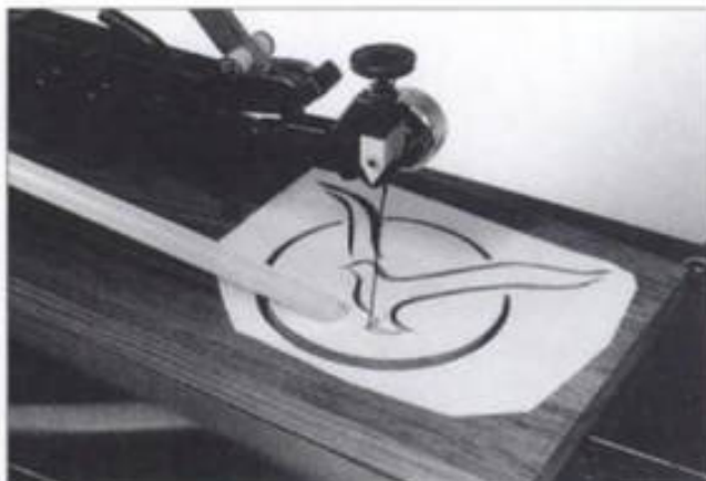
8-30. ▶ Sawing narrow inside openings.
