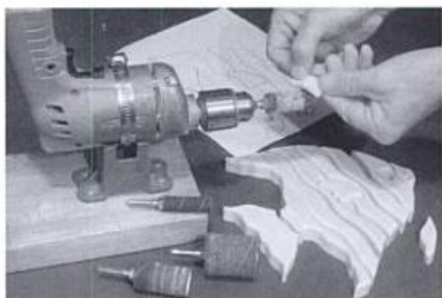
22-7. ▶ Rounding and shaping the edges of the individual pieces with a drum sander.
