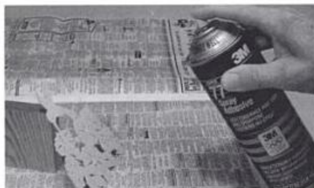
17-16. ► Direct the spray of the aerosol adhesive at a right angle to the surface of an overlay to minimize any glue buildup of adhesive at the edges.
