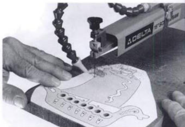
6-3. ▶ A shop-made system that, like many of the newer adjustable sawdust blowers, directs dust particles away from the operator.
