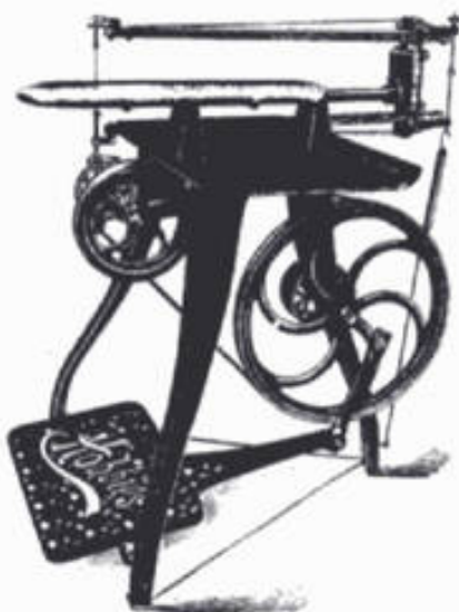
1-31. ▶ The British Norfolk, introduced in 1904, featured a speed control using a system of small and large pulleys. This machine could also be power-driven from line shafts.
