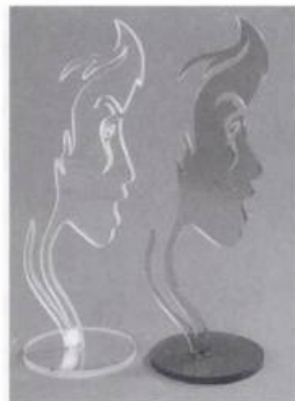
19-7. ▶ Left: Clear acrylic. Right: Tinted polycarbonate. Under the same conditions, the acrylics cut smoother and are less expensive, but are more brittle.
