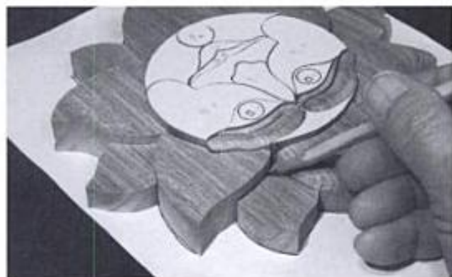
22-9. ▶ Shape (round over) the edges of the lower pieces first. Then mark higher adjoining pieces to facilitate contouring. Notice that not all edges are rounded over.
