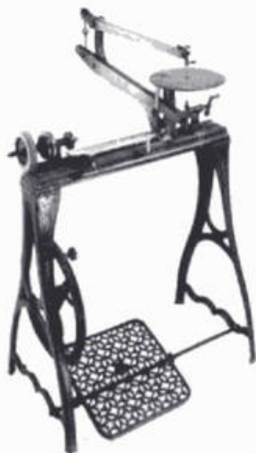
1-29. ▶ The British-made Goodell Scroll Saw and Lathe Combination shown here appeared in 1887 and remained in production for more than 60 years. Notice the grinding wheel and horizontal drill on the left.
