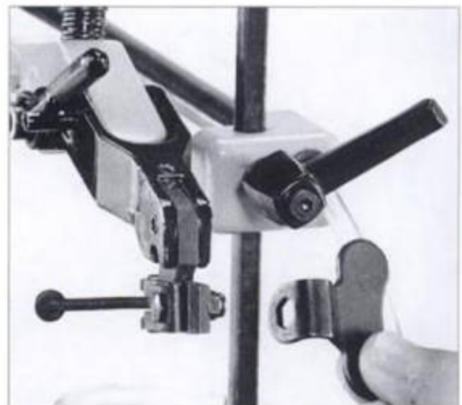
2-19. ▶ Blades of different thicknesses require an adjustment to the opening size and clamping action of the blade clamp. This special wrench turns a locknut on the right of the blade clamp that tightens or loosens the clamping action.
