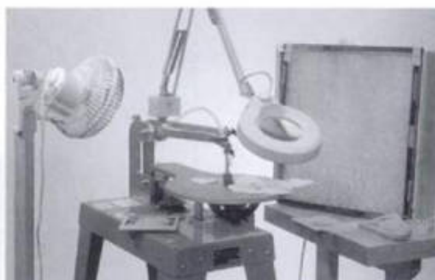
6-11. ► A double-fan setup creates an airflow that carries dust to the furnace filter taped to the larger, square household fan at the right.
