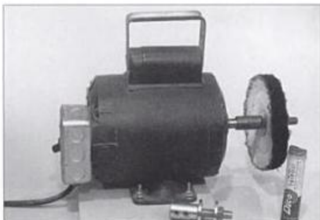
20-14. ▶ An old electric motor converted to a buffer consists of a cotton buffing wheel on a threaded motor-arbor adapter that fits onto the motor shaft.
