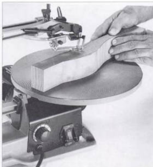
9-5. ▶ Sawing thick wood with the grain such as this is generally much slower than crosscutting and cannot be forced. Use a high speed, a coarse blade, and a perceptive feed rate.
