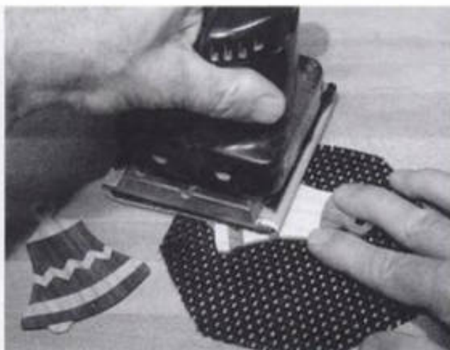
3-40. ▶ A small finishing sander used to level and smooth a segmented ornament.
