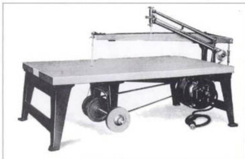
1-36. ▶ This 1927 Barnes electrified scroll saw had a 24-inch throat, a 7-inch blade, and a \frac{1}{4} -horsepower motor. It suffered in competition with other brand saws such as Delta, which featured cast-iron, rather than wood, tables.
