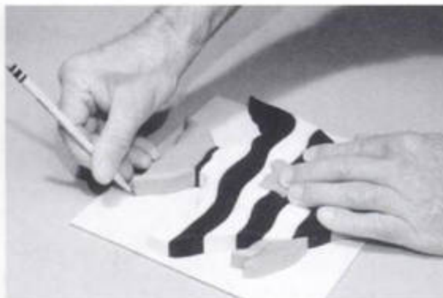
22-13. ▶ Tracing the perimeter for the thin plywood backing.
