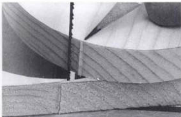
8-20. ▶ When the cut comes around to the starting point, a small dimple may remain as shown.
