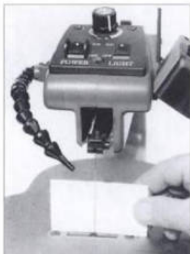
4-8. ► Visually check the blade for side-to-side wobble by holding a light paper (business card) behind the blade with the power on.
