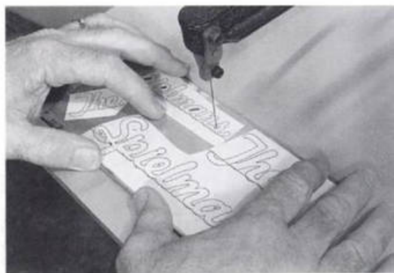
23-24. ▶ Sawing 1/8-inch solid brass.
