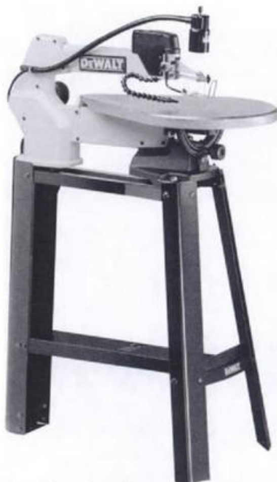
3-3. ▶ Special DeWalt scroll-saw accessories shown here are a work light with a flexible neck and a floor stand. The stand has a rear leg-height adjustment that, when elevated, tips the saw toward the operator for more comfortable operation.
