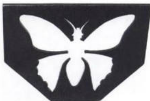
20-8. ▶ Detail cut into 1/4-inch steel plate with a Hegner saw.
