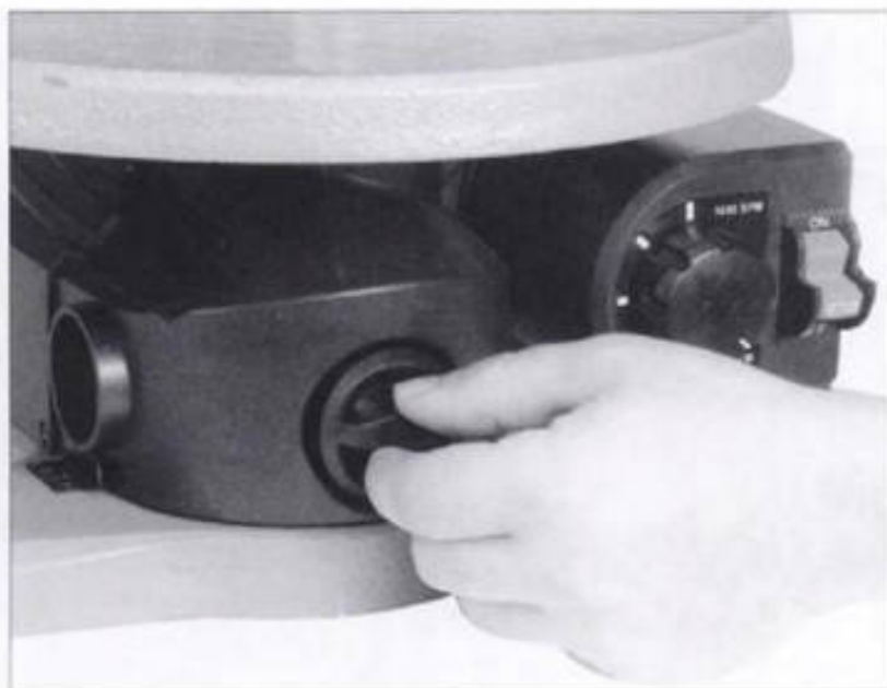
2-26. ▶ This knob must be released to remove the "dust cup" (box), which is necessary when installing a new blade into the lower clamp or accessing the table-tilt lock handle.
