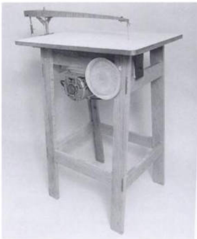
2-130. ▶ A do-it-yourself saw made from a kit provided by The Tool Company. Notice how some of the components are the same as those of the Velocipede Pedal Saw shown in 2-132 and 2-133. The 8-inch disc sander shown is an optional accessory.
