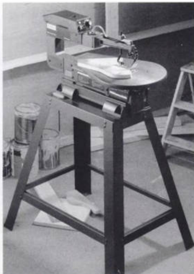
2-8. ▶ The Craftsman Professional 20-inch floor model with its variable-speed control located up front.
