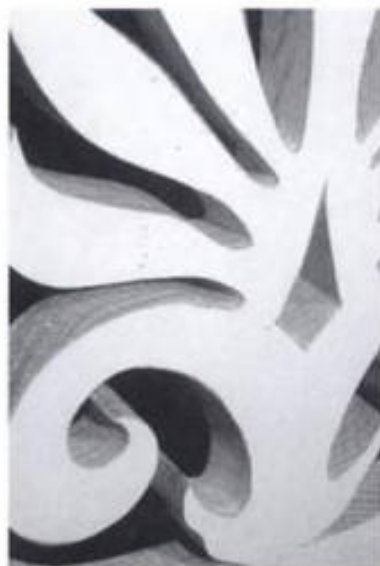
16-25. ▶ Ground blades can be used to produce clean, smooth cuts even in tight turns with \frac{3}{4} -inch oak right off the saw.
