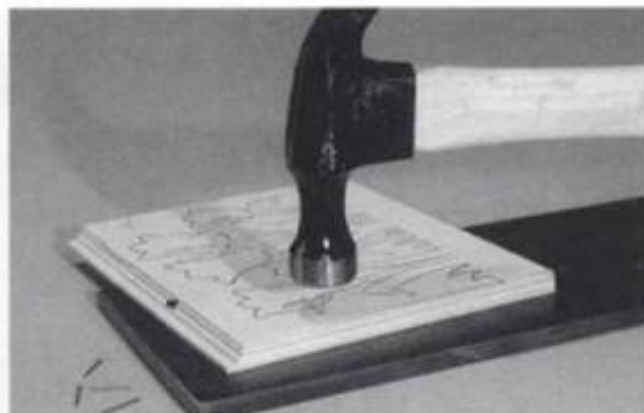
9-10. ▶ A flat piece of steel placed under the stack of four \frac{1}{16} -inch layers of plywood will flatten points of brads or nails when they are driven through the bottom plywood layer.
