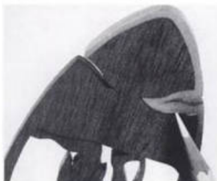
13-4. ▶ A glue-filled kerf may be visible along some of the inlay's edges when employing the vertical stack-cutting inlaying technique.
