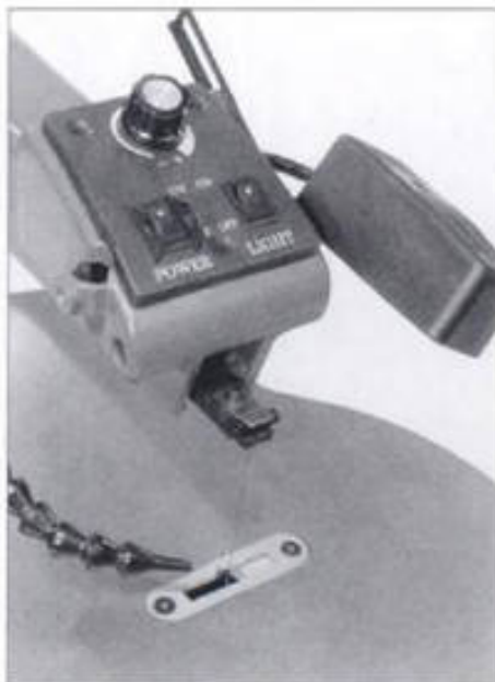
2-138. ▶ The lower blade clamp is only accessible from the left side and requires a T-handle Allen wrench.
