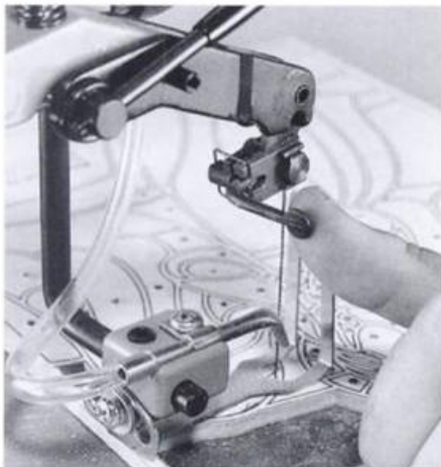
2-18. ▶ Releasing the upper blade clamp. Notice the tension lever above in release position. Also shown here is a close-up of the hold-down and the nonadjustable sawdust blower.
