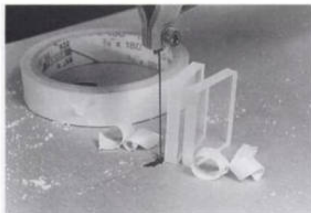
19-6. ▶ A close-up look at the pieces sawn in 19-5. Notice that they have cleaner cut surfaces than the plastic cut in 19-3 and 19-4. They are, however, not as smooth and as polished-looking as they can be (refer to 19-1).
