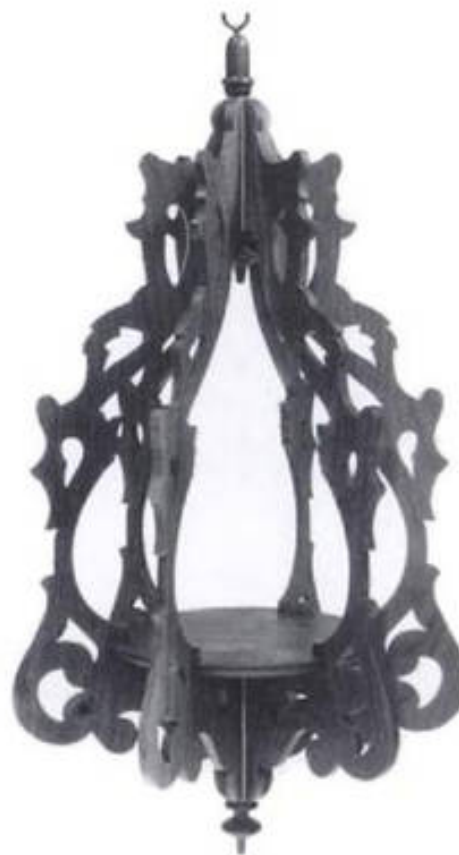
9-3. ▶ Cutting the six identical parts for this hanging plant holder all at once is essentially six times faster than sawing the pieces one at a time.
