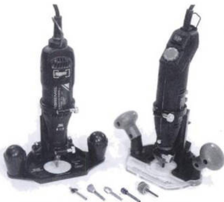
3-32. ▶ Rotary tools, when used with a router-base accessory, are ideal for rounding the edges of small scroll-saw work.
