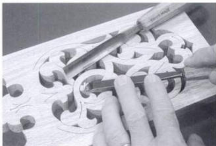
16-30. ► Make slicing cuts to taper the thickness of the wood until a depth of \frac{1}{8} inch or more is reached at the deepest point.
