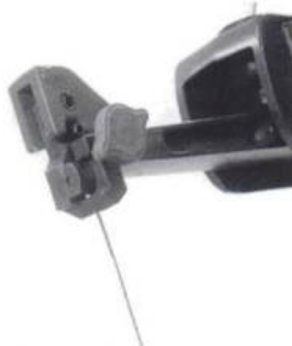
2-9. ▶ The blade clamps on the Sears saws feature toolless, side-by-side pin- and plain-end blade-mounting provisions.
