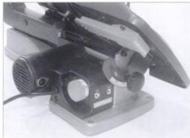
2-13. ▶ View showing the combination push-pull power switch and variable-speed control knobs. Notice the shallow blade-storage drawer located under the table.
