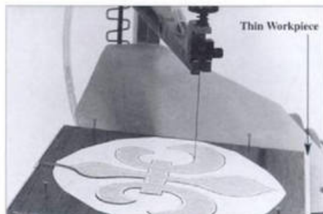
10-10. ► Sandwiching very thin material in between waste plywood as shown provides sawing resistance for better control, and the bottom layer minimizes tear-out.
