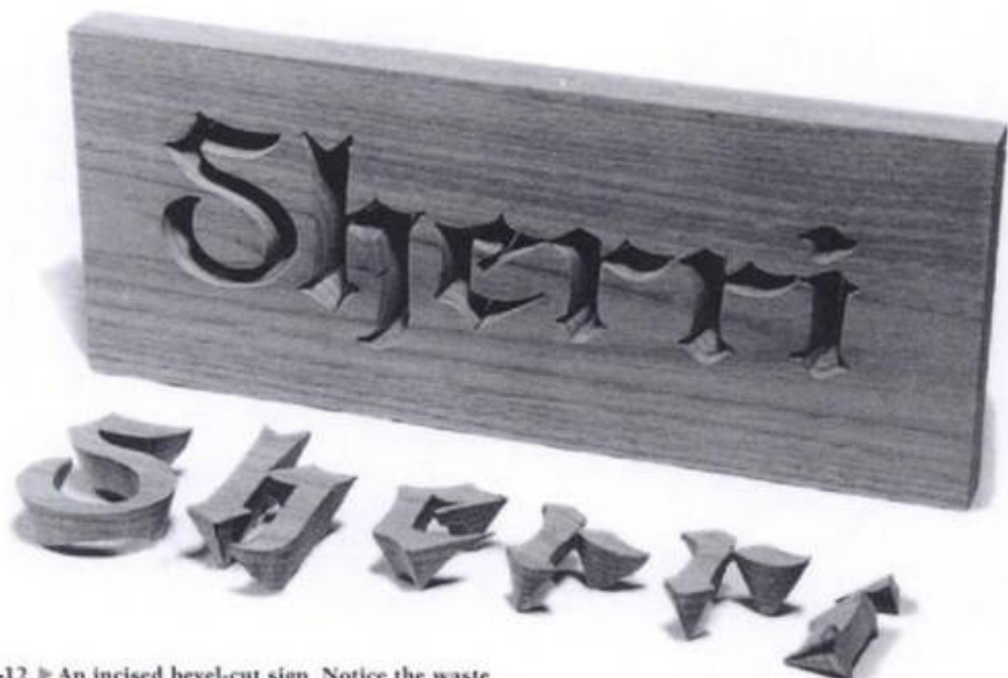
15-12. ► An incised bevel-cut sign. Notice the waste pieces shown in the foreground.
