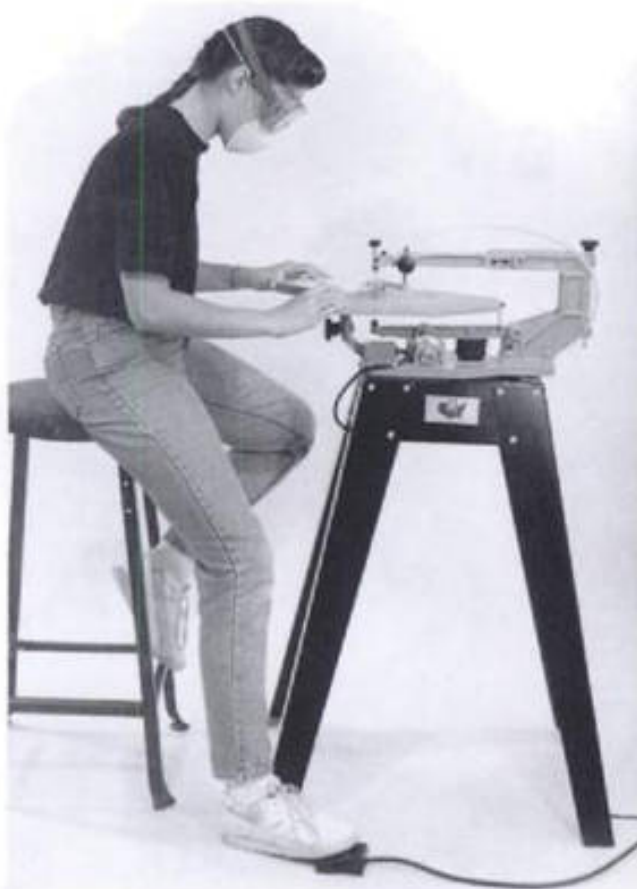
6-1. ▶ A demonstration of good safety techniques: the woodworker's hair is pulled back and her back is straight; there is no loose clothing or jewelry; goggles, a dust mask, a hold-down, and a foot switch are being used; the stool is at a comfortable height; and the work area is clean and well lit.
