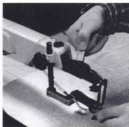
2-94. ► Setting the tension. Notice that the hold-down and guard are attached to the adjustable bracket that holds the dust-blower line.
