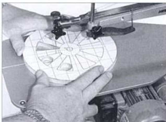
8-23. ▶ Scroll-sawing the straight-line spokes of a plywood wheel.
