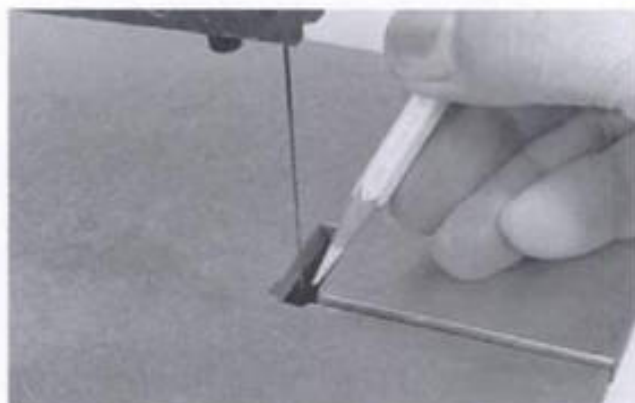
10-4. ▶ The table openings on most saws are too large to safely support sawing thin stock and small parts that may tip or fall through the opening.
