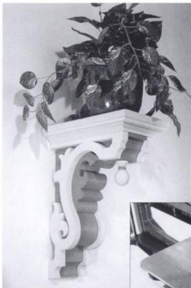
9-14. » Stack-cutting thick layers is an important process for making Victorian gingerbread pieces such as this corbel.
