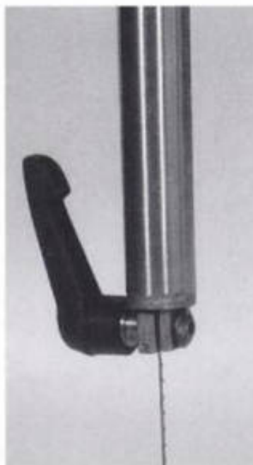
2-61. ▶ A close-up look at the upper blade clamp. Notice the large, multipositionable clamp lever and that the blade is inserted from the rear rather than the front, as done with other saws.
