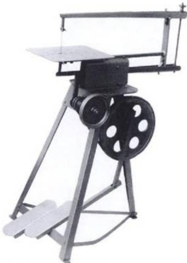
2-89. ▶ This treadle fretsaw, which has all-steel frame construction, is made by Hobbies Limited, in England, and is still available today.
