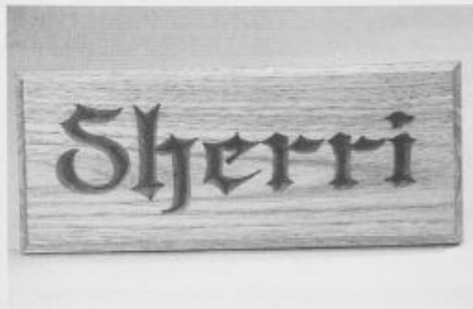
15-2. ▶ A more challenging style of incise-carving is best done using softwood such as this butternut. This technique involves making a number of on-the-spot turns to complete one letter.
