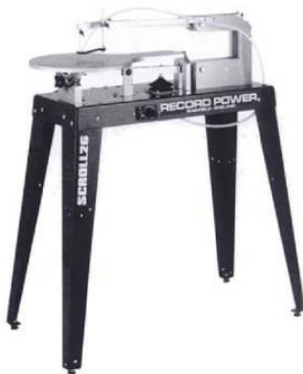
2-112. ▶ Record's 26-inch scroll saw, one of three models available in England manufactured by RBI. (Record also sells a 16- and a 20-inch saw.)
