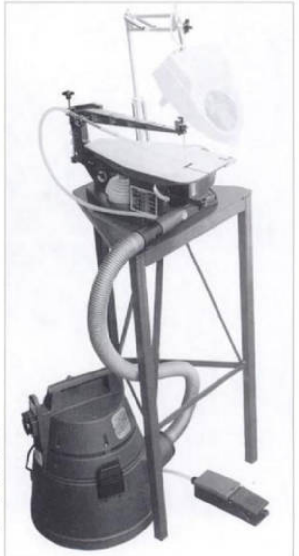
2-85. ► A Hegner saw on the company's typical floor stand. This saw is shown with Hegner's dust-extraction accessory, which pulls sawdust from the top of the workpiece and from under the table. A single-action foot switch controls the vacuum and machine.
