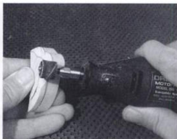
3-33. ▶ Here the rotary tool, with a drum-sander accessory, is used to shape a piece for a segmentation project.
