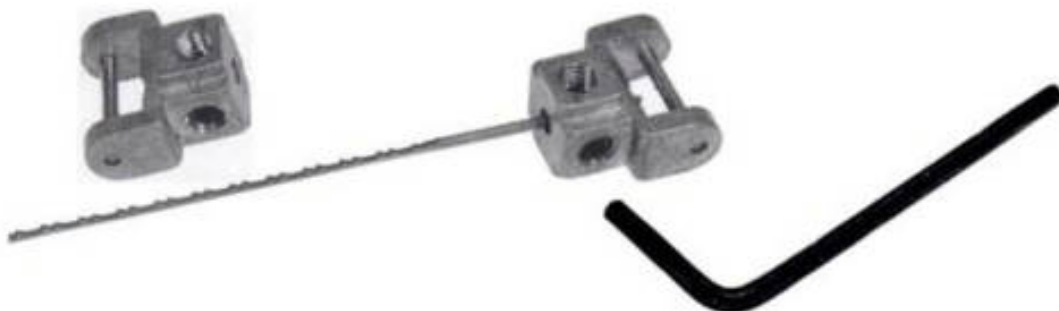
I-15. ▶ The wrench-tightened blade clamps found on older saws and shown here are frustrating and very time-consuming to use.
