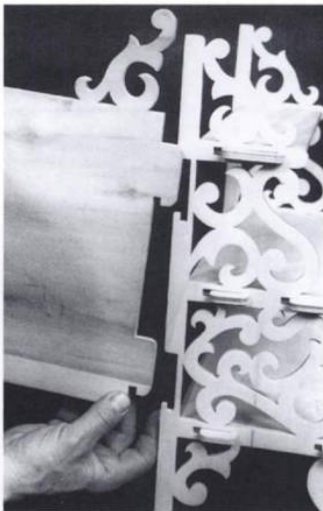
18-7. ▶ A close look shows the "hooks" or "stops" of the tabs and the longer slots that allow the parts to slide and interlock.
