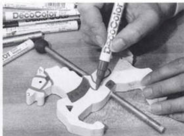
24-7. ▶ Freehand-painting lines using paint pens.
