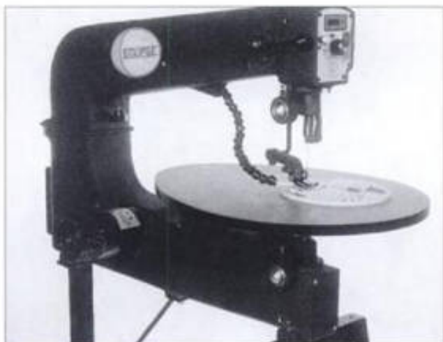
2-37. ▶ At first glance the Eclipse looks like a rigid-arm saw, but inside the hollow C-shaped aluminum housing is a belted oscillating-loop drive mechanism.
