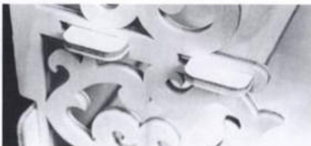
18-8. ▶ A close look at the shelf tabs extending through the slots and then pulled forward to lock in place. The result is a strong joint, but it leaves an undesirable opening behind each tab as shown.
