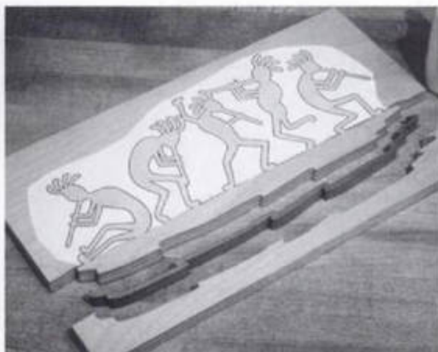
13-26. ▶ The inlay ready to be glued in place and the discarded waste pieces.
