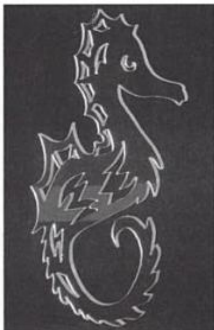
19-15. ▶ One-eighth-inch acrylic cut with a No. 2 crown-tooth blade.
