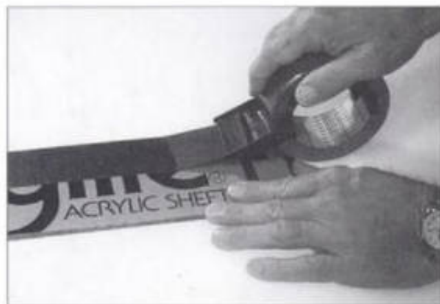
19-8. ▶ Duct tape applied to the top surface either lubricates the blade or keeps the cut particles from reentering the kerf. This prevents the cut from fusing.
