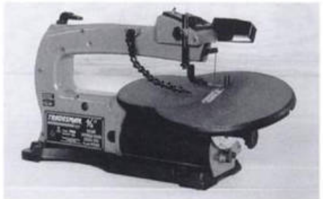
I-17. ► This Tradesman scroll saw and many other saws do not have separate hold-down arms. Instead they have housings that enclose the upper moving arms, protecting the user from accidental injury. Here, the motor and lower moving parts are also well-enclosed. Notice the tension-control lever located at the upper rear and the adjustable air hose.
