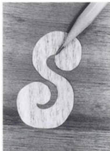
14-24. ► The completed inlay shown enlarged. Notice there is also no trace of the saw kerf or the original blade-threading hole.
