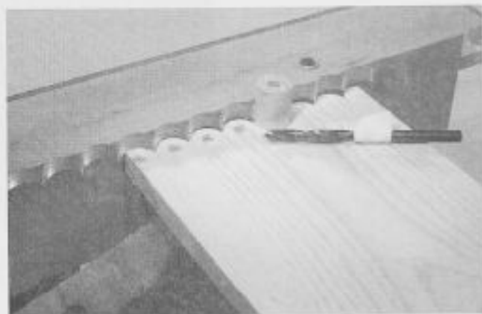
18-50. ▶ Setup for drilling the pin holes. A center-drilled \frac{3}{4} -inch-diameter dowel held cradled against the template locates each hole, and the tape on the bit gauges the hole depth.
