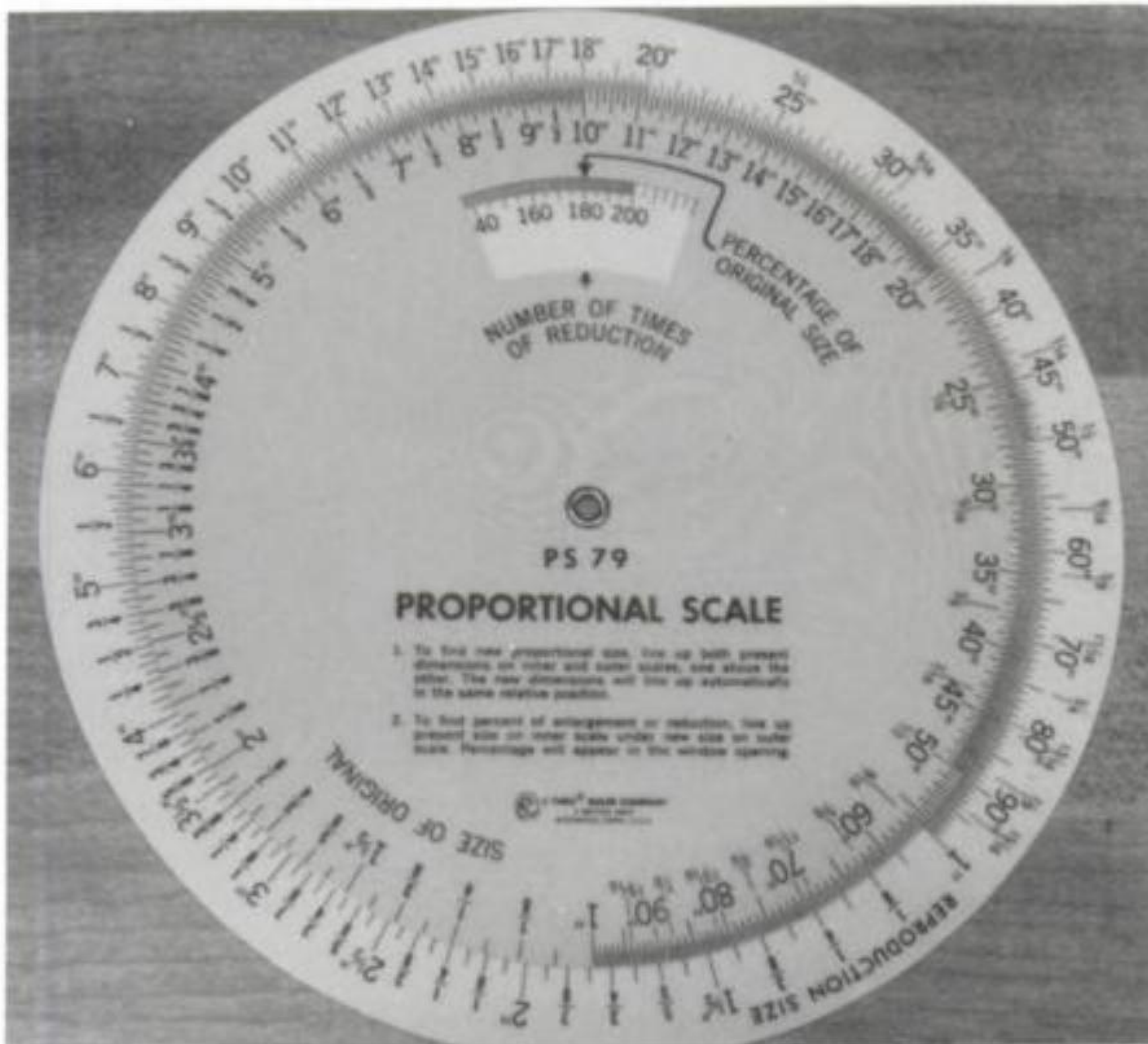
Illus. 1. An inexpensive proportional scale, such as the one shown here, makes enlarging or reducing patterns to a specific size with a photocopy machine quick and precise. It actually tells you what percentage to set the photocopy machine at to get a pattern of a predetermined size.
