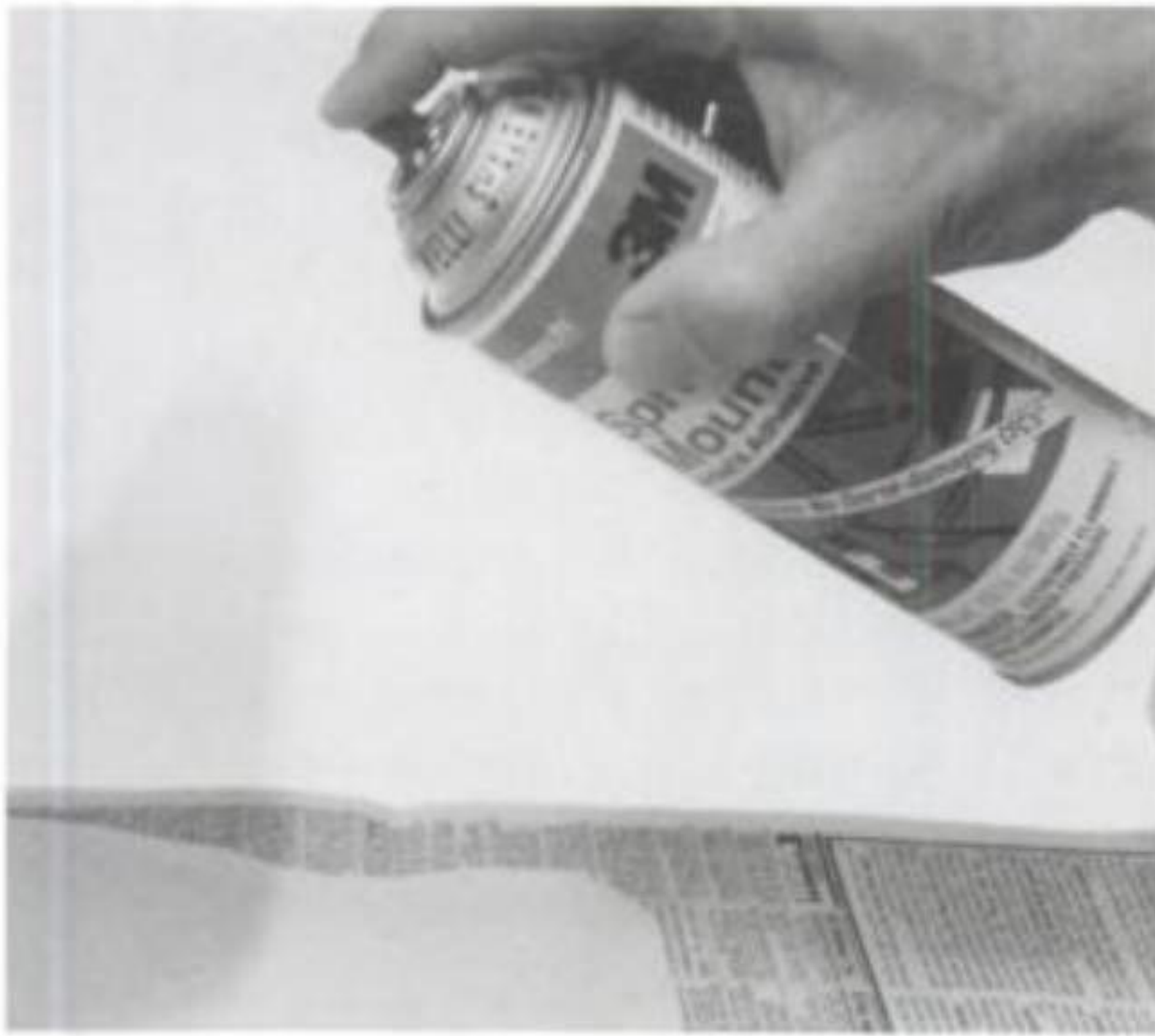
Illus. 3 (left). An aerosol temporary-bonding adhesive is used to coat the back of the pattern. Note that the pattern is cut to a rough size and newspaper catches the overspray. Illus. 4 (right). After you've finished sawing, remove the pattern. The paper should peel off easily without sticking or leaving any residue on the wood surface.
