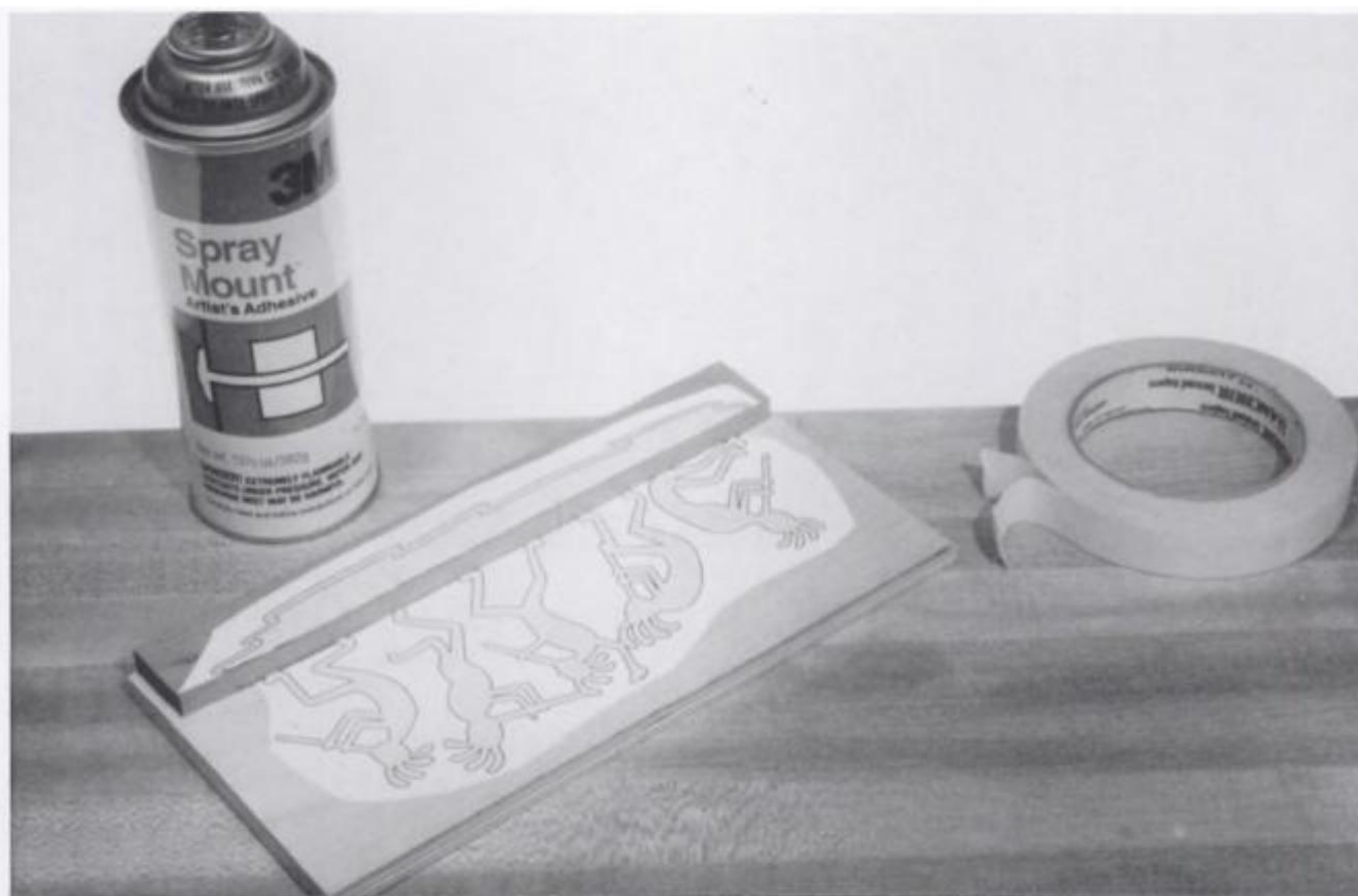
Illus. 19. Step 1. This step involves preparing the inlay and workpiece background for simultaneous bevel sawing. Here, 3/8" redwood is positioned on top of 3/8" Baltic birch plywood and secured with small pieces of double-faced tape. Note that the pattern copies are applied to both pieces with temporary-bonding spray adhesive.
