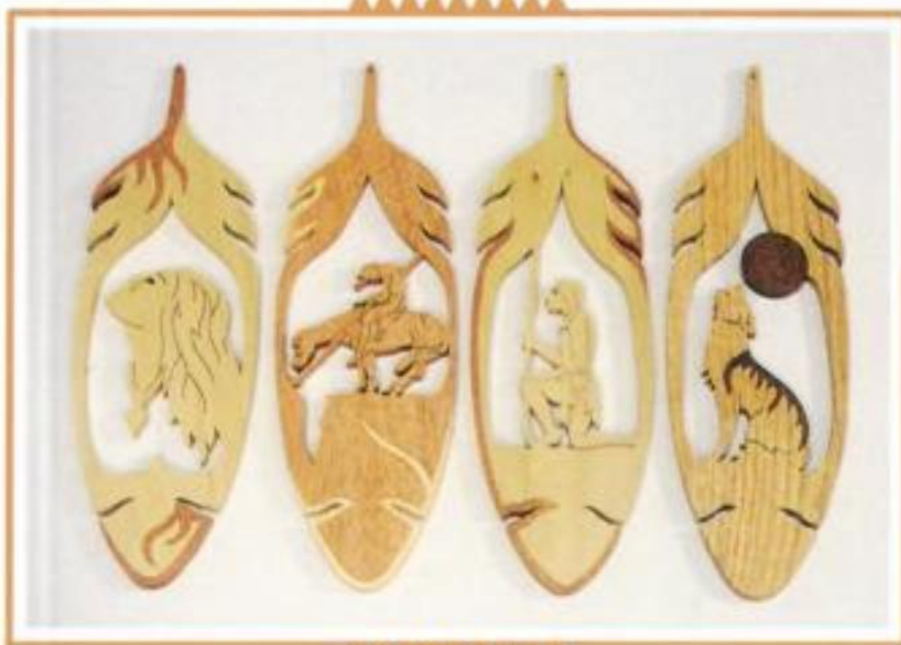
Feathers of \frac{1}{4} -inch hardwood with contrasting inlays created by the stack- or pad-sawing technique (pages 127–130).
