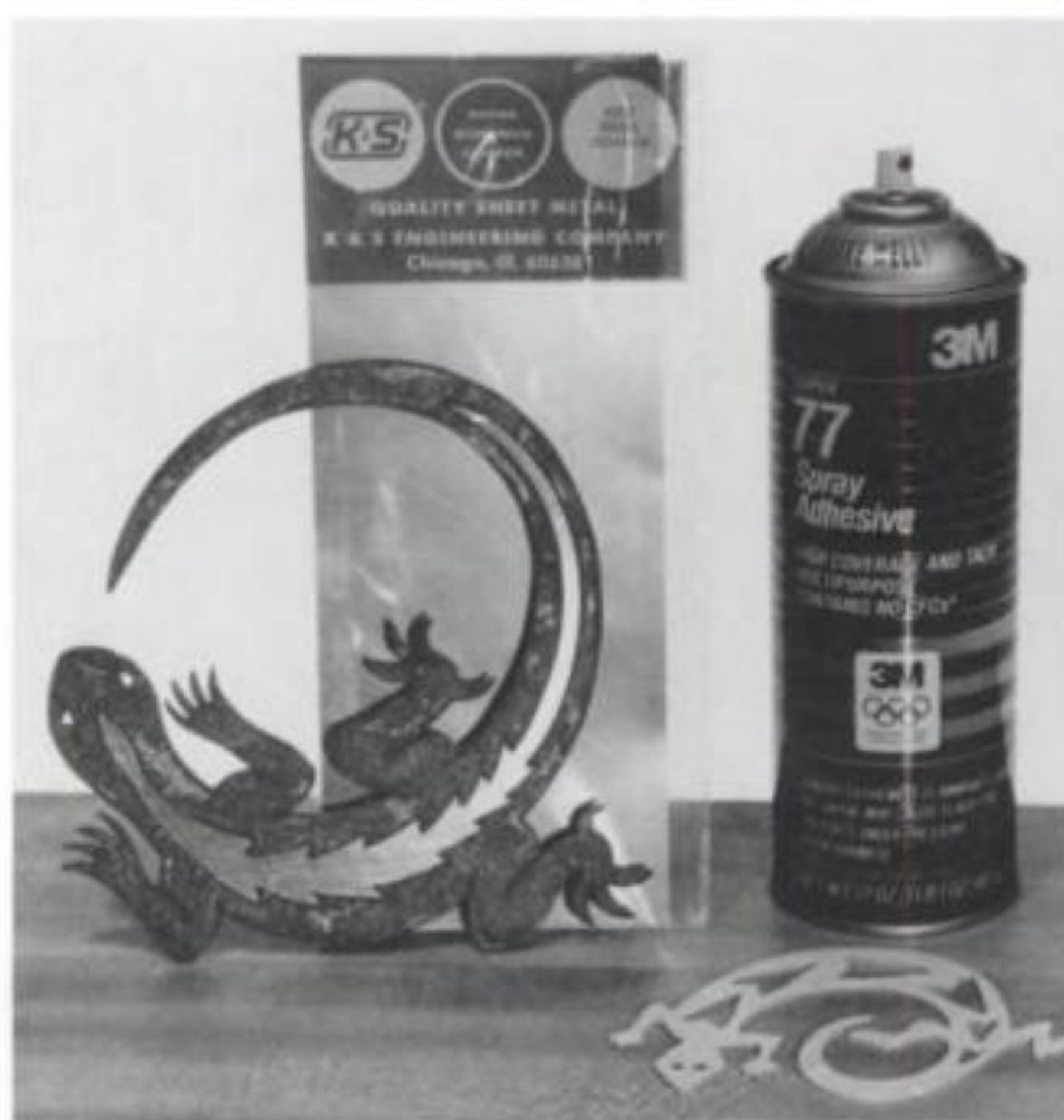
Illus. 10. Thin, soft metals—such as brass, aluminum, and copper—make interesting overlays. Use contact cement or a spray adhesive for bonding.
