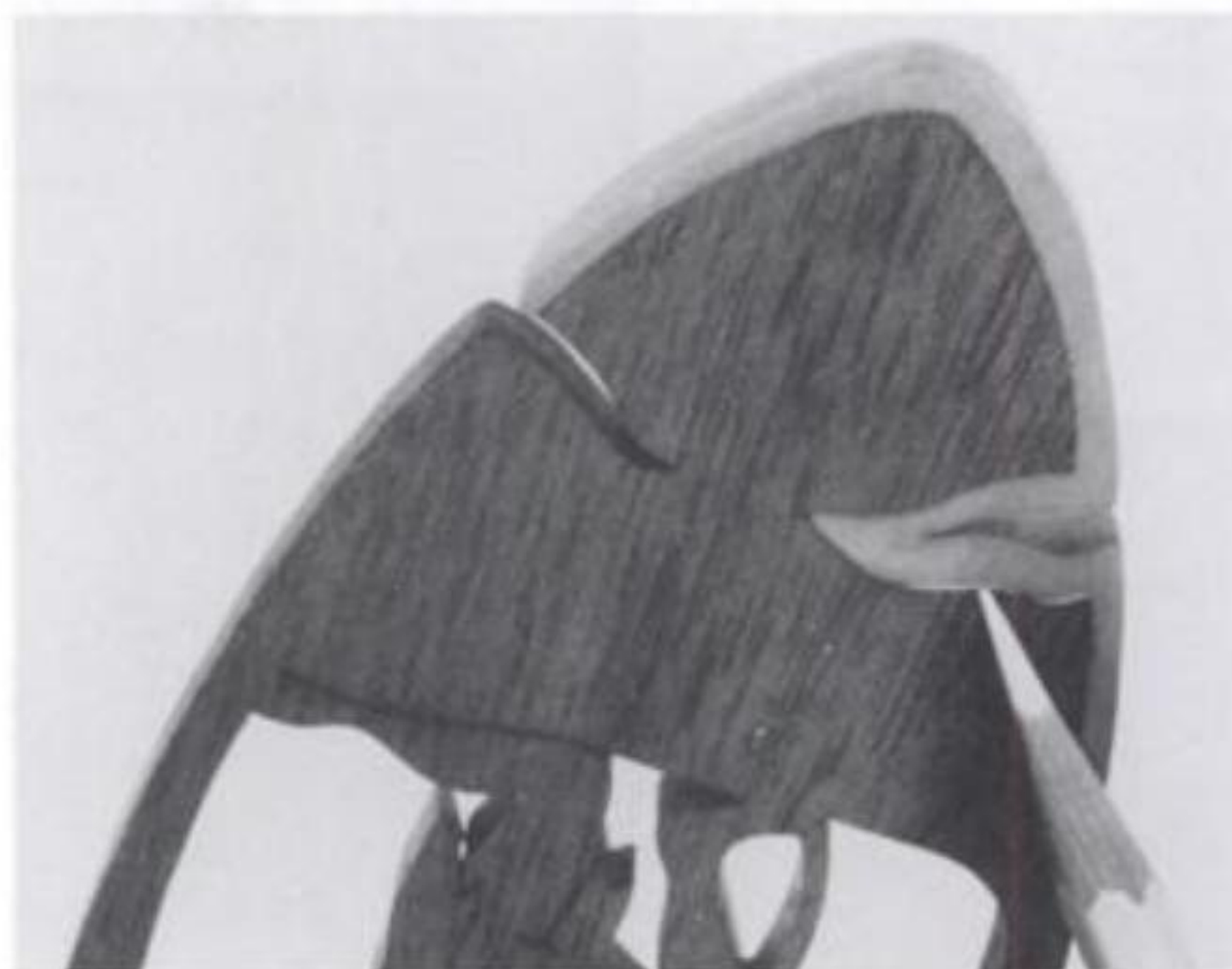
Illus. 18. Some visibility of a glue-filled saw kerf may be evident in some areas, as shown here, when employing the stack-sawn, or pad-sawn, method of inlaying.
