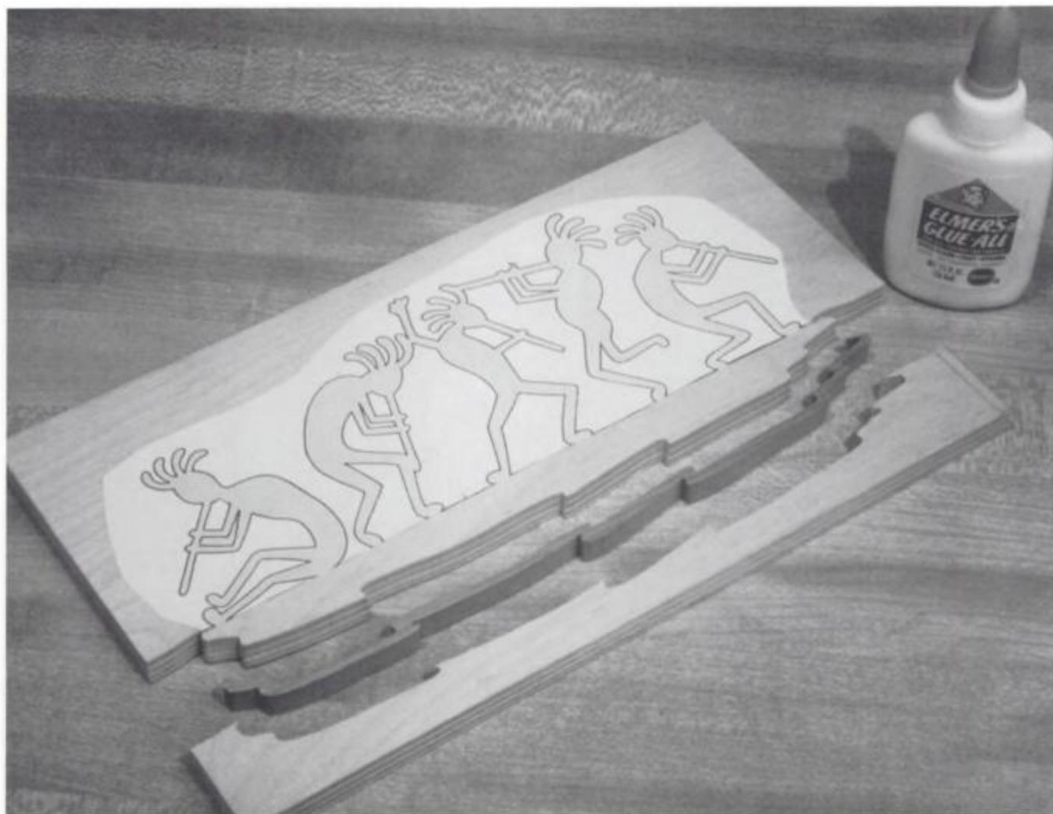
Illus. 22. Step. 4. Glue the inlay in place, and sand the surfaces flush after the glue sets.
