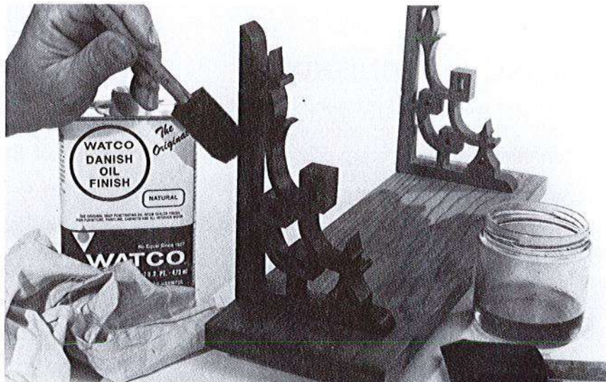
Illus. 361. A sponge brush is ideal for applying oil finishes. Soak the wood freely and wipe off the excess with a dry rag.
