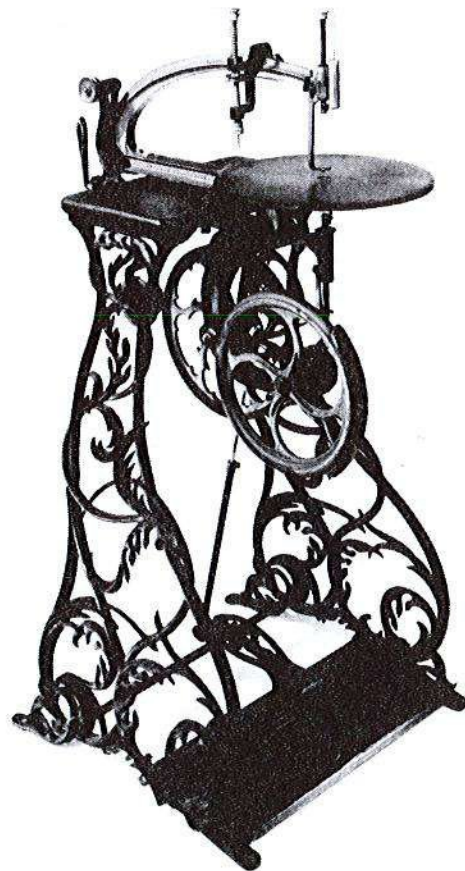
Illus. 36. The Fleetwood, one of the Trump Bros.' earliest saws, had a friction drive.
