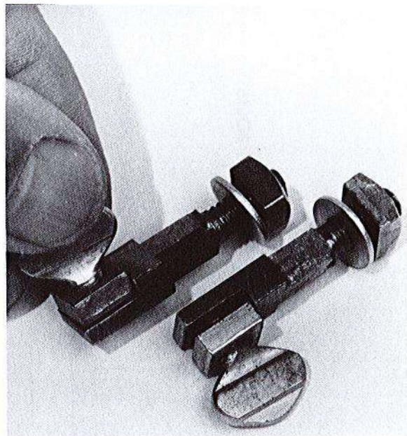
Illus. 391 (above left). A \frac{3}{16} -inch threaded rod can be used instead of bolts. Note the counterbored holes for the heads and nuts. The drawing at lower right shows how the heels of the arms can be modified to change blade size and/or blade tension by changing the base angle. Illus. 392 (above right). A close-up look at the homemade blade clamps.
