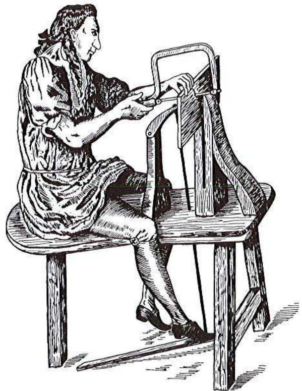
Illus. 8. Buhl sawing around 1775. Note how the workpiece is clamped in a vertical position on the "donkey" or "Buhl horse." The cutting is done with a push stroke. Two jaws hold the work firmly with foot pressure. One hand manipulates the workpiece, in coordination with the foot clamp, while the other hand moves the saw horizontally.
