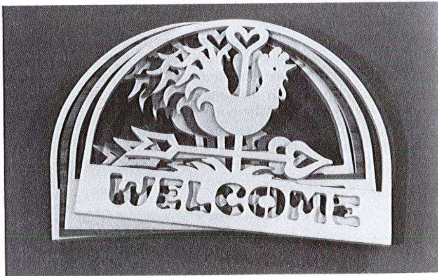
Illus. 235. The resulting pieces. Note that different thicknesses and kinds of plywood were used.
