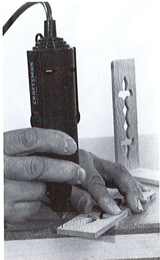
Illus. 79 (above left). The spiral or Archimedean drill is inexpensive, and cuts almost all thin materials quickly. Illus. 80 (above right). The high-speed rotary tool is ideal for drilling "saw gates" and small screw and nail pilot holes, as shown here, in assembly work.
