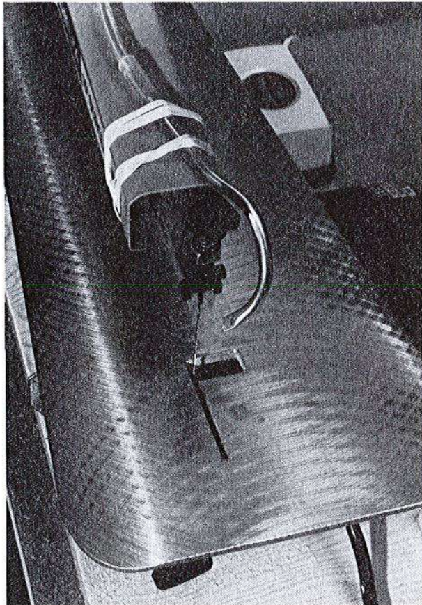
Illus. 146. The air from the aquarium pump is fed into this copper tubing nozzle. Note how the copper is slightly flattened at the end and bent to deflect sawdust away from the operator. Several rubber bands stretched over the tubing hold it all in place.
