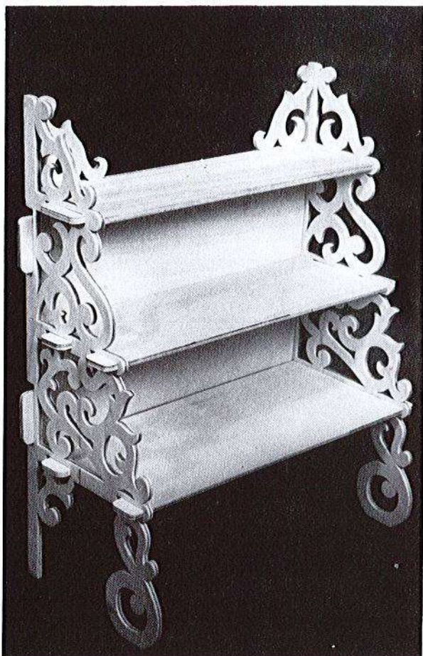
Illus. 322 (above left). This entire project can be assembled or disassembled with locked tab-and-slot joints. Illus. 323 (above right). Here you can see how the back, with integral corner brackets (above), interlocks with the sides to keep the project from "racking" from side to side.
