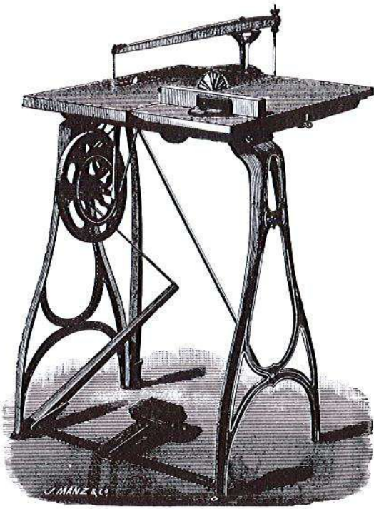
Illus. 47. This 1872 Combined Machine, a product of the W. F. & John Barnes, Co., of Rockford, Illinois, worked as a scroll saw and circular saw.
