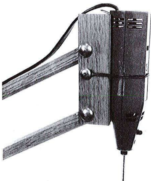
Illus. 396 (above left). Soft wire clamps the power unit to a formed motor mounting block. Illus. 397 (right). The lower rear assembly. Note the 6-inch coil spring on the left.
