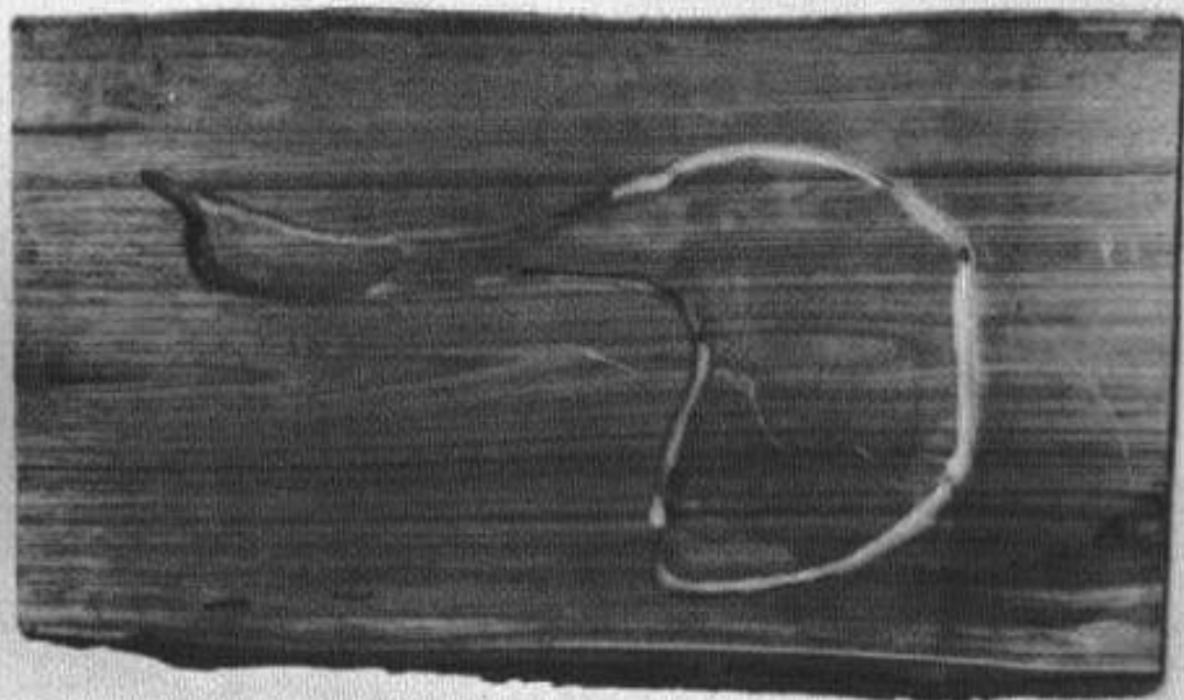
Pierce-cut design in \frac{3}{4} " thick butternut is rounded over and replaced so that it stands out \frac{1}{4} " in relief.
