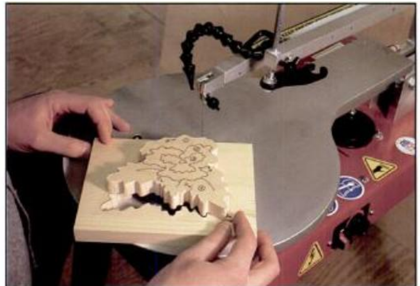
8. Carefully remove the outer scrap piece of wood and discard it.
