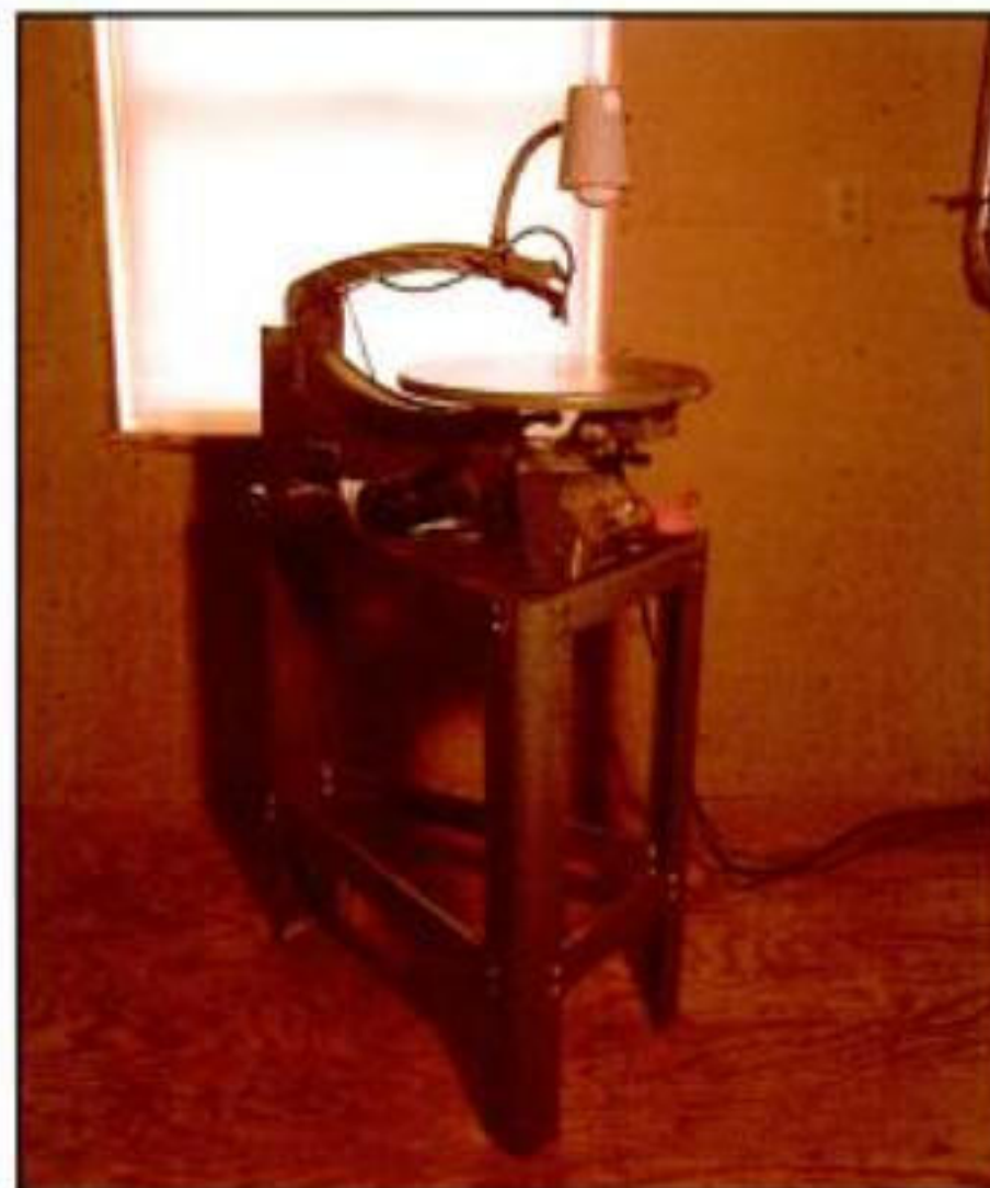
C-Arm scroll saws are best known for their aggressive cutting action. This is a Delta C-Arm (40-601).
