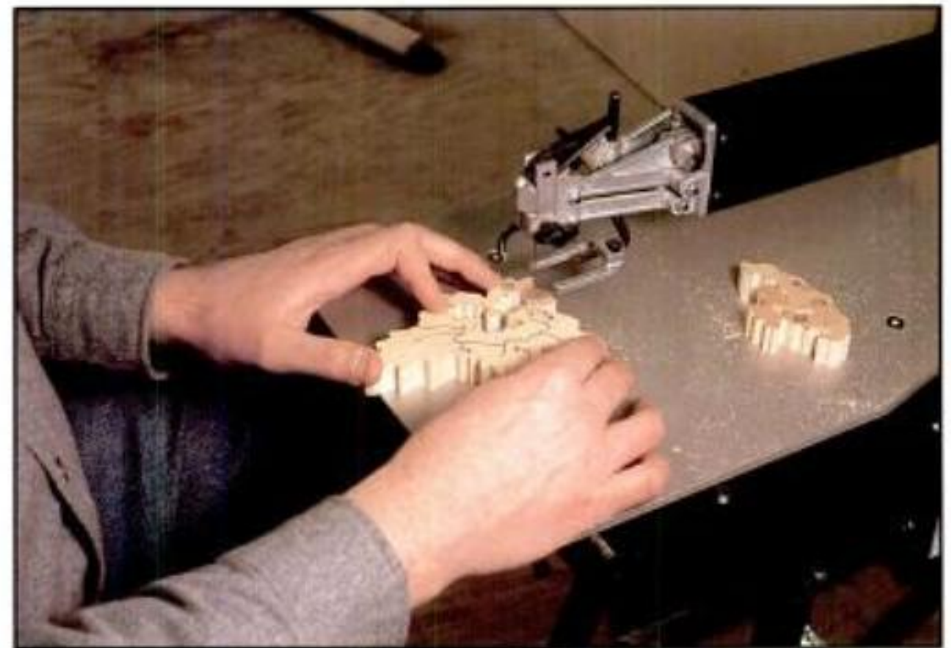
16. Enter and gently back out of the two cuts on piece #2. Be sure to keep a good grip on the puzzle.
