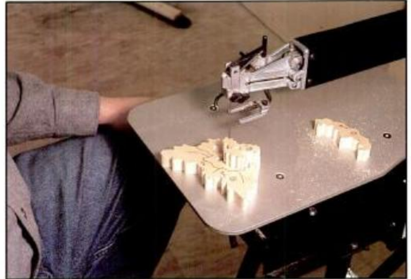
14. When the ripple inside piece #2 is complete, remove piece #3 and set it aside.
