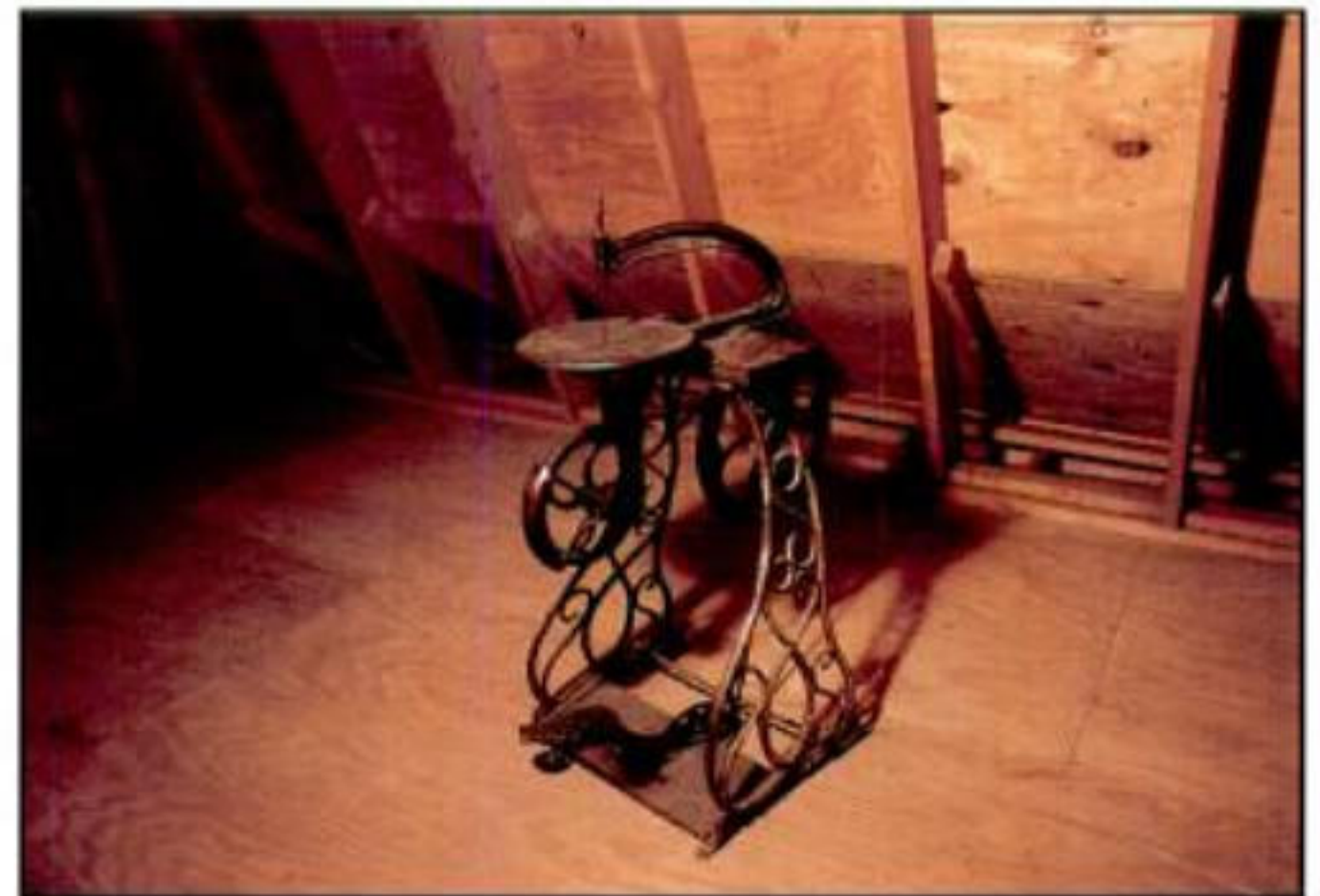
The Seneca Falls Challenge is an antique version of a rigid arm/plunger type scroll saw.
