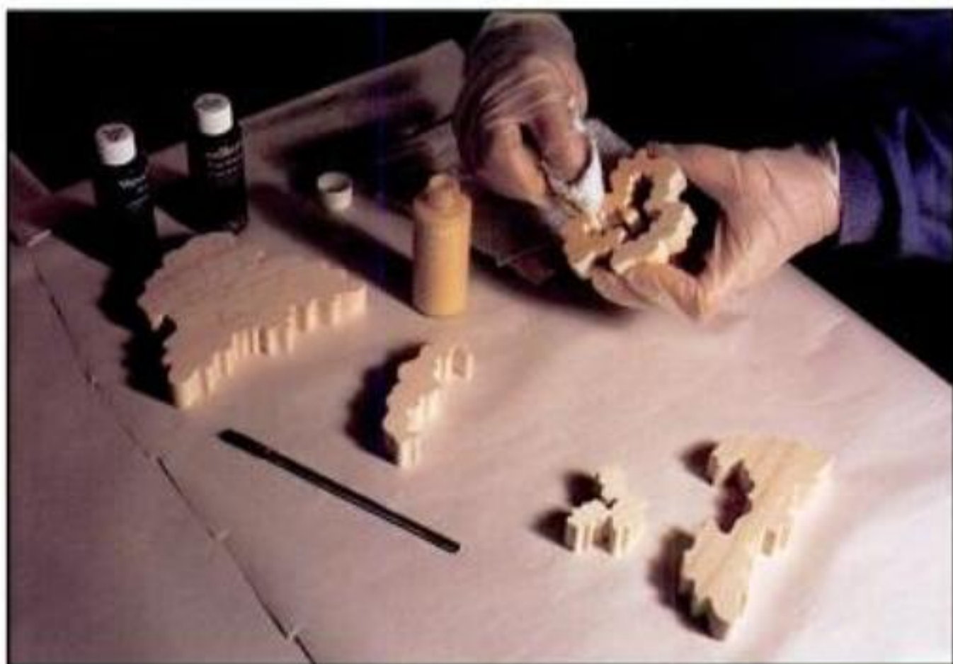
22. Stain the face of the puzzle first. Dip a cloth in the color and wipe it on in the direction of the grain.
