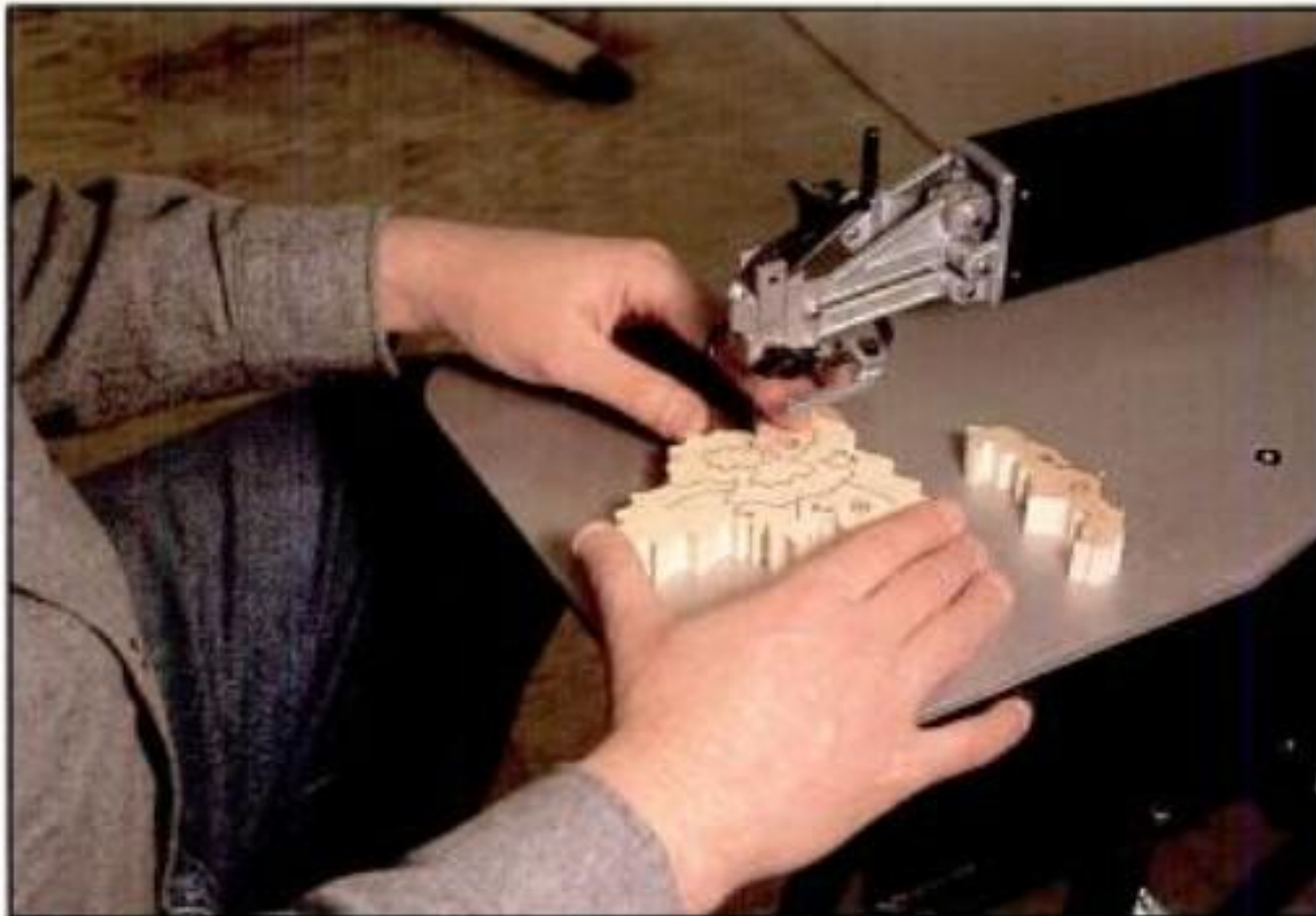
13. Cut piece #3 out of piece #2. Cutting the ripples in this piece is good practice.
