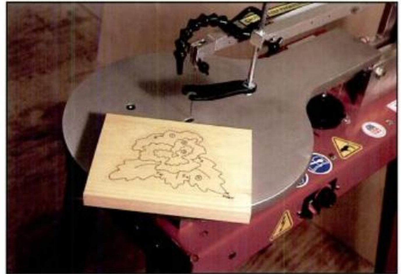
2. We recommend a #5 skip-tooth blade for the external cut on this piece.
