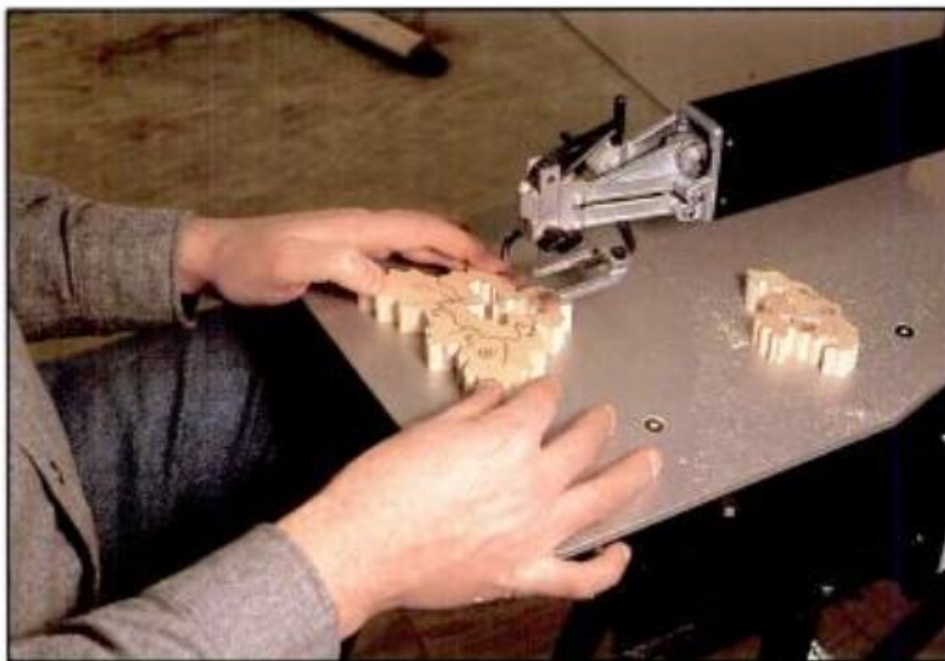
15. Cut out piece #2 where it joins piece #4 at point A.
