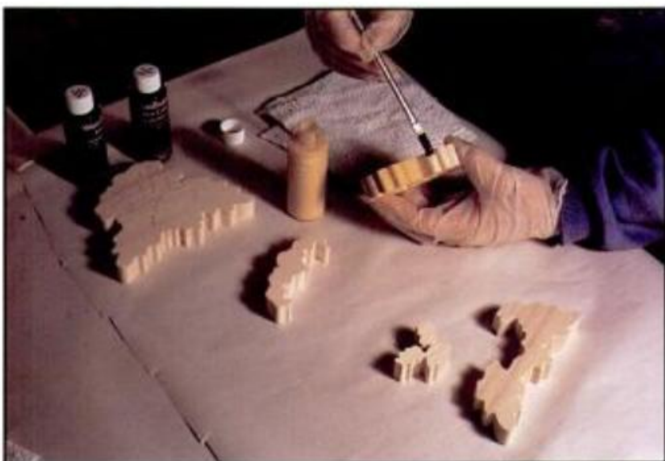
23. Apply stain to the end grain with a small glue brush.
