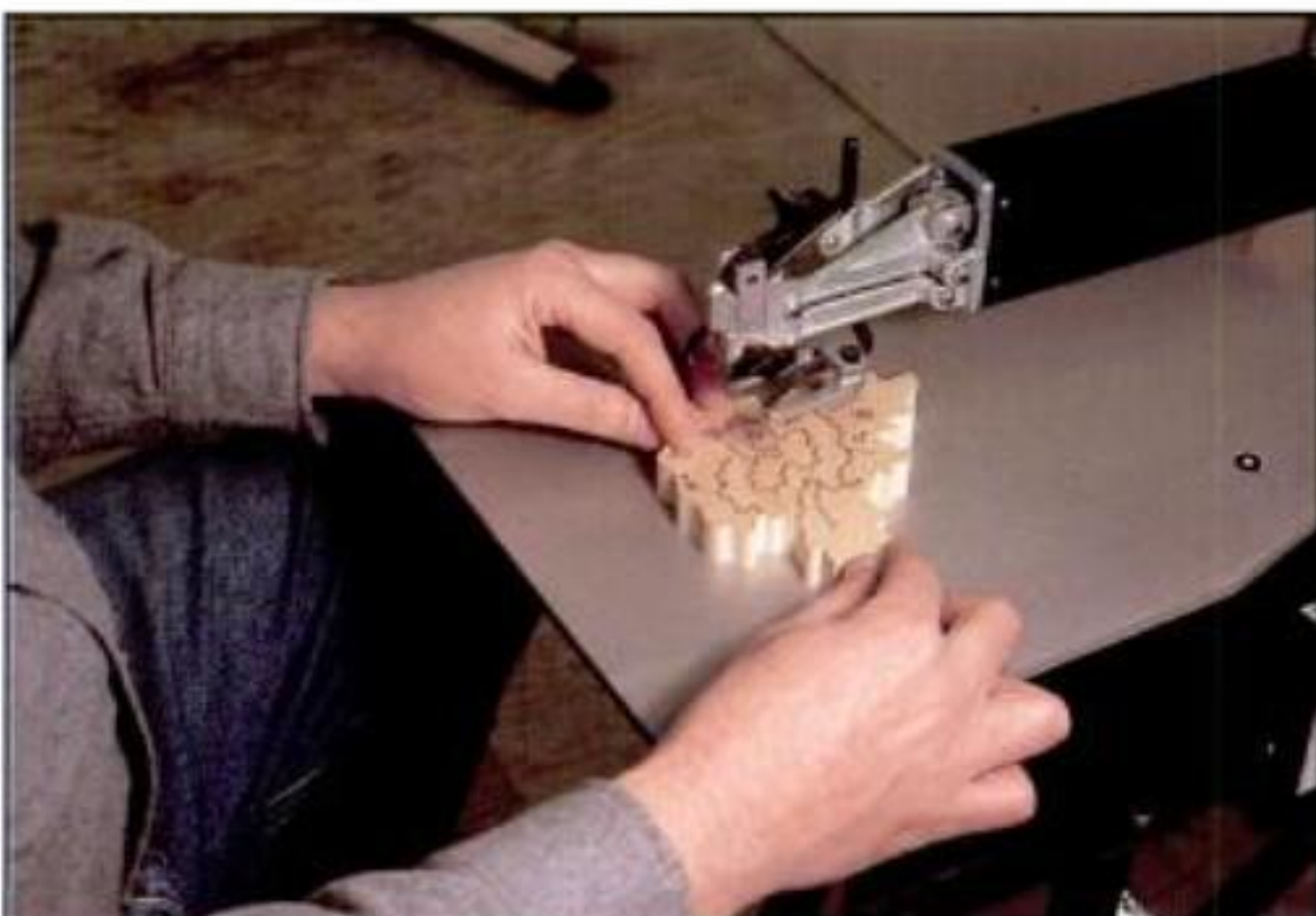
11. Carefully pivot to avoid breakage.
