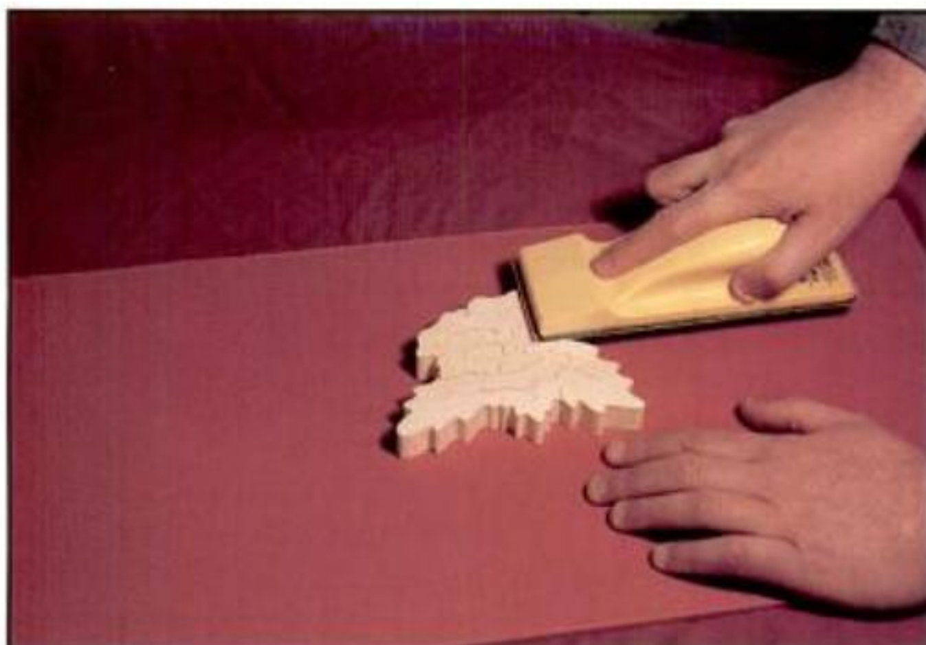
19. Using 100 or 150 grit sanding pad, sand with the grain in a back-and-forth motion.
