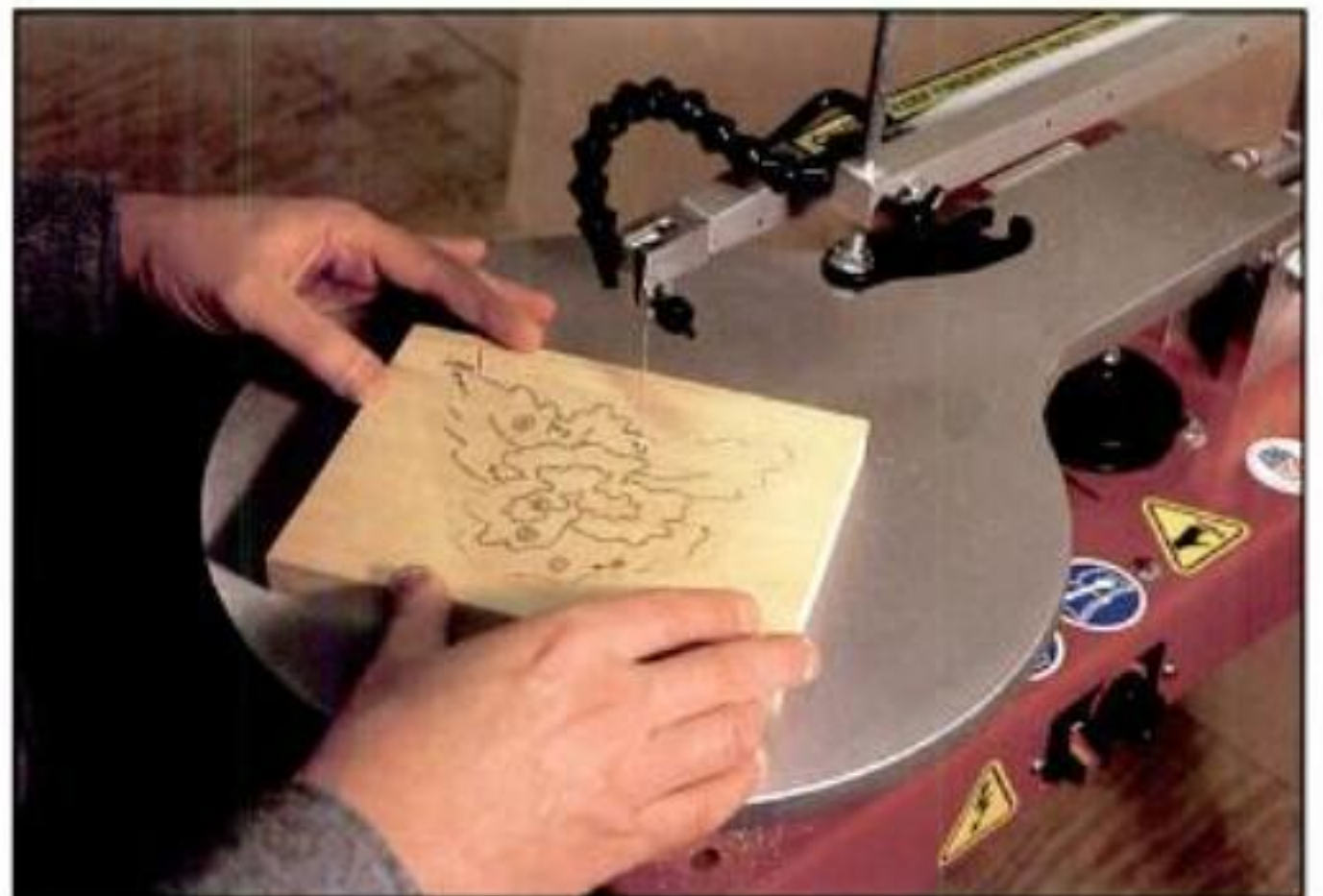
6. Pivot the wood on the blade to make a sharp turn. Continue to point C.
