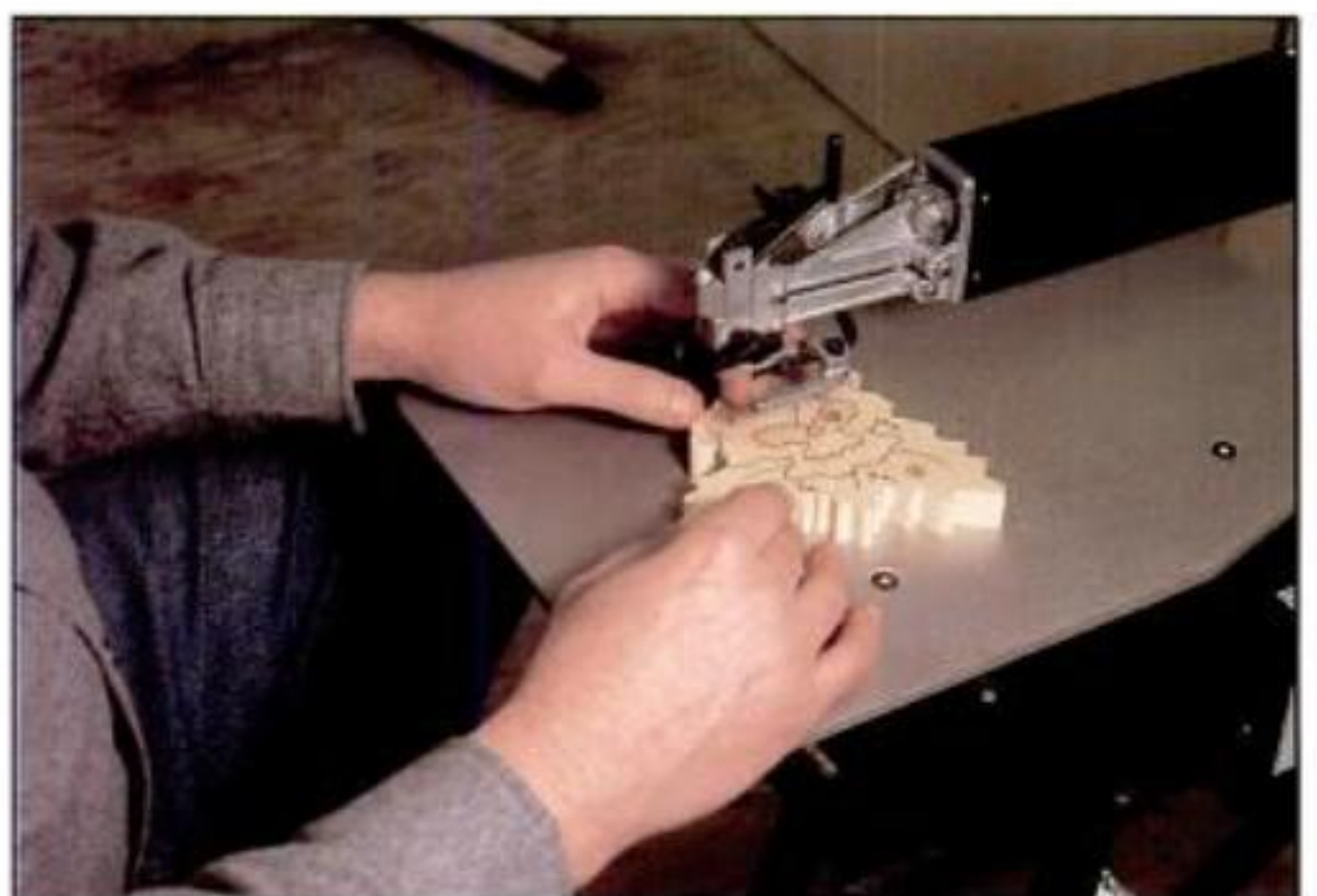
12. Slow down at the exit point to avoid ripping or tearing the end grain.
