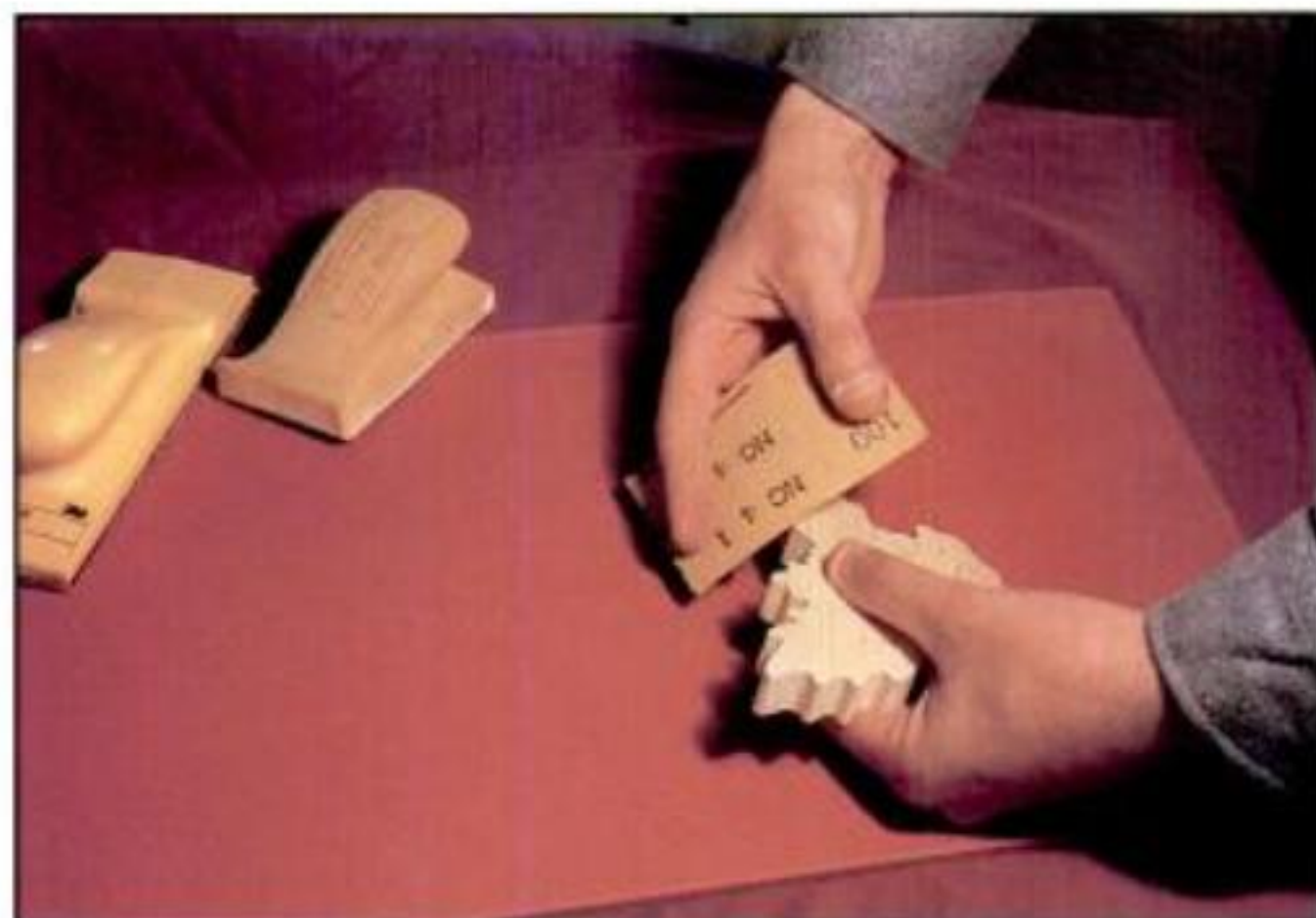
20. Sand the edges of the puzzle with a downward motion.
