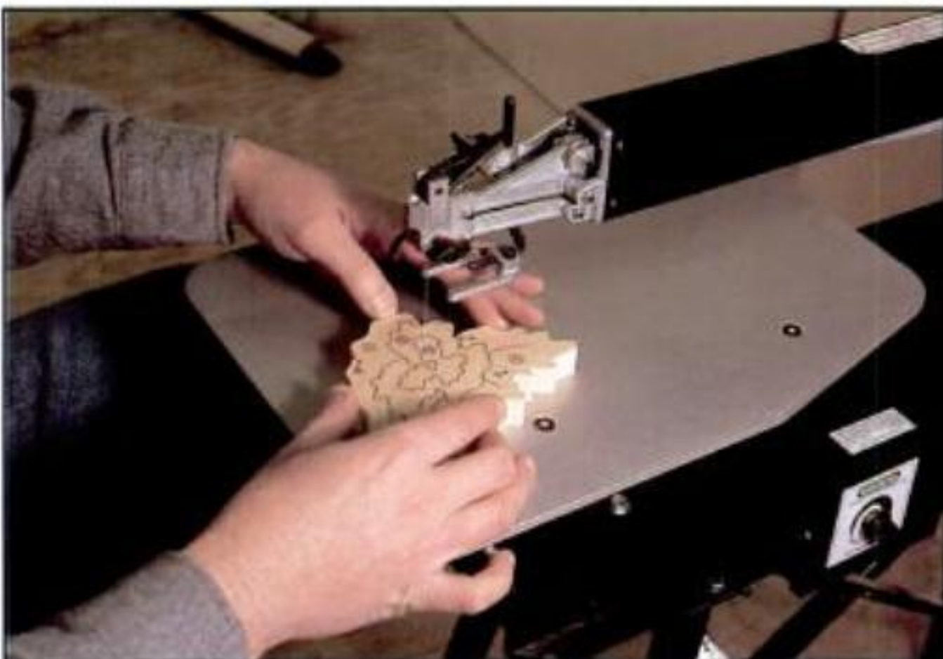
9. Switch to a #2 skip-tooth blade to make the internal cuts.
