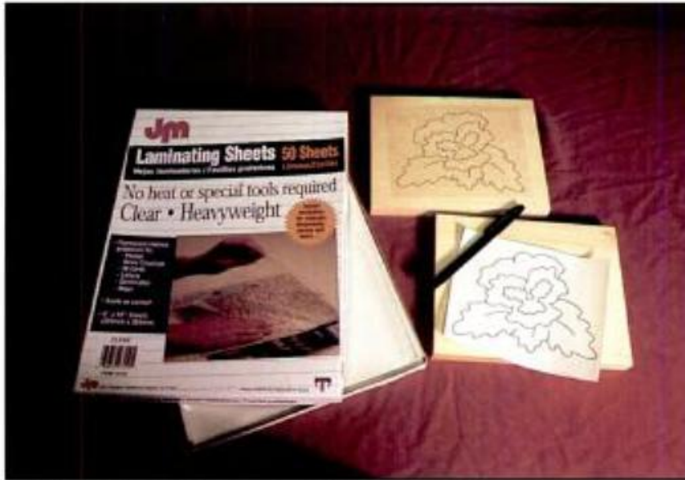
1. Transfer the pattern to the wood. We used laminating sheets for this project.
