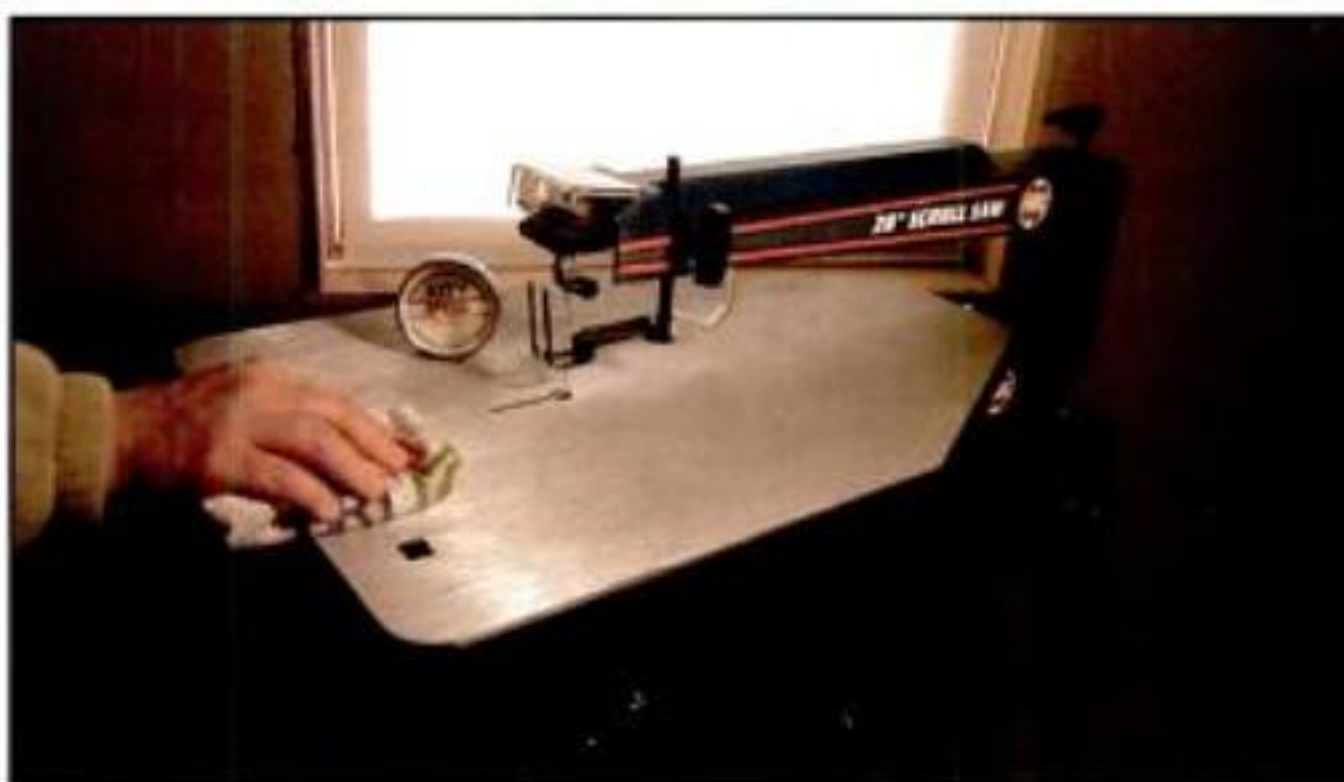
Lubricate the table with paste wax to help reduce friction. (Kitty Speed®, the lubricant shown in this photo, is no longer available.)
