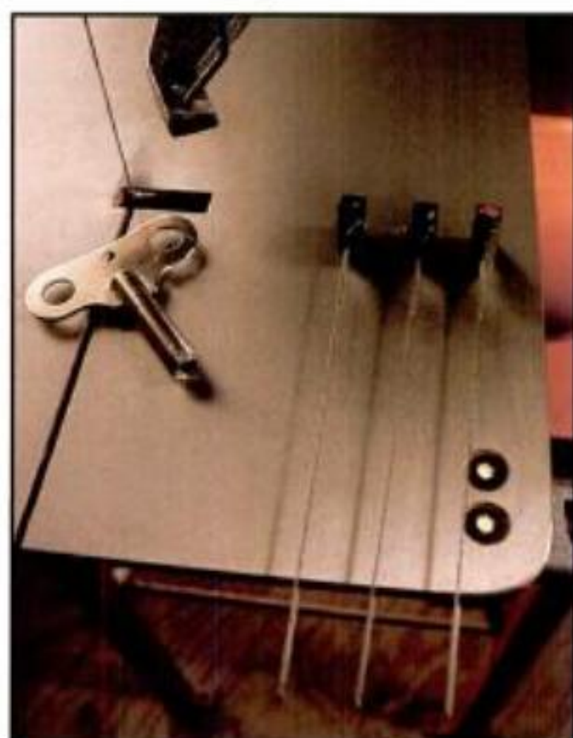
Color coding chucks with nail polish will help you to keep them separated.
