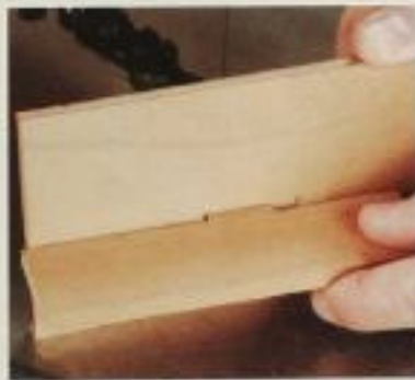
Step 2: Slide the tabbed piece over until it butts up against the inside edge of the slot.
