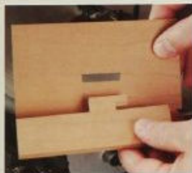
Step 1: Insert locking tab in slot until the back of the tabbed piece butts up against the face of the slotted piece.
