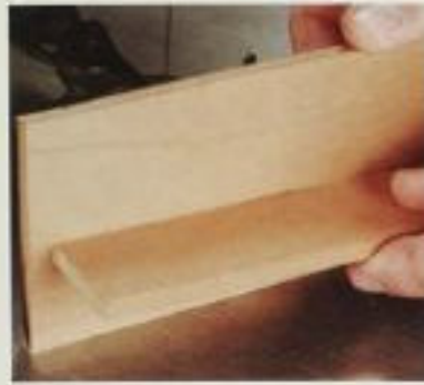
Step 3: When the locked tab piece is slid over completely, it should totally conceal the slot. To disassemble, just reverse the process.
