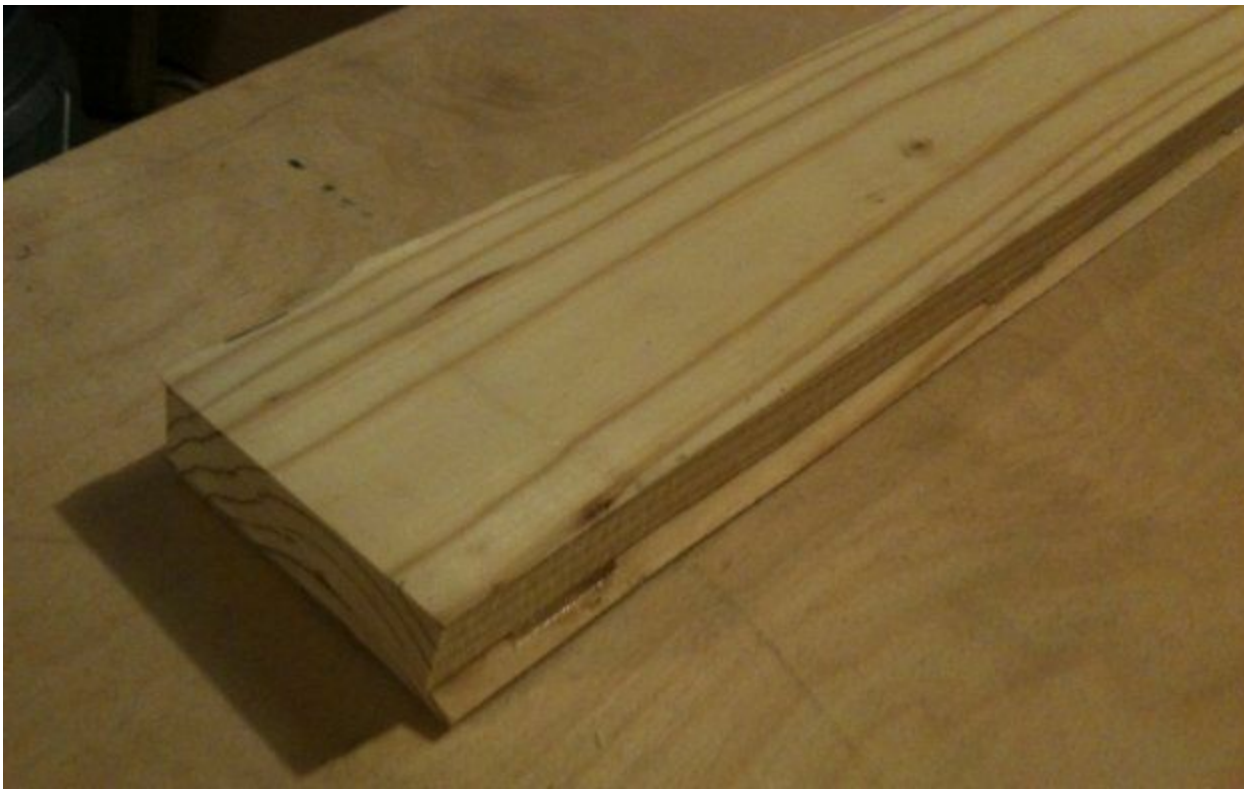
Figure 3 – The bevel ripped 2x4 is temporarily held together with a few beads of hot glue. The faces with the band saw marks are on the outside so they can be planed off with a jointer or thickness planer.
