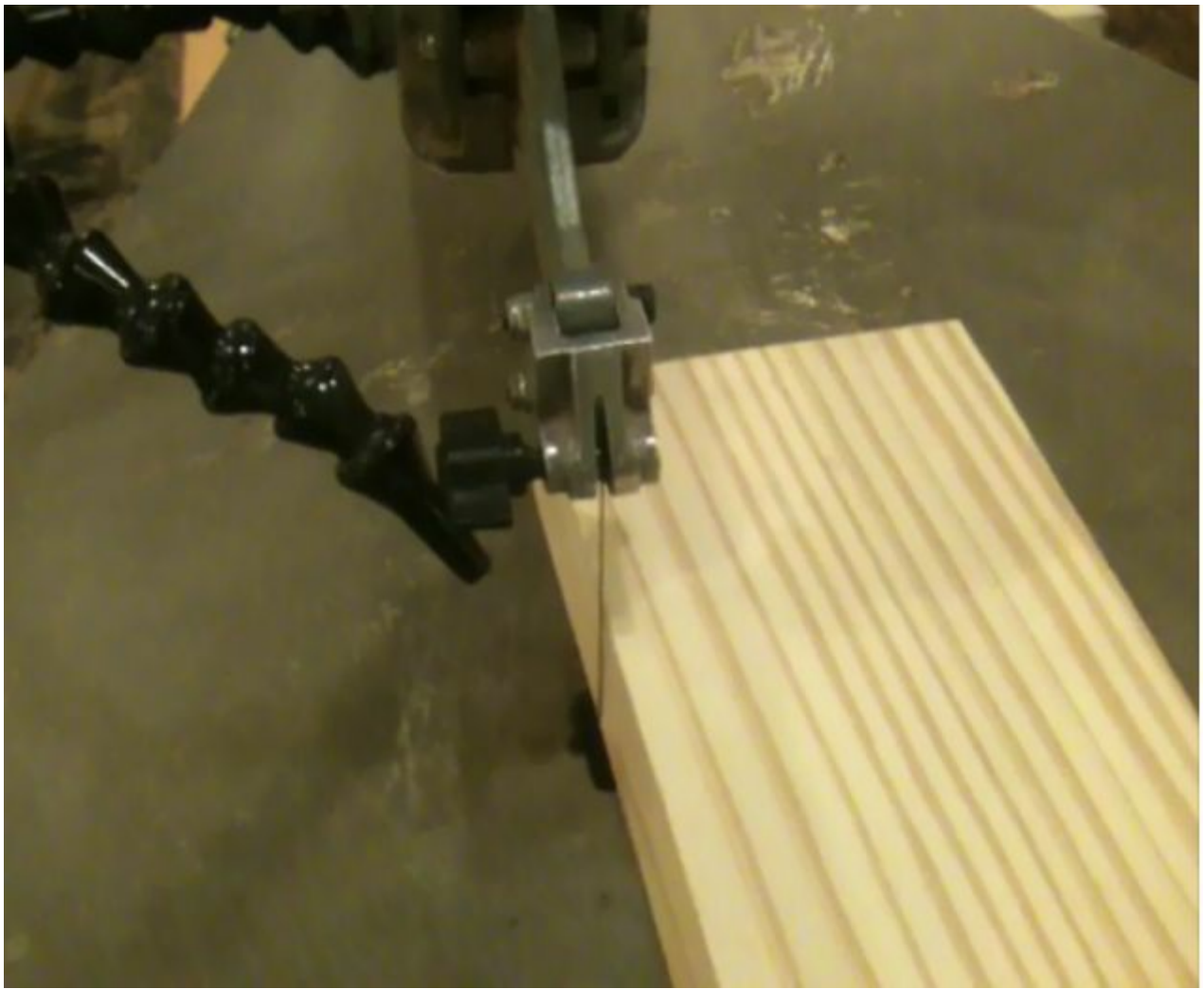
Figure 6 - Set the bevel angle by tilting the table until the blade is parallel to the thick edge of the wedge as shown.
