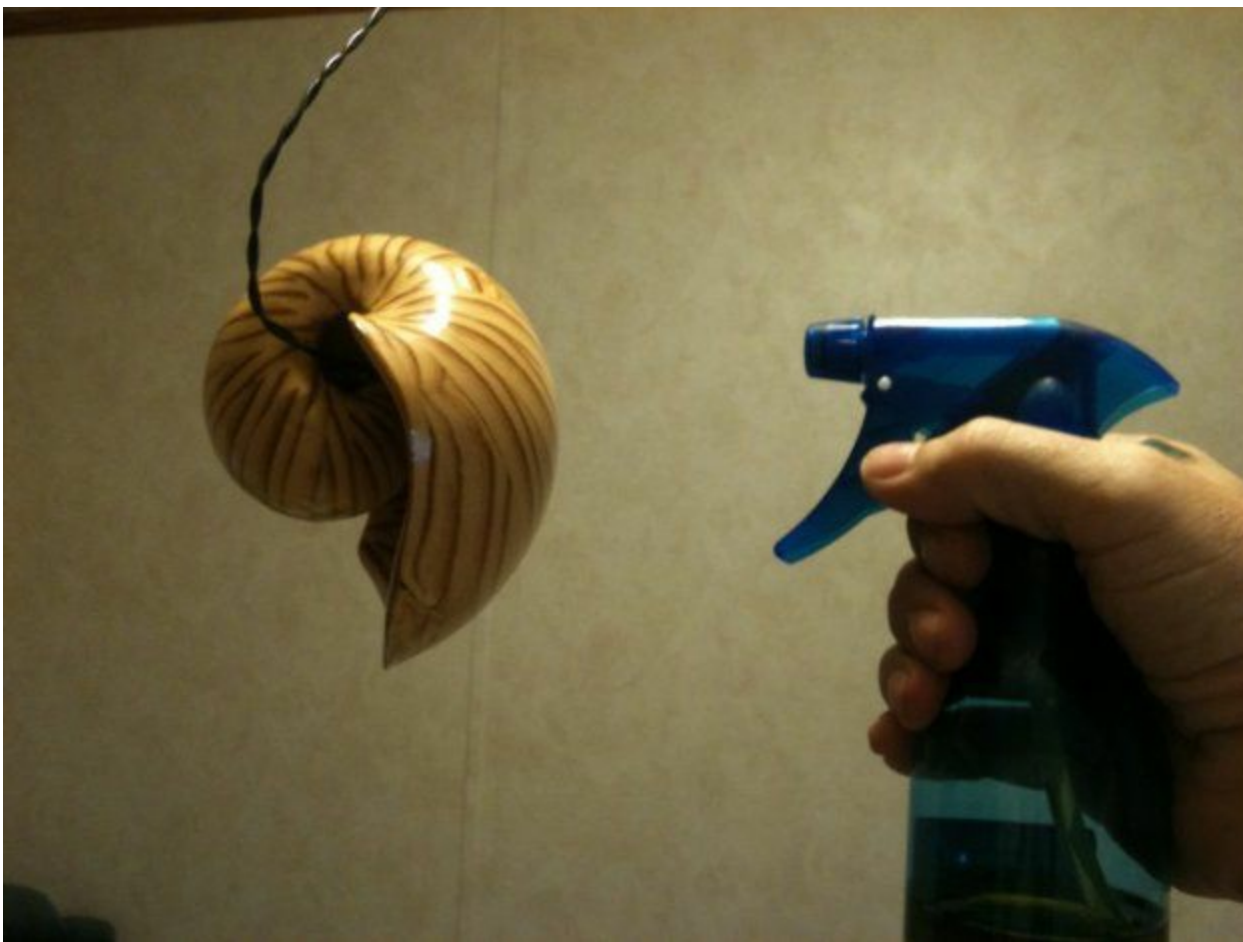
Figure 18 – The finish is applied as a mist using a cheap pump sprayer. With the proper mixture of thinner and finish to reduce surface tension, the finish is allowed to flow to the low spot and drip off.
