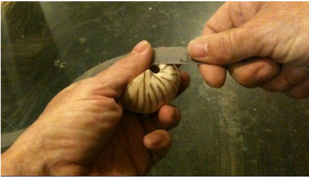
Figure 14 – Strip sanding an area that will be harder to reach after the next group of segments is added on.
