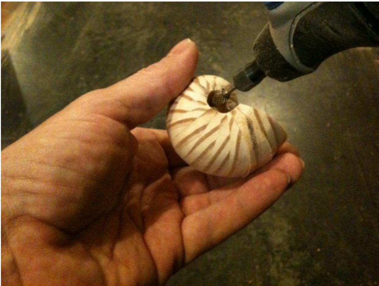
Figure 16 - smooth the central hole with a rotary tool as segments are added before the area becomes harder to reach.
