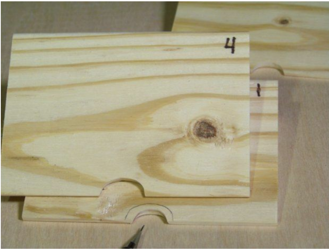
Figure 8 – After each wedge has been used to cut a segment from, the next segment will be hollow. If the wall of the segment looks like it is going to be too thin then add more segments. Later as the segments become larger, they also become thicker.
