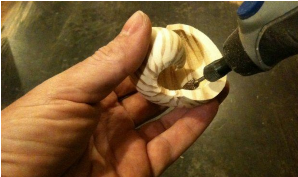
Figure 13 – Smoothing the interior. The flat faces from the saw cut need to blend together to form a smooth continuous curve.
