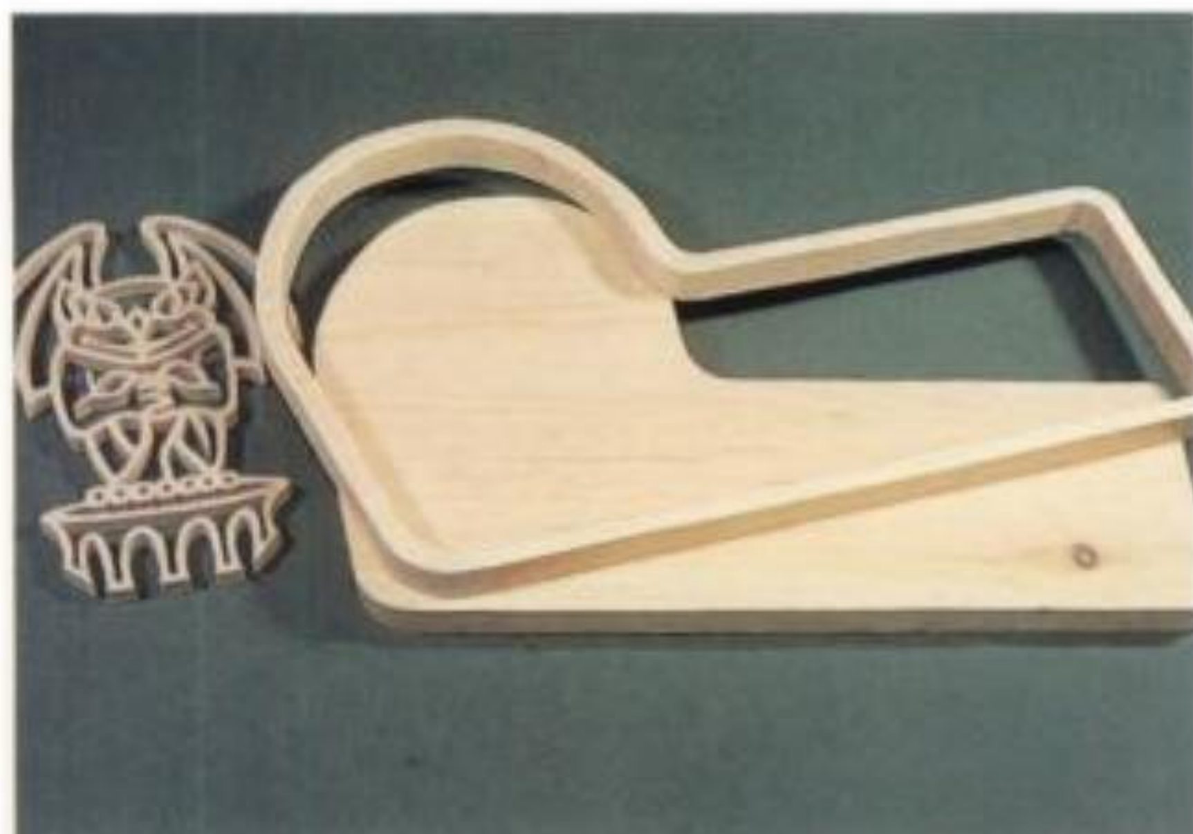
10-3. The raised border is made with one continuous bevel cut all around the plaque.
