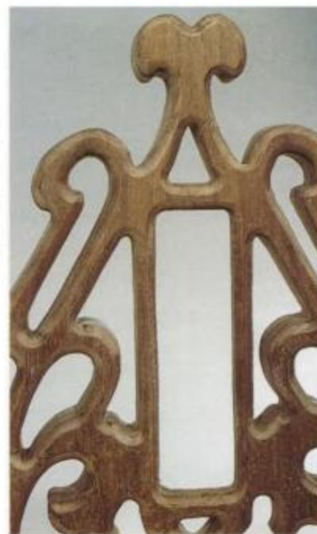
7-23. A close-up of the edge. A sharp bit, multiple passes, and a soft horizontal feed should produce clean cuts with few if any burns.
