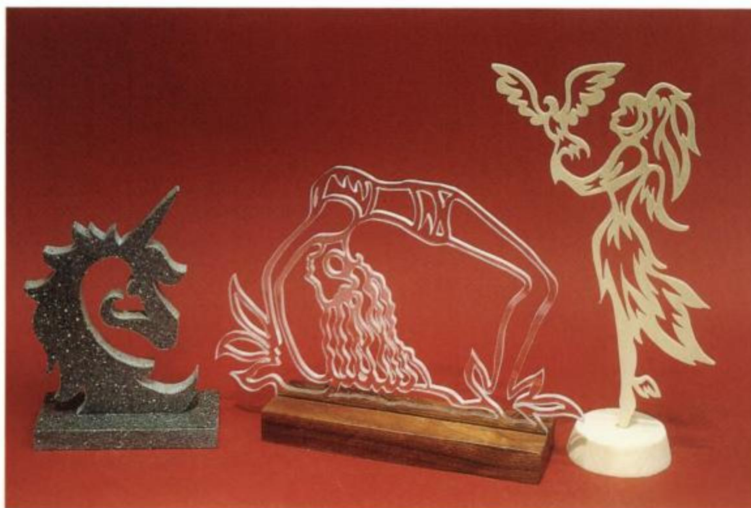
2-19. Left: Unicorn cut from \frac{1}{2} -inch Corian. Center: acrobat cut from \frac{1}{8} -inch clear acrylic plastic. Right: “Wings” cut from \frac{1}{8} -inch Baltic birch plywood. All designs by Bev Carmody.
