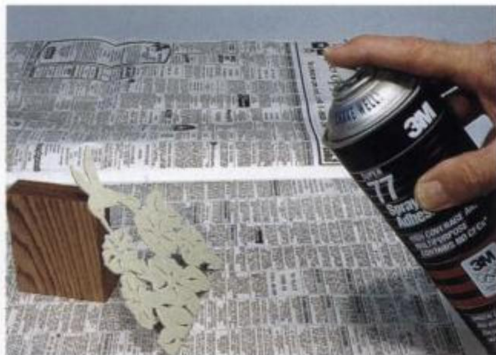
9-8. Spray the adhesive directly at a right angle to the surface to minimize glue build-up at the edges.
