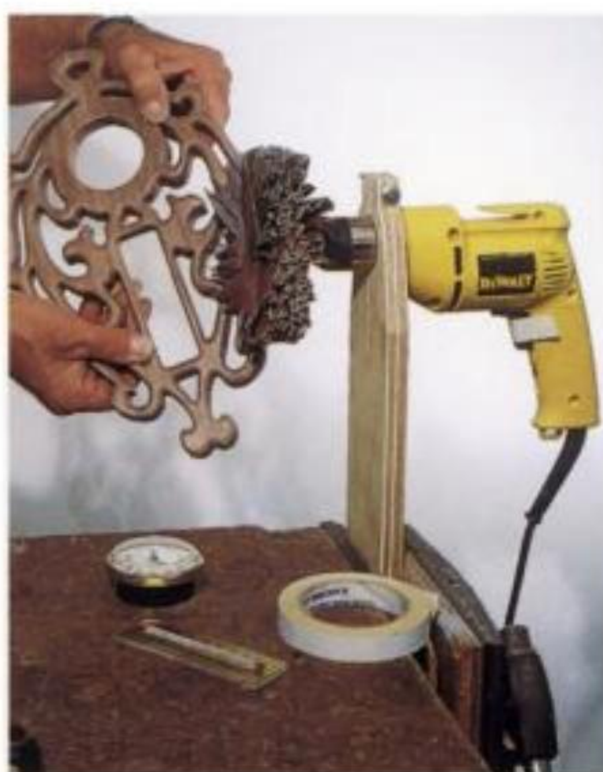
7-24. Sanding is easy with the flutter wheel. Notice how tape holds the trigger switch of this variable speed drill; the switch is turned on at the best speed choice.
