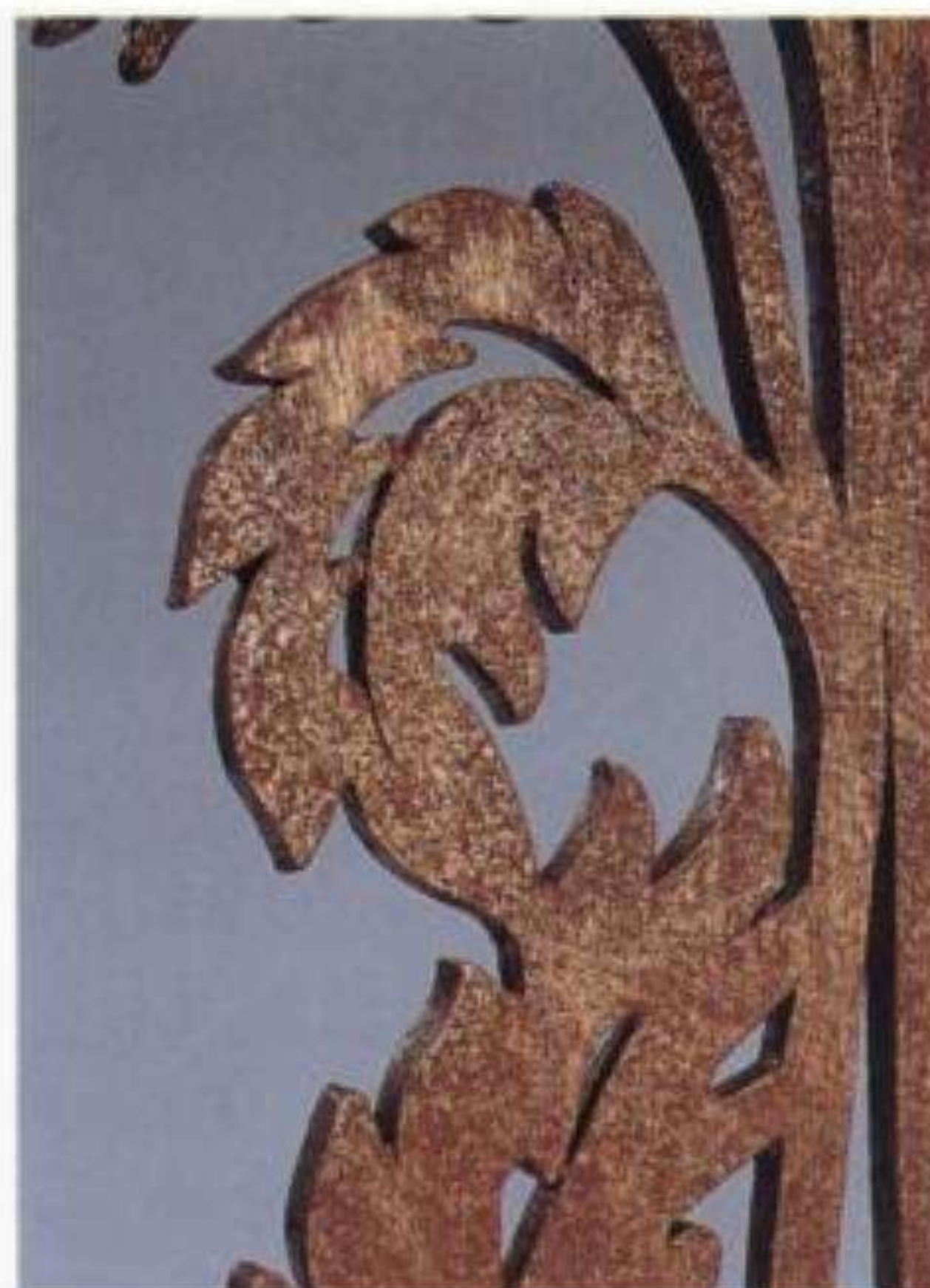
12-5. A close-up look at another metallic finish. This is a burgundy patina solution applied over a liquid copper coating using a plastic bottle and spray mister.
