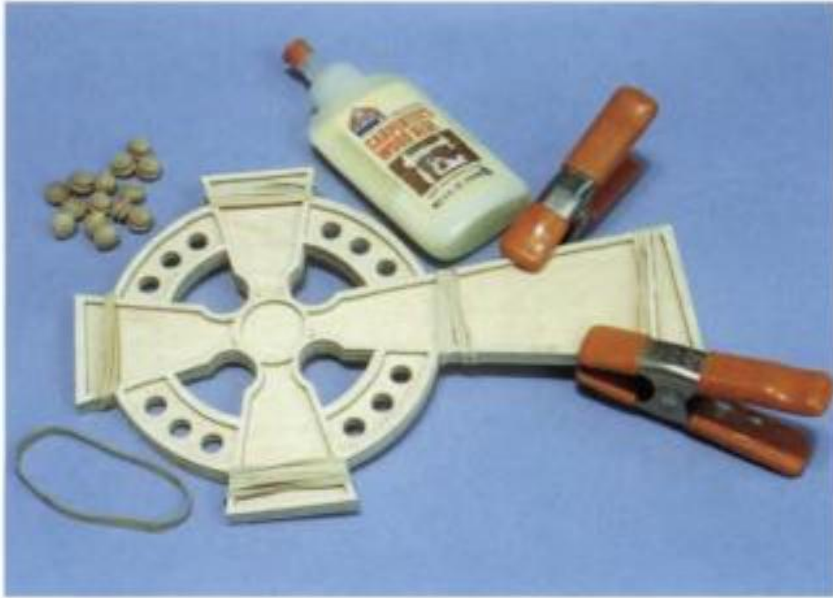
4-16. Gluing the border(s) to the backer(s).
