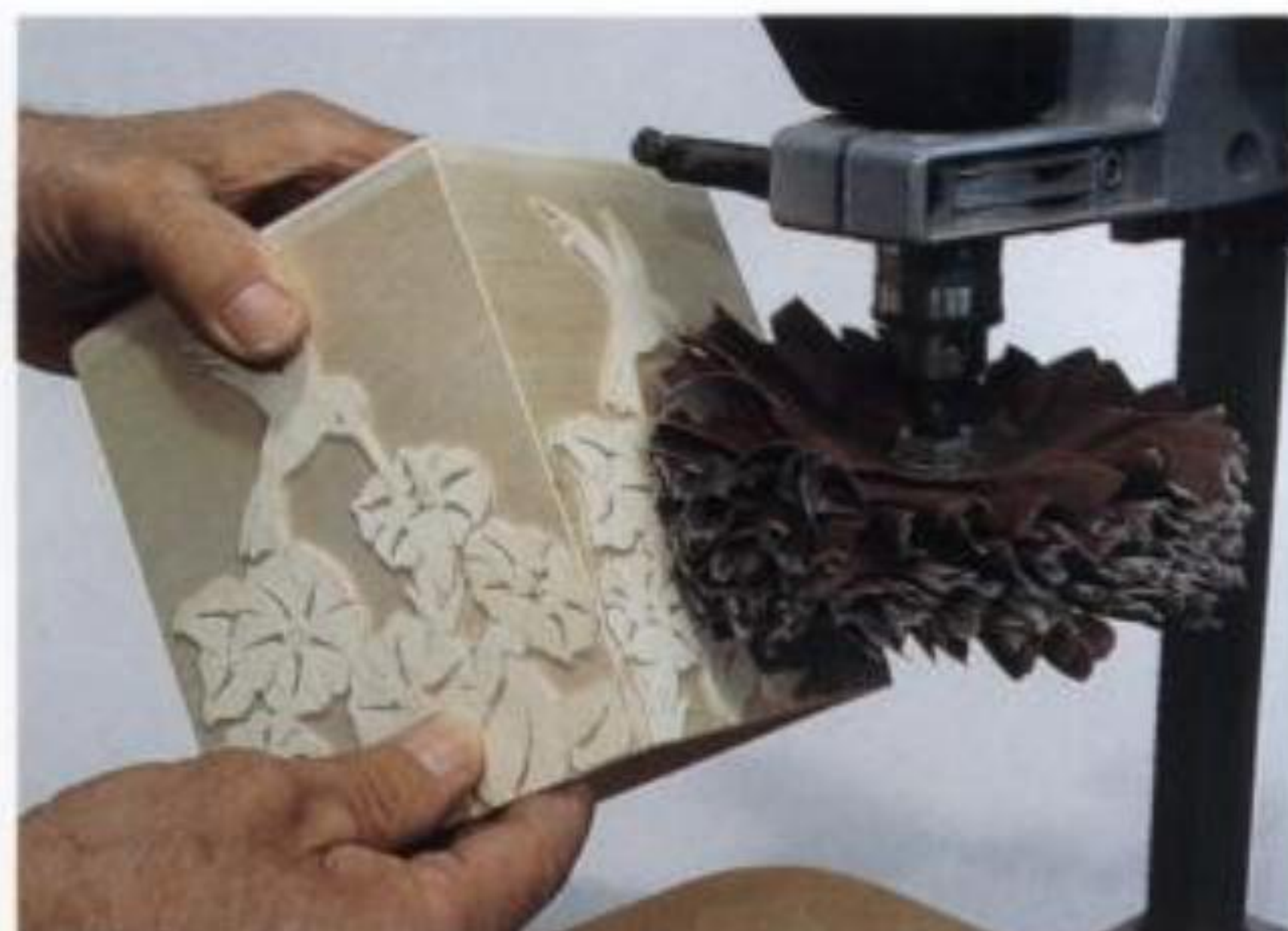
9-9. Using the flutter wheel to soften sharp edges.
