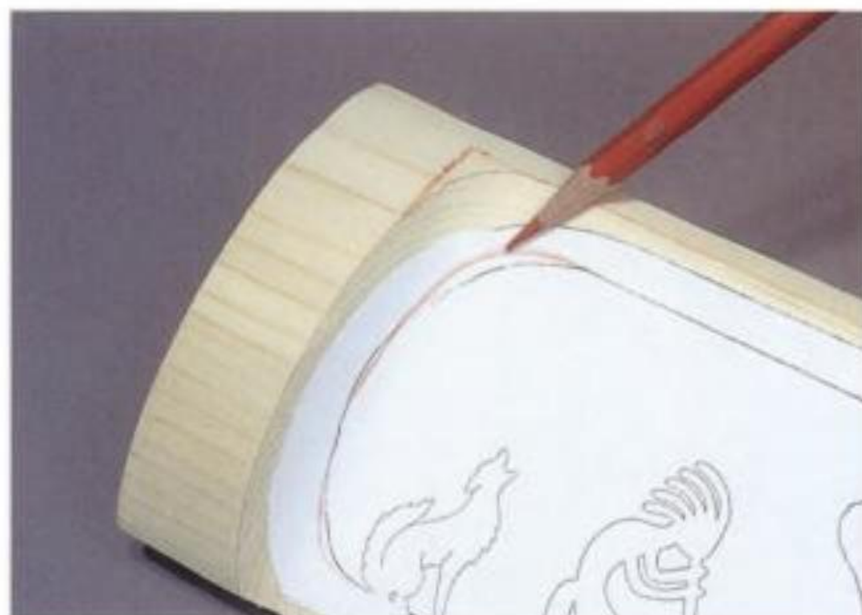
11-5. Modifying the curved lines (shown in red) on the inside of the "window" pattern. This may be necessary to ensure that the resulting frame-like surfaces will be the same width all around.
