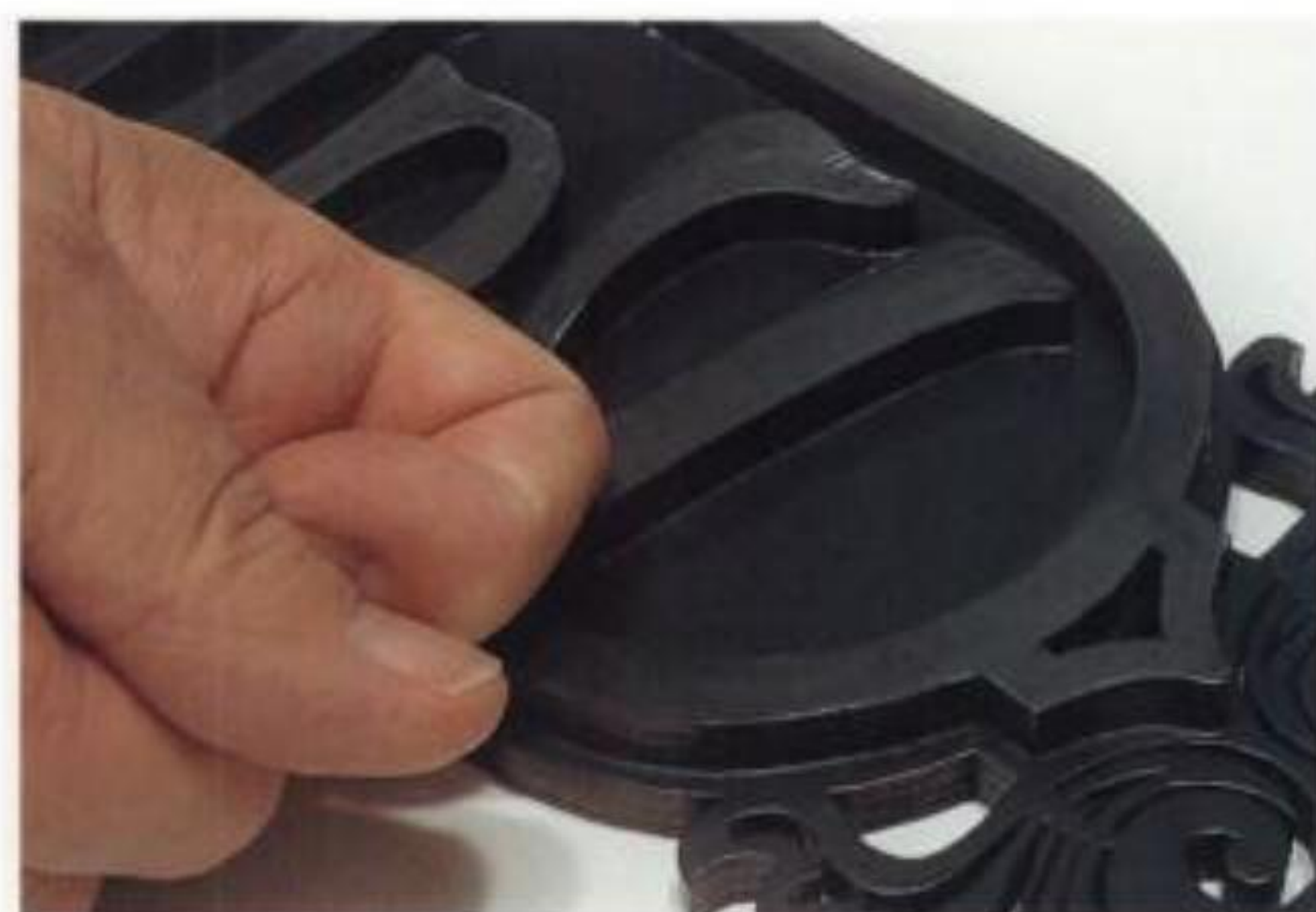
10-12. Testing the dryness of the "size" with your knuckle.
