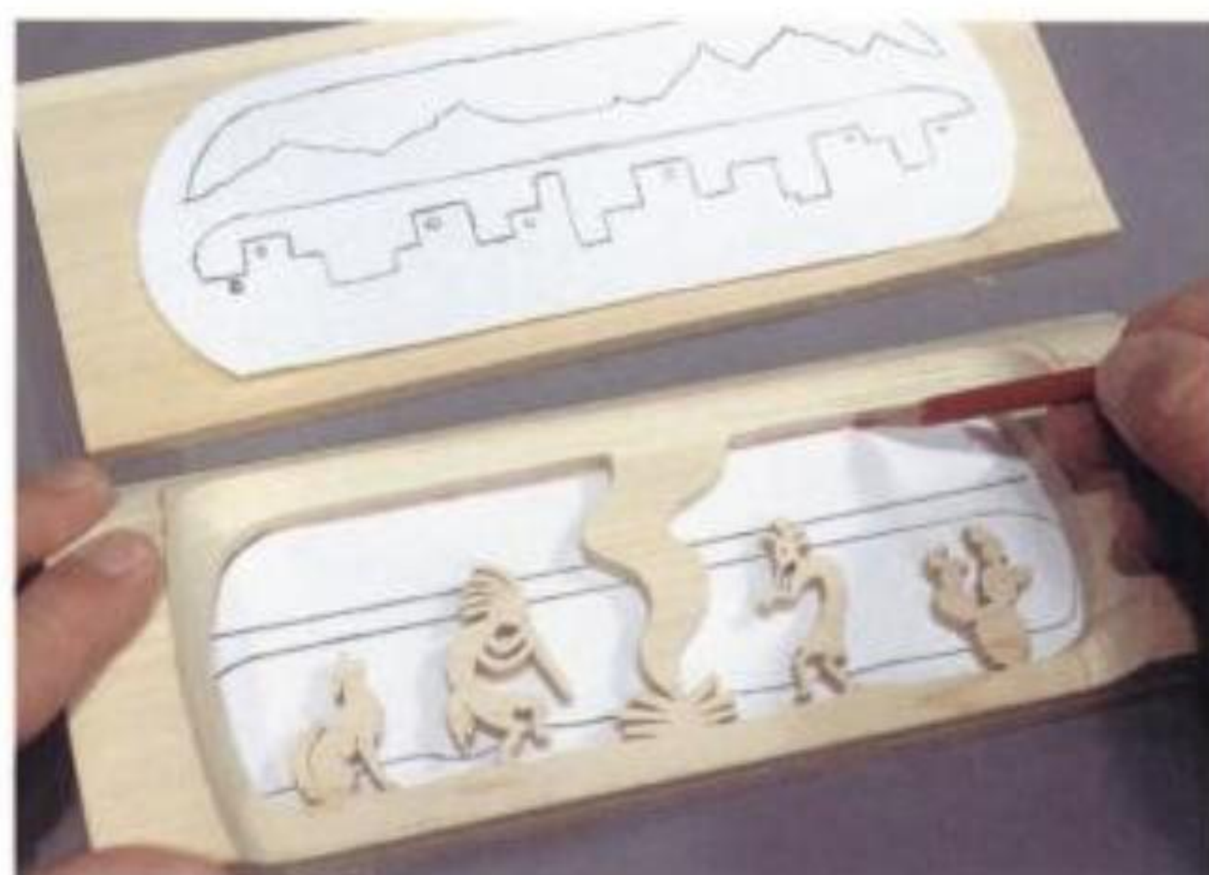
11-6. The window silhouette becomes a pattern to modify the perimeter line of the inside opening of silhouette no. 2.
