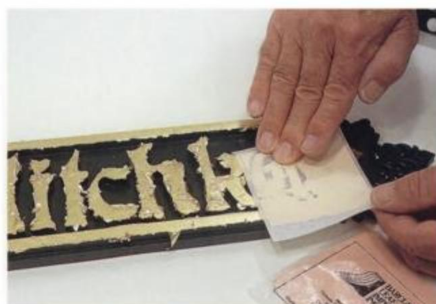
10-15. Use fingertips to transfer gold leaf to small areas, to fill in voids, or to cover small, open spaces. one about \frac{1}{8} inch.
