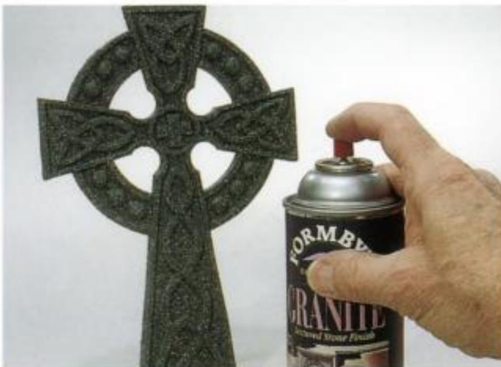
4-20. Applying a textured stone finish with an aerosol spray.
