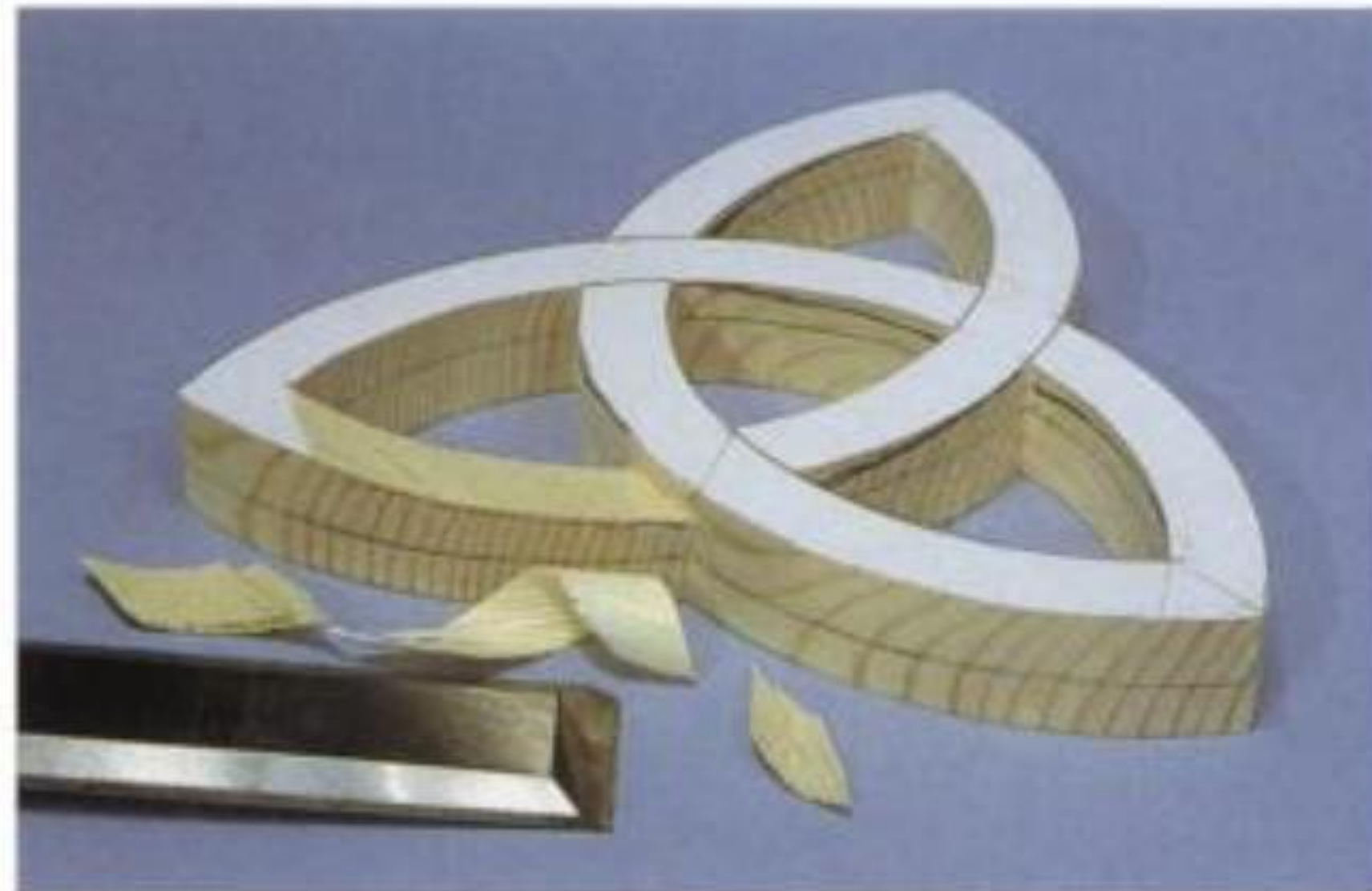
9-21. Carving to taper and reduce the thickness is done in six areas as shown. Here a flat chisel was used.
