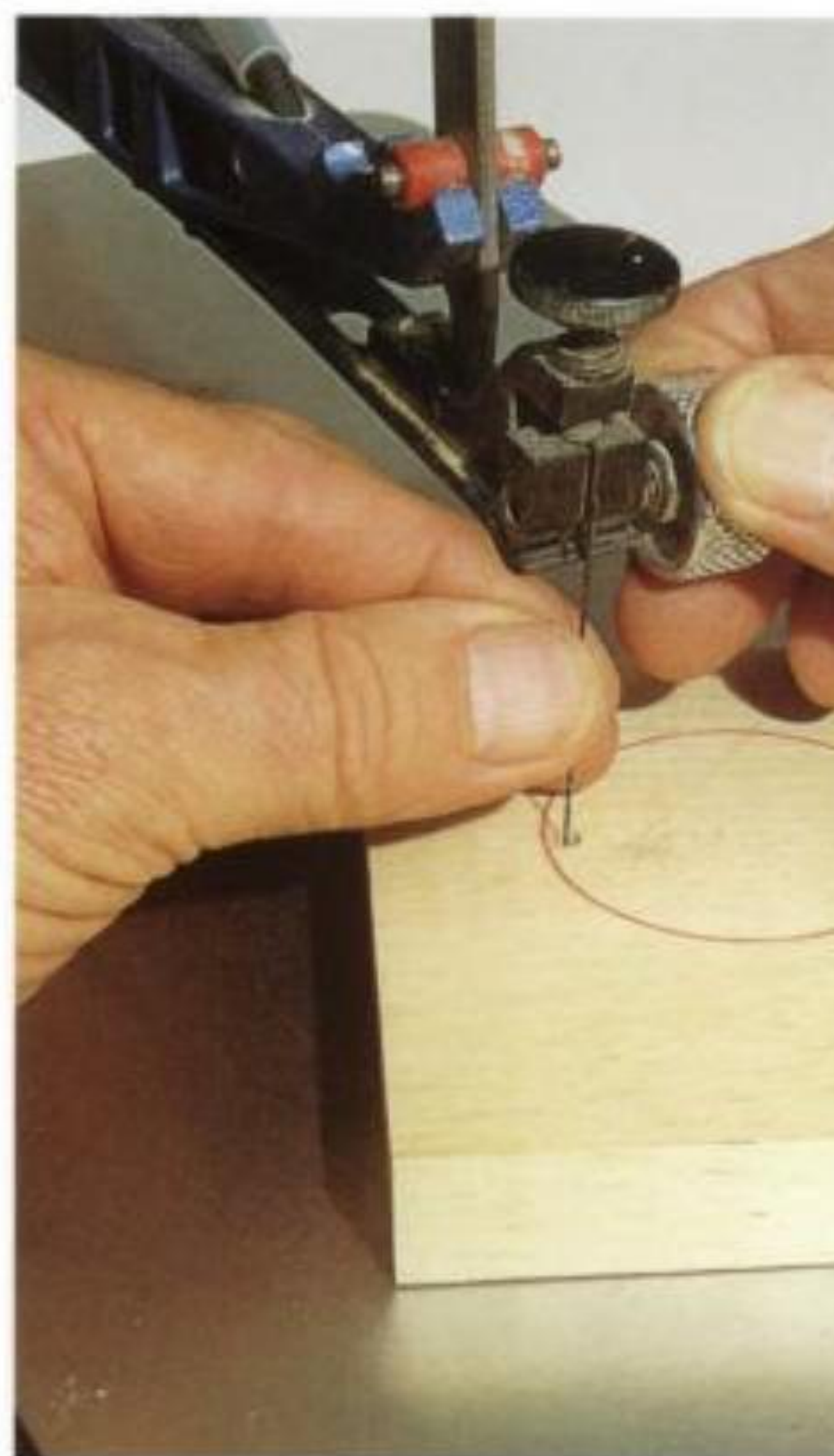
1-15. Threading the blade through a hole drilled in the waste to make an inside cut such as an opening for a clock insert.
