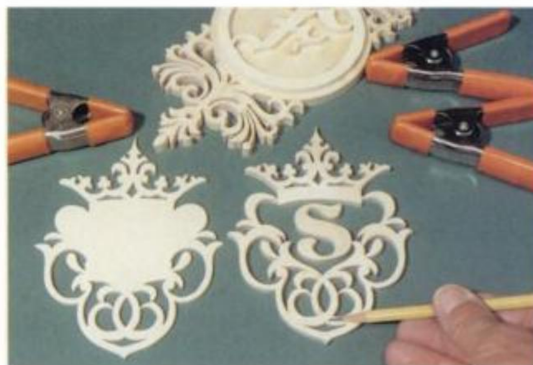
10-6. The outside perimeters of both the backer and overlays are stack-sawn together and then separated for sawing the inside openings.
