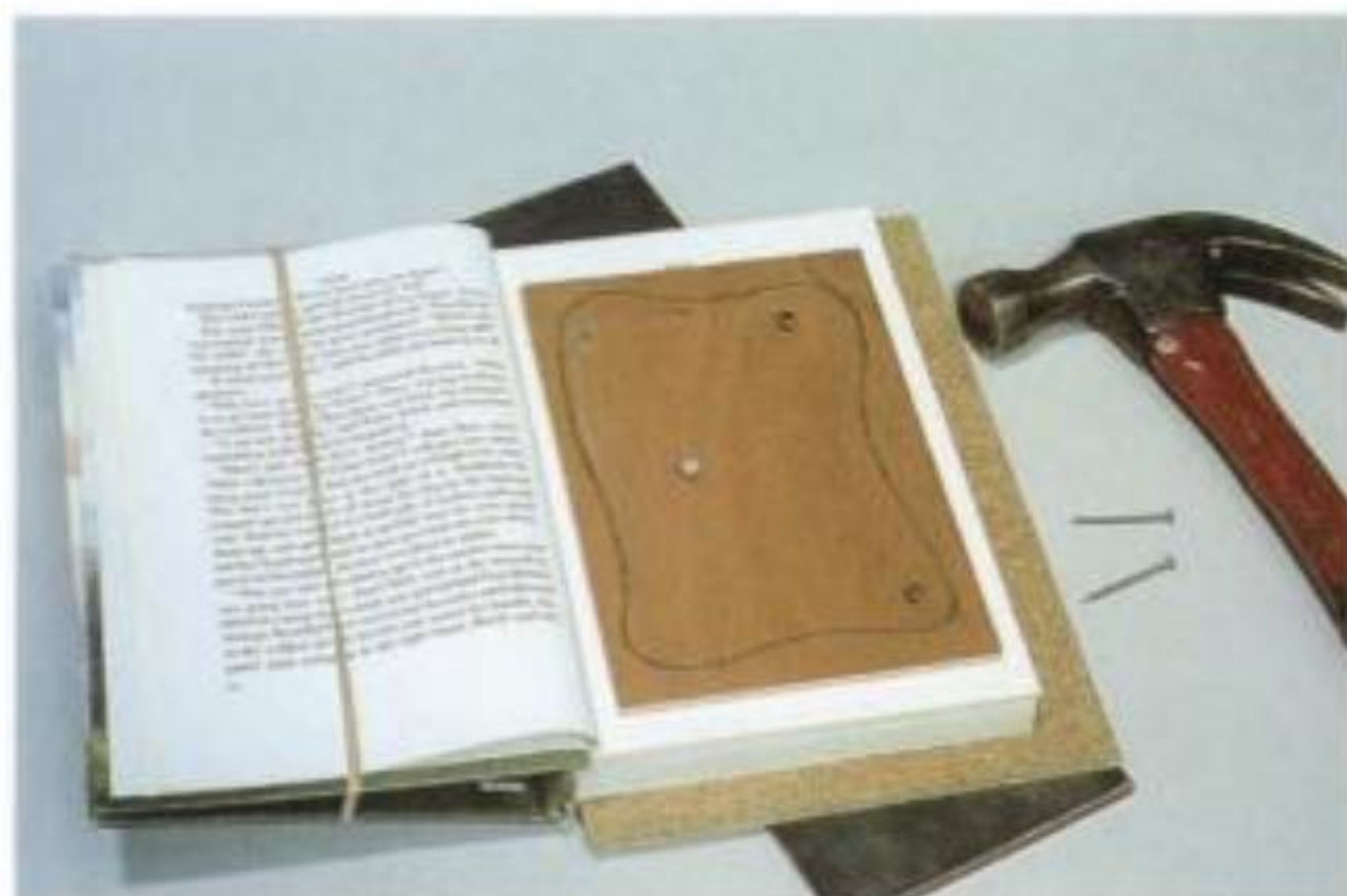
9-2. With both covers turned back, nail the inside pages together sandwiched between two pieces of waste plywood. Notice the metal plate.
