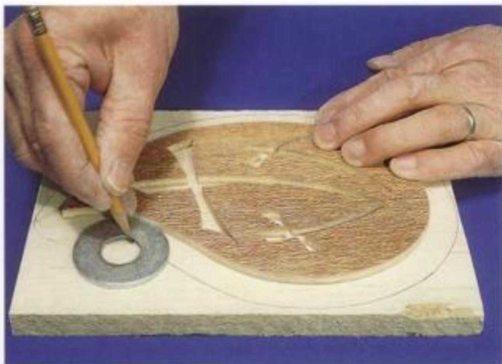
4-5. Drawing a line parallel to an irregular edge with the aid of a metal washer.
