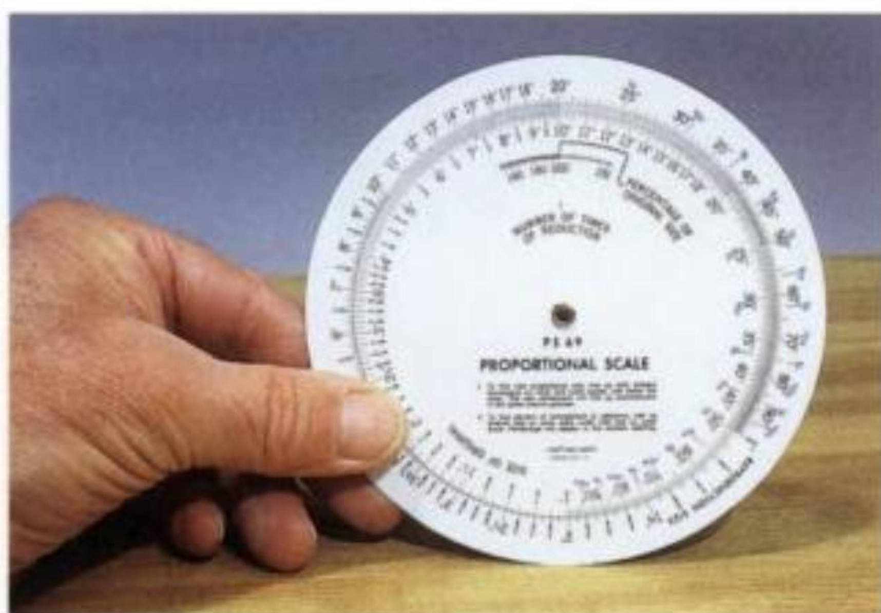
1–10. The proportional scale will quickly determine the exact percentage of enlargement or reduction when using the photocopy machine.
