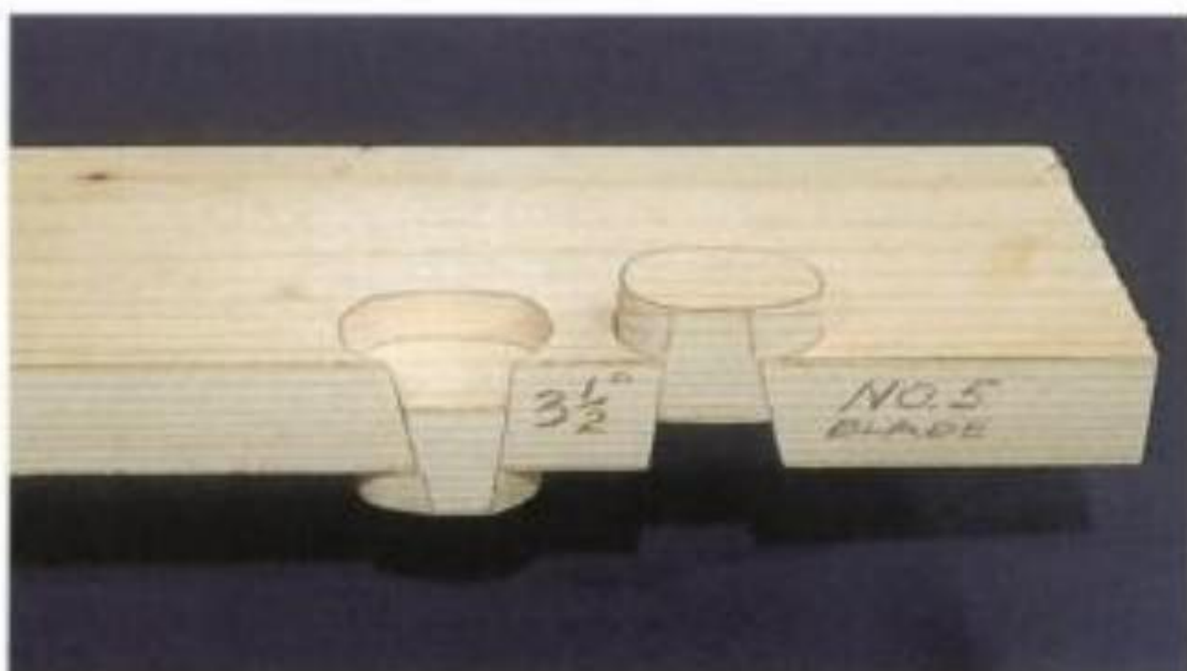
9-16. Test bevel cuts made with the table tilted left. Feeding the work counterclockwise into the blade creates a recessed surface (left) and feeding clockwise will produce a cut piece raised in relief (right).
