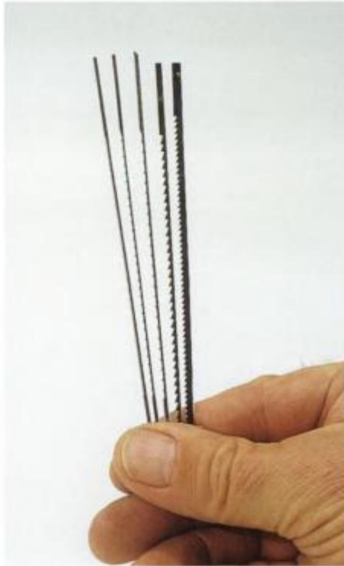
1-7. A variety of scroll saw blades. As a rule, use smaller blades for thin stock, tight turns, and small spaces. Use larger blades for thicker stock and larger curves.
