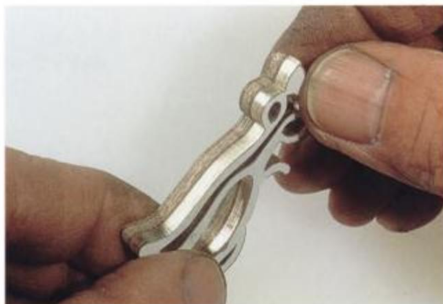
2-16. The edge is relatively smooth on this piece of brass sawn while supported on a waste wood backer.
