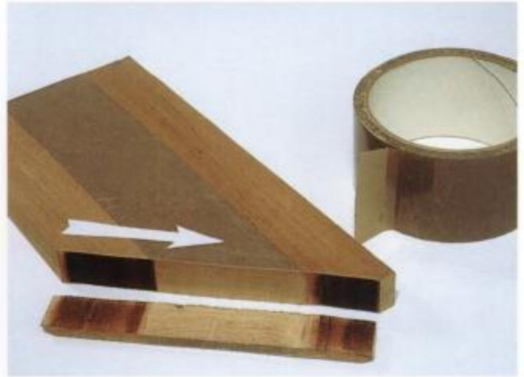
I-17. This photo clearly shows the dramatic effect plastic packaging tape has in alleviating burning tendencies when sawing solid cherry or other difficult-to-cut materials. A worn blade was used throughout the cut, in a left-to-right feed direction. Notice how the finish quality improved in the central area where the surface is covered with the packaging tape.
