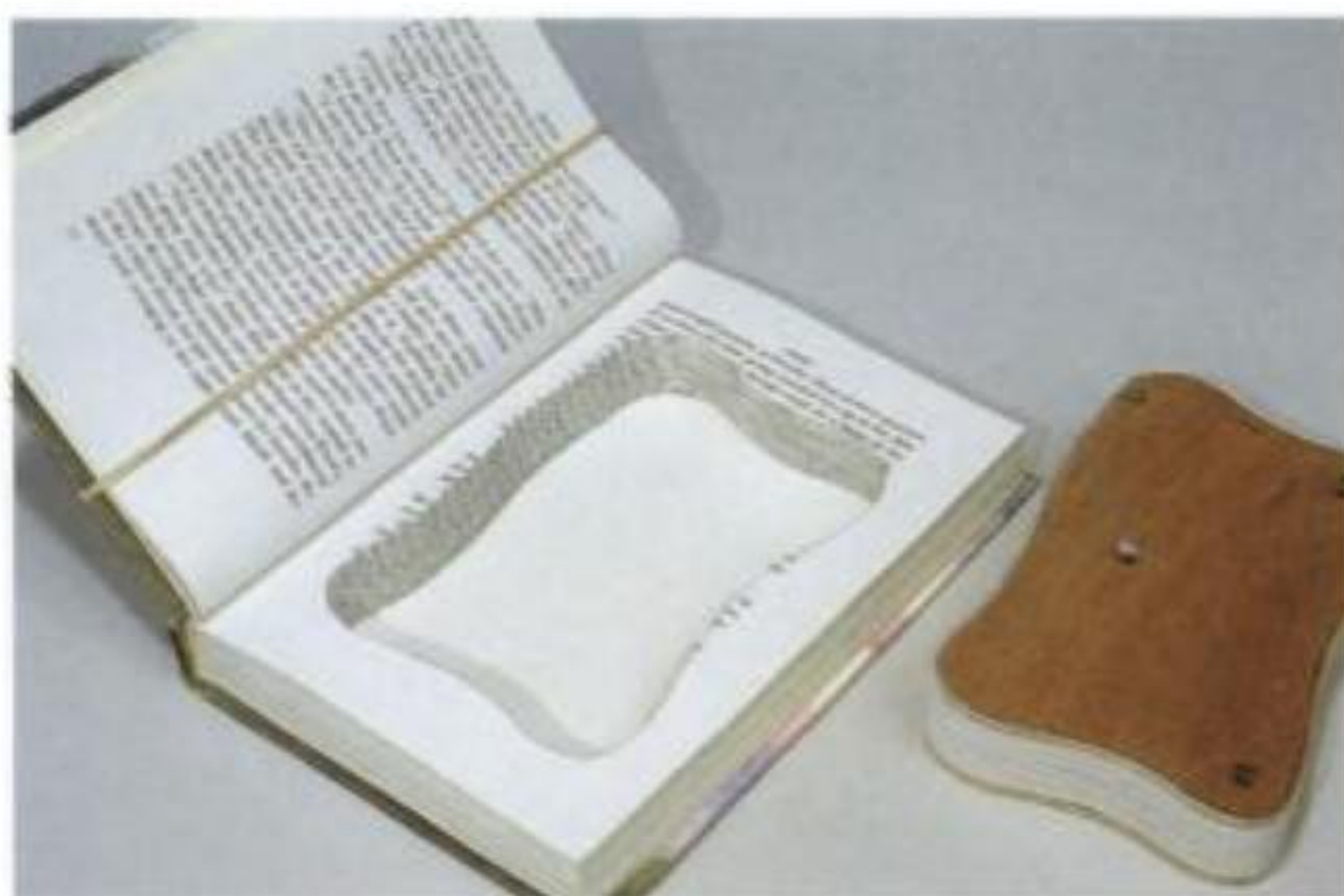
9-4. The completed compartment, neatly cut, and the stack of waste.
