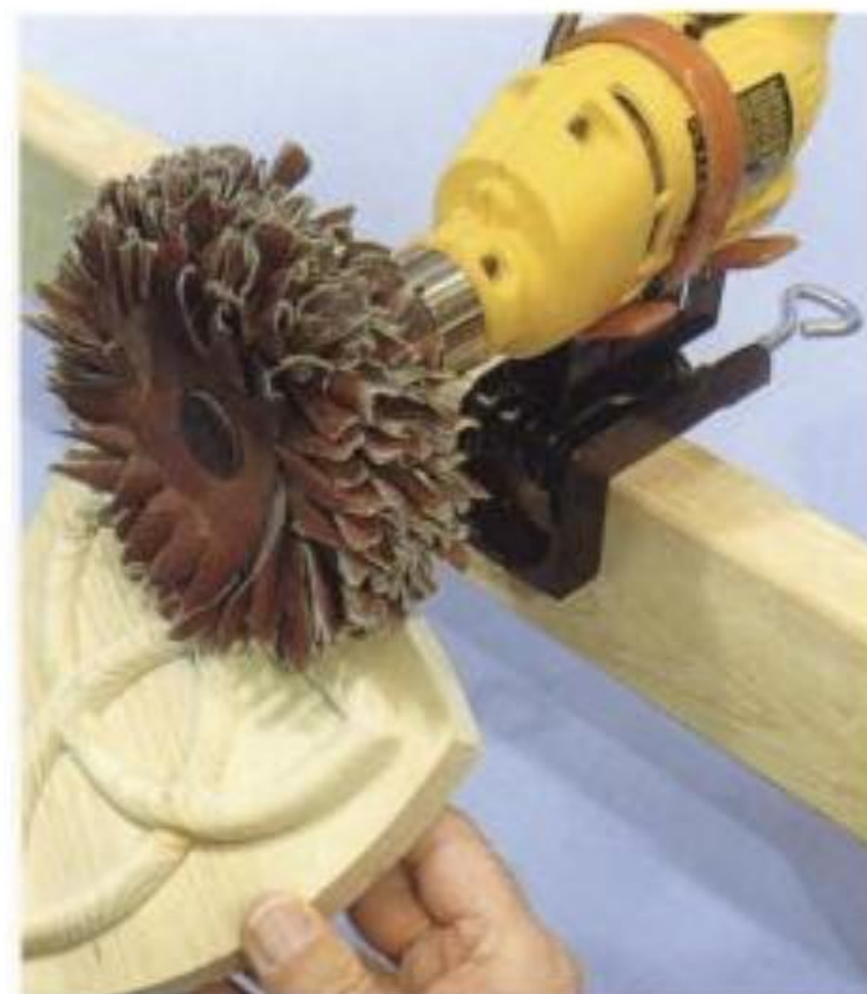
9-23. Shaped and sanded parts glued in place get a final sanding with a flutter wheel. (See 9-15 for glue application.)
