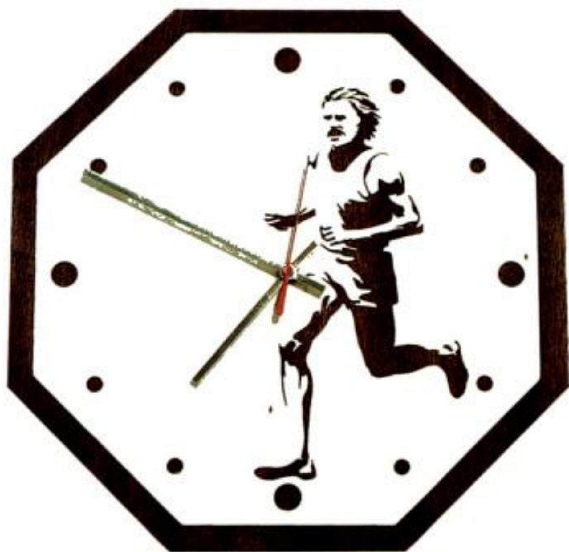
7-14. The sports clock consists of pierced \frac{1}{8} -inch-thick birch plywood over a \frac{1}{4} -inch stained plywood backer.
