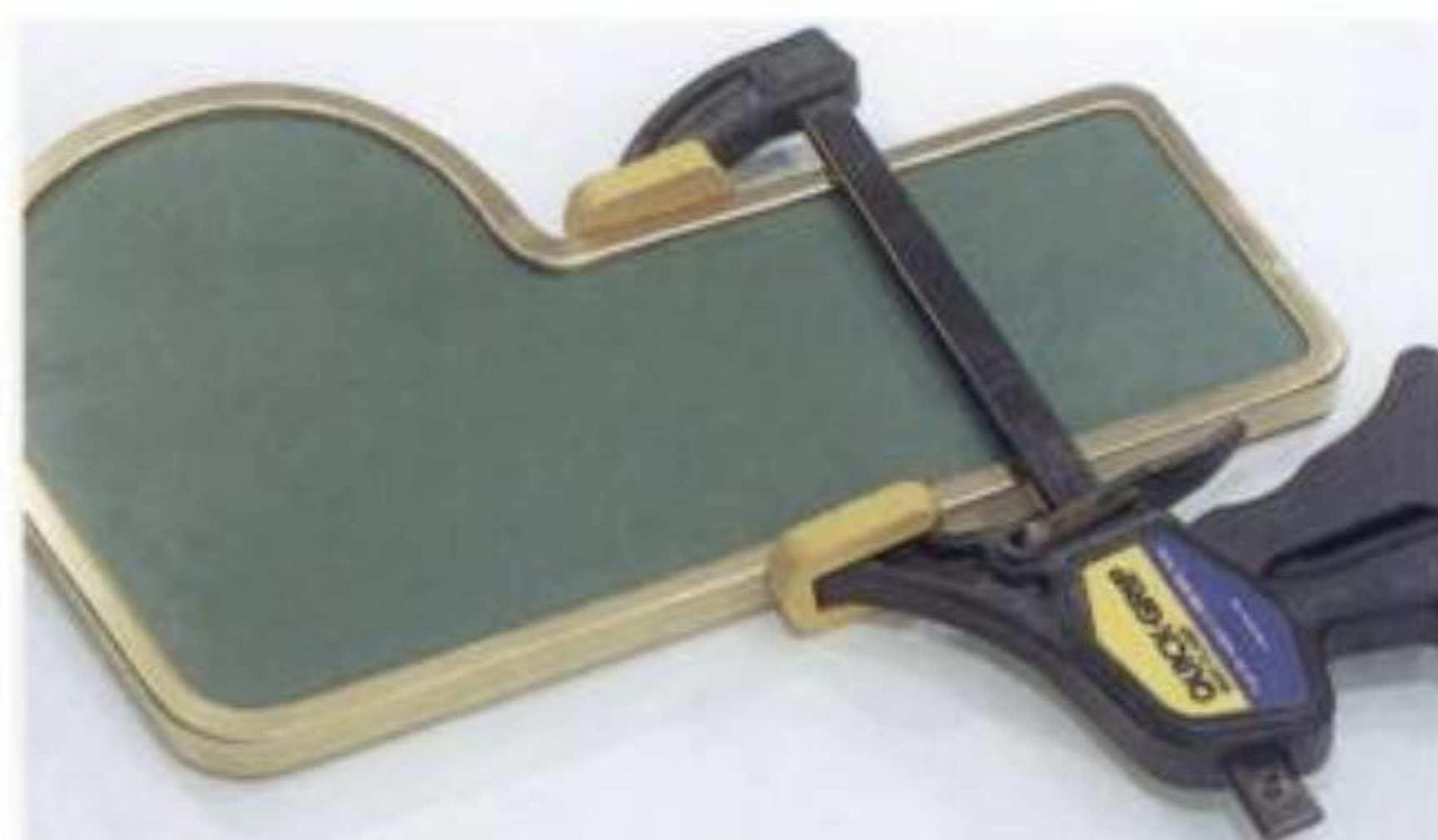
10-4. Moderate clamping pressure is necessary to eliminate the tendency of a gap from developing at this area when gluing the border in place.
