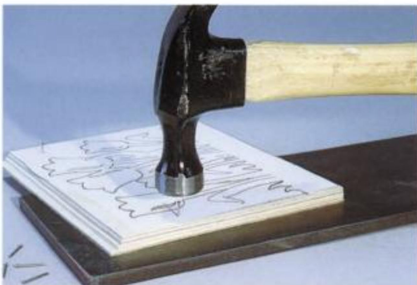
1-14. Driving brads through several layers of very thin plywood for stack-sawing. When done over a steel plate as shown, the nail points peen so they will hold the bottom layer secure and not scratch the saw table during cutting.
