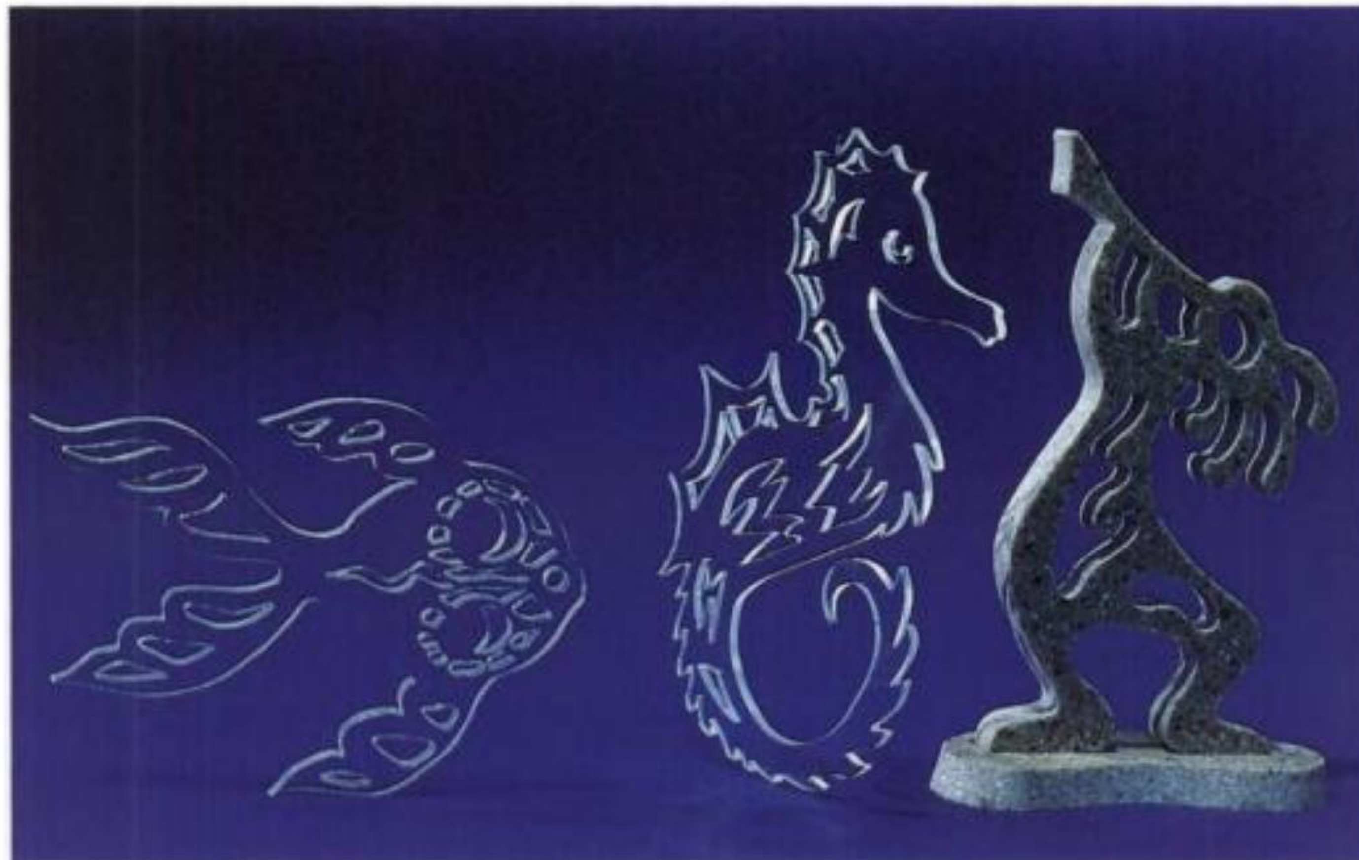
1-3. Acrylic sheet plastics are available in clear, translucent, solid colors, and mirrored types. Corian (shown on the right) is one of various hard surface materials that cut extremely well with the scroll saw.
