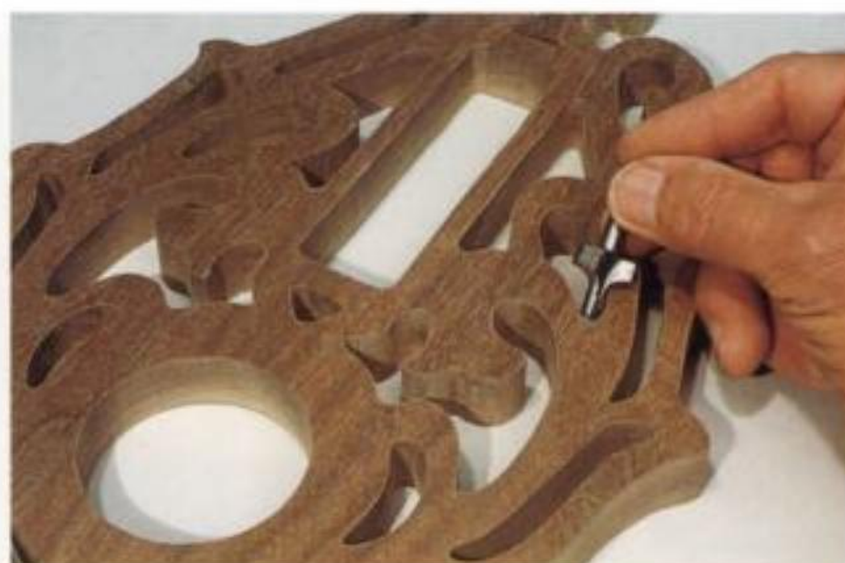
7-21. Use a round-over bit with an integral pilot as shown to round over the clock's edges.
