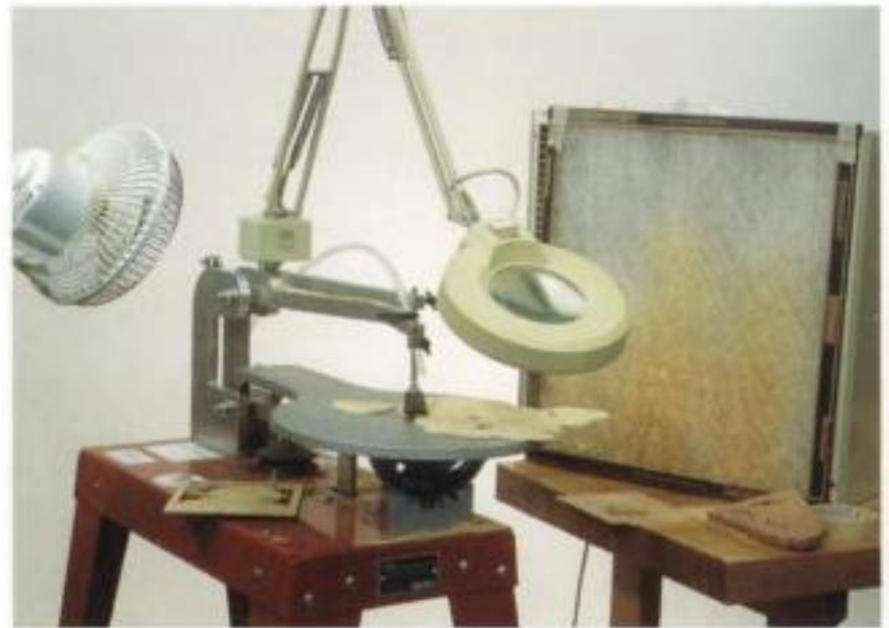
1-9. A practical setup that collects airborne scroll-sawing dust and also works well for sanding, routing, and other dust-generating jobs. At right is a square household fan with a furnace filter taped to it. To the left, a small second fan to help move the air.
