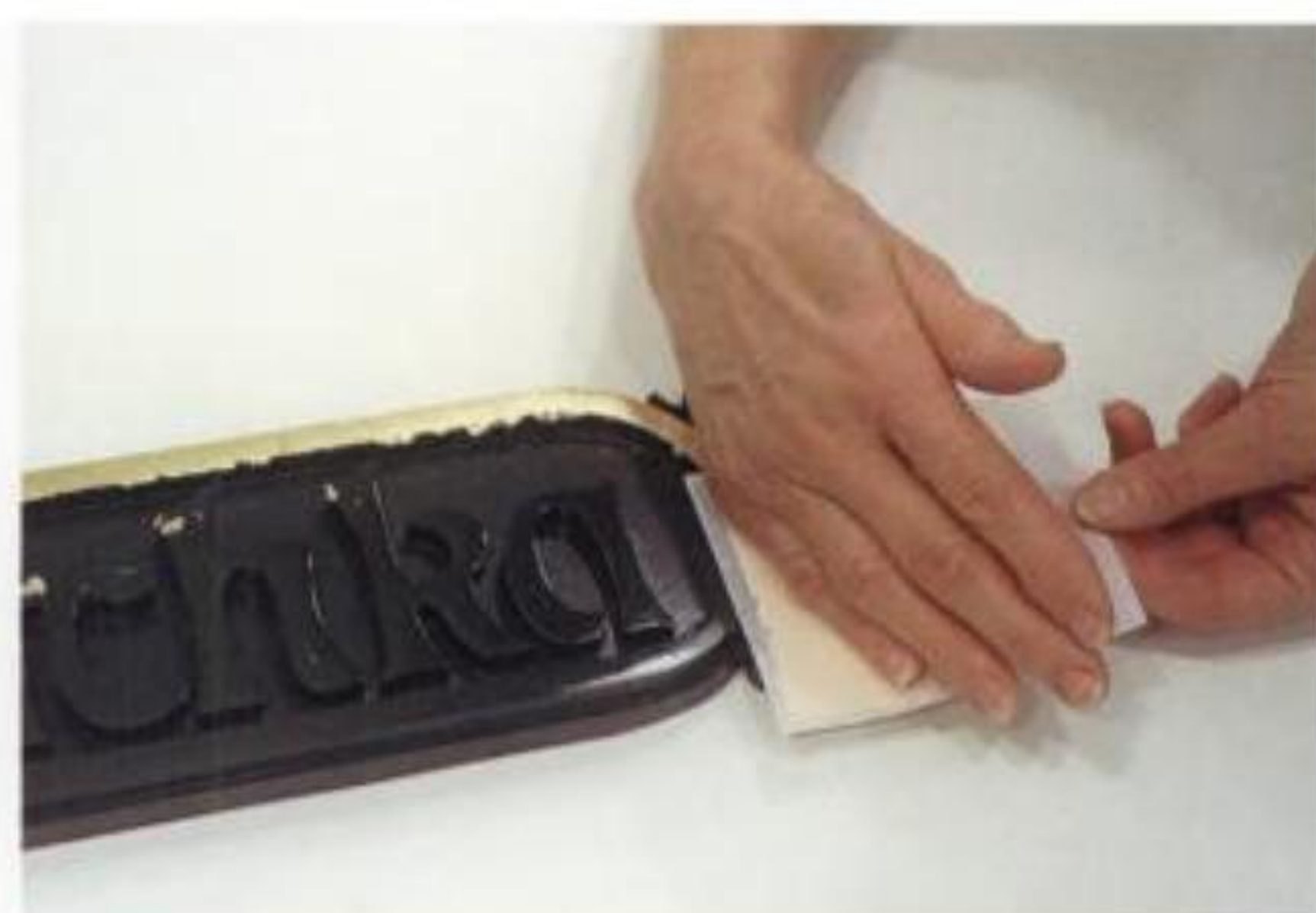
10-14. Laying down the gold leaf. Use the side of your hand to apply moderate pressure. Apply each piece overlapping the previous one about \frac{1}{8} inch.
