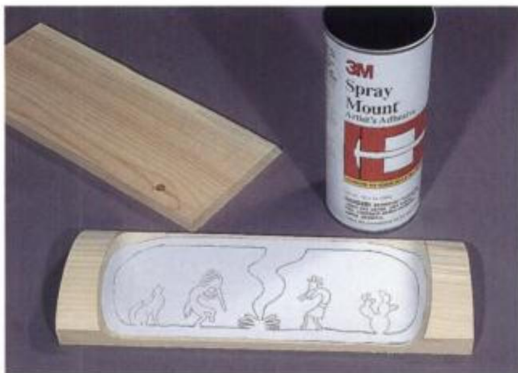
11-4. Apply the window silhouette pattern; center it on the workpiece.
