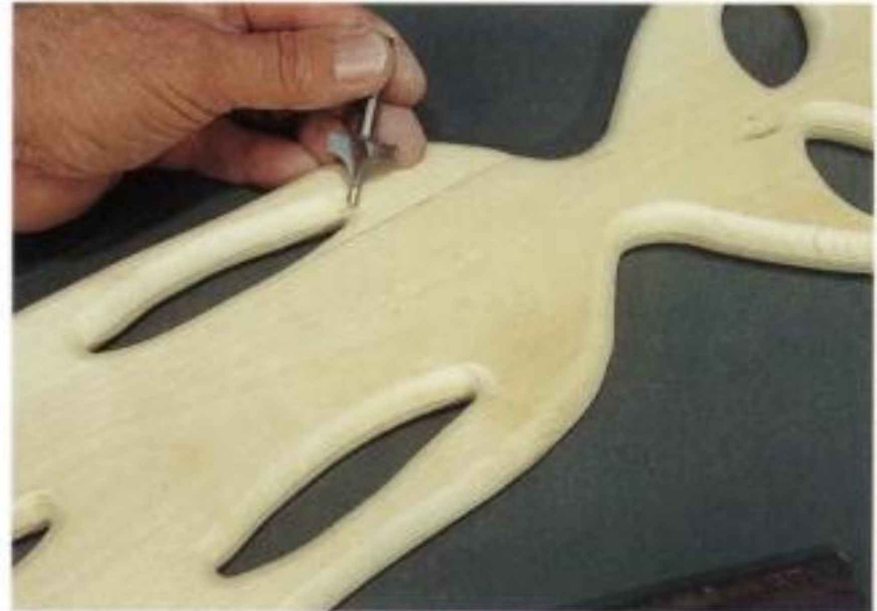
2-28. Rounding over the edges using a bit with a small integral pilot that gets into tight corners.
