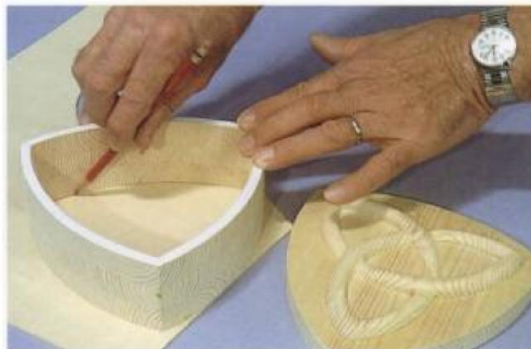
9-26. Tracing the inside of the box on plywood, which is then sawn and tacked (without glue) under the lid to keep it aligned.
