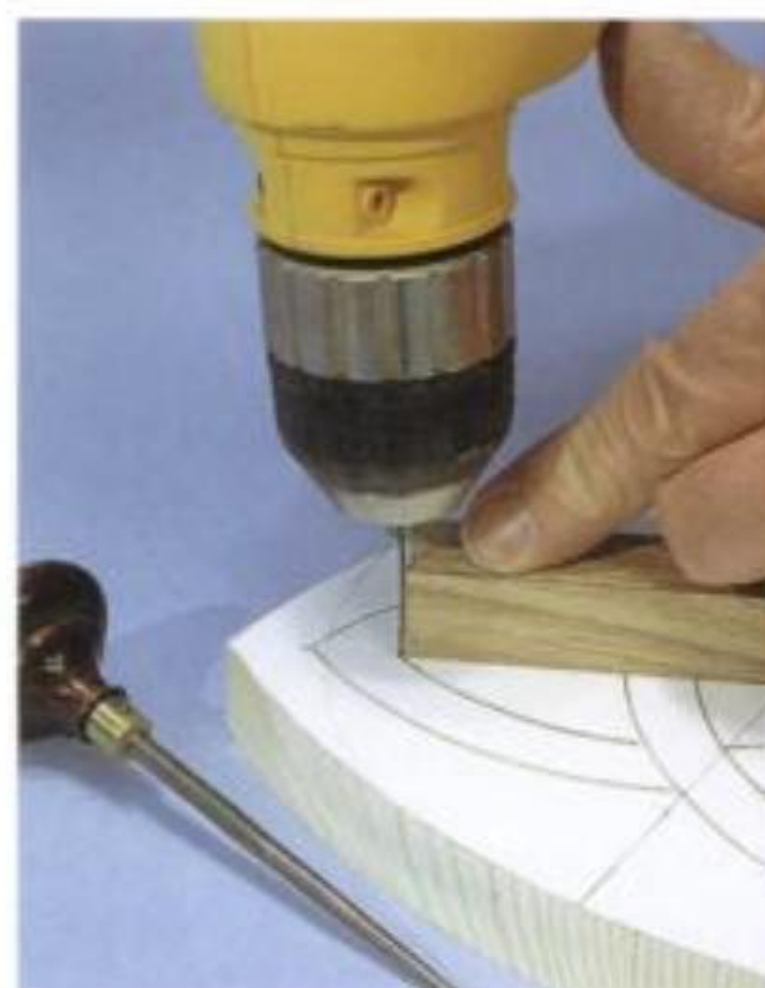
9-17. A small stick cut at the correct angle guides the drill direction.
