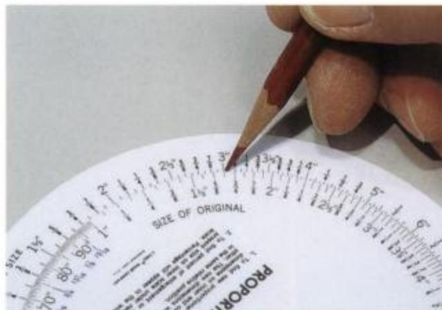
1–11. Simply rotate the scale to match up marks indicating the size of the given copy to the mark indicating the new copy size desired, as shown. Then read the percentage given in the proportional scale’s window.
