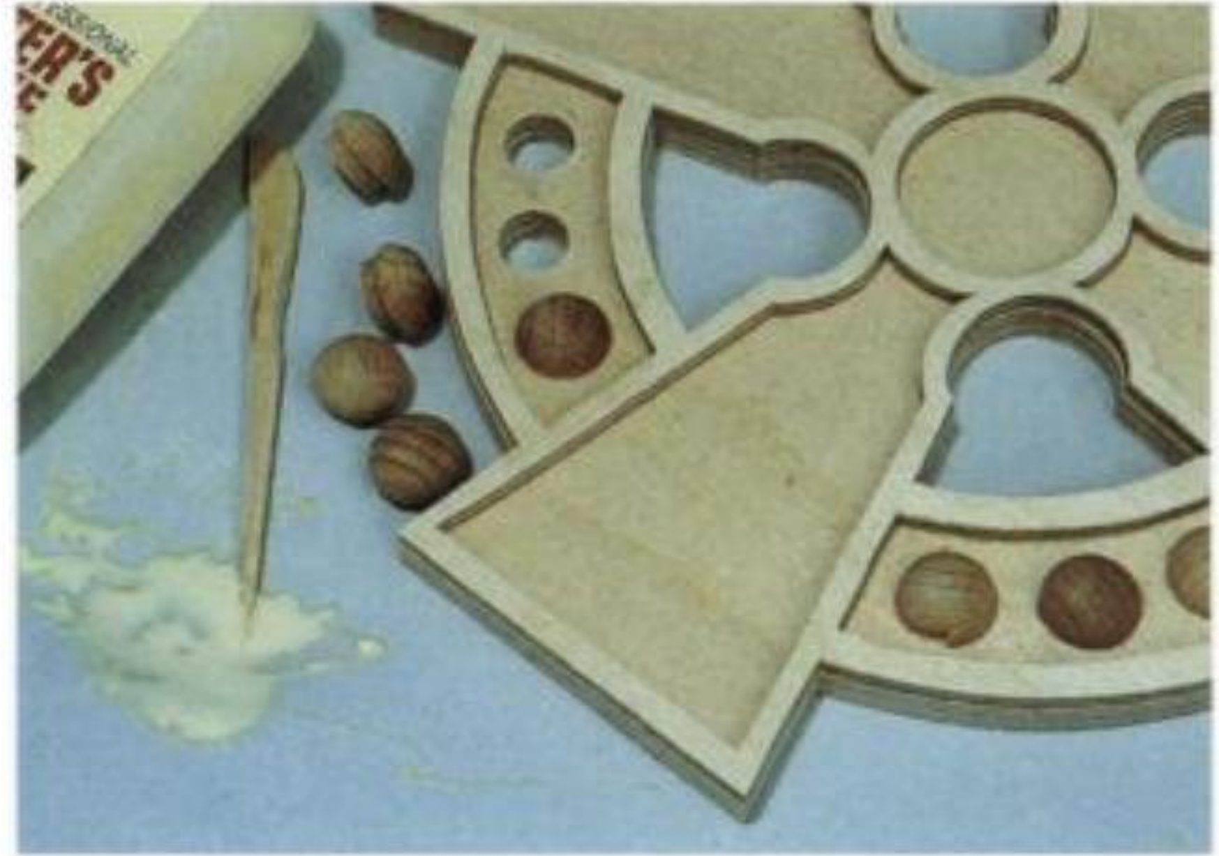
4-17. Gluing in the screw-hole buttons.
