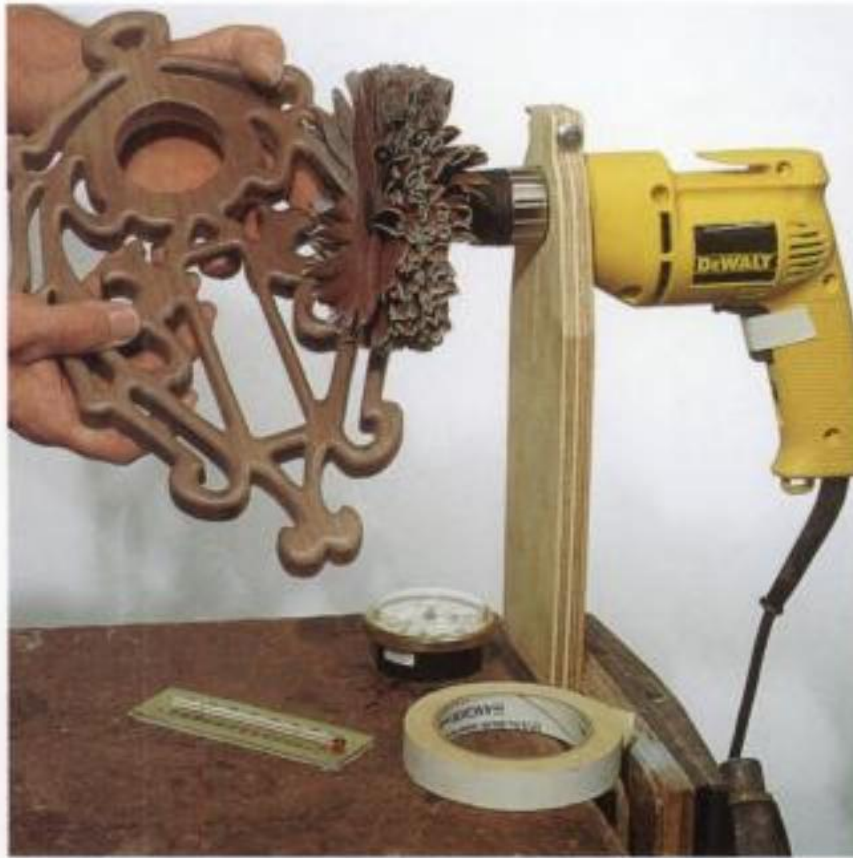
I-16. Using a flutter wheel removes feathering, softens sharp corners, and smooths routed edges as shown.
