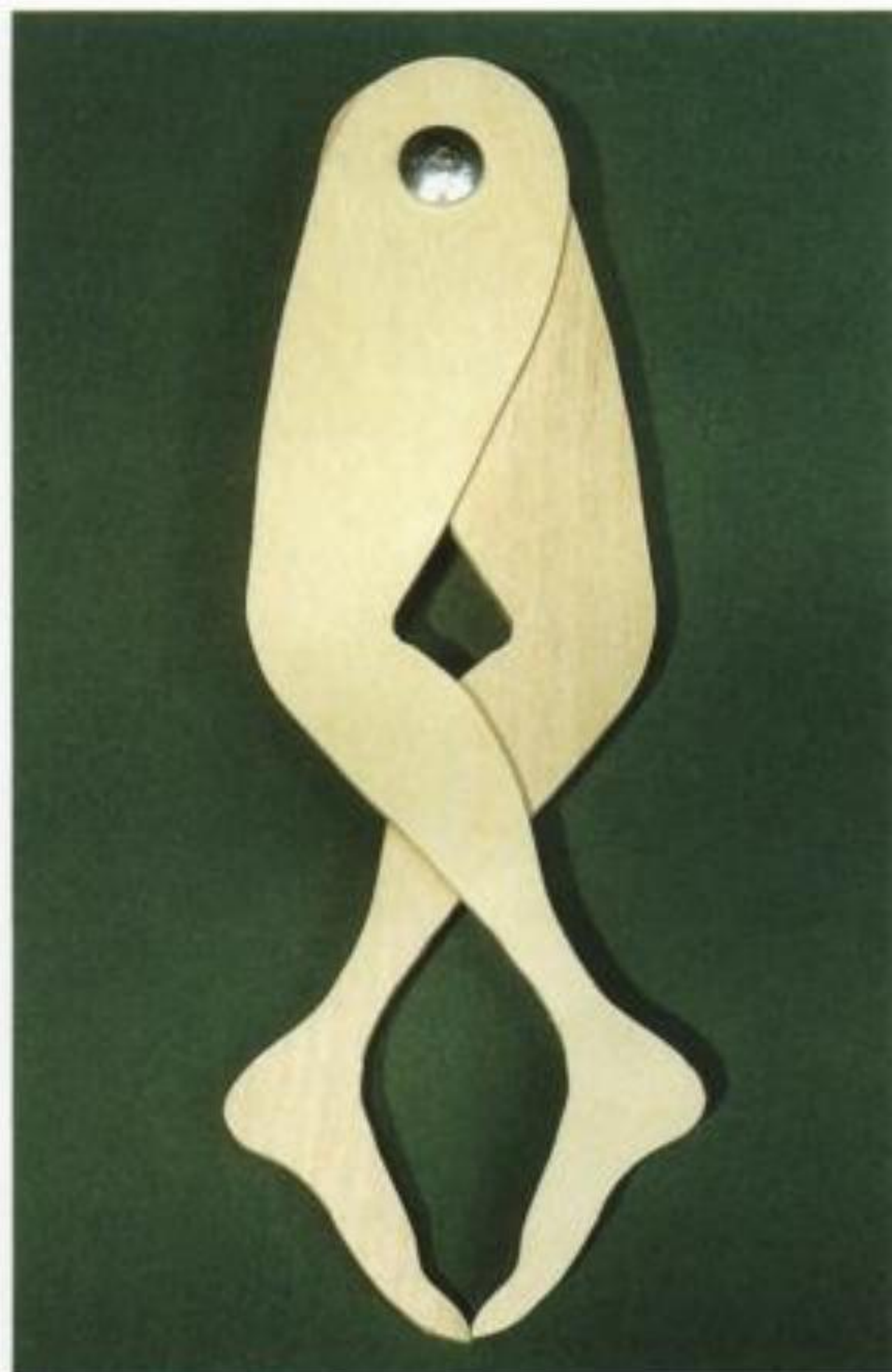
2-3. This caliper, based on a century-old design, is a fun project to make and have around any shop.
