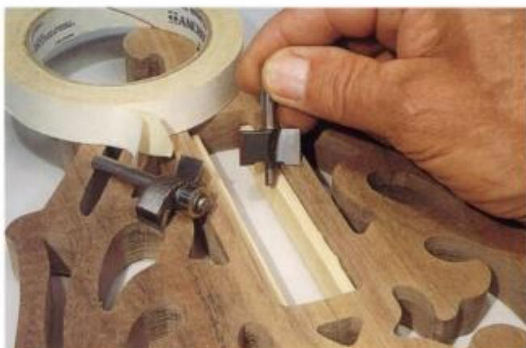
7-20. Double-faced tape holds small strips in place for routing to create a \frac{1}{8} -inch rabbet when using a typical \frac{3}{8} -inch rabbeting bit.
