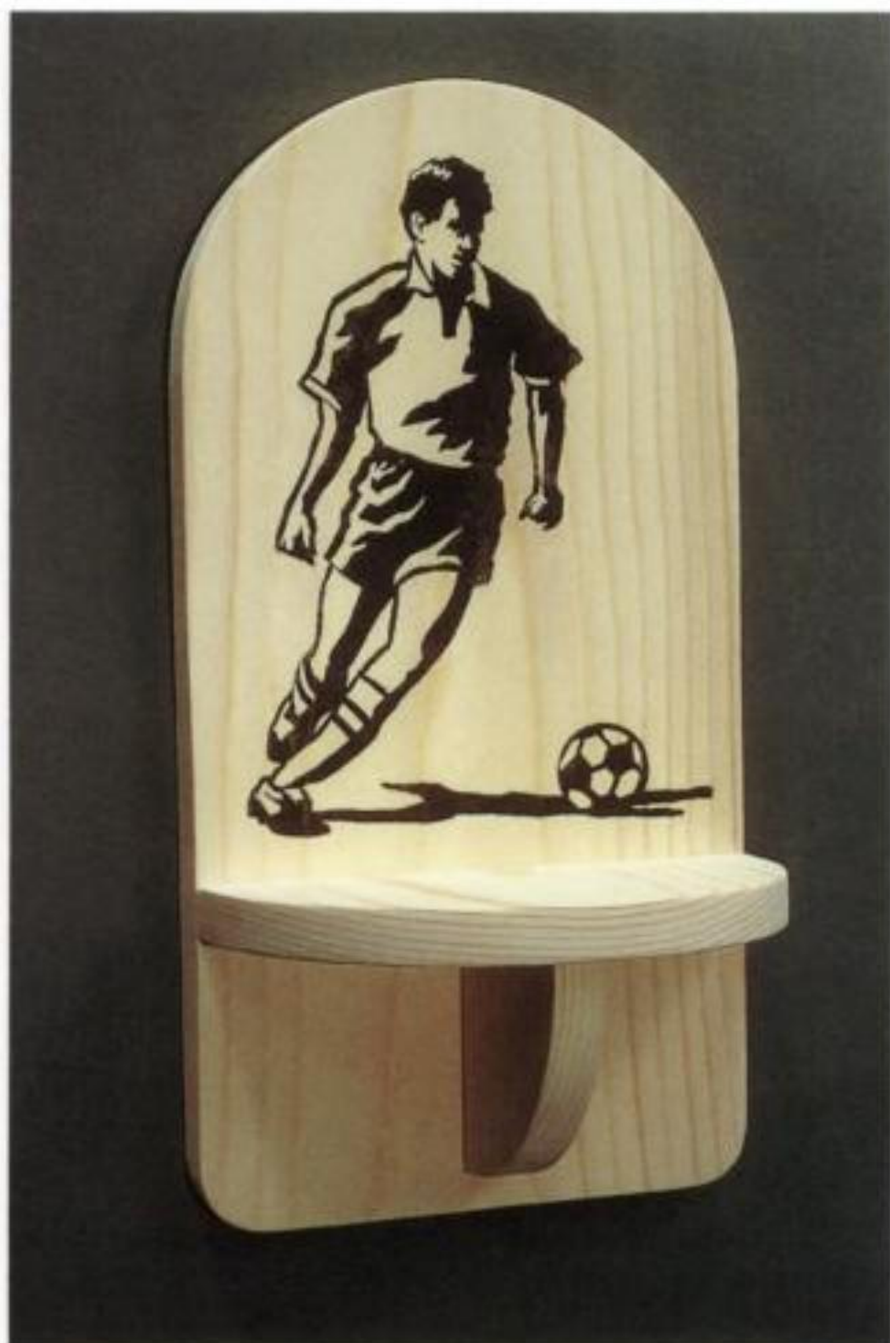
6-7. This easy-to-make shelf can be decorated with any suitable thin plywood overlay or, more quickly, decorated with an electrically heated "image transfer tool" that transfers photocopied graphics to wood surfaces.
