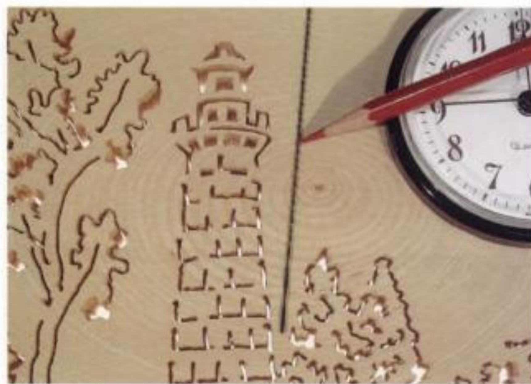
7-11. Close-up view that shows the wide kerf and rough-sawn surface produced with large spiral scroll-saw blades.
