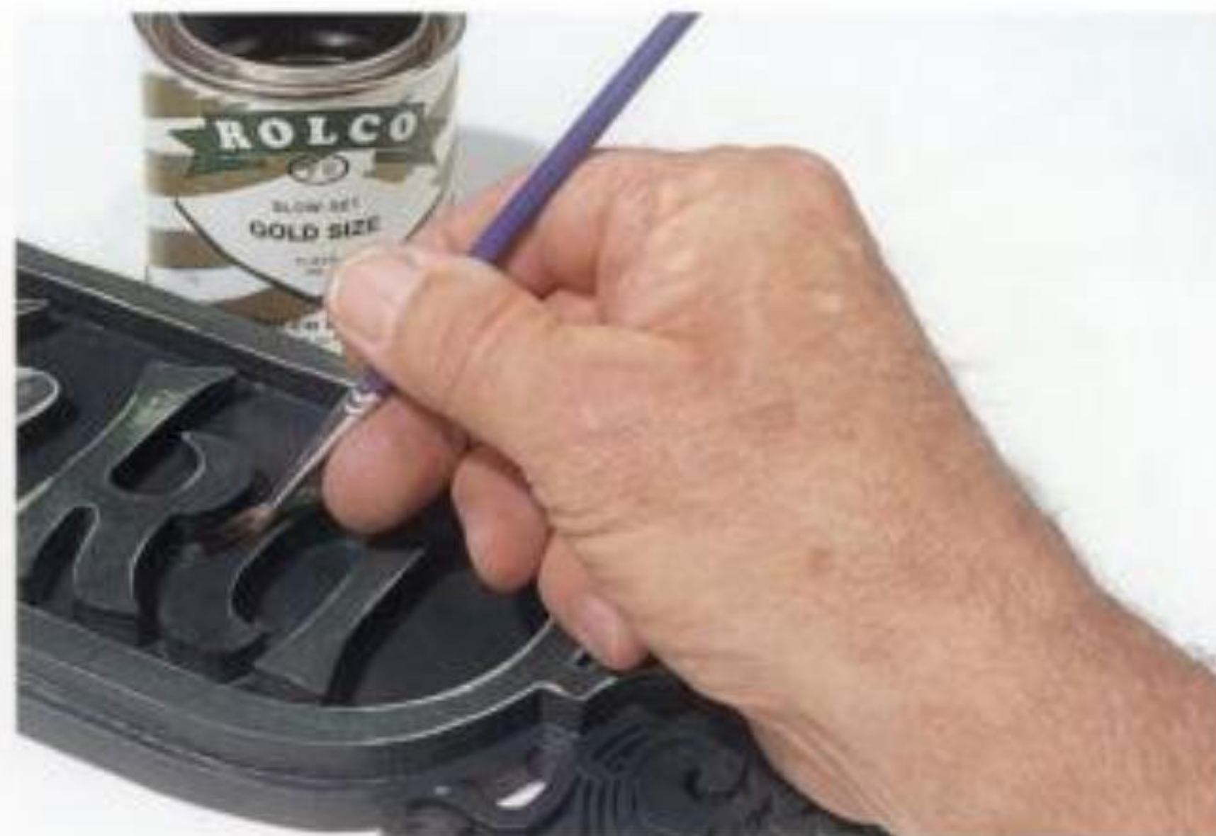
10-11. Carefully brush on the "size" (adhesive) for the gold leaf.
