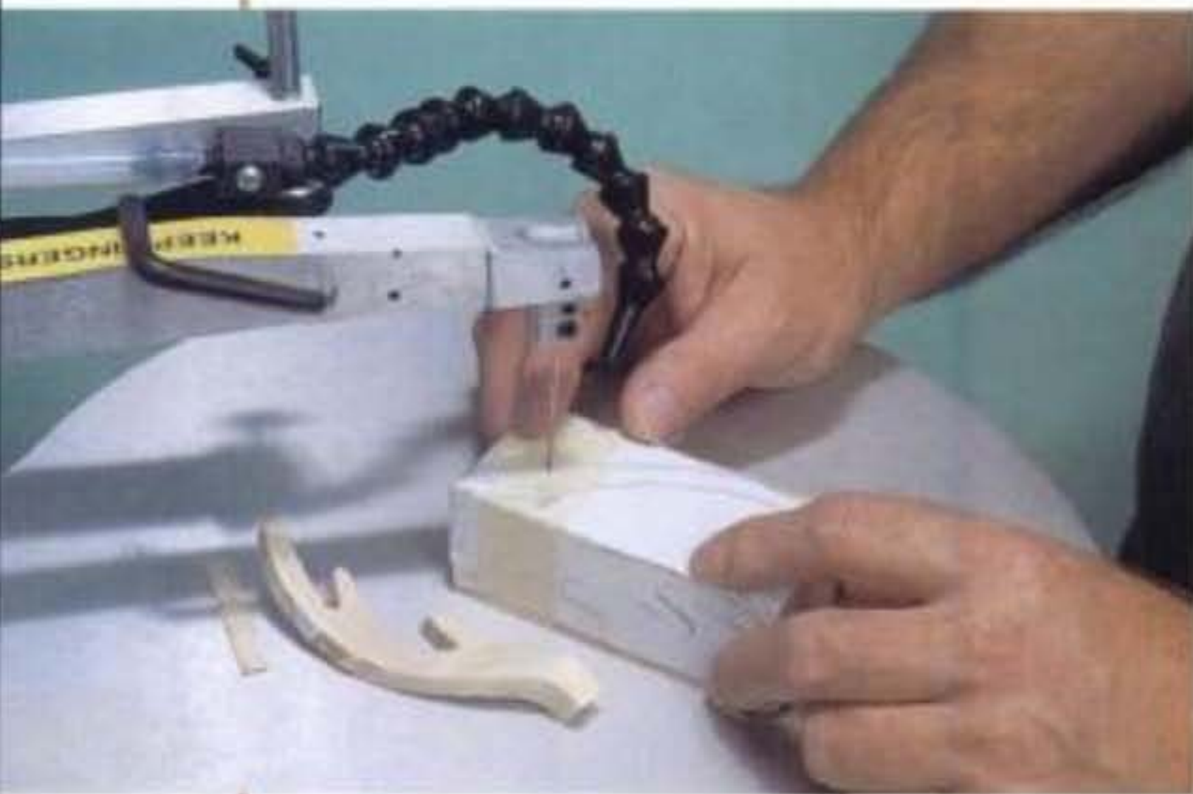
Making the "second cut" on the same antler piece. Note the sample antler piece sawn out and partly shaped with its corners rounded.
