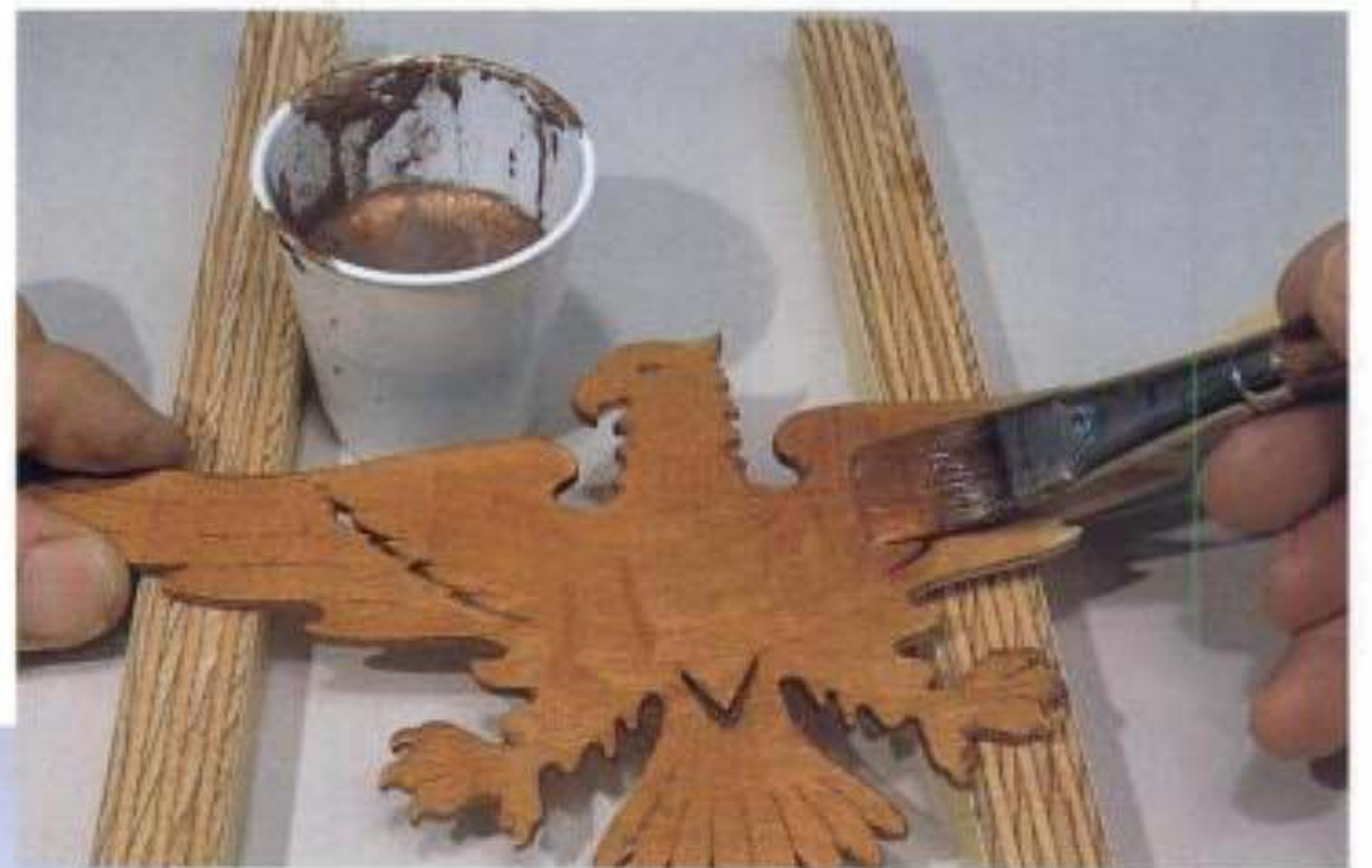
Preparation for an easy-to-achieve patina finish on 1/8" plywood. First the project is coated with a clear sealer followed with a coat or two of water-based bronze or copper liquid metal, as shown here.
