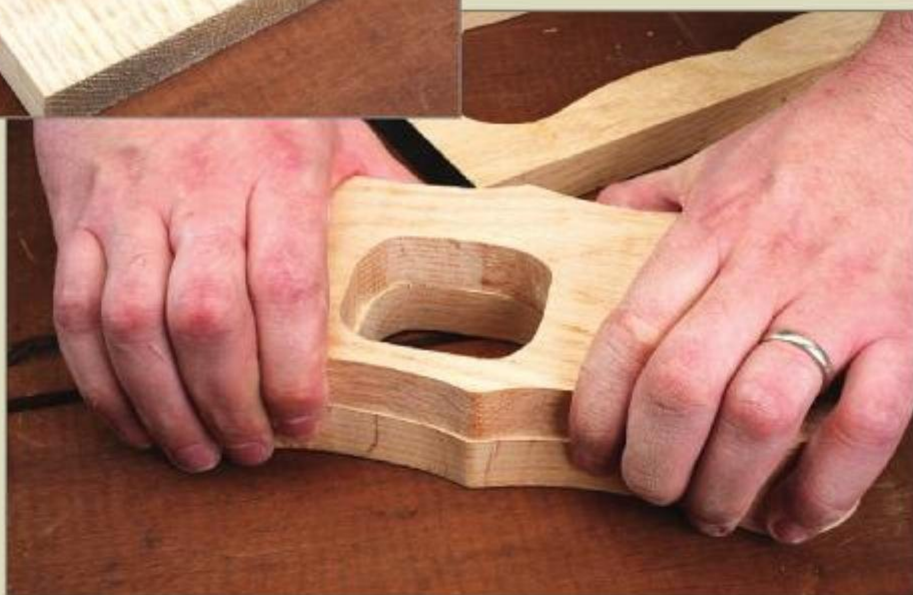
Figure 10. Once both pieces have been cut, line them up, attach them with screws, and sand the area where they meet until it is flush.
