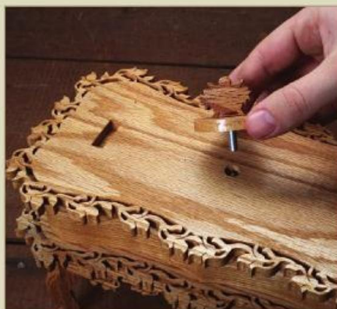
Figure 17. Attach the metal turntable to the wood and attach the figure to the top of the wood. Then, screw the turntable into the music box movement. Our movement had room for only a key or a turntable, so we will use the turntable to wind the movement.
