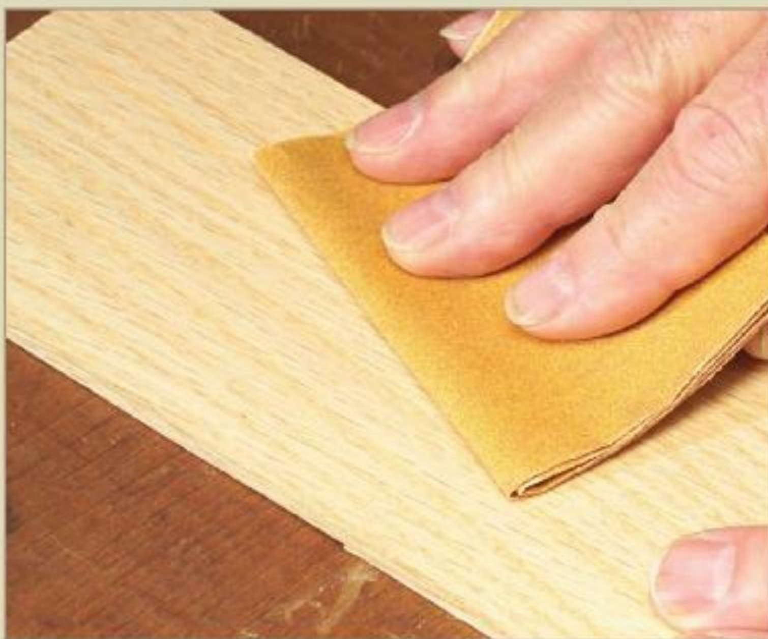
Figure 1. Be sure to sand the workpiece before applying the pattern. You may also want to sand the wood lightly once you have cut the design and removed the pattern to eliminate any “fuzz” and to get rid of any glue residue.
