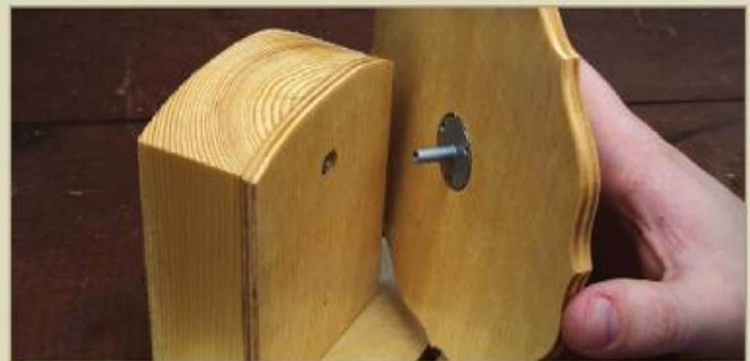
Figure 15. Attach the metal turntable to the wood turntable and thread the metal turntable onto the music box shaft.
