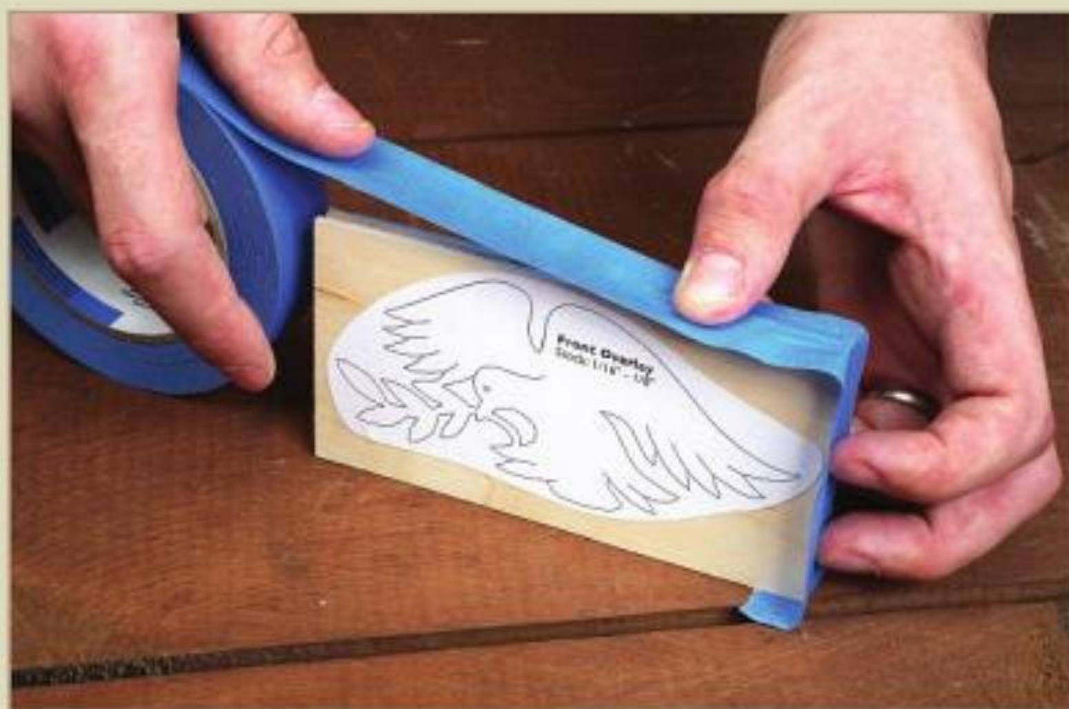
Figure 11. Masking tape or painter's tape (shown) placed around the edges can be used to hold a stack together. Some scrollers also like to cover the surface of the wood with tape before adhering the pattern to help lubricate the blade as it cuts. Placing double-sided tape in the corners of the stack can also be an effective method of holding the stack together.
