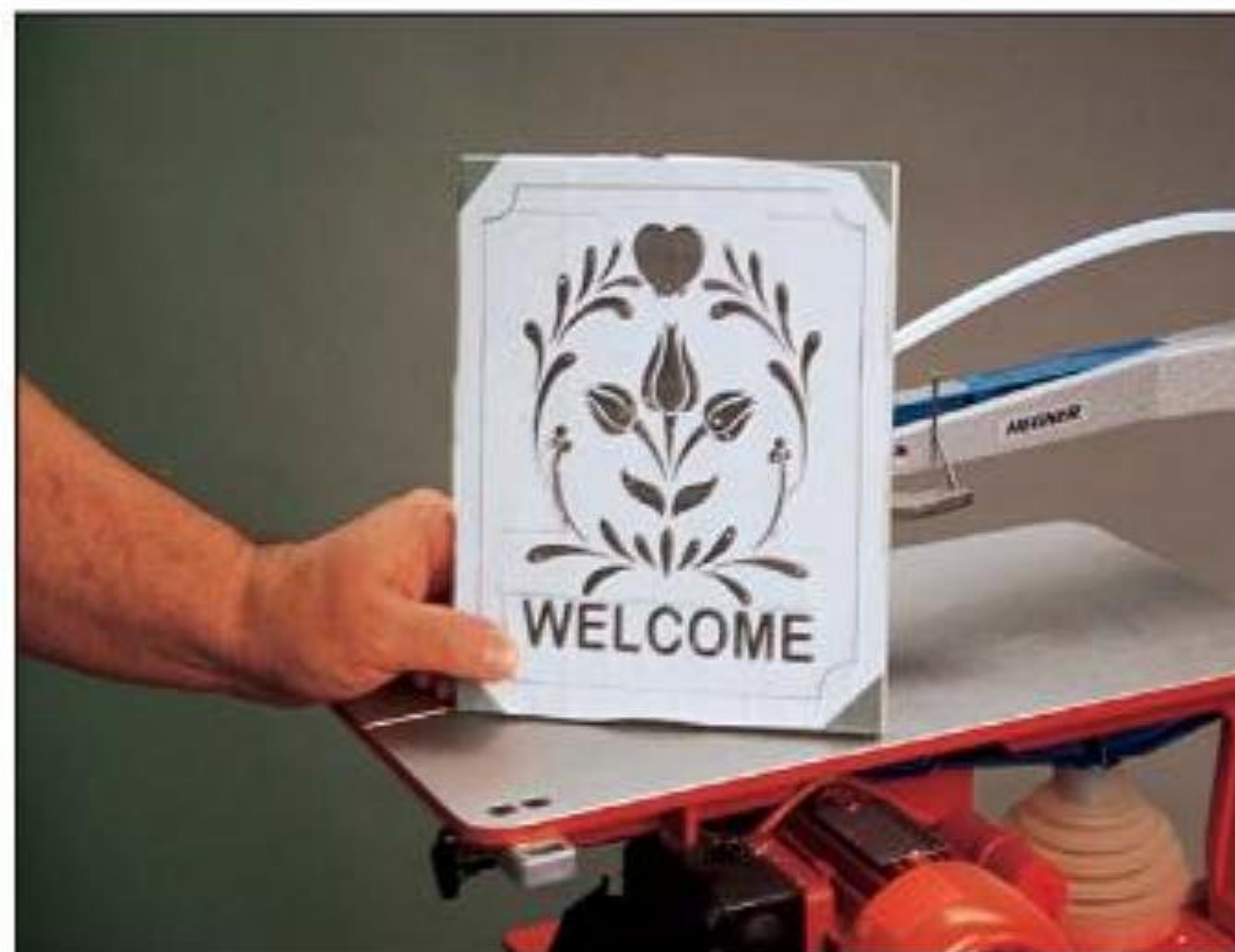
Covering the bases: Apply the pattern to the duct tape immediately after gluing and let it set for about five minutes.
