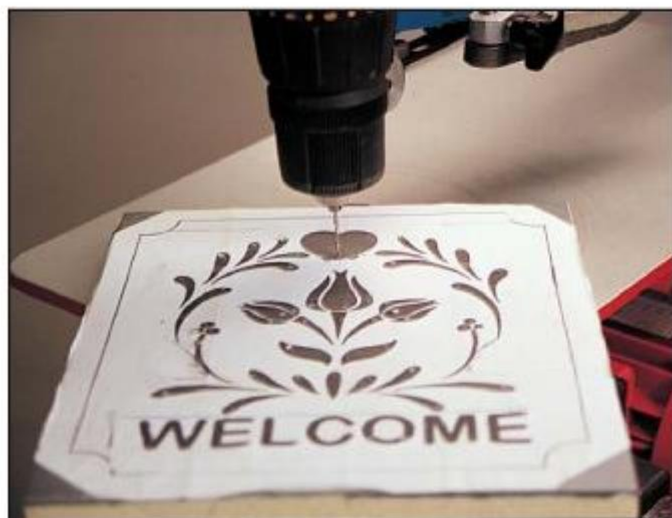
Drilling down: Use a \frac{1}{16} " drill bit to make the blade entry holes for the Floral Welcome Trivet's inside cuts.
