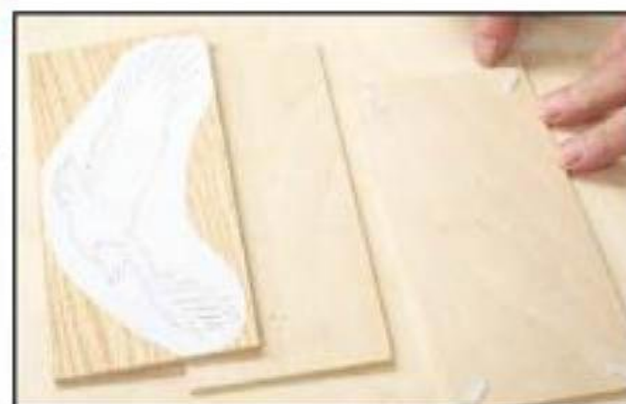
Use double stick tape in the corners to attach pieces for stack cutting.
