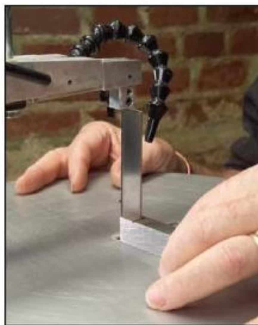
Ensure your blade and table create a 90°-angle using a square.
