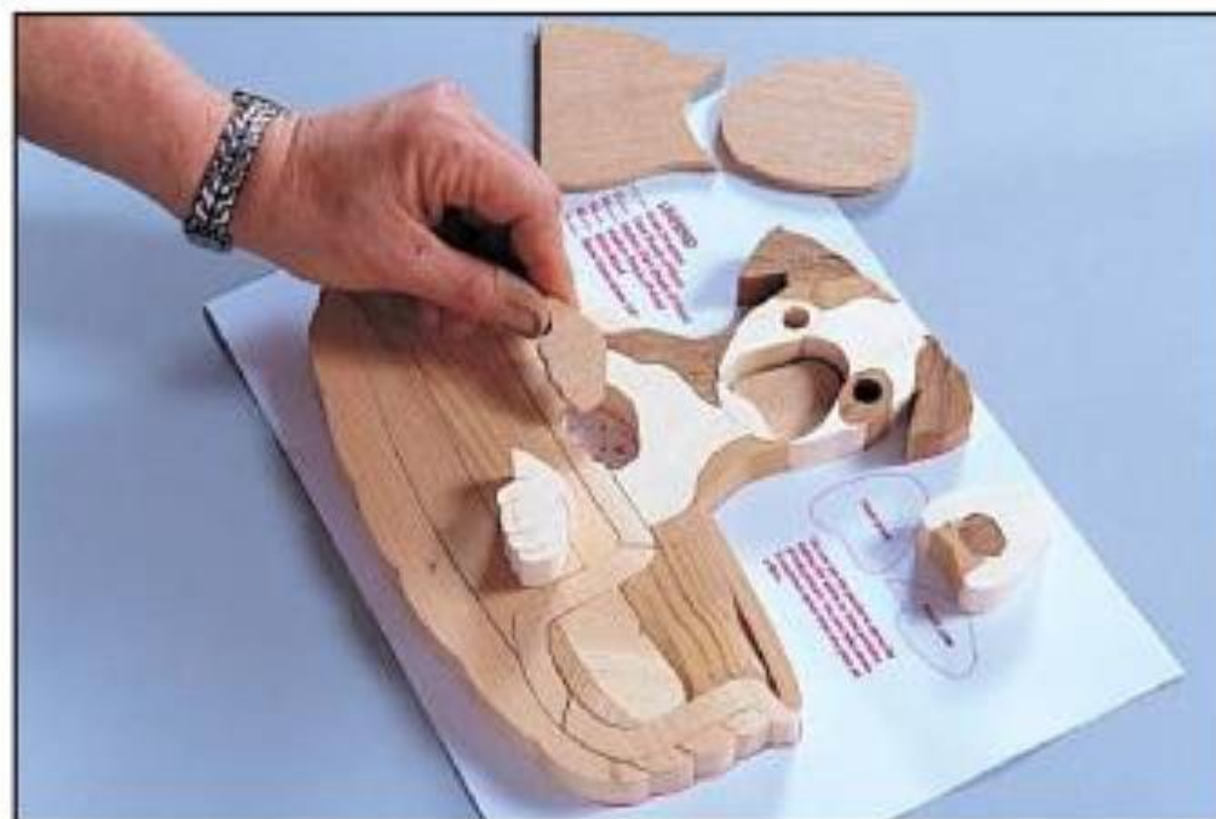
Step 4: Sanding shims for the puppy's face, neck, and body sections make for more consistent contours.
