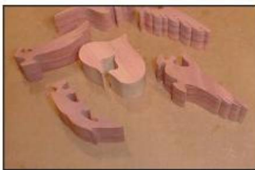
After Sand-O-Flexing, the rough edges are now smooth.
