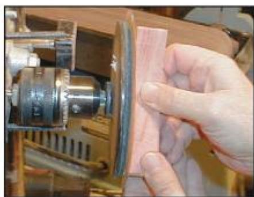
To do both flat and edge sanding, I chuck my disk sander into a drill held in place by a drill stand. Here, I am flat sanding.
