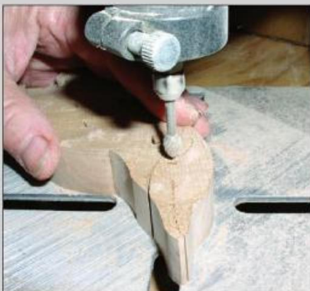
Figure 5.3: You can detail a drilled eye with a teardrop-shaped burr in a rotary power tool.
