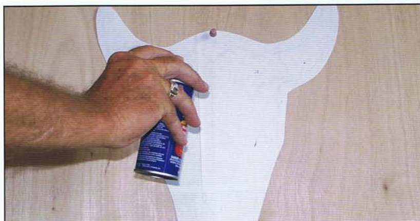
Glue the Pattern to the Wood. Spray temporary bond adhesive on the back of the pattern only.
