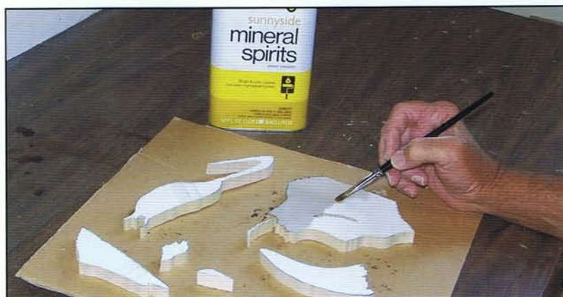
Remove Stuck-On Patterns. Mineral spirits can help to remove stuck-on pattern paper.
