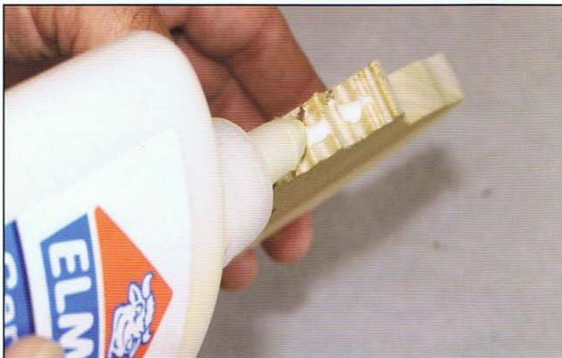
Adding Strength with Glue. Wood glue lends strength to joints but takes time to dry.
