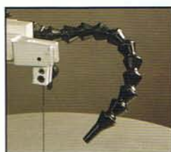
Get Rid of Dust. An adjustable dust blower minimizes dust on the pattern lines.
