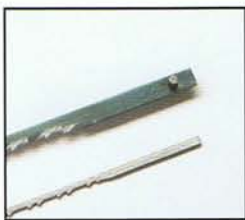
Pin vs. Plain. Choose plain-end blades (bottom) instead of pin-end blades (top).
