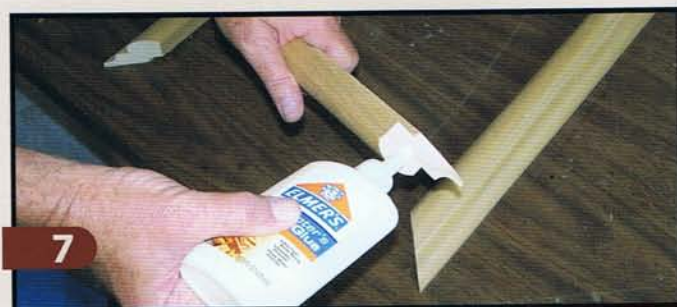
7 Remove the frame clamp and apply wood glue sparingly to the face of the corner cuts.
