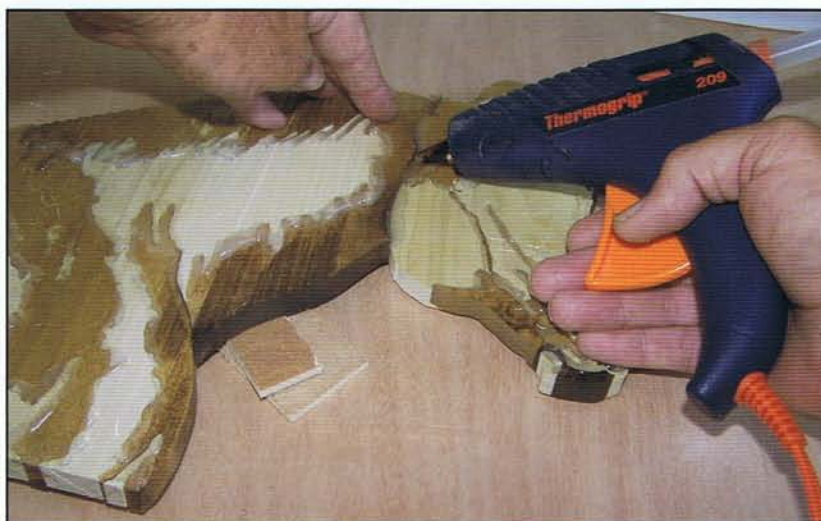
Shims for Assembly. Shims are small pieces of \frac{1}{8} " plywood placed between the segment and the worktable that keep the segment at the desired elevation until the glue sets up.
