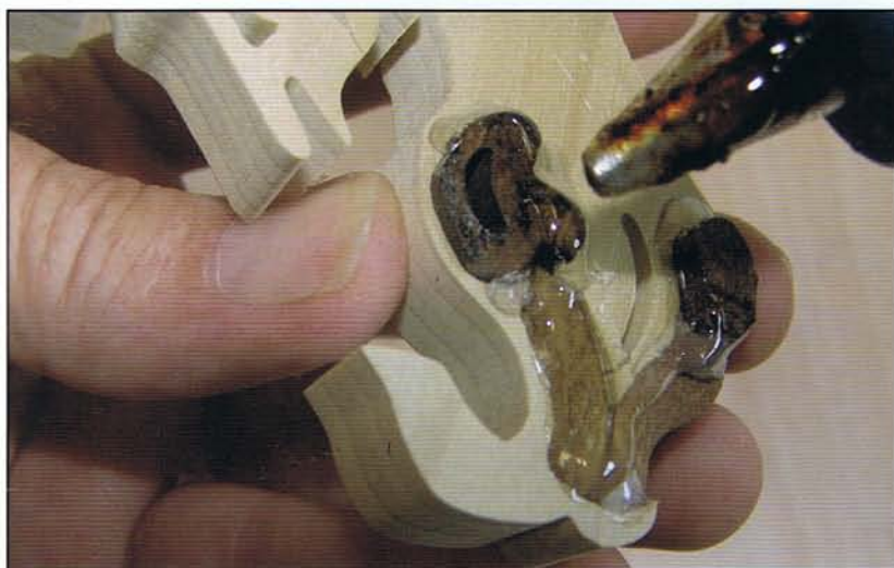
Using Hot Glue. Hot glue dries quickly and holds the relief pieces in place.
