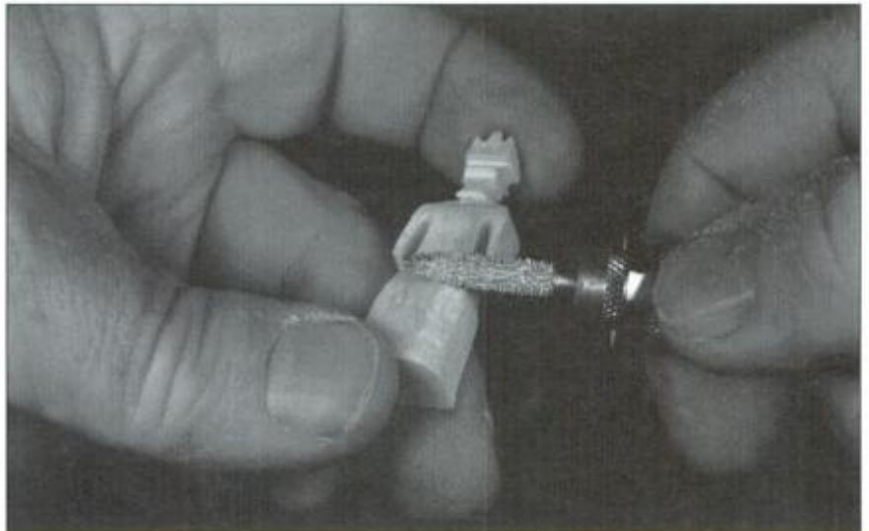
Figure 1.5 A hand-held rotary sanding tool is used to remove the square corners on a Wise Man. The long small-diameter carbide cutter works best for removing square corners of craft items.
