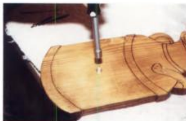
25. Tightening the washer and the hex nut.
