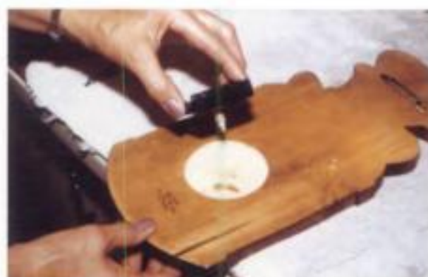
24. Inserting the quartz clock movement. The clock shaft should fit through the \frac{5}{16} " hole.
