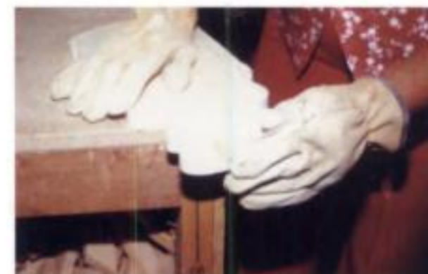
13. Sanding the edges by hand.
