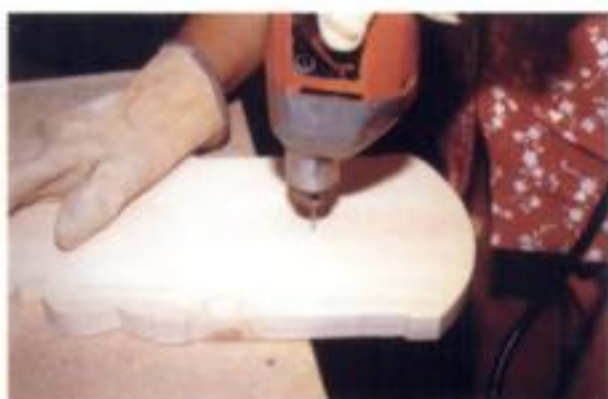
14. Drilling the pilot hole.
