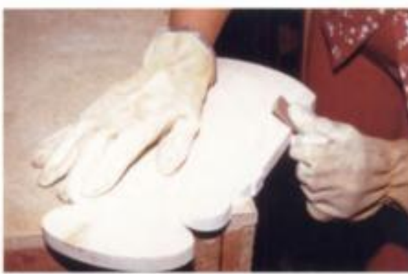
18. Taking the sharp edges off the top side of the wood piece.
