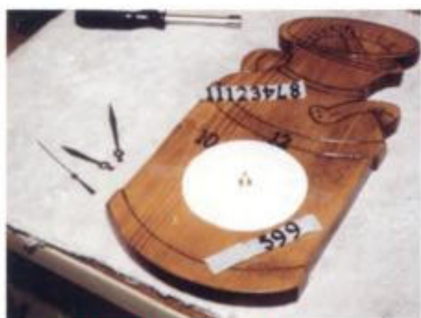
26. The template is used to position the numbers on the clock face.
