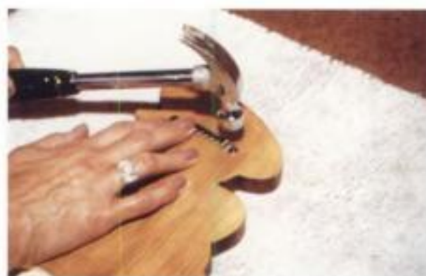
23. Nailing the sawtooth hanger on the center of balance.
