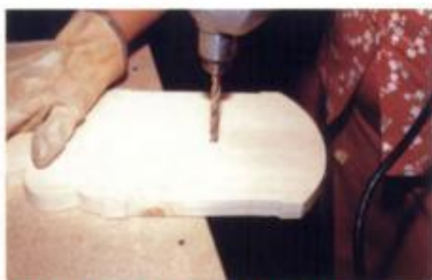
16. Drilling the \frac{5}{16} " hole for the clock shaft.
