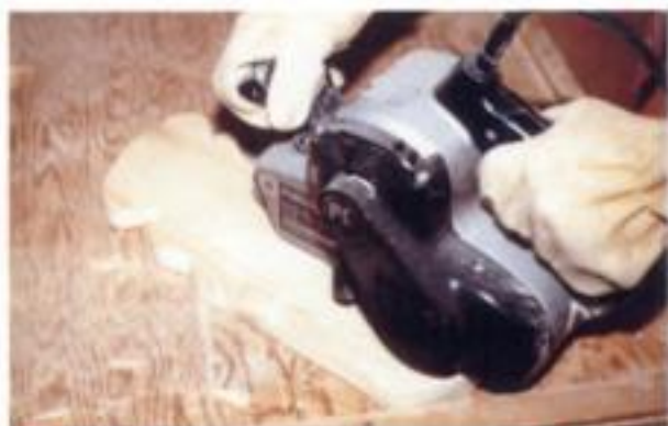
17. Sanding the wood piece with medium-grit (220-grit) sandpaper.
