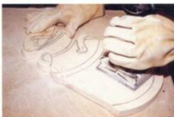
21. Sanding with 320-grit sandpaper after wood-burning.
