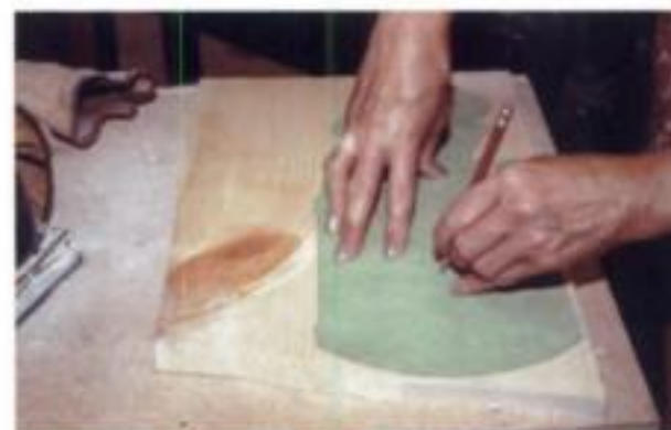
10. Tracing the outline and marking the hole for the clock shaft.
