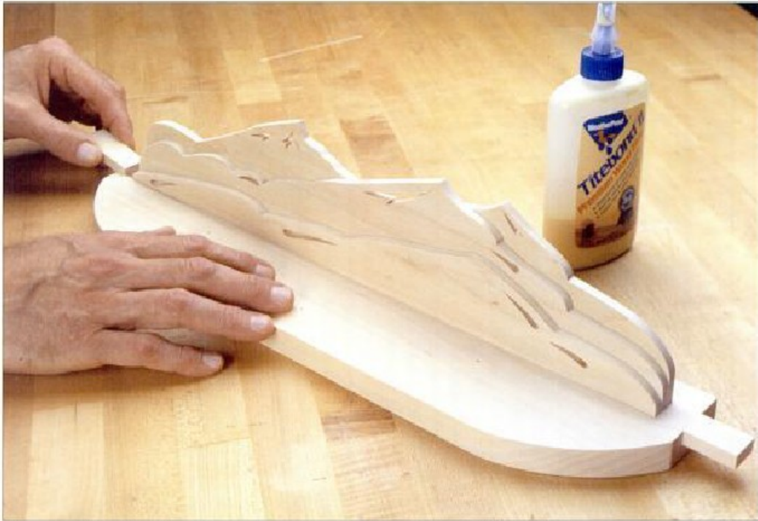
Glue the fillers in place, leaving \frac{1}{32} " gaps at each end between the mountain and fillers. Remove the mountains, and wipe off any glue that squeezed out from the groove.
