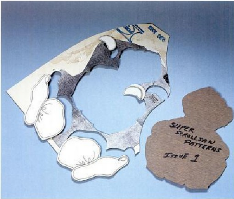
1–2. Make permanent templates for those patterns that will be frequently used. A variety of materials, including cardboard, \frac{1}{8} " hardboard, and even plastic, can be used for templates.
