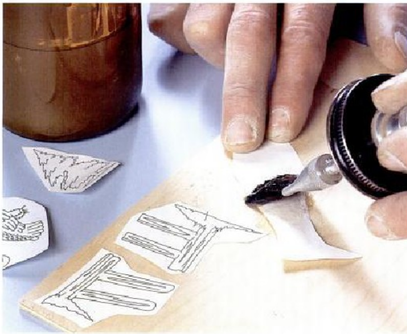
1-1. Many scrollsawyers use rubber cement for sticking on paper patterns because it's quick, holds the pattern firmly, and cleans up in a jiffy.
