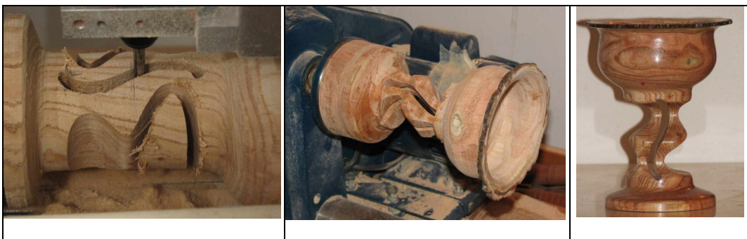
Figure 7. A vase with a neck that was CNC machined. On the left, the initial rotated stock is machined on the XYZ table. The middle figure shows the part after the CNC process was complete, back on the lathe. Finally the image on the right shows the final piece.
