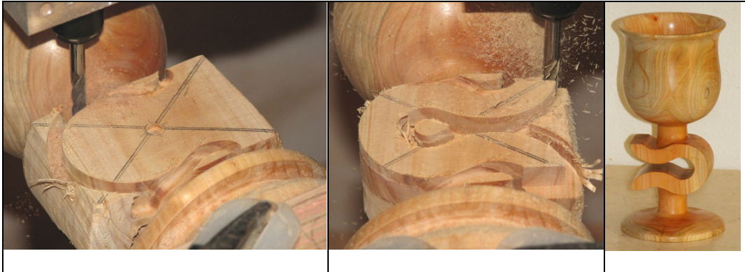
Figure 8. Another vase with a neck that was CNC machined. The left and middle images show the CNC steps on the XYZ table. Finally, the image on the right shows the final piece.
