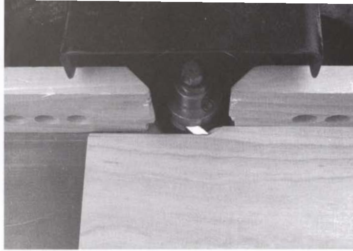
Shape a test piece until it reaches the outfeed fence. With the shaper off, move the outfeed fence forward until it just makes contact with the stock. Then lock it in place.
