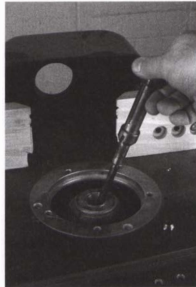
When changing spindles, align the keyway in the spindle with the pin in the arbor.
