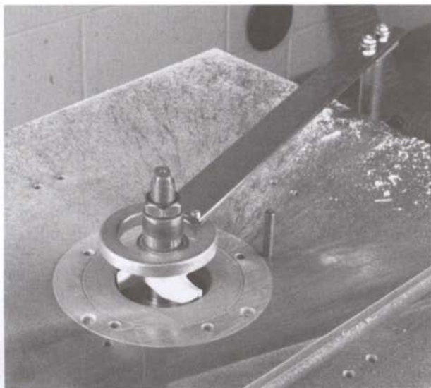
Guards are designed to protect your hands while shaping. The ring guard (left) is suspended over the cutterhead. The Safe Guard II (right) mounts on the spindle, above the cutterhead, and can be used with the shaper fence.
