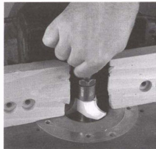
Rotate the cutterhead by hand to make sure it clears the table insert and the fence.
