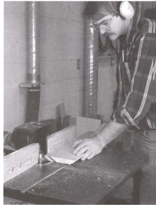
Always wear safety glasses and ear protection and try to keep your hands 6 in. from the cutterhead.
