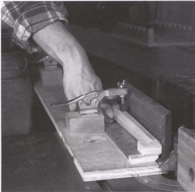
This tapering jig requires the use of a standard fence, which aligns the stock and jig to the cutterhead.
