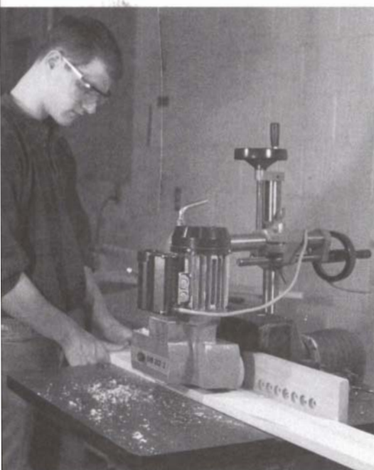
The power feeder holds stock firmly against the fence and table and propels it safely past the cutterhead.
