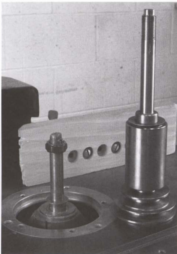
An optional extra-long spindle provides greater reach on wider, thick stock.
