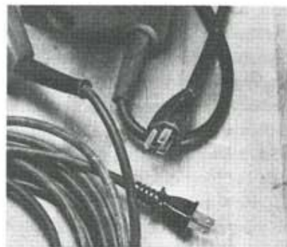
The cord can convey something about the router. On a quality tool, the cord is heavier and better insulated. There's a reinforcement, as on both of these machines, where the cord enters the motor housing, so the insulation won't crack and break at this heavy wear point. The cord on a Milwaukee router (top) is distinctive in its girth, while that on Makita's D-handled model is distinctive in its length—17 feet.
