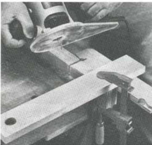
You can expedite the work if you stand all the pieces to be lapped on edge, gang them together, and clamp them with scraps on the outsides. Cut through the lot of them in one swipe. Here, a T-square guides the cut.
