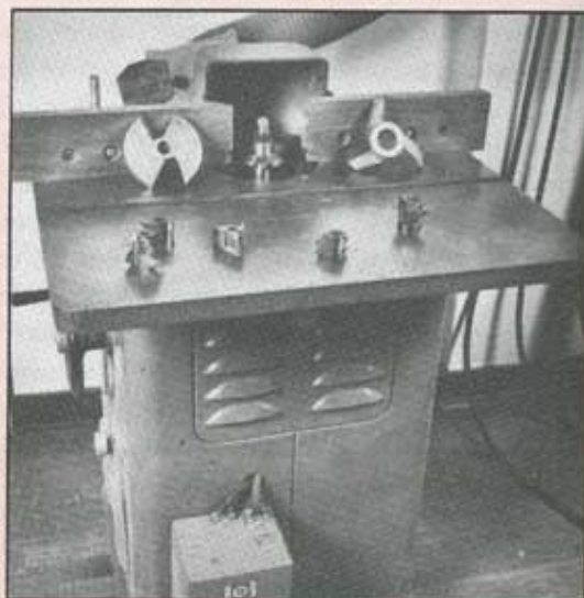
A true shaper is a cast-iron-and-steel shop behemoth, as you can see.
