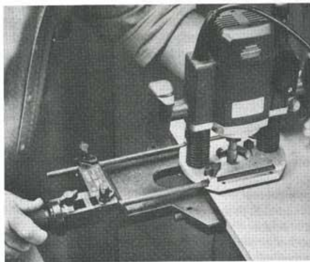
This edge guide, an accessory for Bosch's newest plunge routers, has all the features you should look for in a guide. The plastic wing nuts that seat against the mounting rods are easy on the hands and vibration-proof. Loosening the wing nuts on the guide allows you to dial in the exact setting you need with the fine-adjustment knob. It's easy to set precisely, and it won't work loose during use.
