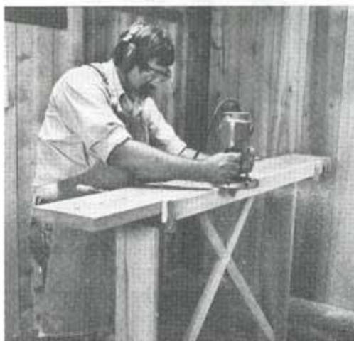
Perching a router on the edge of a workpiece is always precarious. But the narrow top of the router bench allows you to easily clamp such work to its edge. Then the router can bear on the bench top.
