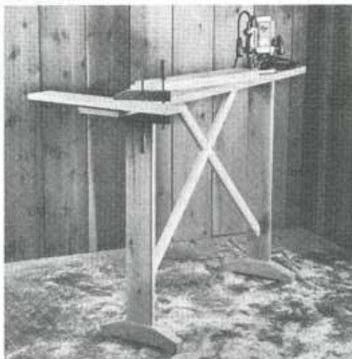
It's tall. It's skinny. But don't let its looks deceive you. This router bench is really handy for all sorts of hand-held router operations. And other woodworking tasks as well.
