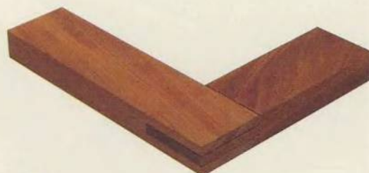
Open mortise-and-tenon joint
