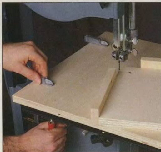
This quarter-circle-cutting jig is an ideal time-saver for rounding corners for tabletops. The jig pivots around a fixed point, taking the guesswork out of cutting perfect arcs.
