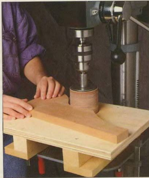
Although the drill press is used primarily to bore holes, it can also perform other woodworking tasks, such as sanding curved surfaces.
