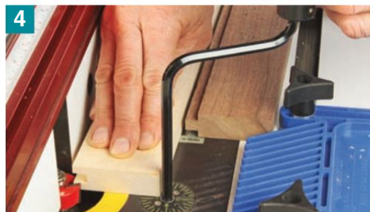
4 Use the grooved workpiece as a reference for raising the rabbeting bit carefully to its final height. The top of the cutters should be flush with the inside wall of the groove.
