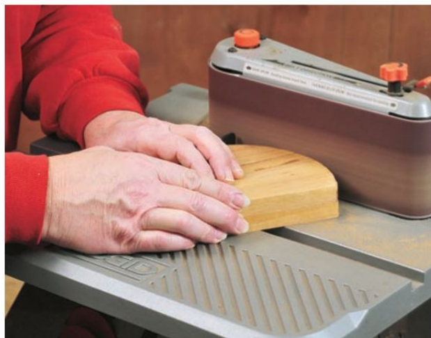
Figure 1: The author sands the two sides to their final shape. While they are being sanded, the sides are held together with double-sided tape. This technique virtually assures that the sides are identically shaped.
