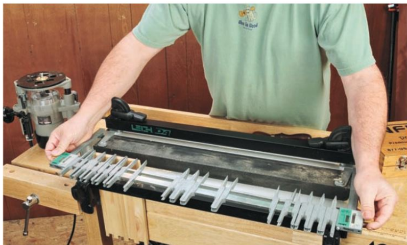
Photo 10: Some through-dovetail jigs, like the Leigh D4 Jig shown here, have adjustable fingers that enable you to vary the pattern and spacing to customize your joinery.
