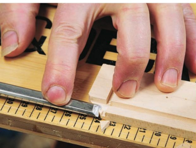
Figure 6: Once the small clearance miter has been cut onto the lower rear corners of the drawer sides, a small triangle of stock must be removed using a sharp chisel.
