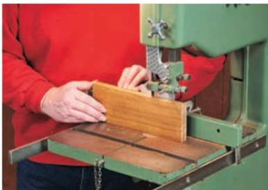
Figure 10: Resaw stock for the tambour slats.
