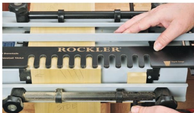
Photo 3: Install and clamp the mating board horizontally in the jig. Use spacer blocks to ensure even clamping pressure.
