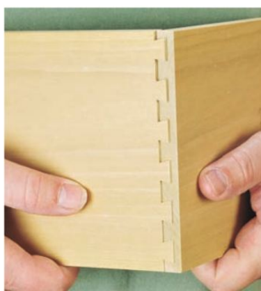
Photo 7: Assemble the test joint and evaluate the part fit. Likely, you'll need to make a few more adjustments to your setup.
