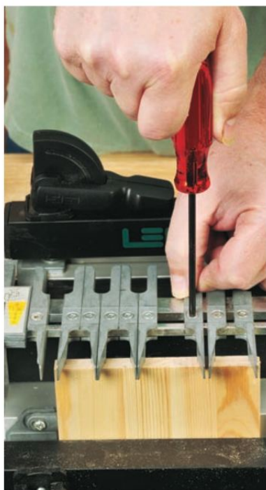
Photo 11: Clamp the pin board vertically in the jig, and adjust the guide fingers to create an attractive pattern of pins.
