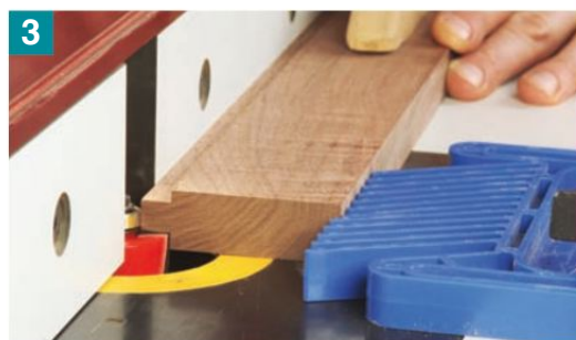
3 Rout away the bulk of the waste for the tongue in a series of shallow passes, flipping the workpiece from one face to the other after each pass. Continue to raise the bit about 1/8-in. for each pair of passes until the thickness of the tongue is close to fitting the groove.
