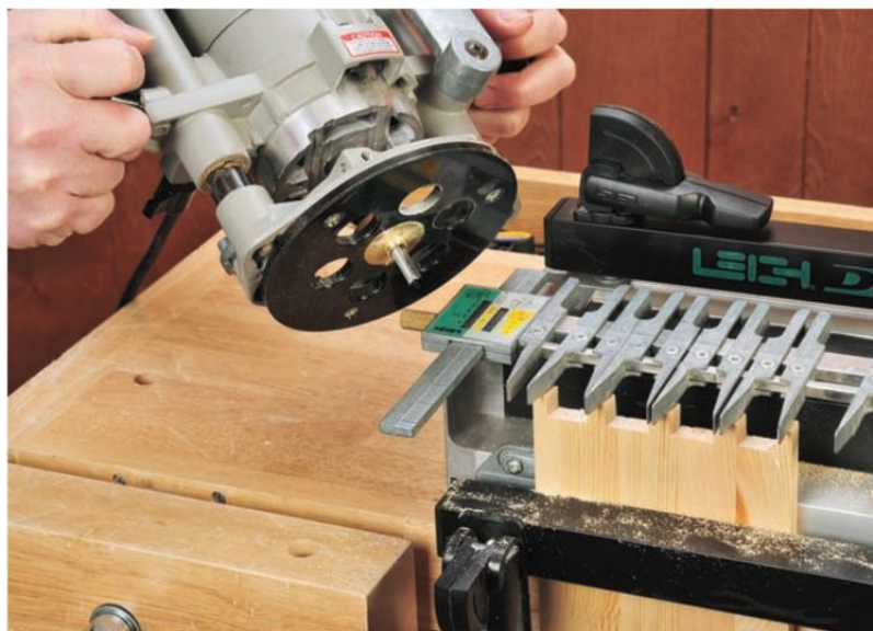
Photo 12: Cut the pins with a guide collar outfitted in your router base and a 5/16"-diameter straight bit. Feed the router from left to right to cut away the waste.
