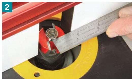
2 Adjust the faces of your router table's fence so they are flush with the bearing's rim on the rabbeting bit. Close up the fence facings, if possible, to reduce the gap around the bit.
