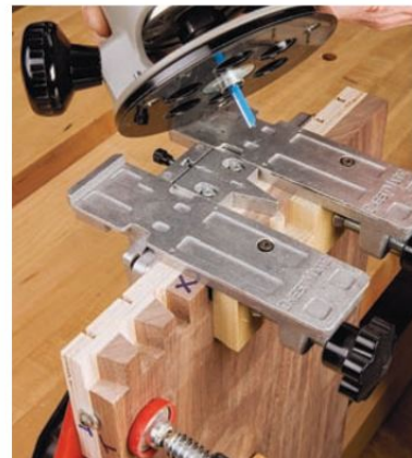
A tab under the pin and tail inserts locks positively into saw kerfs you cut in your custom template. They index the router cuts.
