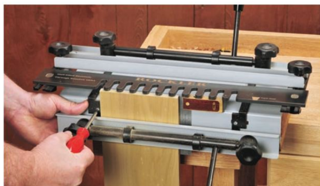
Photo 2: Square and clamp the vertical test board in the jig, and adjust the jig's stop flush against the edge of the workpiece. Make sure the board end is snug against the template bottom.
