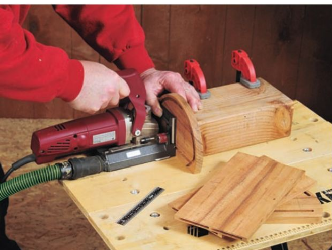
Figure 5: The author used biscuits to join the shelf and the bottom to the sides of the box. Note the stop block clamped to the work surface. It is cut square and holds the side 90° to the table and biscuit joiner.
