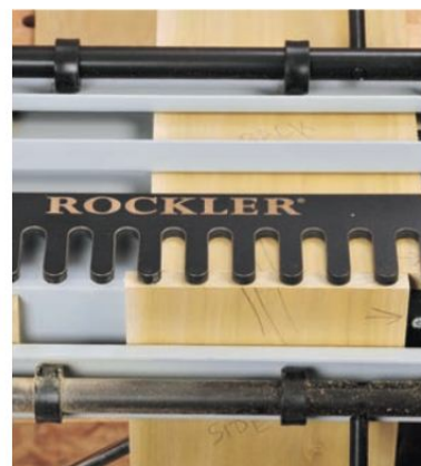
Photo 8: When routing half-blind dovetails, orient the matching pairs of workpieces with their inside faces pointing out.
