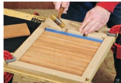
Figure 12: Wedge the slats into the jig.
