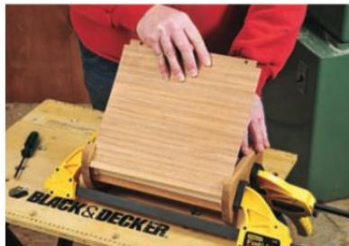
Figure 17: Test-fit the tambour sheet.
