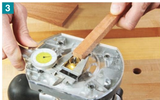
3 Rip a spacer from scrap that exactly matches the outside diameter of the template guide you'll use for this jig.
