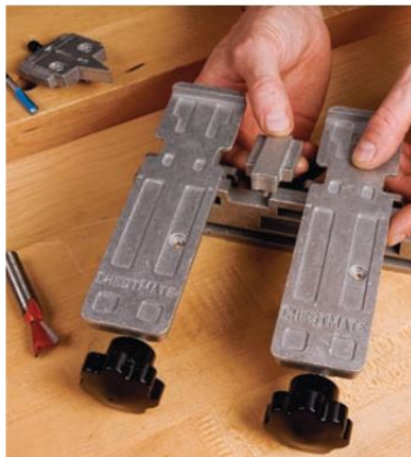
Changing over the Chestmate between pin and tail cuts is easy: loosen the jig wings and slip in the appropriate pin or tail insert.
