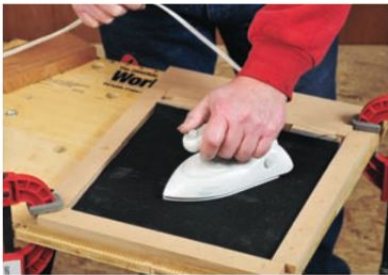
Figure 13: An iron sets the glue.
