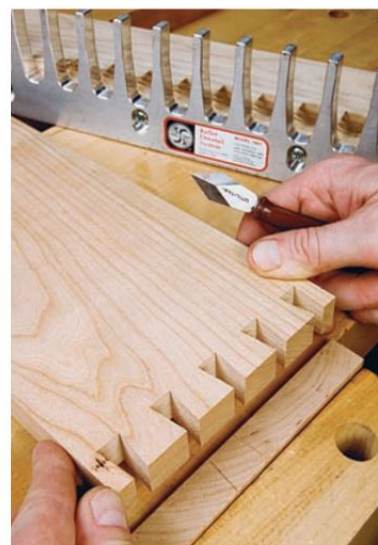
Registering the pin board for accurate joint alignment is as easy as holding the boards together and knifing a pair of tail lines onto it.
