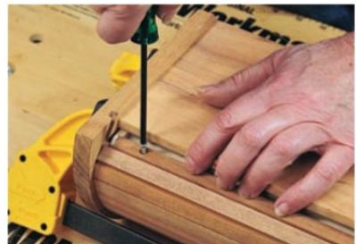
Figure 18: Attach the tambour to the drawer.
