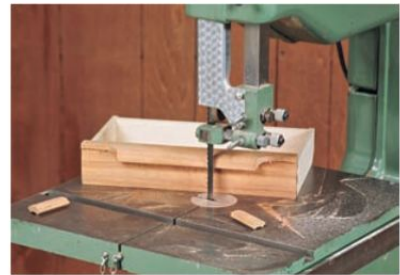
Figure 9: Shape the drawer pull.
