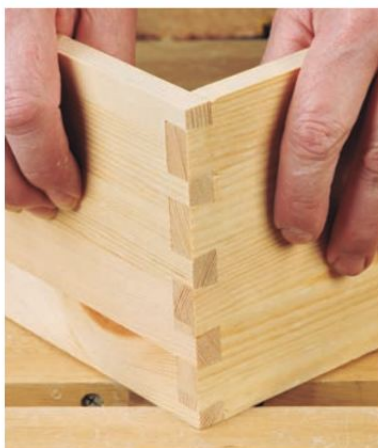
Photo 9: On through dovetails, the ends of both the pins and tails are visible in the finished joint, forming a pleasing pattern.
