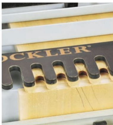
Photo 6: Before unclamping the boards from the jig, check to make sure you've routed away every bit of waste material in and around the template fingers.
