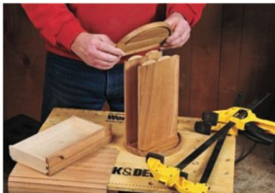
Figure 16: Dry-clamp the box together.
