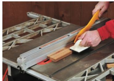
Figure 11: Gang cut the slats to width.
