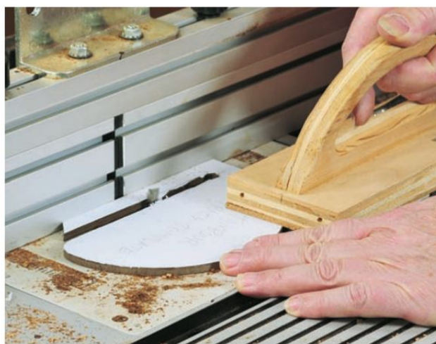
Figure 2: Making a template to guide the router while cutting the tambour track is an essential step. Once again, the template is used to provide dependable uniformity in the machining process.
