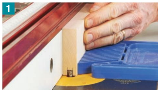
1 Make two passes with a straight or spiral bit, flipping the workpiece end-for-end between passes, to cut a centered groove.
