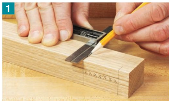
1 Lay out the mortise you want to make with this jig on your workpieces. Draw reference lines on both the faces and edges.
