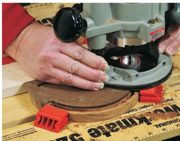
Figure 3: While routing the tambour track, keep constant pressure on the edge of the guide template. Loss of control during this operation will likely result in a ruined side piece. A plunge router works best here.
