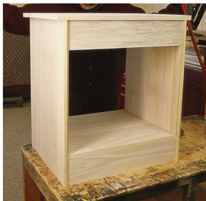
The carcass is essentially complete. All that's missing is the back, which I leave off until after I paint it and install the drawers.
