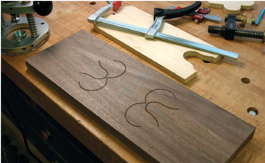
Step two. The completed tulip design faces away from the drawer center and is spaced just outside the bump design.
