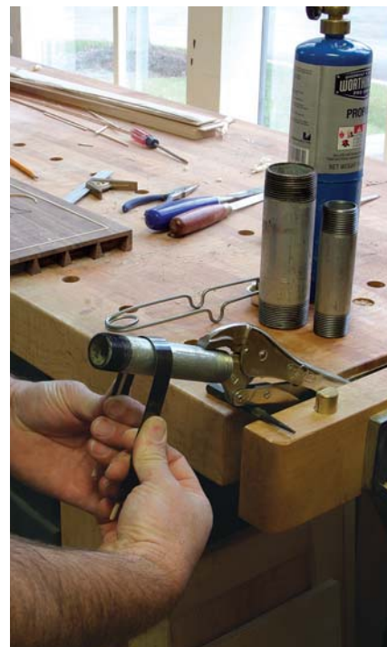
Hot pipes. The heat from the torched galvanized pipe steams the water and dries the string at the shape needed to fit into the grooves. It's always good to have pipes of various sizes on hand.
