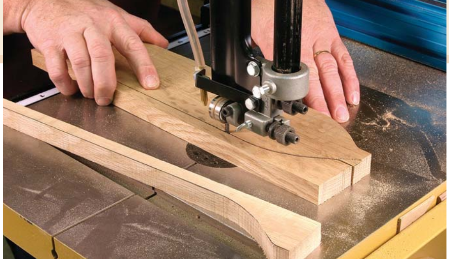
Cut the corbels from a larger piece of stock at the band saw. Cleaning the cut at a spindle sander makes short work of the task.
