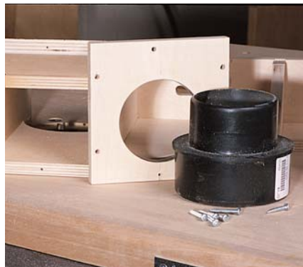
Inside view of the dust chute from the rear including the plastic 4" to 3" dust collection hose adapter. Rout the 3" hole for the adapter with the circle-cutting jig or use a "fly cutter" in your drill press.
