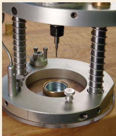
Stretching the point. Collet reducers, chucked into regular collets, can help to lengthen a router bit's reach.
