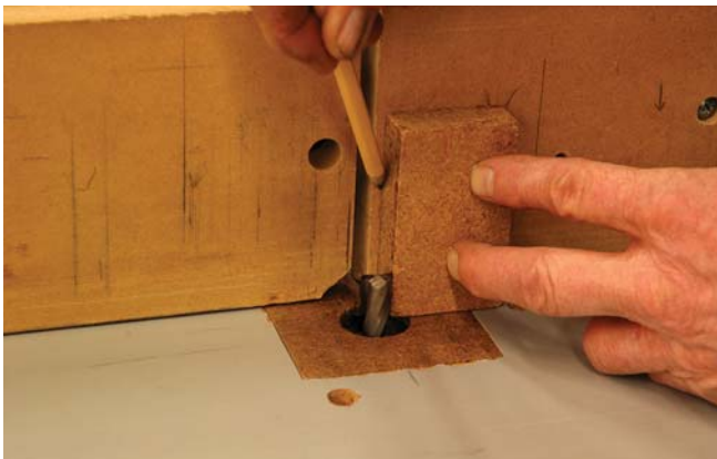
Bit of rotation. As you rotate the bit by hand, it pushes your scrap piece away. When the scrap stops, you've found the starting point of your cut. Align your mortise layout on these marks.
