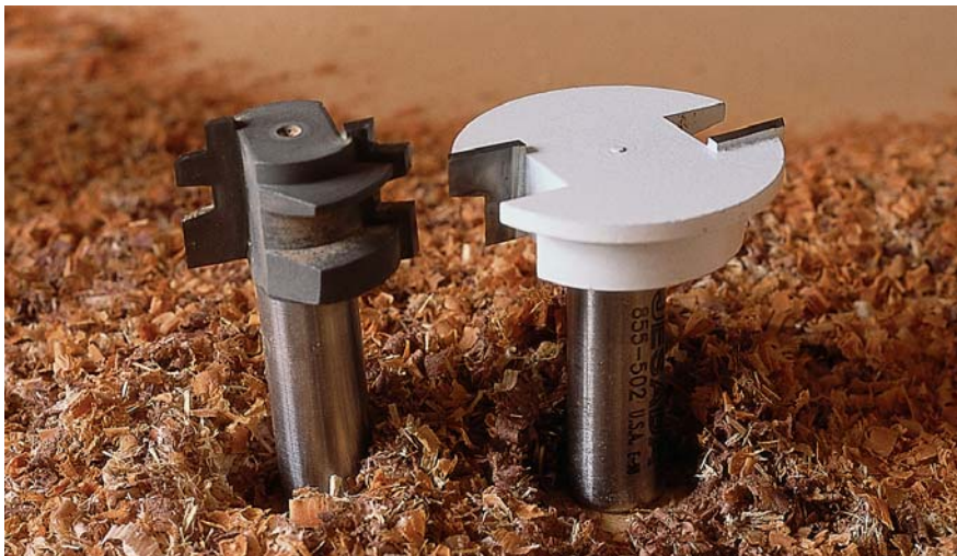
Two bits will cut a drawer-lock joint. The miniature glue-joint bit (left) is less flexible on stock thickness but produces a joint with more interlock. The drawer-lock bit (right) is more flexible in terms of the thickness of wood it works with. It cuts joints for both bottoms and corners.
