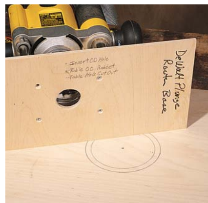
A larger base for the router was the ticket for bridging the open areas left by routing out the plywood for the router's base. It was later used as a small circle cutting jig for the tabletop and plastic inserts. Use the same cutter and it's easy to keep track of dimensions for cutting inside or outside circles.
