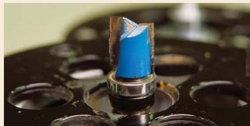
The first step involves plowing out a simple dado with a pattern-cutting bit, shown above.
