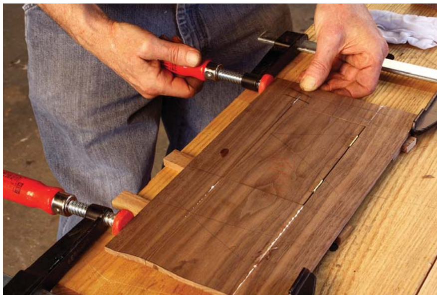
Perfect match. The back door is cut with four straight cuts from a single panel; the hinges are installed before reassembly.
