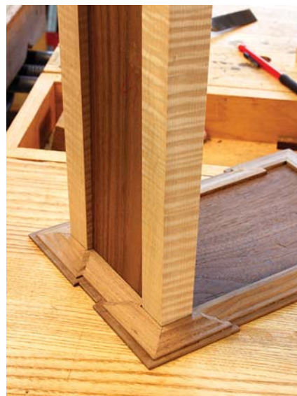
One at a time. Each panel is fit to the top before attempting to fit the entire carcass. That makes it easy to find the troublemakers.
