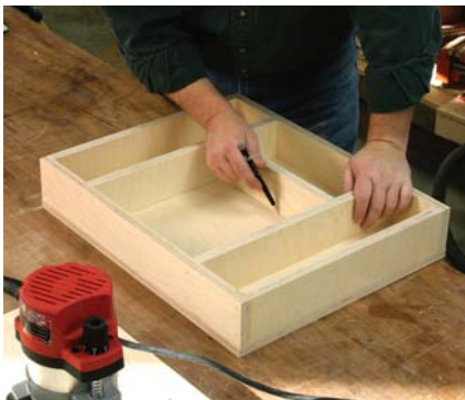
More marking: With the frame assembled and resting on the bottom piece, mark out the notch that will allow the router to extend through the top.
