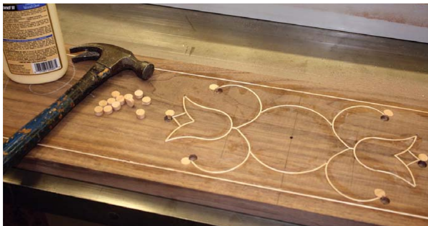
It's a perfect match. The face-grain plugs that become berries are fit into holes drilled with a ⅜" drill bit. Because of the flat-grain to flat-grain gluing surfaces, the berries will stay put.
