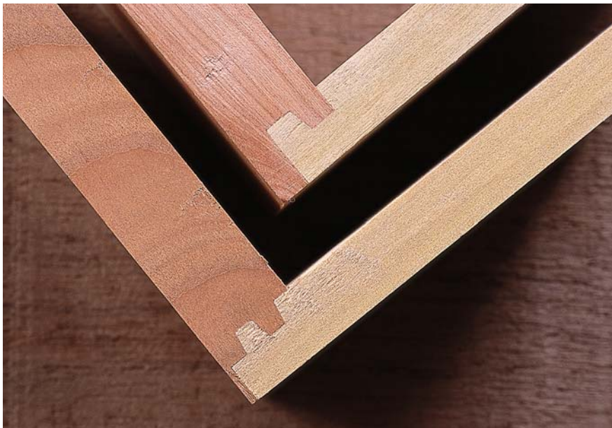
Two ways to cut a drawer-lock joint: The joint at top was made using a drawer-lock bit; the one at bottom was made using a miniature glue-joint bit. Both are strong and quick to make.
