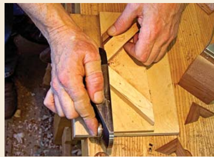
Shoot to fit. This fixture holds the workpiece at the correct angle and guides the block plane to perfect the ends of the mitered pieces.
