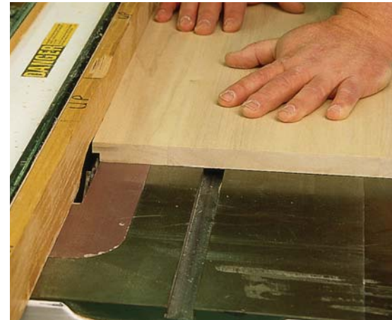
After resetting the dado height and adding a sacrificial fence to my rip fence, I was able to cut the rabbets for the back on each side.
