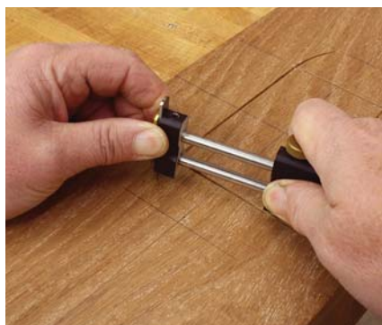
Begin radius work. Use a back-and-forth action as you scratch the pattern and be mindful to keep the pivot point planted.
