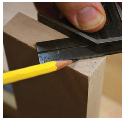
Lay out the column. On the end of the quarter-column stock, mark off a 45° angle to begin the layout process.
