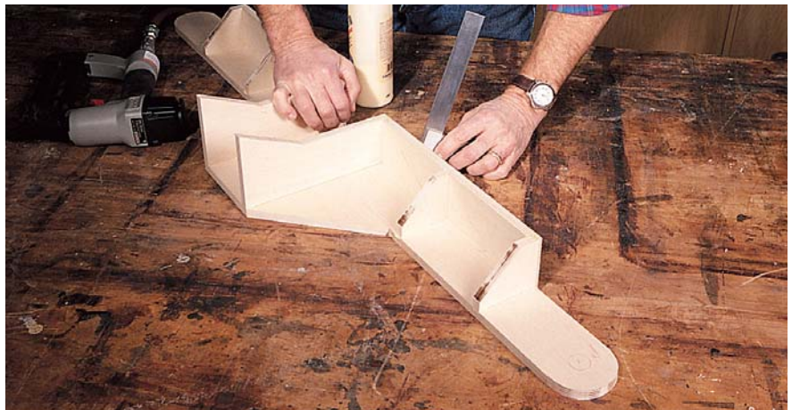
As you assemble the fence, make sure it is square along its length. Be sure and check it again after it is clamped up.
