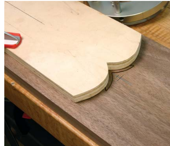
Plunge to begin. The tulip top string groove is the first of two grooves that require that you see the bit as you work – or develop a feel for when to stop at the line.
