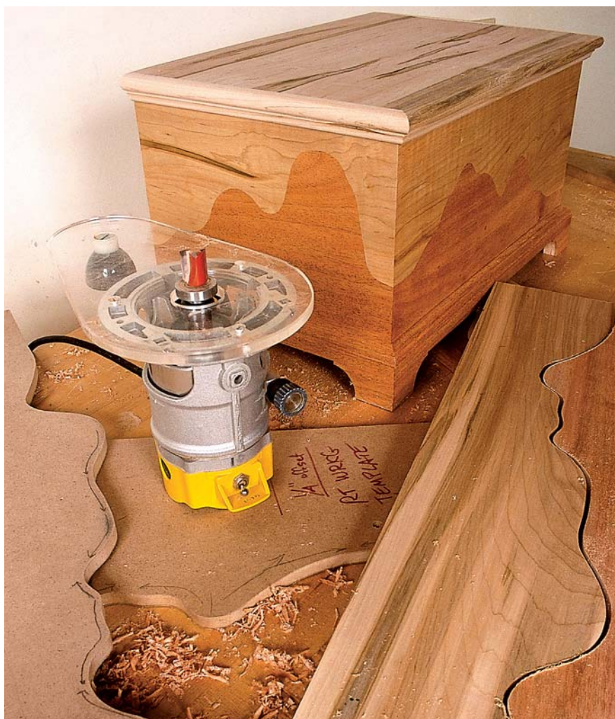
Joining stock edge-to-edge along a wiggling, squirming line may be purposeful, but mostly it's for fun. Templates and a shop-assembled offset pattern bit are the secret.
