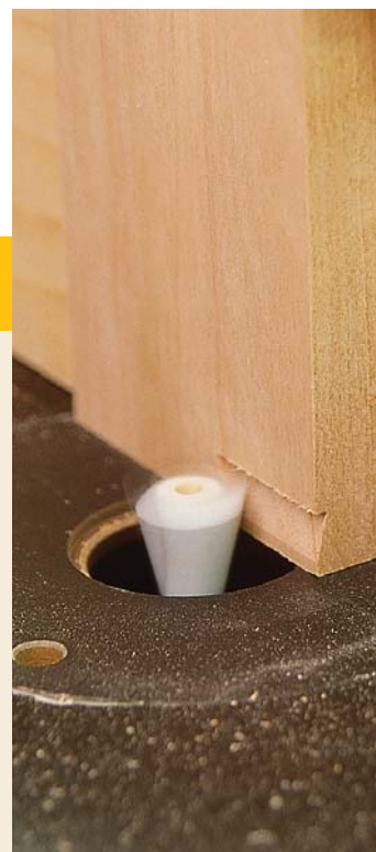
You can easily rout the tail of the joint on your router table with the matching dovetail bit.
