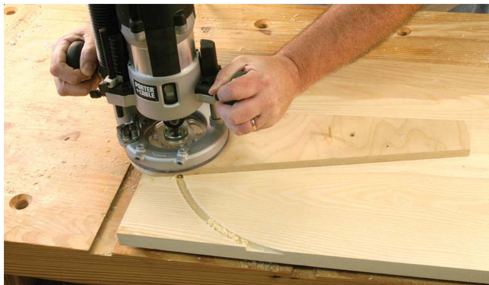
Safe and secure. The guide bushing turns in the hole as the circle is cut. At no time is it necessary to remove your hands from the router. Elevate the workpiece or the bench is will also get a groove.
