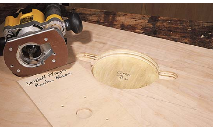
A larger base for the router was the ticket for bridging the open areas left by routing out the plywood for the router's base. It was later used as a small circle cutting jig for the tabletop and plastic inserts. Use the same cutter and it's easy to keep track of dimensions for cutting inside or outside circles.
