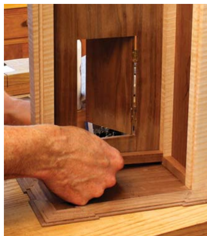
Hold on there. Square cleats glued to the bottom of the top capture the panels. Final assembly comes after the panels are ebonized and the columns are oiled.
