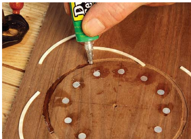
Drop in. The inlay materials were purchased as pre-cut parts from a luthier's supply store. These parts could also be fabricated from wood or other materials.
