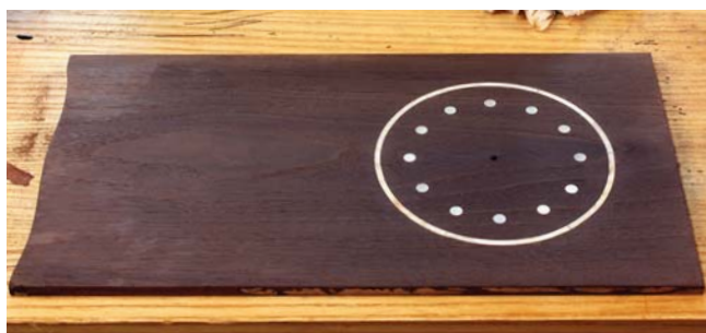
Inlay-safe. The solution has no effect on the mother-of-pearl inlay. Residue from coloring is removed with a non-woven abrasive pad, then the panel is ready for assembly.
