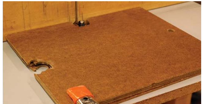
Shims step your cuts. Set your bit for its final depth of cut and use shims to surround it. Remove a shim after each cut to make the next cut deeper.
