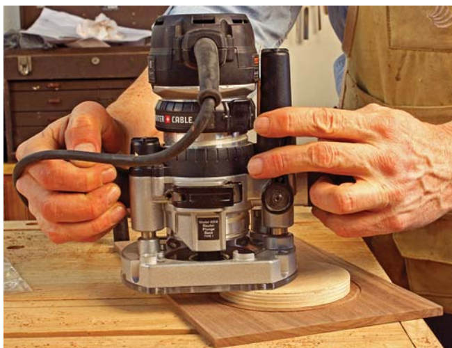
Take a turn. A plywood circle is used as a template for the router guide collar to follow when making the groove for the inlaid ring.
