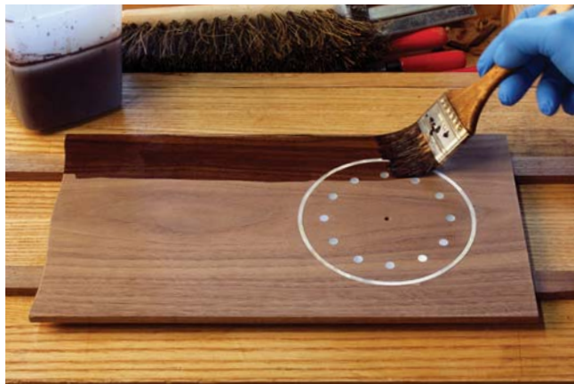
Nothing yet. The ebonizing solution won't change the color immediately. The chemical reaction between the rusty vinegar and the tannic acid in the wood takes a few minutes.
