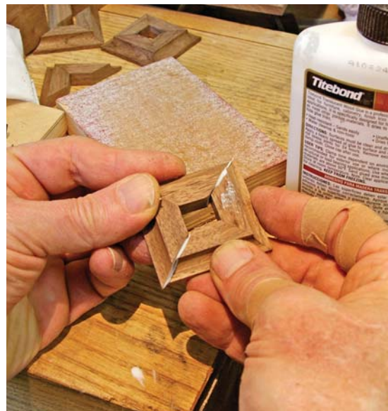
Two easier than four. Each half of a foot is put together, then two pairs are assembled to fit the tenons on the ends of the legs.
