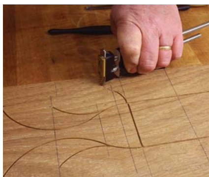
Two arcs, one radius. The short S-shaped line is a double arc made with the cutter set at a 1" radius.
