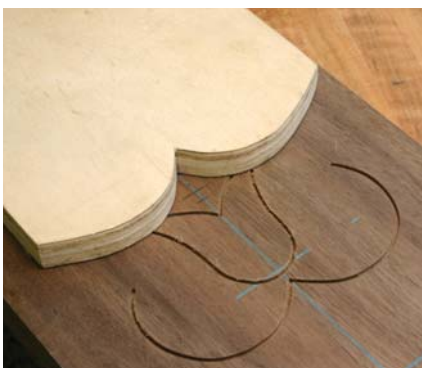
A simple reversal. Flip the wave pattern then set the distance between the pattern and the previous groove at 1" for the two top drawers and 1¼" for the lower drawers.
