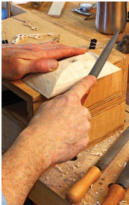
One, two, three. Rasps remove the band saw marks, refine the shape and smooth the surface of the dome.
