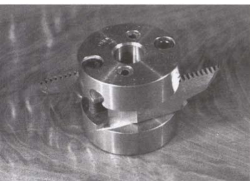
The knives for this locked edge cutterhead were custom-ground.
