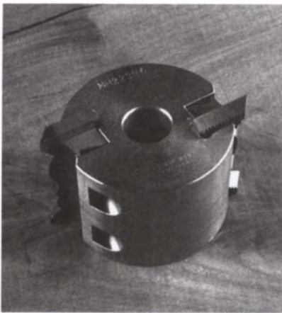
Insert cutterheads hold knives in the head by way of matching serrations in the knives and the head.
