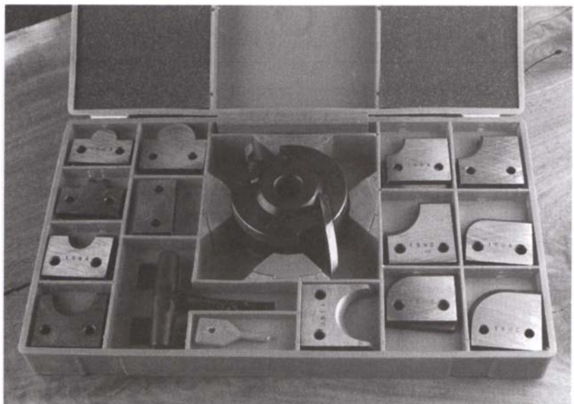
This insert cutterhead set utilizes pins that slip into holes in the knives to hold the knives in the head. Pressure from a gib maintains the interlock.
