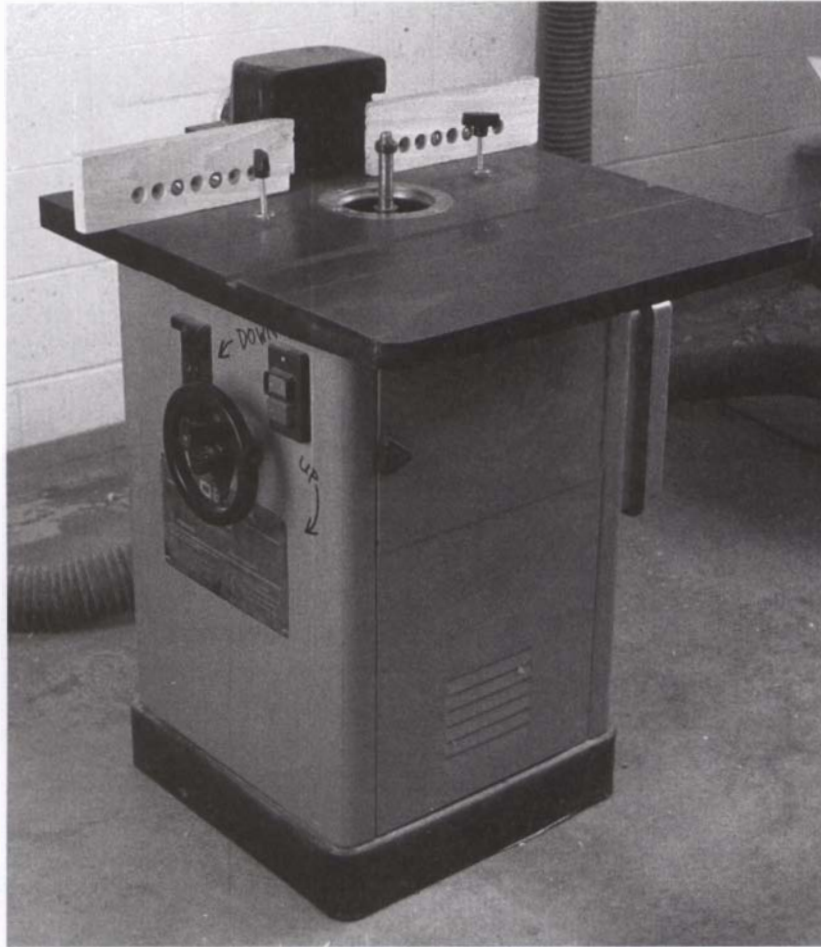
This 3-hp shaper with a \frac{3}{4} -in. spindle accepts a wide array of cutters, fences and jigs to handle many different applications—from small moldings to large panels for architectural doors.
