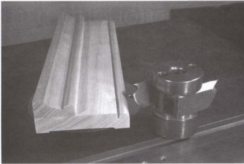
This window casing was milled with custom-ground knives. Grinding custom profiles enables you to shape unique or old casing profiles at a fraction of the cost of having the molding custom-milled.
