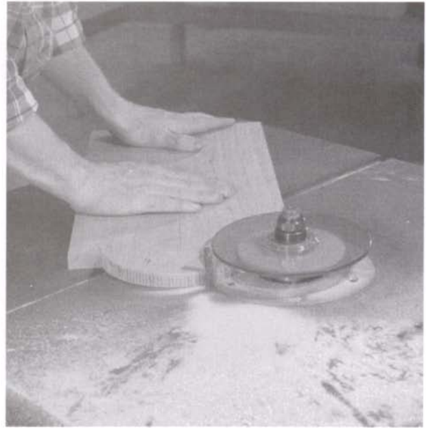
When shaping the top rail (left) and arched panel (right) freehand, use a rub collar and work from the starting pin. A ring guard should also be used.
