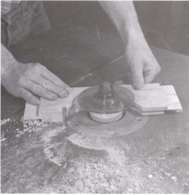
When shaping the top rail (left) and arched panel (right) freehand, use a rub collar and work from the starting pin. A ring guard should also be used.
