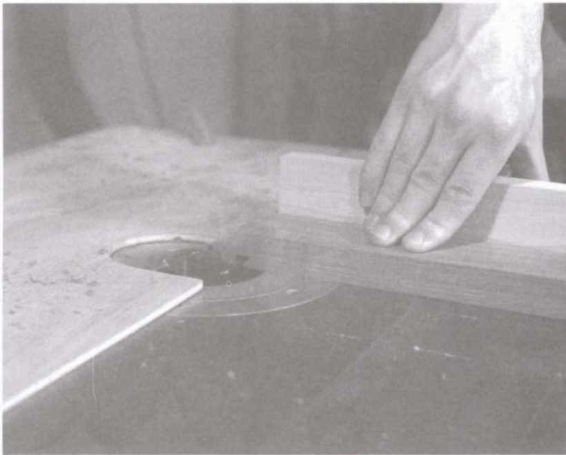
A piece of 1/4-in. plywood clamped to the table serve as the fence and depth stop. It also allows the long tenon to pass over the cutterhead.
