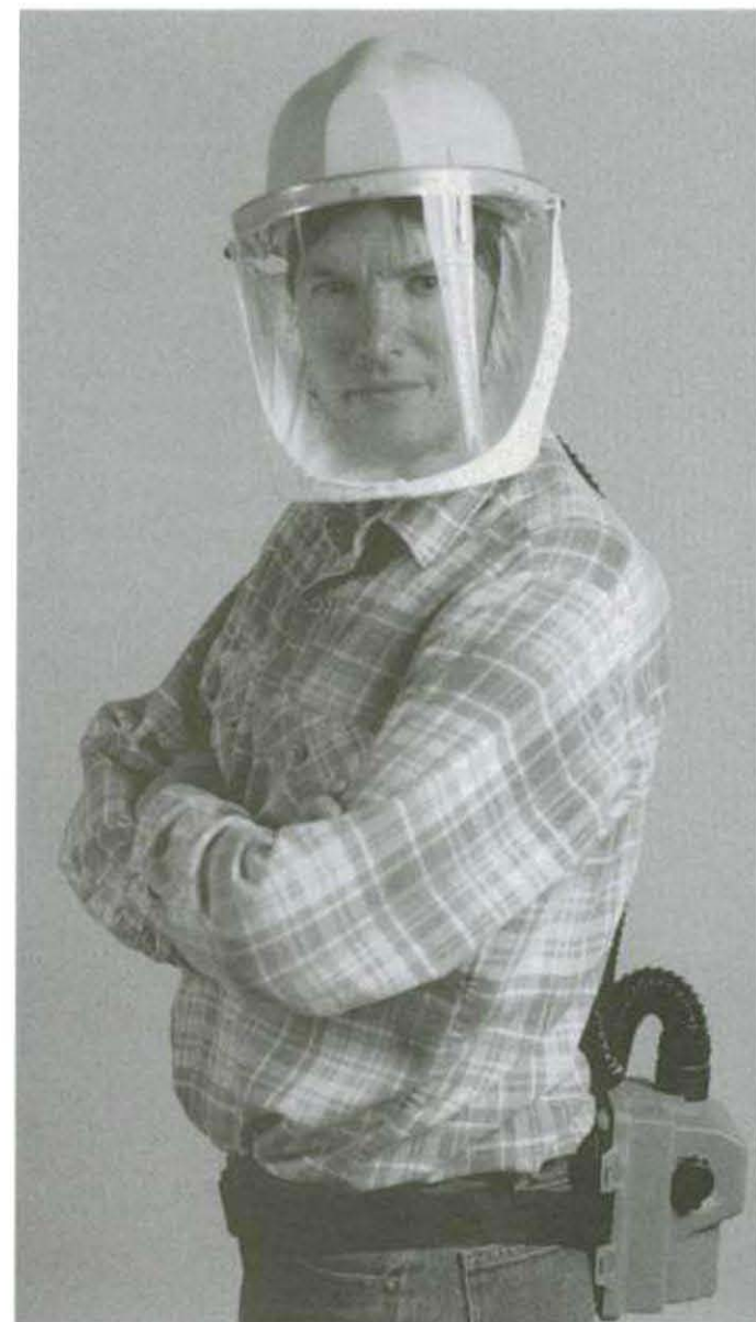
An air helmet will protect your eyes and lungs from chips and dust.
