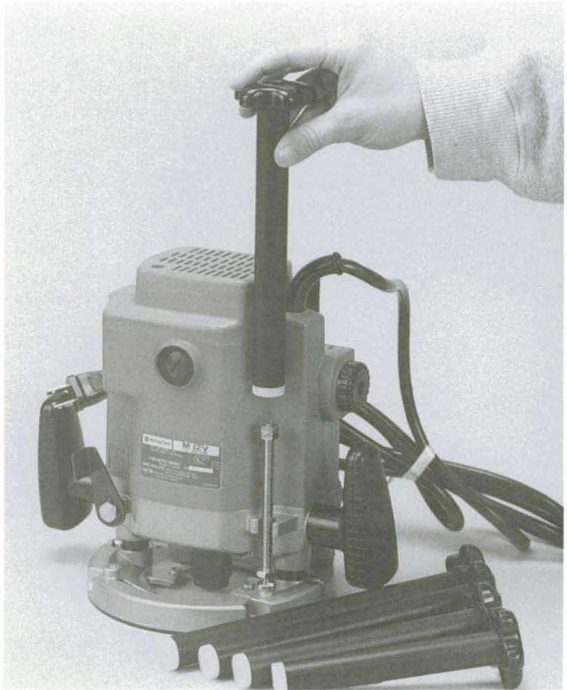
Depth-of-cut adjustment under the router table is more convenient if the nuts are replaced with an after-market router knob. On some routers, this knob is a standard item.
