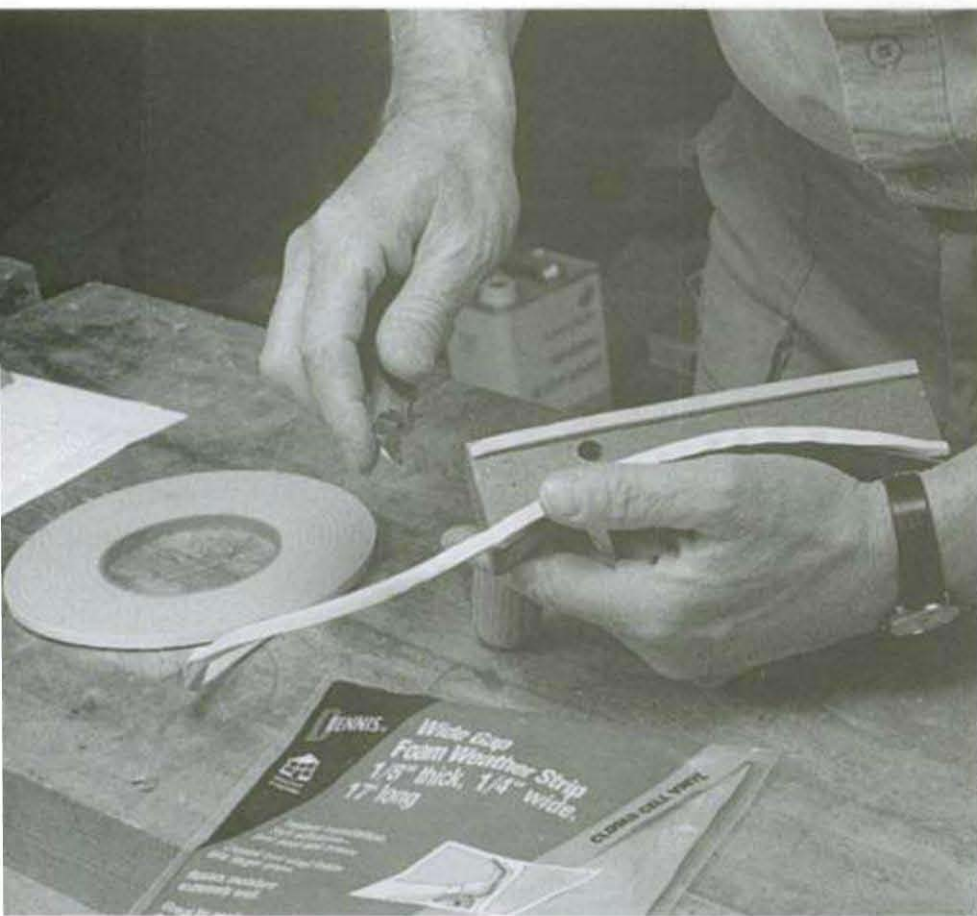
Gasket the perimeter of the fixture with pressure-sensitive weatherstripping. (The hole will receive the vacuum fitting.)
