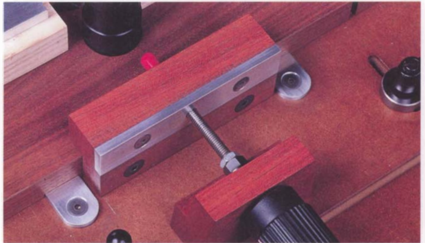
The author's router table fence is driven with a machine screw. The 1-in. aluminum bars fit into ways cut into the bottom of the fence so that it tracks straight and doesn't twist.
