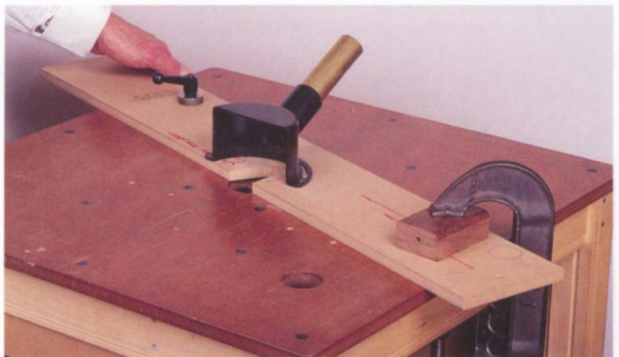
Big cutters require larger clearance holes than is necessary for most operations. A spare MDF fence can solve the problem.
