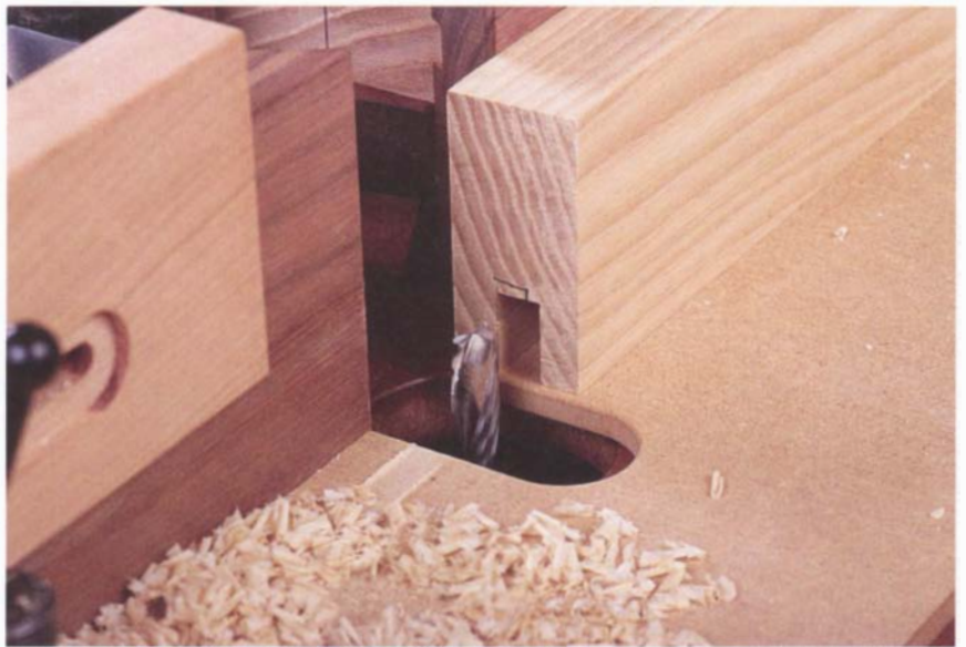
Stopped open mortises are safely done on the router table.
