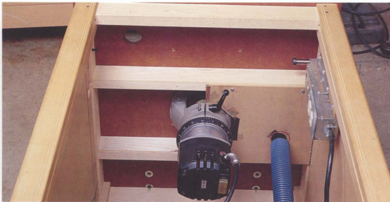
The hefty supports underneath the top ensure that the MDF panel stays flat—a key consideration for router table design.
