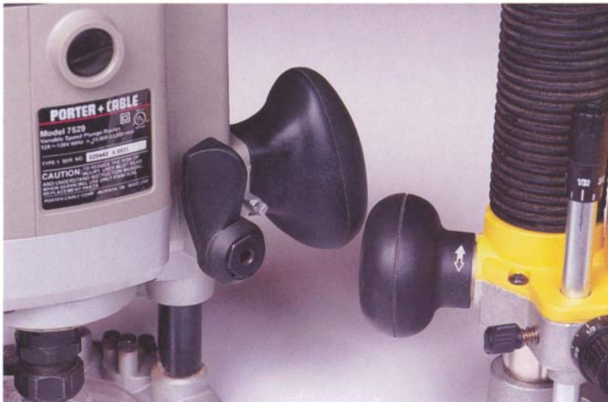
The DeWalt 621, right, has its motor lock in the left-hand knob. Spin it to lock or unlock. The Porter-Cable motor lock, left, is "on" in its default position. A twist of the lever unlocks it.
