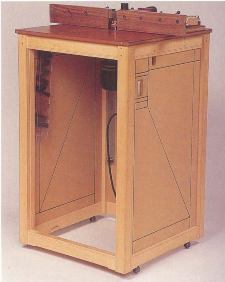
The author's router table has an MDF top that's supported by a series of ribs underneath. He uses a fixed-base router so he can permanently attach the casting and remove the router motor for bit changes.
