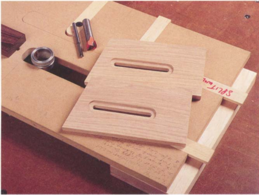
Slotted mortises require a jig. Here, the workpiece fits underneath, and the pattern bit runs in the slot.
