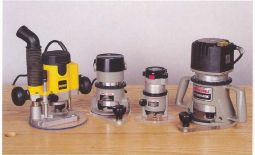
This ensemble is not cheap, by any stretch, but for a lifetime woodworker they will cover most routing challenges. From left: DeWalt 621 plunge router, PC-690 mid-range fixed base router, 310-PC trim router, PC-7518 fixed base router.
