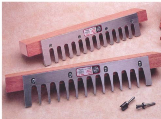
The Keller Dovetail System uses matched templates to cut precisely through dovetails on fixed centers. The idea is to do only through dovetails, but do them well and with a minimum of setup. (Photo courtesy Keller & Co.)
