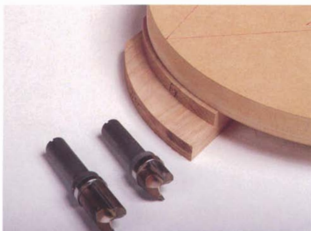
Shifting the template back routs a curved rabbet.
