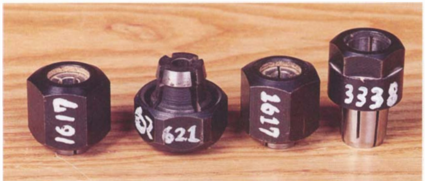
These collets are similar. Mark them so you won't accidentally put one in the wrong router. Since the collets are captured on their nut, they pull out of the armature and never stick in the router.
