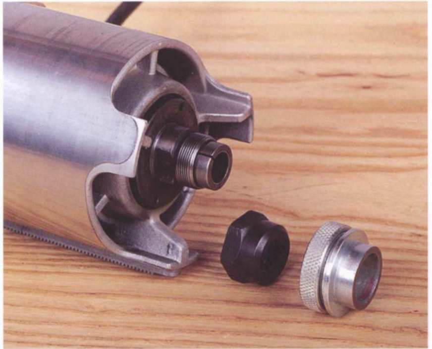
The three motor pack projections add another 1 in. of travel to this DeWalt 610, which is also shown with round collet nut and collar.
