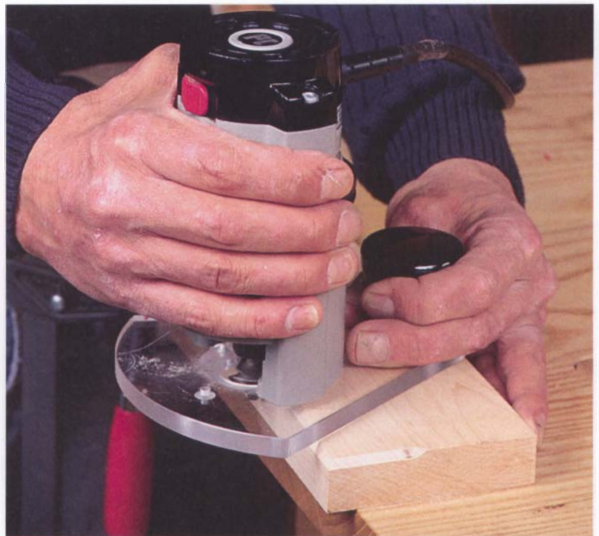
The PC-310 trimmer and offset subbase are a good match to trim (bevel) these edges. The work can be seen through the plastic base while the router is kept flat on the work.
