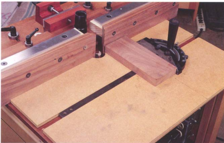
Two pieces of \frac{3}{8} -in. MDF clamped to the table provide a temporary pathway for the miter-gauge blade. This method doesn't compromise the router table by cutting into it for a groove.
