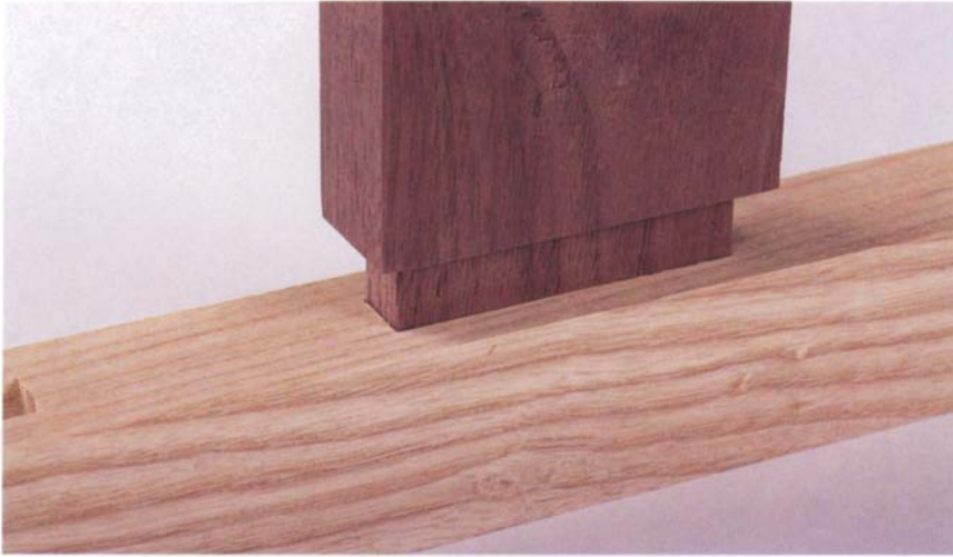
Mortises and tenons require fixtures for quality and repeatability. A good fit like this imposes a lot of demands on the jigs.
