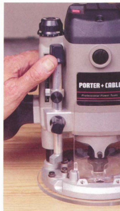
The depth stop on the Porter-Cable 7529 can be worked while your left hand is still on the grip, a smart safety move.
