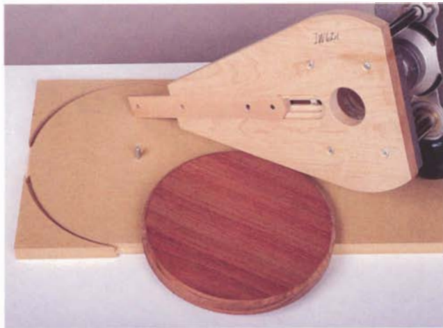
A homemade circle jig can be easily made up from hardwood scrap. An adjustable slide rides in a groove and pivots on a pin.
