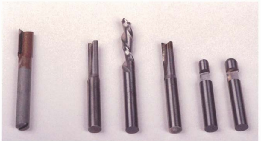
Solid carbide bits last longer than the same-sized bit with brazed-on carbide tips, left. Unfortunately, few cutters are solid carbide.
