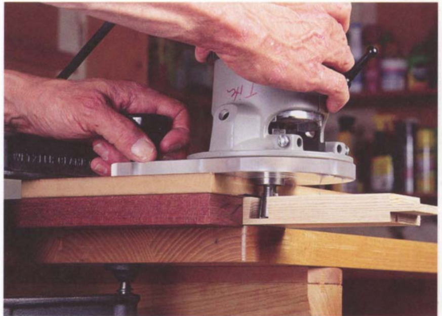
Cross grain dadoes and dovetails are easily cut with a fixed-base router and collar guide.
