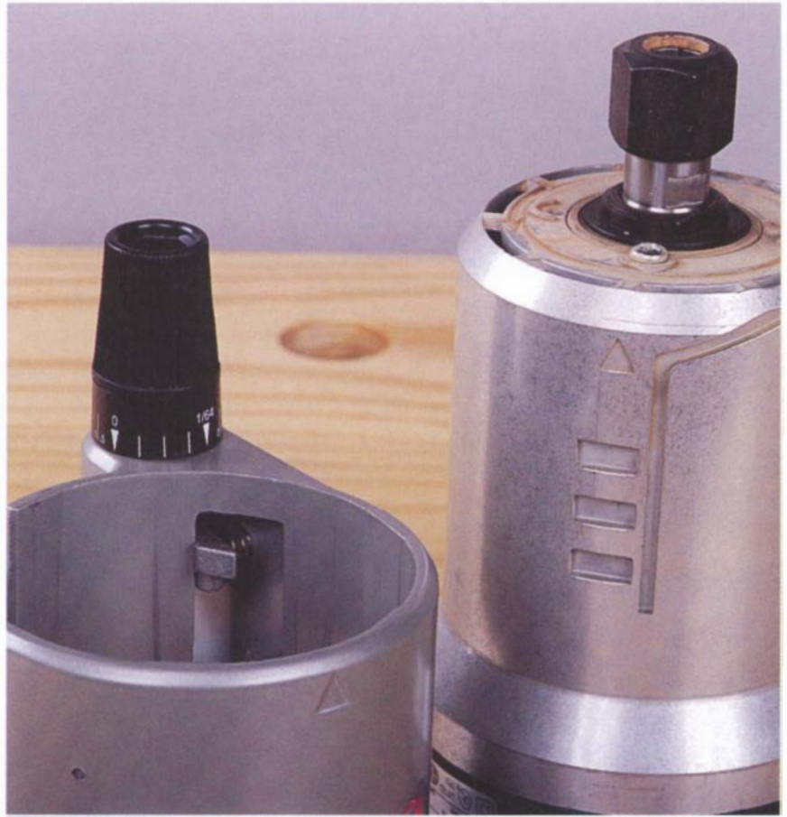
A spring lock engages a notch in the casting for the rough 1/2-in. changes on the Bosch 1617.
