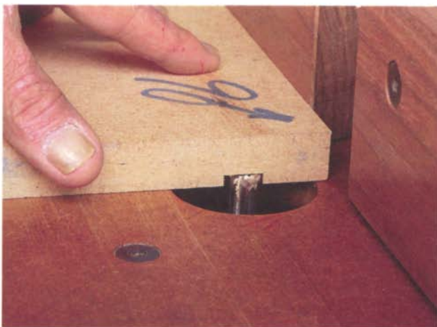
Making the groove is so effortless, one may forget there is a cutter soon to emerge as the work passes over it.
