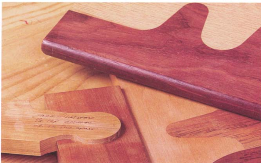
Complementary template joinery is about the only way to join wood along curvy lines. One sample is a lap, left, one is glue jointed, middle, and the other is tongue and groove, top.
