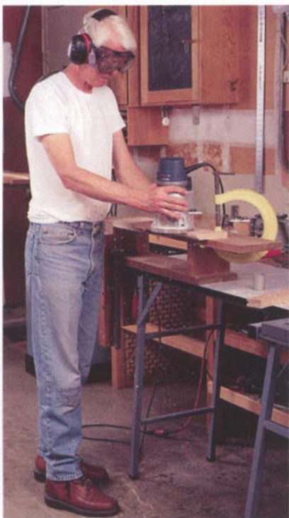
A router horse elevates the work and is more convenient than a router table for many operations.
