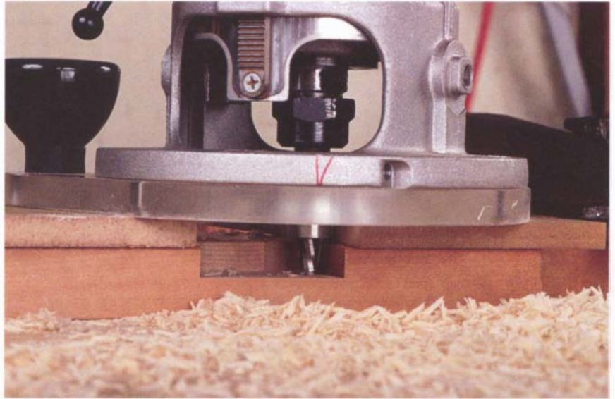
Collar guides are used with templates for joinery, like cutting this half lap.
