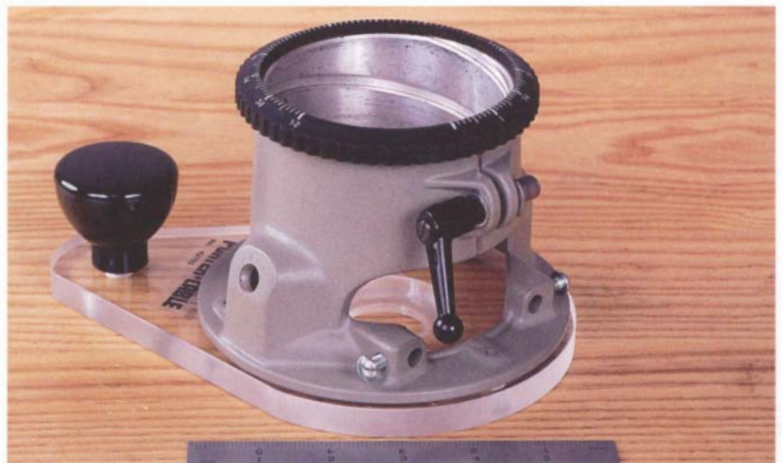
The locking lever of this Porter-Cable 690 router has been replaced with a longer version. The extra length provides more torque for easier locking.
