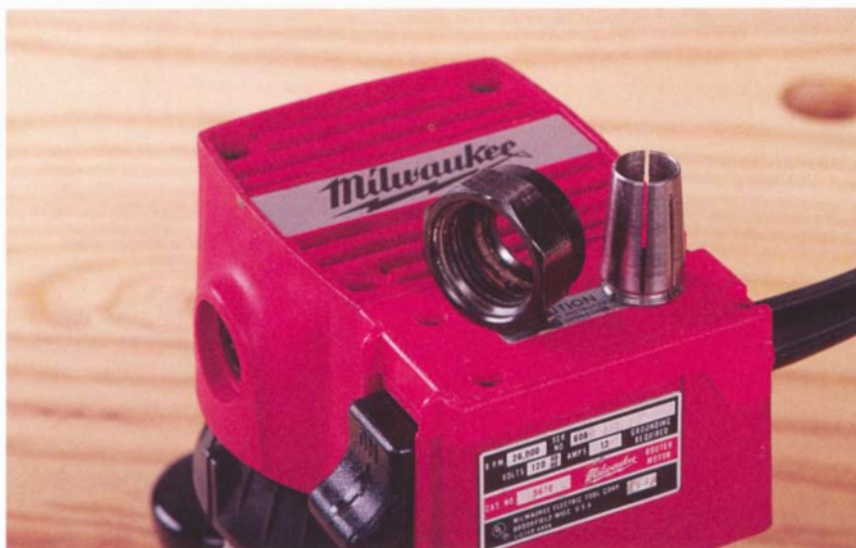
The Milwaukee 5680 has the only eight-sided collet nut and is one of the first with an eight-slotted self-releasing collet.
