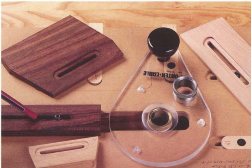
This slot-making jig limits the slot length with a stop. The slot width is one cutter diameter because the collar can't squiggle in its slot.
