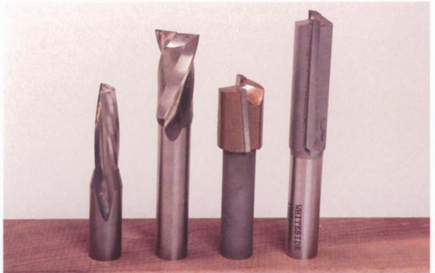
Straight cutters come in three primary styles: spiral bits, first and second from left; on shear; and standard straight cutter. The spiral and on-shear bits cut more cleanly than the straight bit.
