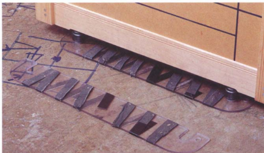
The router table box rests on four 1-in. ball casters that are screwed into threaded brass inserts. Two Lexan brakes keep the 80-lb. box from rolling away.
