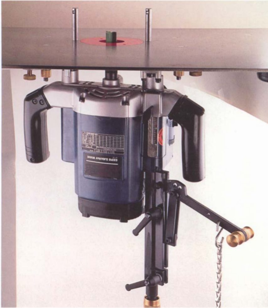
Lee Valley's Router Bit Jack is attached to the depth stop of a plunge router. The tool allows depth changes with a lever. (Photo courtesy Lee Valley.)
