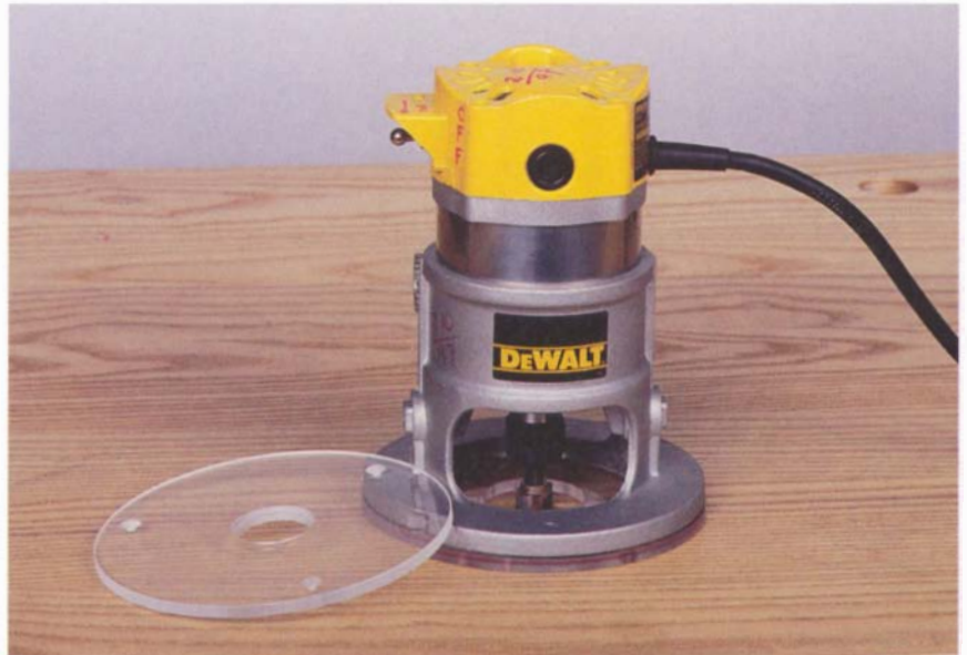
The DeWalt 610 shown here can be supplied with a clear plastic, round replacement subbase for collar guide use. The flat head provides a stable base for turning it upside down for bit changes.
