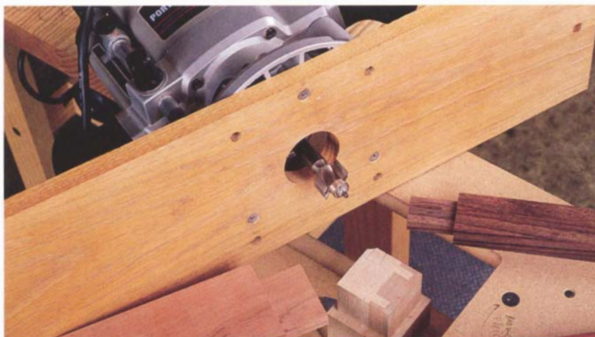
This platform jig uses an oversized base and a ball bearing rabbeting bit to form a square tenon on the end of a workpiece.
