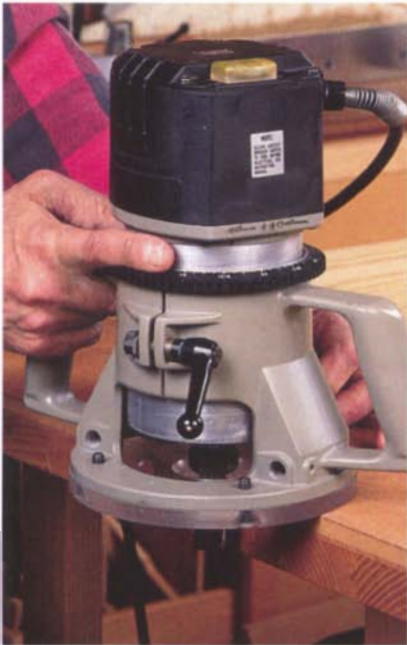
Wide glue-ups pose serious dimensioning problems. A jigsaw, router, and template can be used to square off the ends.
