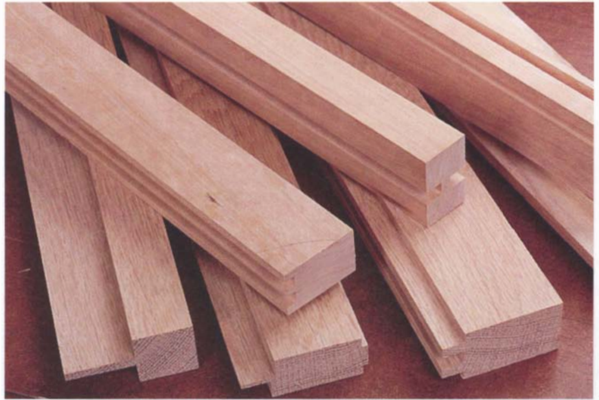
Tongues and grooves of all sorts can be made on the router table with straight bits.
