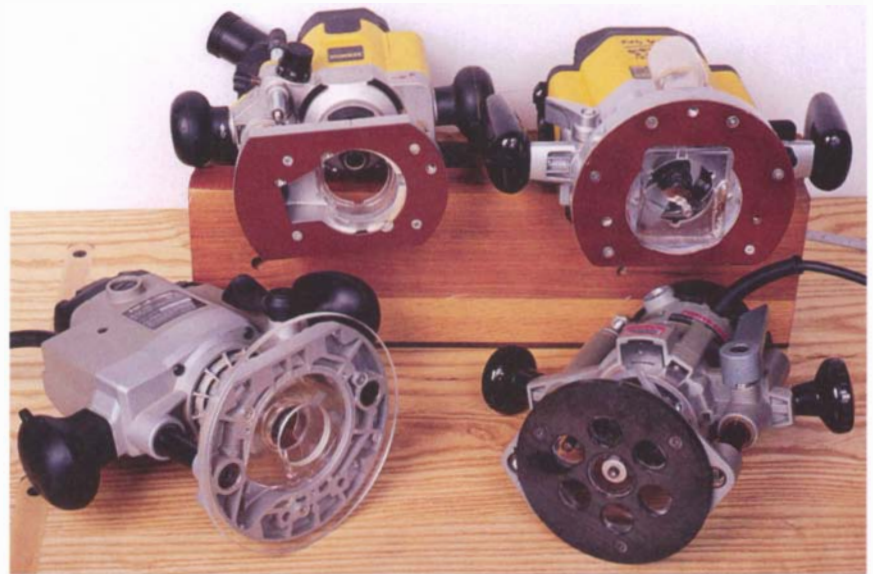
Plunge-base castings are all different, but they share some instability when routing along the edges of the work. The plunge router, at lower left, has been fitted with an aftermarket round subbase for greater stability.
