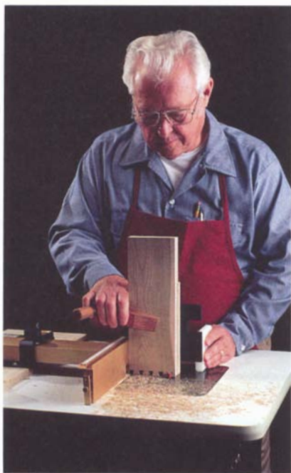
The JoinTech fence adjusts continuously and can be used on other stationary tools. (Photo courtesy JoinTech.)
