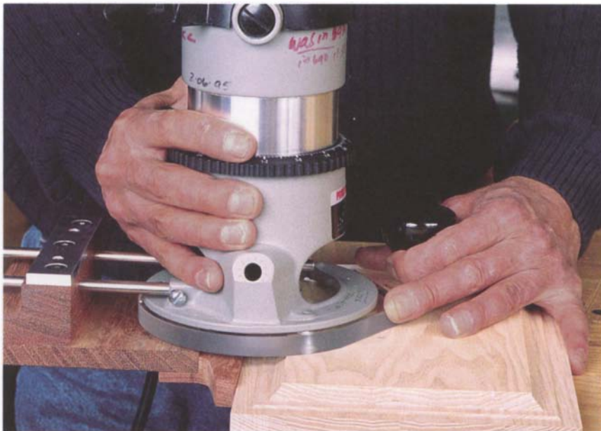
Keeping the whole setup flat is important when making a raised panel.
