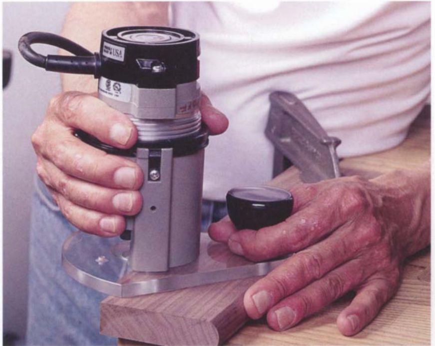
The author's offset subbase provides increased control for edge work, especially around turns and on ends.
