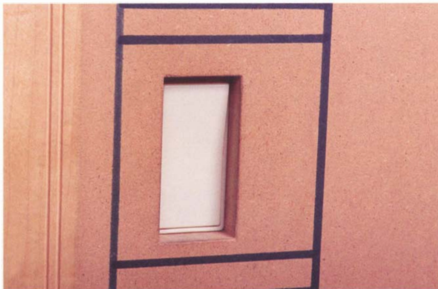
A 15-amp rocker switch buried in a mortise prevents accidental startups, but is easy to shut off.
