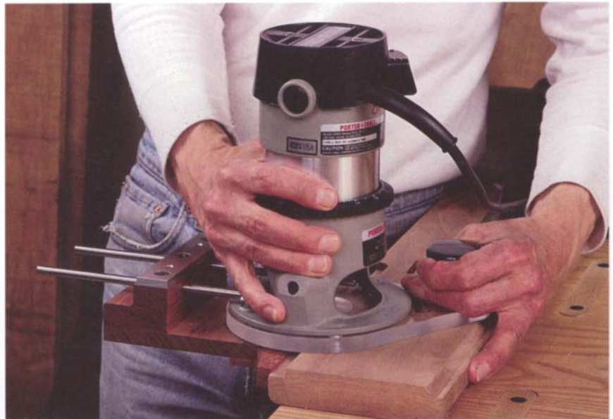
Edge guides can be easily adjusted to vary the width of a cut. A 1/2-in. bit, for example, can make a 5/8-in.-wide rabbet.
