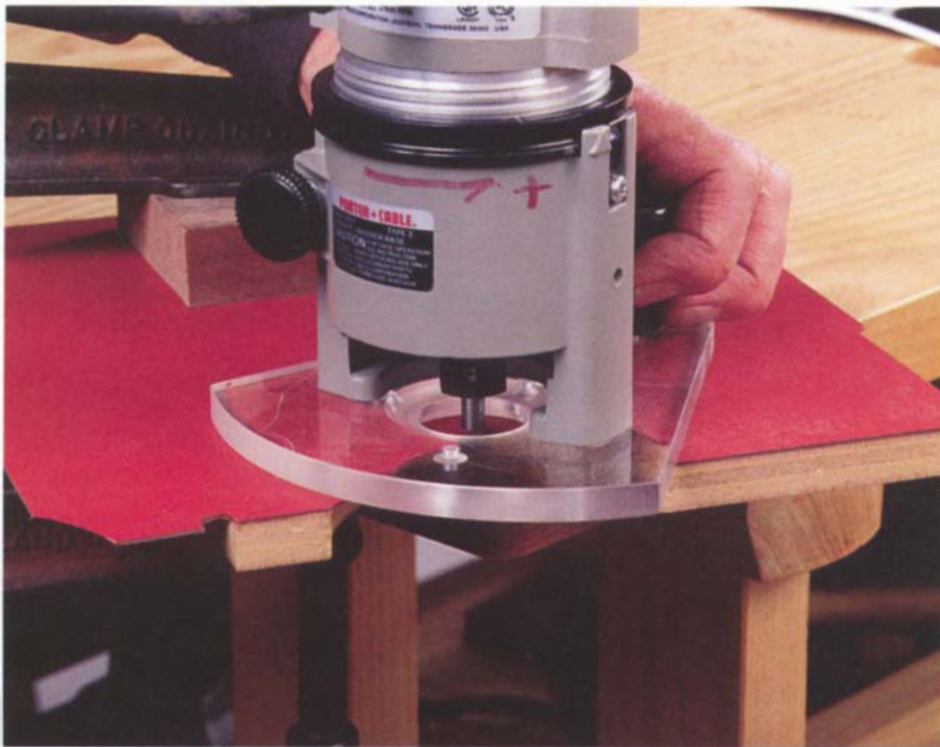
Trim routers may get their heaviest use in countertop fabrication. Here, plastic laminate is being flush-trimmed after being glued down on the particleboard substrate.
