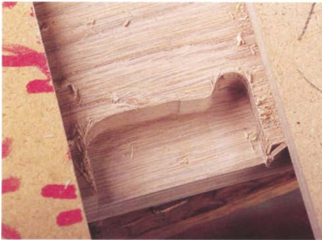
Only the right corner will tear on this crosscut, so a spoil board clamped on the edge will prevent tearout. The cutter spins in to the work edge on the left and can't tear.
