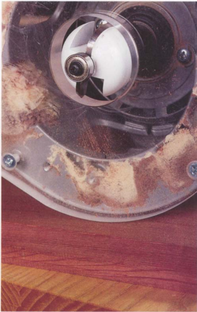
The side pressure from a bearing can be so high that it mars the work. If this is a problem, sometimes two bearings can be used.
