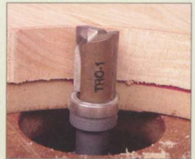
A cutter with a bearing bigger than the cutter diameter will lighten the cutter load for the first pass. A second pass with a pattern bit flush with the cutter will leave a smooth surface.
