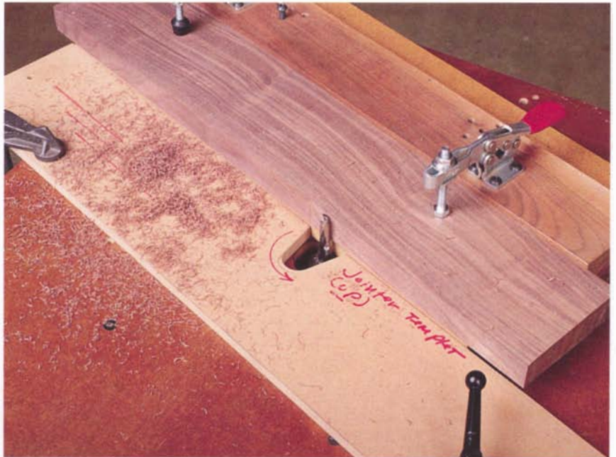
The fence on the work holder can be adjusted parallel to its work edge. With the cutter surrounded by an MDF straight fence, you can joint and machine to width in one operation.
