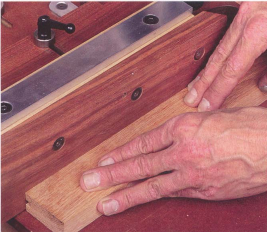
Always push down and against the fence beyond the cutter when operating a router table.
