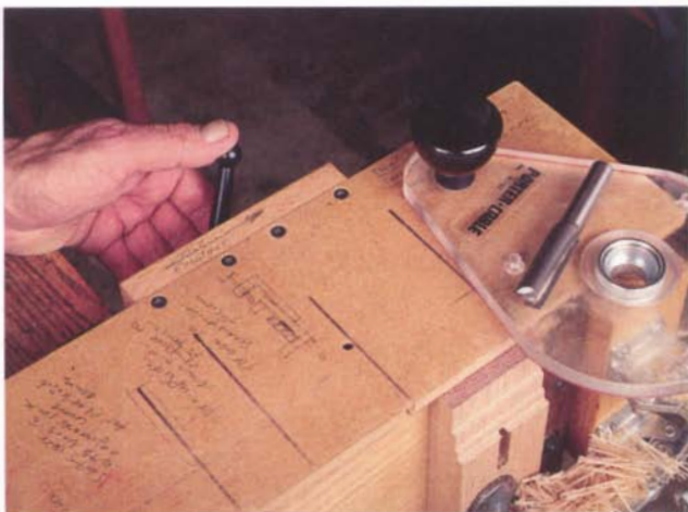
This adjustable tenon jig is used with collar guides to cut precise tenons. One turn of the lever is 0.055 in. of template travel.
