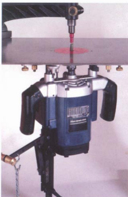
This over-arm pin router assembly is used with a template attached to the top of the workpiece. It's very efficient for making multiples of pieces with a complex shape. It's also capable of inside template routing. (Photo courtesy Lee Valley.)
