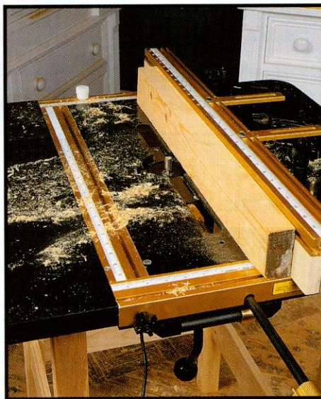
▲ The fence can be turned around so that the router runs lengthways, making it ideal for mortice and tenons
