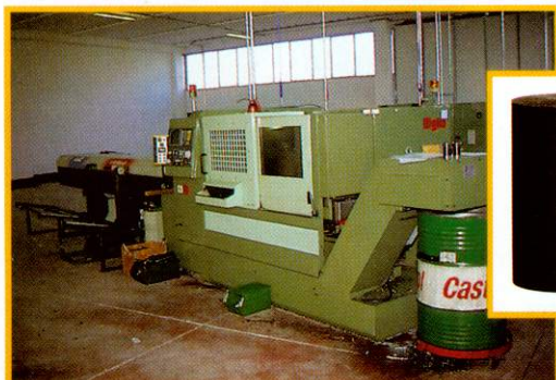
Fatigue proof steel-bar is fed into CNC lathes
