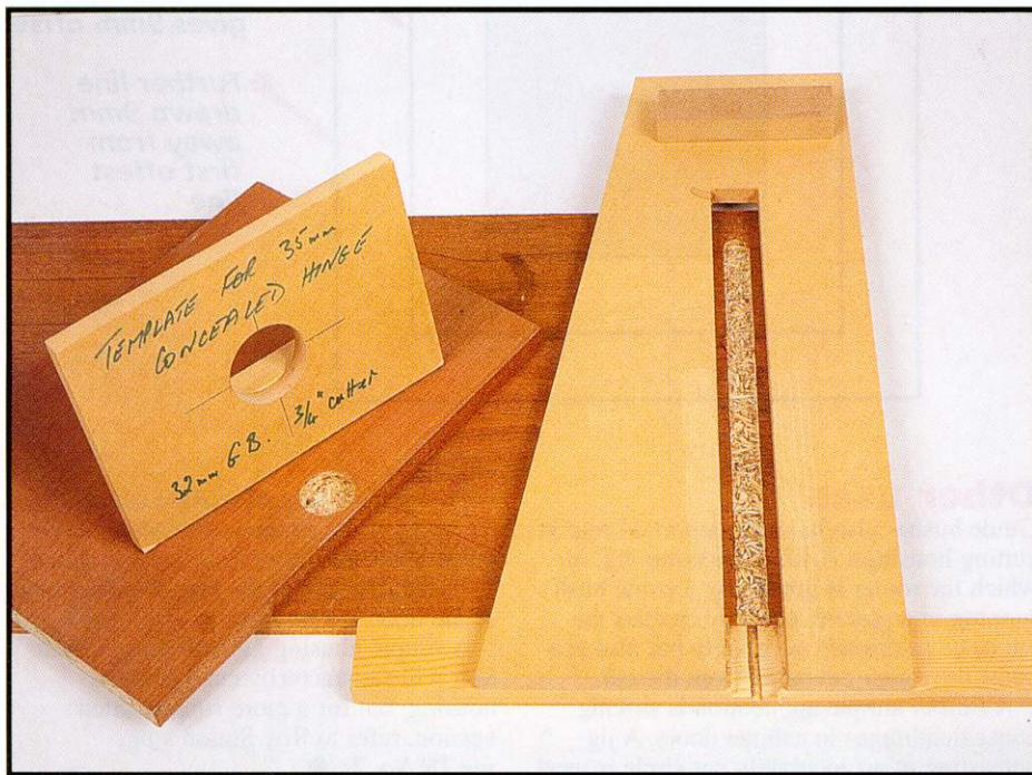
◀ Photo 6 Stopped housing being cut with a simple jig using a guide bush, plus hinge sinking jig with example of hole
