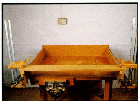
▲ Glue blocks inside the cover to help hold the plinth in place
