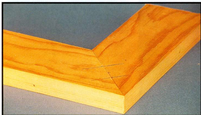
▲ Inserting biscuits into mitre joints is also possible with care
