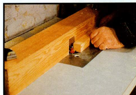
▲ Set up the cutter on an off-cut
