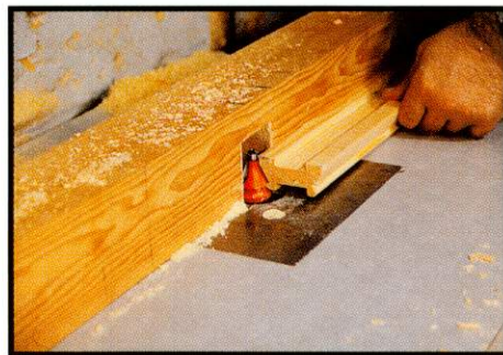
▲ The baserail uses the same cutter as the handrail
