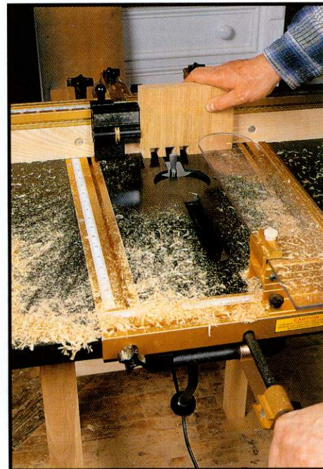
▲ The 'push me-pull you' cut action initially seems a little alarming, but holding the work with one hand while moving the router with the other feels OK
