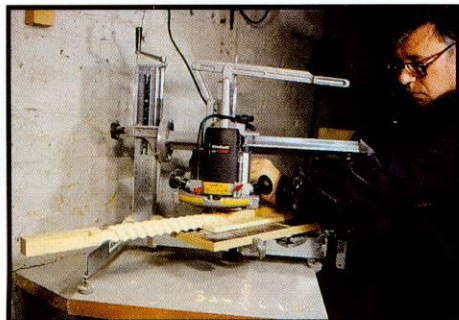
▲ Alternative but more complicated spindle design
