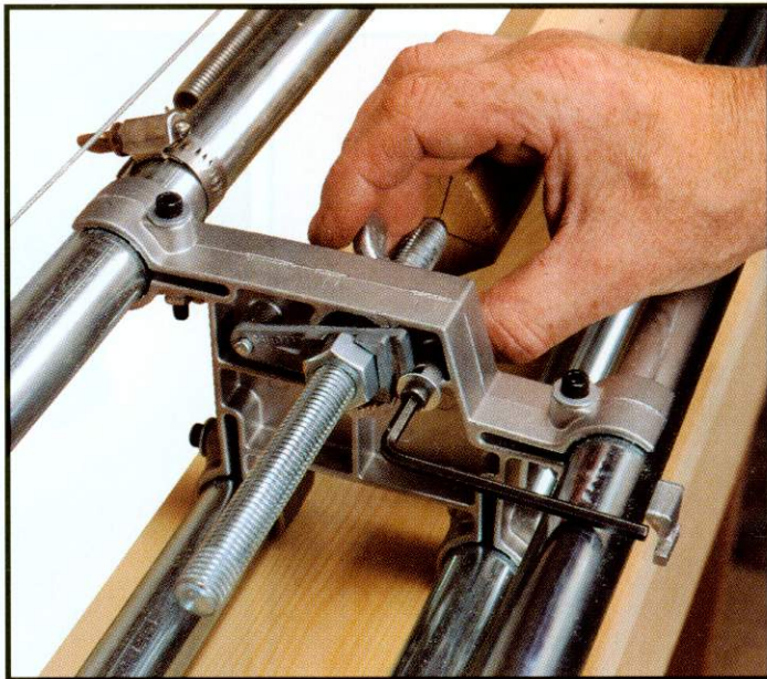
▲ Adjusting taper plate for parallel work
