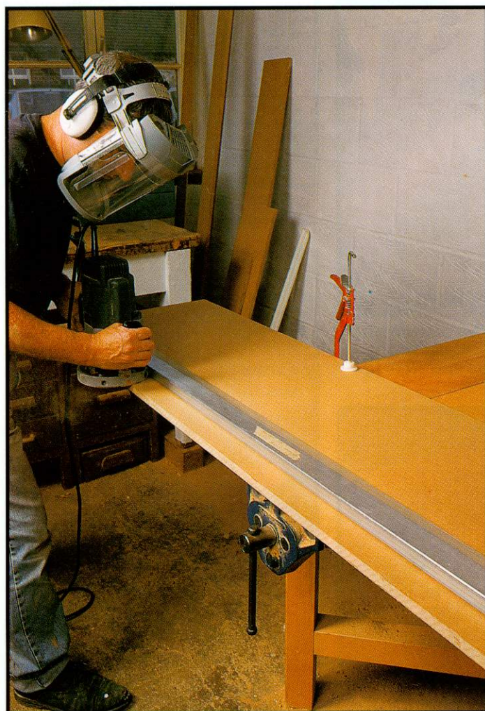
▲ The sheet of MDF is trimmed to size and edges cleaned up with a router
