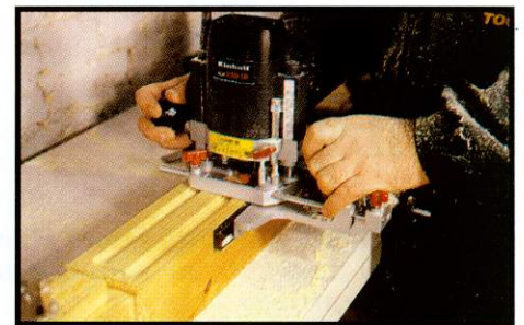
▲ Use a side-fence to rout the flutes
