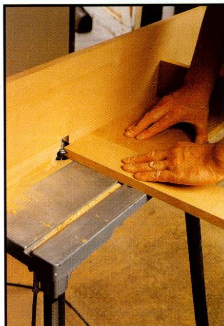
▲ The grille panel frame is easily made using a profile and scribe cutter set
