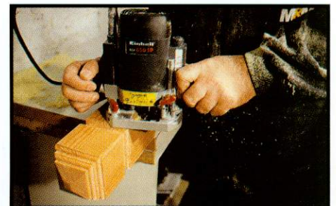
▲ A bearing-guided beading cutter finishes the corner
