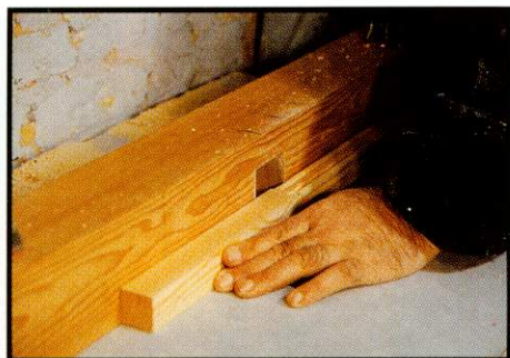
▲ Feed the workpiece carefully onto the cutter when starting the moulding
