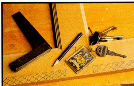
▲ Mark out the ventilation slots top and bottom of the panel
