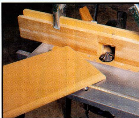
▲ The moulding on the top is formed using a large roundover cutter followed by a smaller one on the other side
