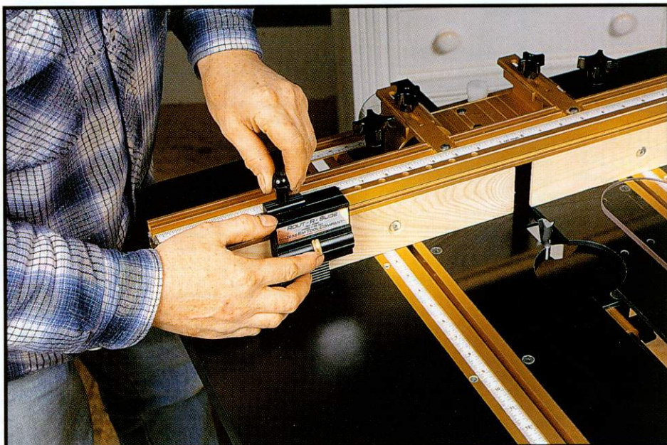
▲ A handy feature is the alloy stop which can be set at 25mm (1in) intervals
