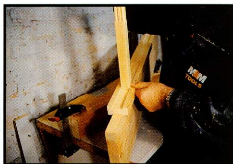
▲ Check the groove for fit
