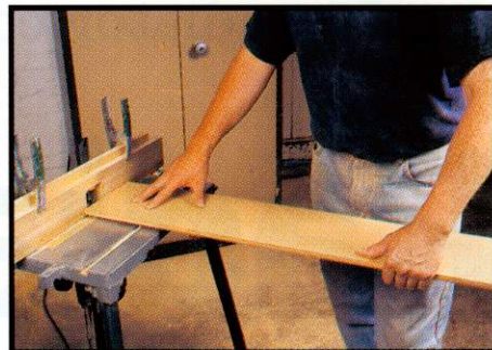
▲ Use a false fence with a small gap to support the workpiece when routing the ends
