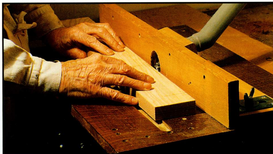
▲ The router inverted in a workshop-built routing table means the feed direction is right to left
