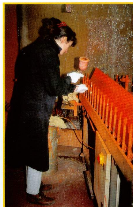
Any cutters that need it are finish-sprayed by hand
