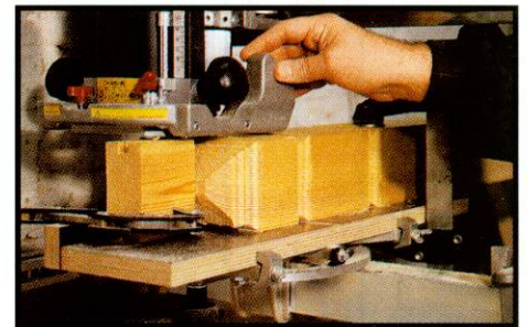
▲ The end cap and cross-mouldings are created using the router mounted on a Eumenia
