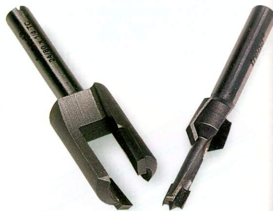
▲ Counterbore and plug cutters make a neat job of screwed joints
