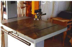
The large table on this bandsaw provides ample support for the workpiece. Note the auxiliary table that fills up the area between the table and the frame.
