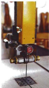
The upper guides are mounted on a sliding post that adjusts up and down to accommodate different thicknesses of lumber.
