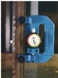
A meter that clamps onto the blade is the most accurate way to tension a bandsaw blade.
