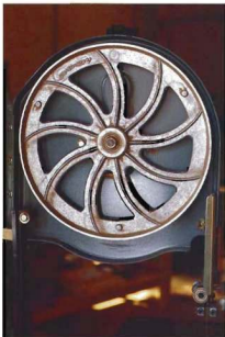
Bandsaw wheels cast from aluminum perform well when properly balanced.
