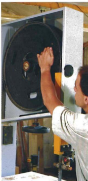
Tracking the blade is a two-handed job. Spin the upper wheel while adjusting the tracking knob until the blade rides on the center of the tire.
