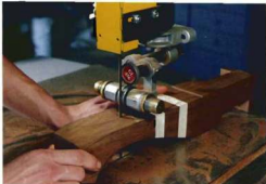
The bandsaw is the only simple way to cut compound curves such as those in this cabriole leg.
