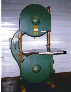
Weighing well over a ton, this 36-in. Tannewitz industrial bandsaw has a cast-iron frame that's rigid enough to tension wide blades and heavy enough to dampen vibration.
