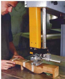
The bridges support the leg while sawing the second face.
