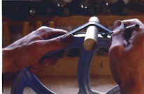
A dowel raises the tire off the rim so you can apply the glue underneath it with a small brush.
