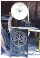
Although it looks a little rough, this 20-in. bandsaw needed only a good cleaning and a new set of tires. The price was less than half that of a new 14-in. saw.
