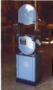
A 14-in. bandsaw like this one is inexpensive and versatile. It is the cornerstone of many home and small professional shops.
