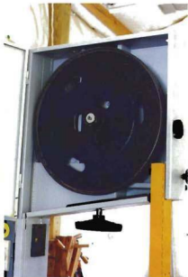
Cast-iron wheels have a slight advantage over aluminum wheels. The weight of a cast-iron wheel creates a flywheel effect, and the added inertia helps to propel the blade through the wood.
