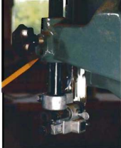
This simple friction device, found on a 14-in. bandsaw, uses a spring-loaded bearing to prevent the guidepost from falling.
