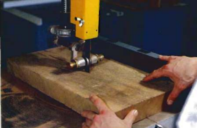
Ripping thick stock on a bandsaw is safer and easier than using a table saw. Use a wide blade and a sturdy fence.
