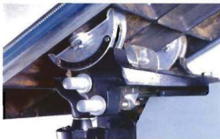
Trunnions bolted to the underside of the saw table allow it to tilt for cutting angles. (Photo by Scott Phillips.)
