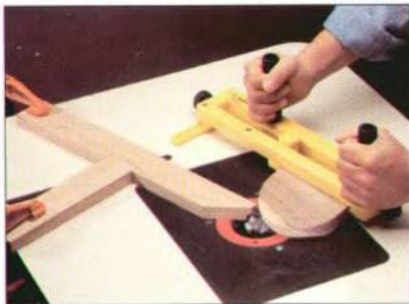
Jigs are essential for making a router both a safer and a more versatile tool. The workpiece handler shown above on the right is ideal for feeding small stock across a router table while keeping the operator's hands clear of the bit. The shop-made fence on the left provides a bearing surface for the workpiece and partially guards the bit.
