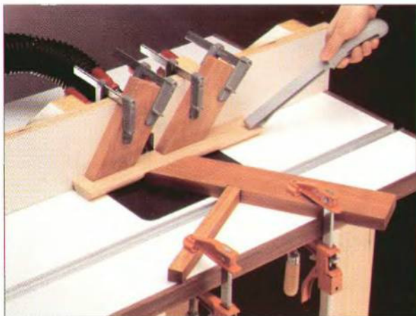
Three featherboards—two clamped to the fence and one to the table—hold the workpiece shown above safely against the fence and table while a push stick is used to feed the stock into the bit. Dust and wood chips are being extracted by a dust collection hose attached to a dust hood built into the fence.
