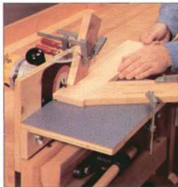
Mounted parallel to the tabletop, the vise-mounted router table shown above cuts one side of a sliding dovetail. Instructions for building this jig are on page 59.
