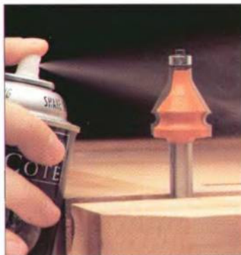
Lubricating a router bit with a silicone-based lubricant before and after using it will help prevent the cutter from overheating.
