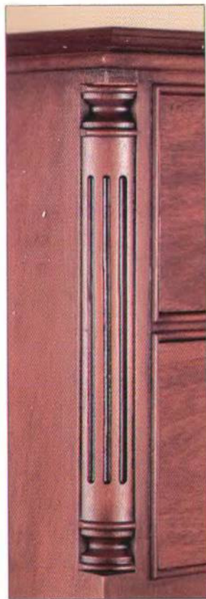
Fluted quarter columns add a touch of elegance to the Queen Anne highboy shown above. The flutes were cut by a router using the jig and technique illustrated on page 120.
