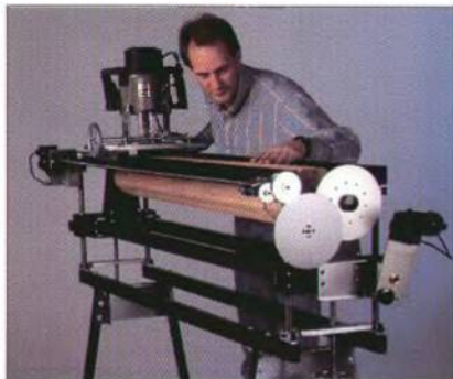
The commercial milling machine shown above transforms the router into a carving tool. Much like a lathe, the machine secures up to three workpieces between centers. Fixed to a metal plate, a router can then be fed along the bed of the machine by hand or with a motor drive. The router can also be left stationary while the crank is turned at the other end of the machine, rotating the workpiece into the bit.
