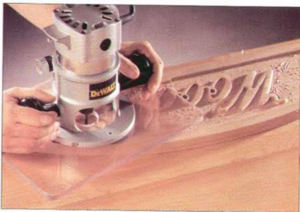
Fitted with a clear acrylic sub-base and a 1/4-inch veining bit, a router is used freehand to carve lettering into a piece of wood. The sub-base is transparent so the user can view the cutting action, and it is wider than a standard sub-base to help keep the router steady on the workpiece.
