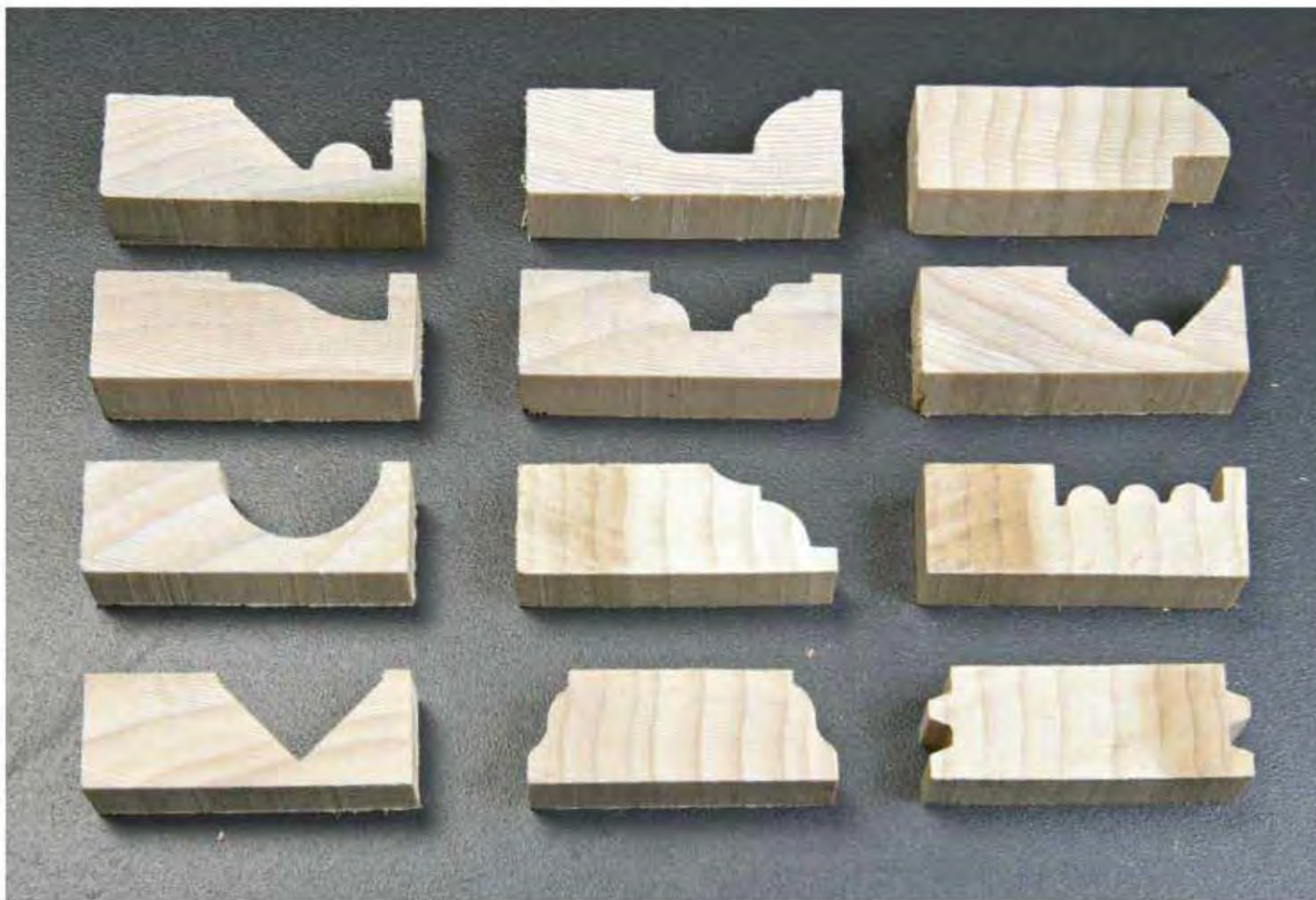
A profile library of cuts made with your knives allows easy layout of custom moldings.
