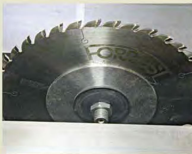
A stabilizer is a thick metal disk that mounts directly against the blade body.
