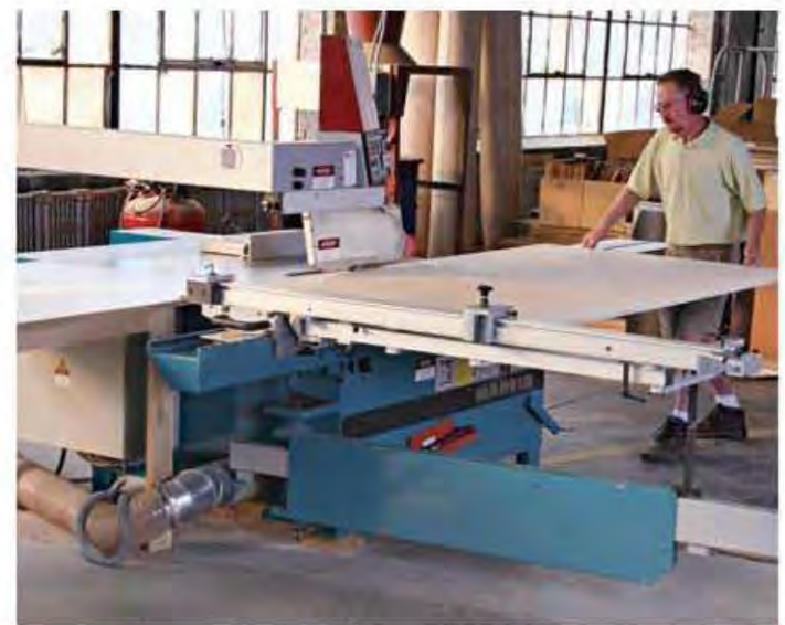
This behemoth panel saw makes cutting sheet goods a snap because of its 10-ft. table travel and other features.
