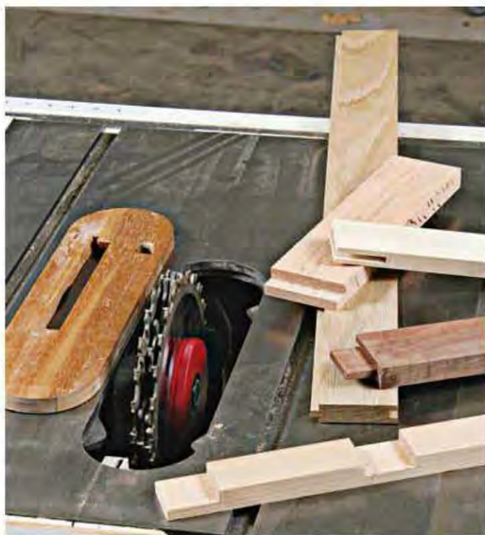
A dado head is invaluable for cutting rabbets, dadoes, grooves, tenons, and open mortises on the tablesaw.
