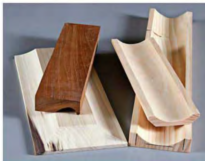
The symmetrical coves at right were cut using an angled fence with the blade vertical. The asymmetrical cove at left was cut with an angled fence and a tilted blade. The raised panel is a result of half-coves.
