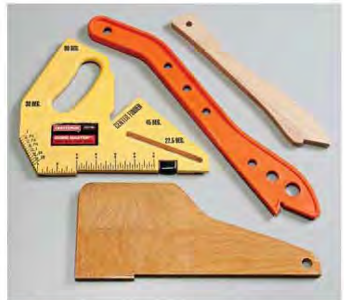
The long-handled push sticks at top provide minimal stock control. The shoe-style push sticks allow good downward pressure as well as positive forward feed force.
