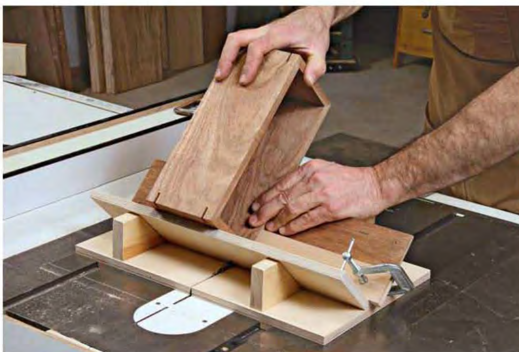
A cradle jig is necessary to hold boxes and other casework at the proper angle when cutting slots for keyed miter joints.
