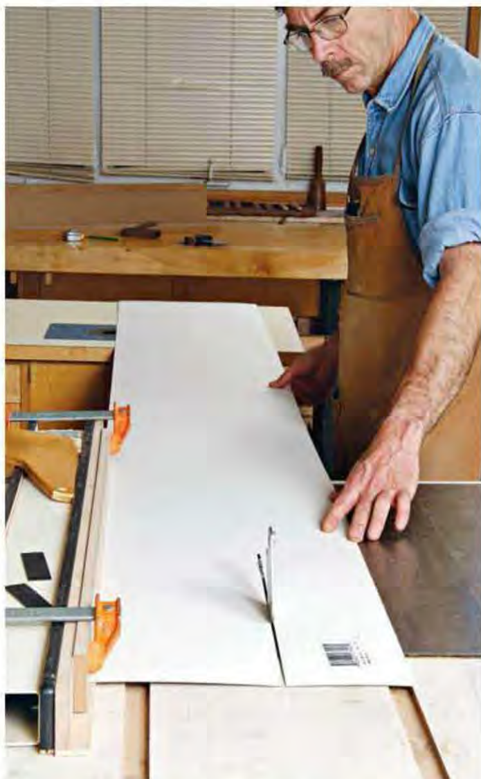
A router table the same height as the saw serves as great infeed support for floppy, thin materials such as this piece of plastic laminate.
