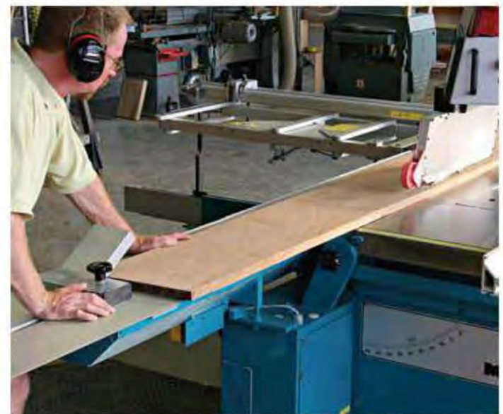
A panel saw can rip a straight edge on a board. Pinch the board at its ends onto the sliding table and then push forward.
