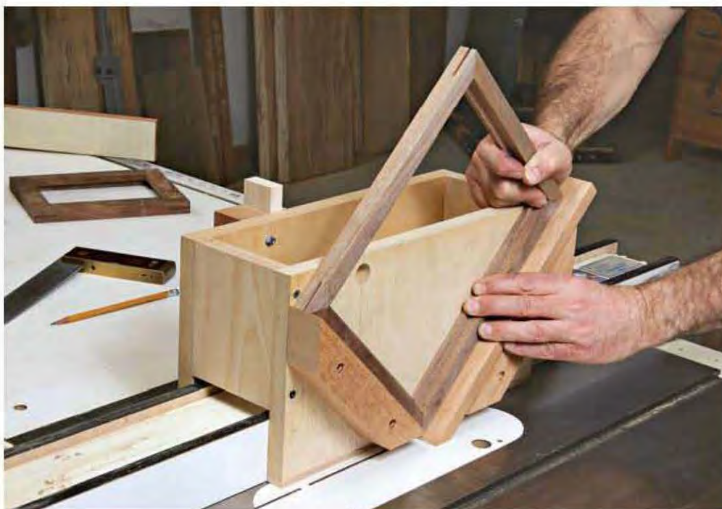
A jig for cutting slots for keyed miters carries the glued-up frame across the blade at 45 degrees.
