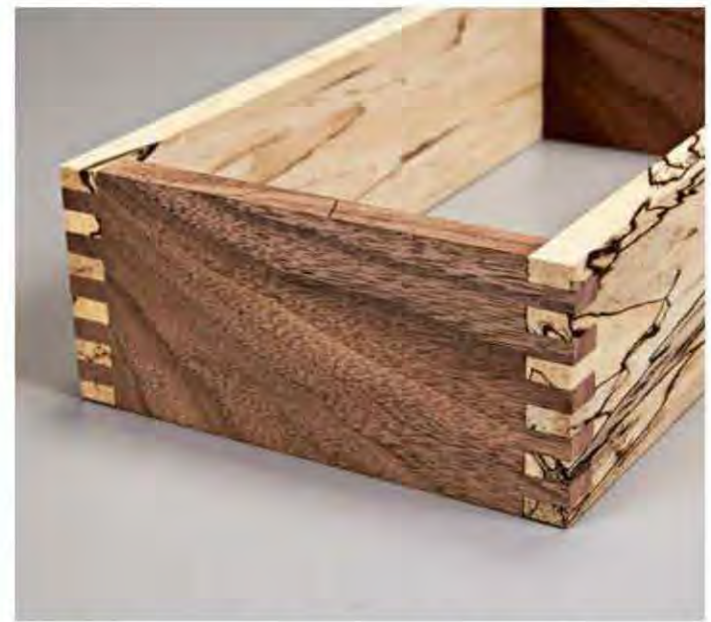
The interlocking fingers on a finger joint provide a strong mechanical connection as well as plenty of face-grain glue contact.
