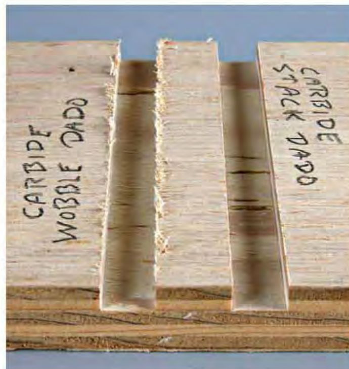
A cut from a wobble dado (at left) will require considerable sanding compared to a cut from a good-quality stack dado (at right).
