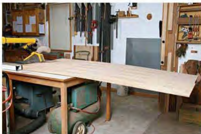
An outfeed table that extends 50 in. past the saw splitter will prevent a standard 8-ft.-long panel from tipping after the cut.
