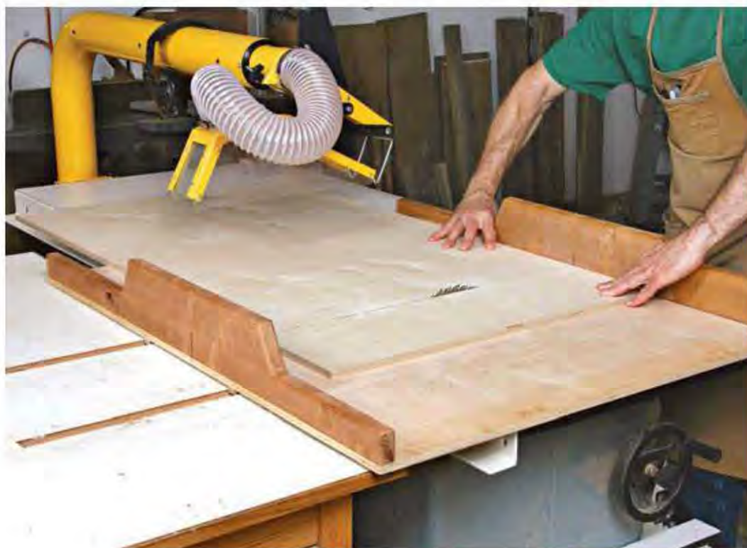
A shopmade crosscut sled that rides in your saw's miter gauge slots is just the ticket for crosscutting panels and other large workpieces.
