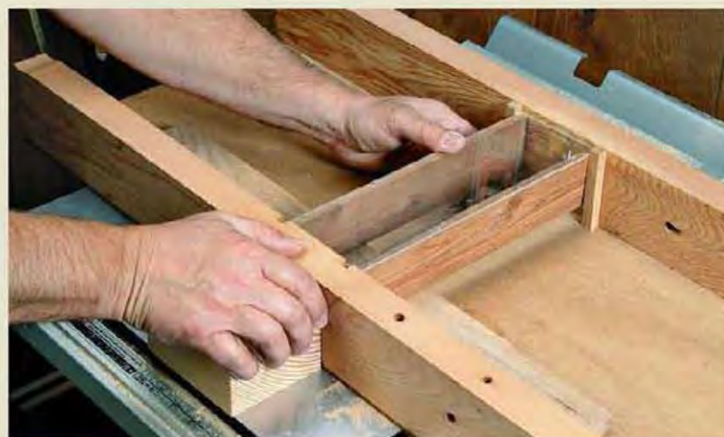
Sandor Nagyszalanczy's crosscut sled includes a blade guard that can be slipped in place atop the workpiece to be cut.
