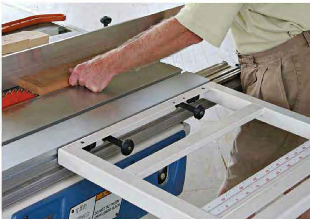
The protruding sliding table bed on a European saw necessitates working more from the side of the saw rather than from the front.
