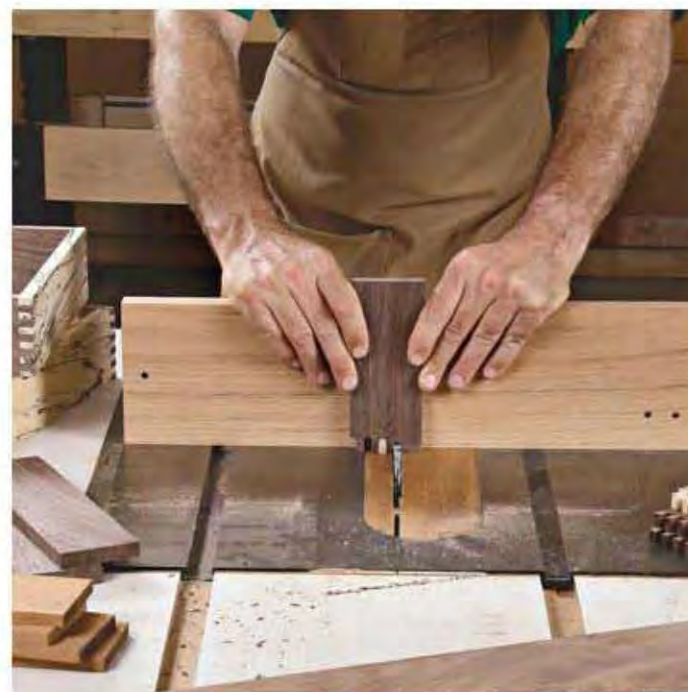
A finger joint jig is quite easy to make and allows you to cut strong, attractive box and drawer joints.
