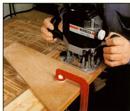
Photo 2 Rebate being cut with a hand-held router and a simple jig. Note anti-breakout piece behind workpiece – Photo 2 shows the rebate being hand-cut in the end of a board using a \frac{1}{8} in straight cutter and a simple jig.
