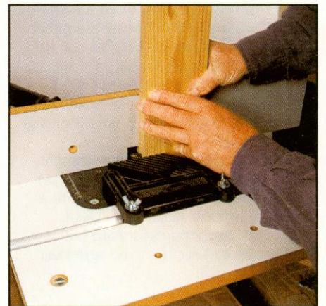
Photo 7 The second cut in the drawer front makes the groove for the side tongue
