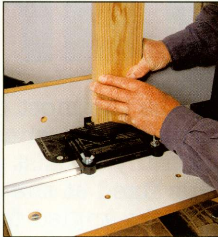
Photo 5 The end of the finished joint being trimmed with a flush-trimming cutter
