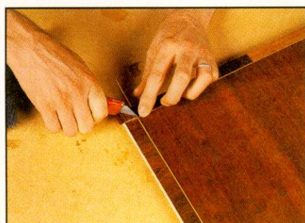
Cutting through both layers to form a mitre
