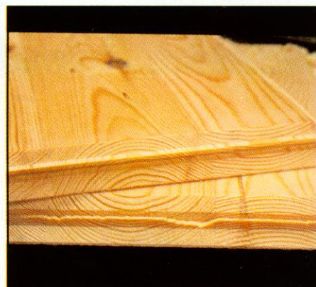
Beware of damaging tear-out on cross-grain passes
