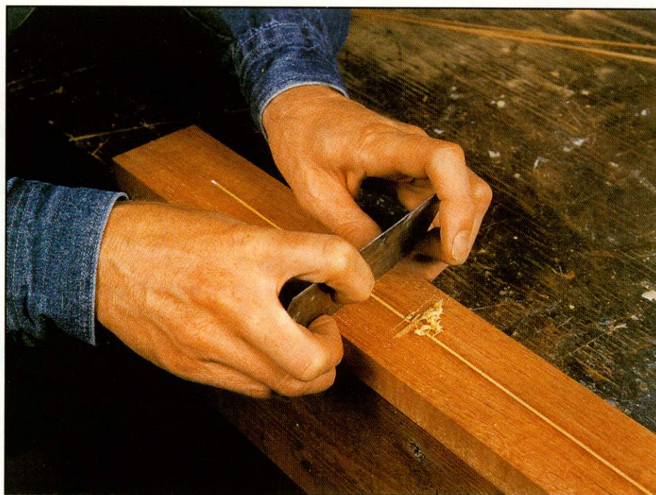
Stringing should be cleaned up with a quality cabinet scraper
