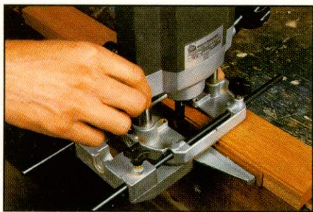
Back-feeding the router gives a cleaner rebate for edgebanding
