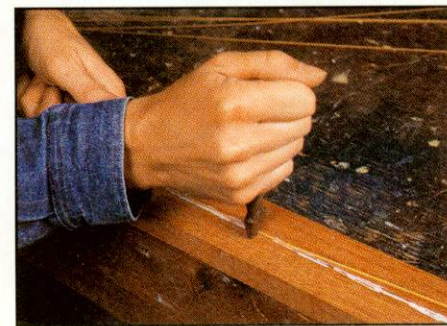
Be sure to press the stringing in very firmly
