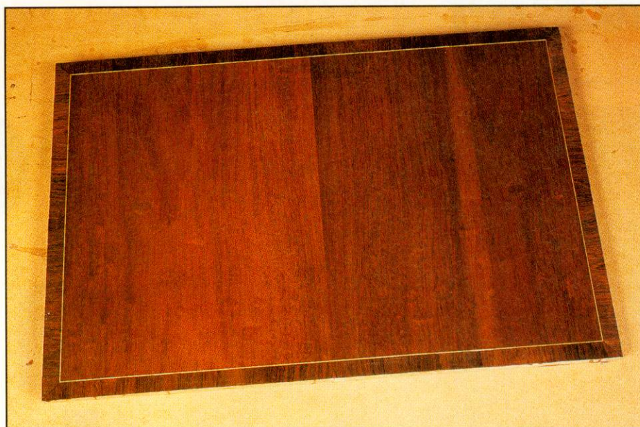
Complete all four sides then set aside to completely dry before trimming and crossbanding the edge
