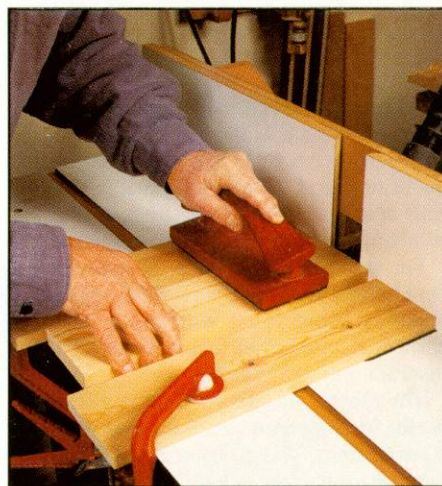
Photo 9 The end grain of the first board being slotted for a biscuit joint on my home-made table. Note the use of a safety push block and the two boards used to set the limits of the cut
