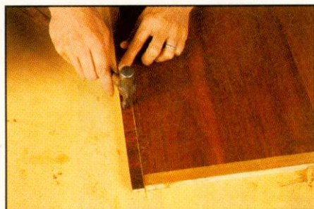
Lay the first piece of crossbanding and stringing against the main veneer
