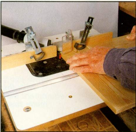
Photo 4 Cutting the rebate of a rebate-and-groove joint
