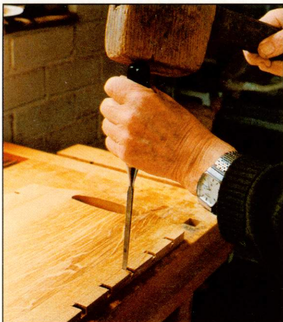
▲ Cutting the sockets on the front piece...
