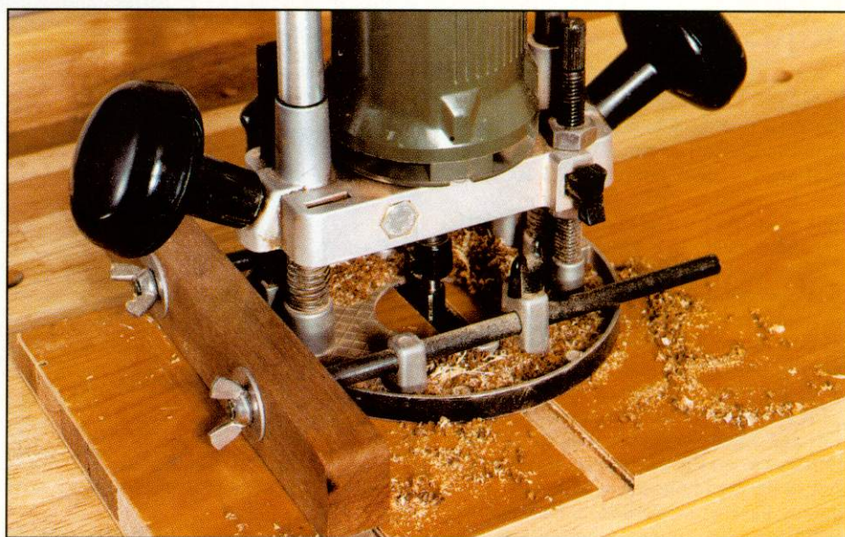
▼ Routing a housing with the foot jig
