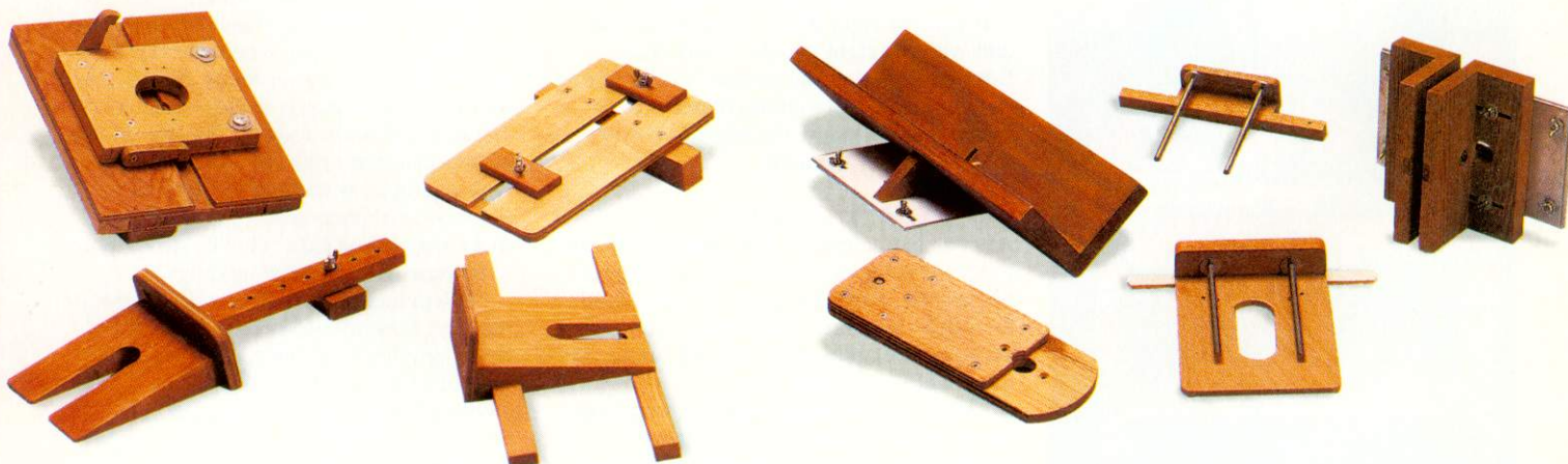
▼ Examples of Bob's ingenuity, including sub-bases for angled routing
