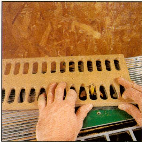
▲ Making a copy jig overhand, pre-drilled entry holes are needed here
