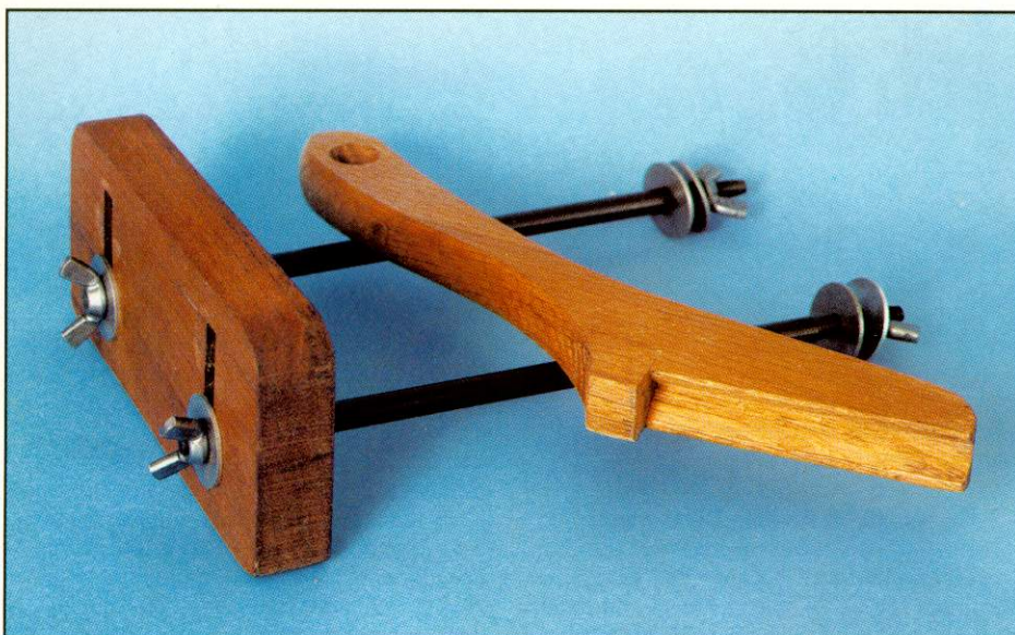
◀ Vanguard Routing Rods and a V-groove push-stick help keep things safe
