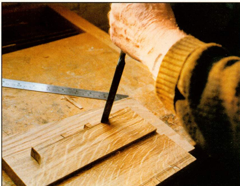
▲ ...and cutting the tails in the side piece
