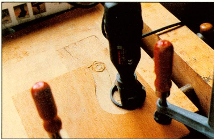
▲ The template in place to guide the Dremel through the scroll pattern
