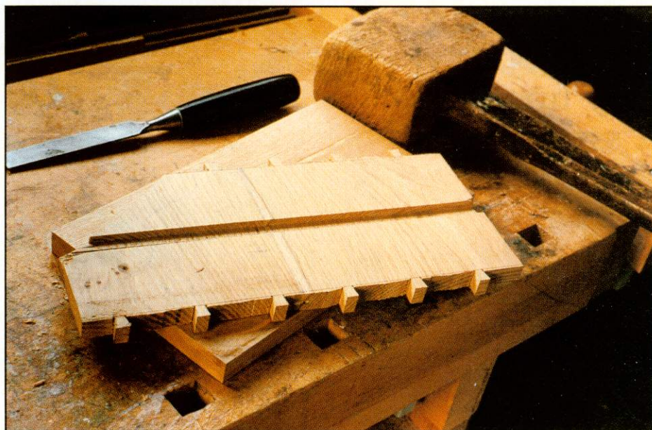
▲ Groove cut in the side piece to take the divider
