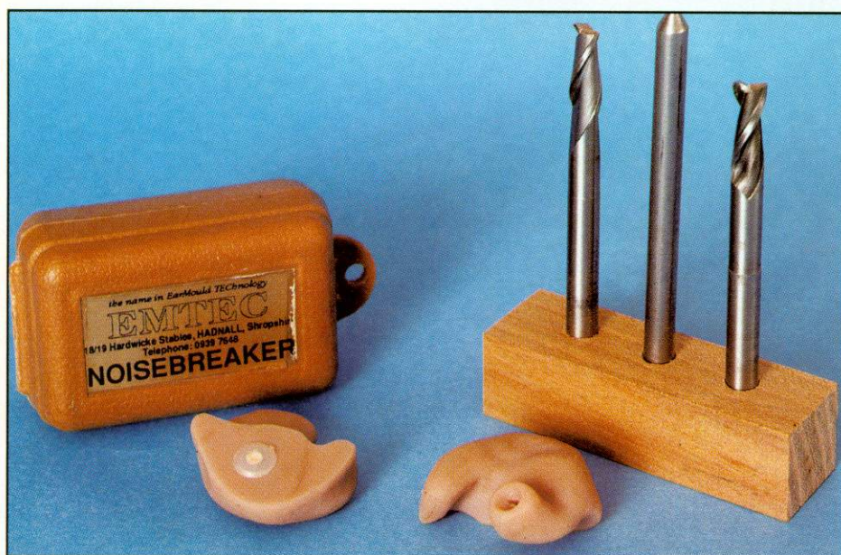
◀ Ear defenders, a 1/4in locating point, and two 1/4in milling cutters, good for cutting deep mortices
