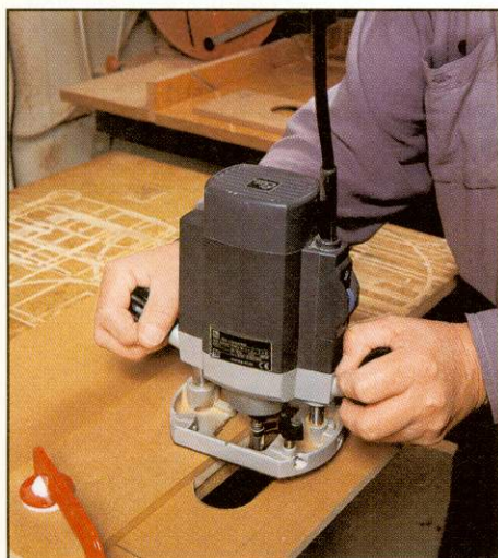
▼ Template being finished with router, profile guide-cutter and straight edge
