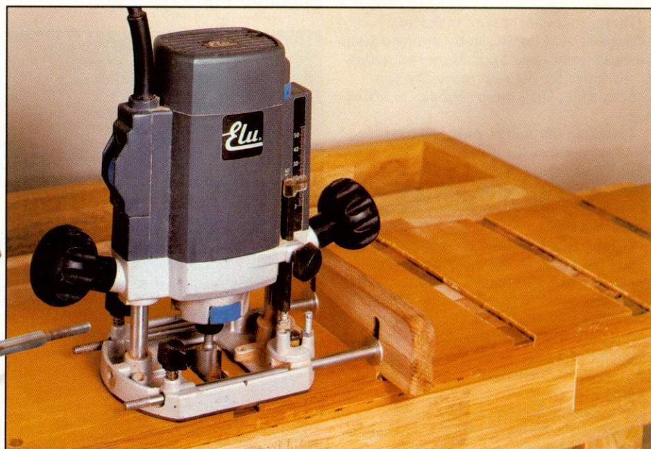
▼ Foot to fit the housings with router rods
