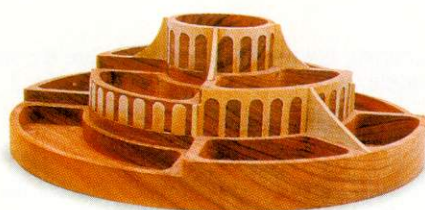
▲ The Lemonwood fillets added, veneer rampart arches glued in place. Waste from the veneer is used on alternate quadrants
