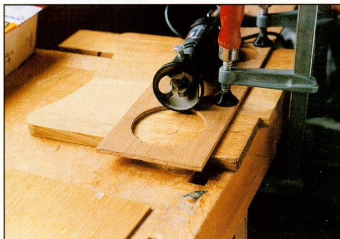
▼ Template for the circular parts of the pattern
