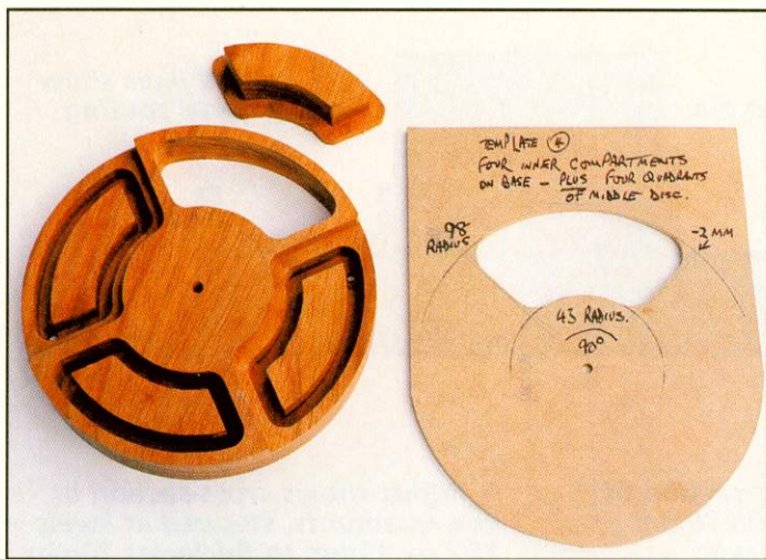
▲ Second disc routed in outline with one of the compartments cut out...
