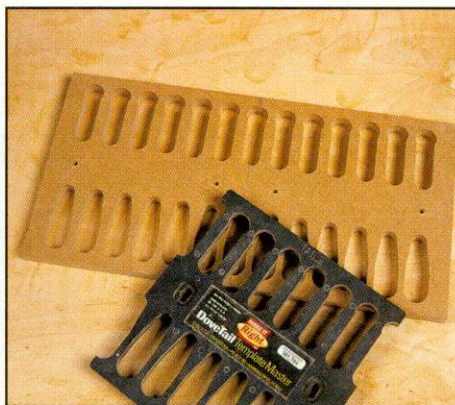
▼ The finished jig copy
