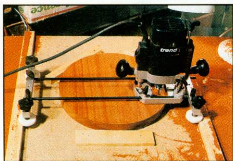
▲ Using the Trend pivot frame jig to plane the base disc flat
