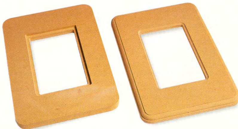
▼ Two finished frames, one shows the rebated back, the other the moulded front
