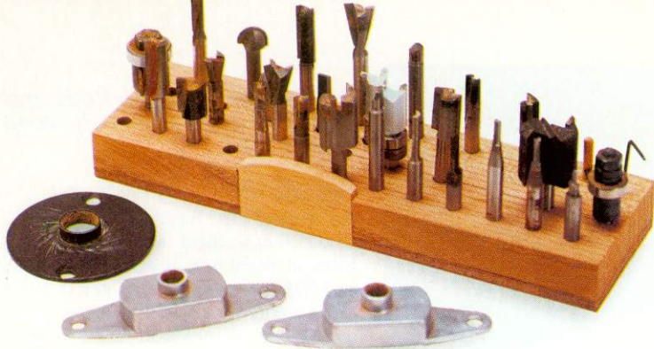
▲ A variety of cutters, including straight, dovetail and bearing-guided cutters. The alloy guidebushes are an older Bosch pattern
