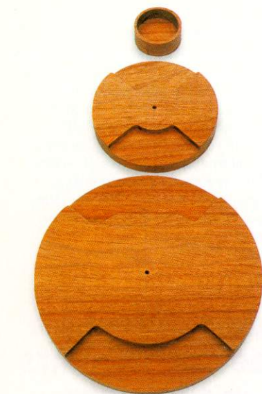
▲ The three levels, ready to rout the compartments...
