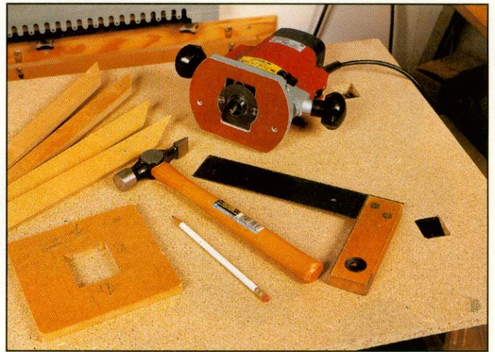
▲ Cutting table with router, 1 1/4in cutter, 24mm guidebush, and template. Note the 'universal template' of straight edges
