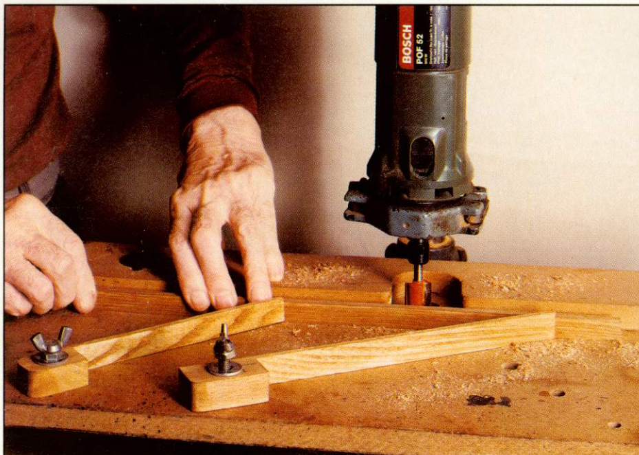
▲ Overhead routing with the small Bosch router in an old Wolf drill stand. Note the adjustable fence with chip extraction
