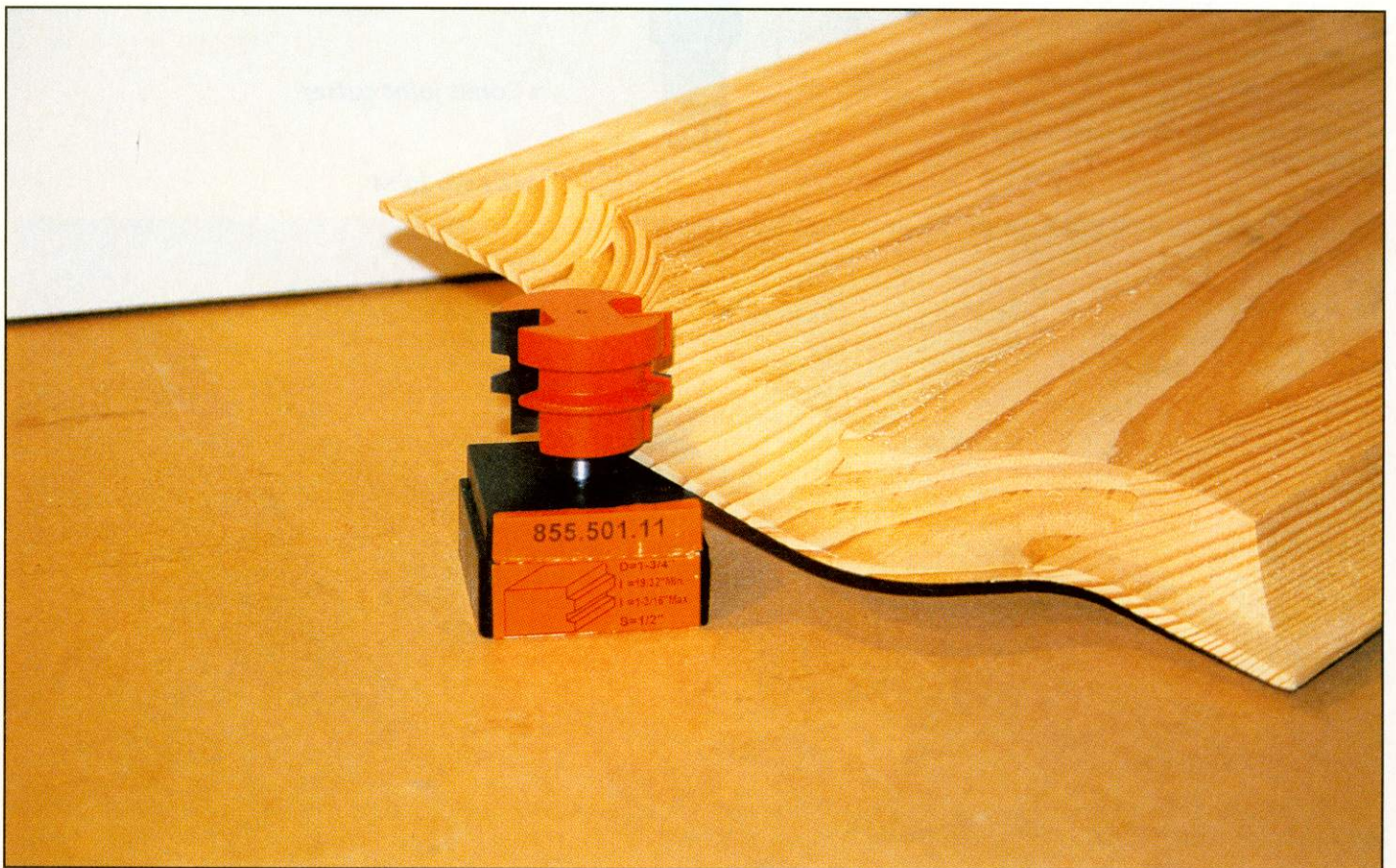
▲ Using two cutter blades and a square blade with the comb joint cutter ▼ A reverse glue joint and cutter, blended with a raised and fielded cutter
