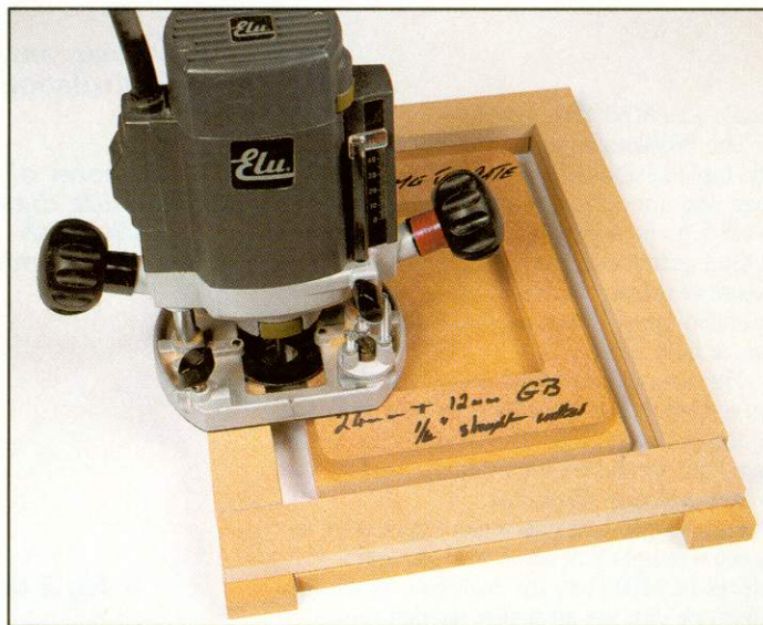
▲ The template on the workpiece with packing pieces around the outside to stabilise the router, made with scraps of MDF and a hot-melt glue gun
