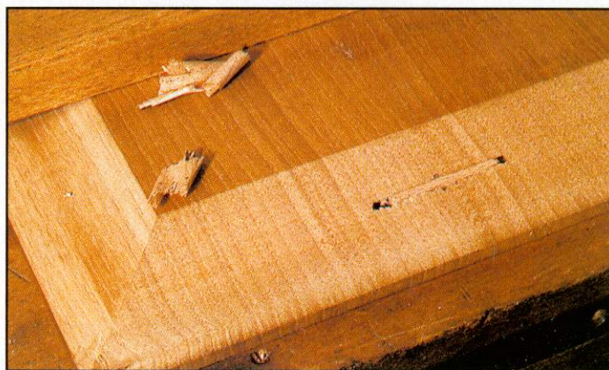
▲ Remember to site dowels or biscuits well clear of the fielding
