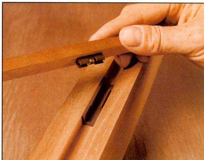
▲ The S-Klick clips straight in to mount small sections
