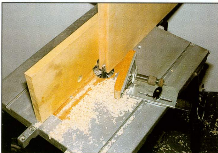
▲ Routing the 1/4in rebate. Note the high fence
