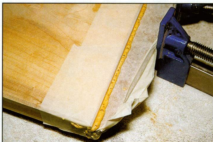
▲ Gluing the handles onto the board. Note the masking tape and foaming adhesive
