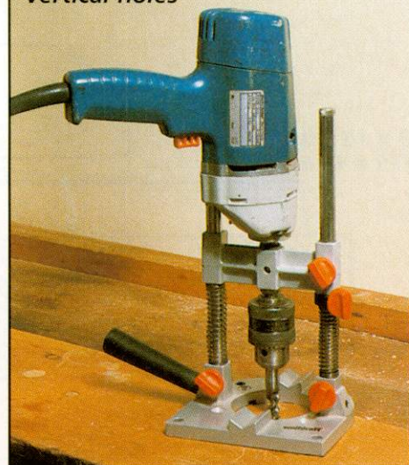
The drilling aid ensures truly vertical holes
