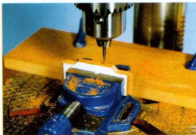
Turned legs being mortised out on a drill press with a 2mm rotary rasp fitted
