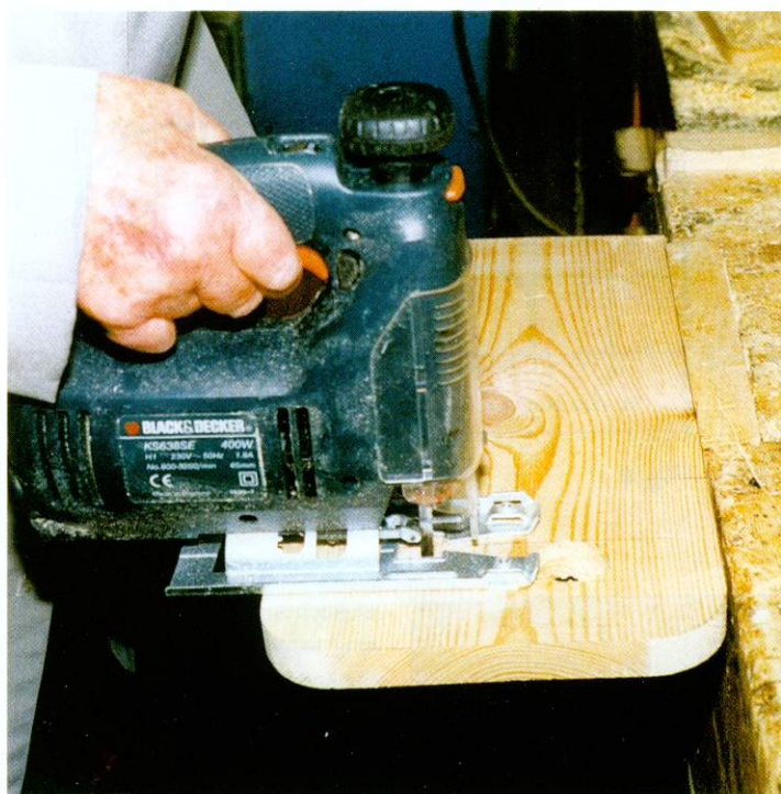
Cut hand hold between holes.
