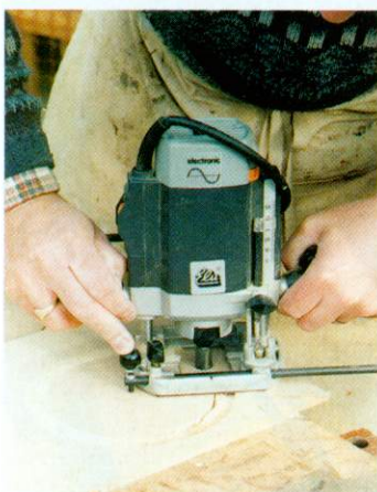
A trammel bar is used on the router to cut a disc from the MDF. The disc is discarded
