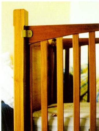
Self designed brass brackets
