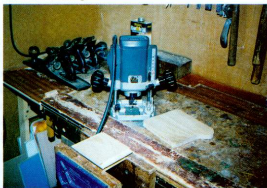
Half lap routed workpiece to be cut to width for two sides, also base before routing
