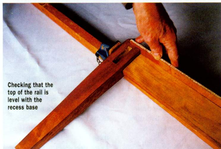
Legs and rails before assembly
