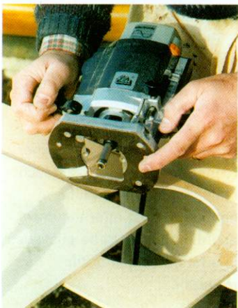
A bearing guided straight cutter is used to make the final template
