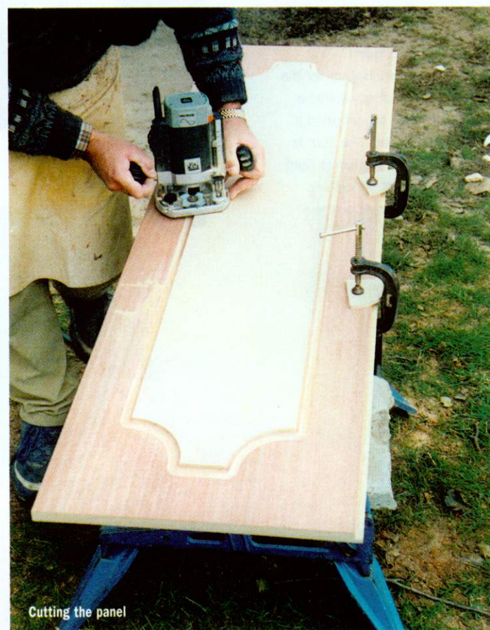
The completed template is pinned centrally on the bath panel. The guide bush and cutter can be seen
