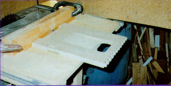
Bottom of leg being cut away
