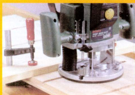
The side panels receive 8 grooves each to accept the side runners. The router is guided by a clamped on fence
