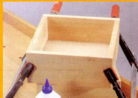
The four drawer sides are joined with dowels and glue. Cramp the parts together
