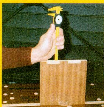
Checking depth of recess
