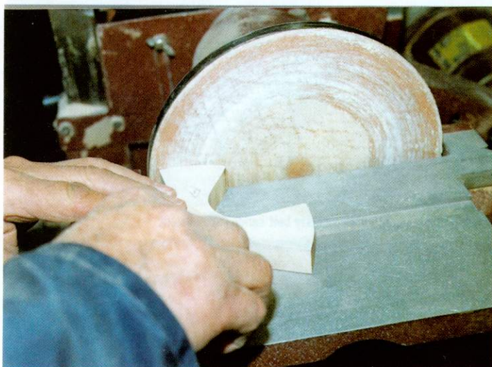
Cleaning up the external surfaces
