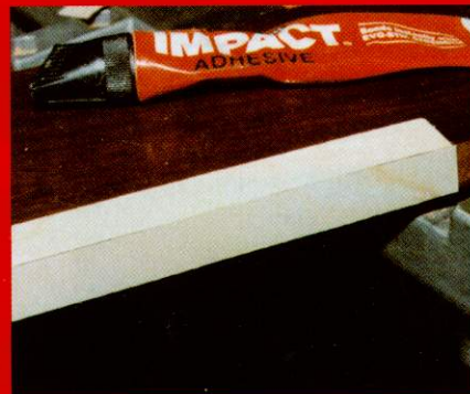
Impact adhesive used to fix Formica
