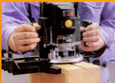
The runner grooves, stopped at the front, are cut into the drawer sides. Guide the machine with a straight fence
