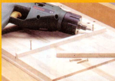
The side runners must not be fixed with glue. They are fixed with countersunk wood screws to allow the wood to move
