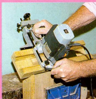
Mitre jig in action with a router
