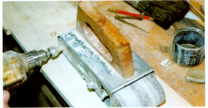
Sanding plank smooth with a trusty belt sander attachment
