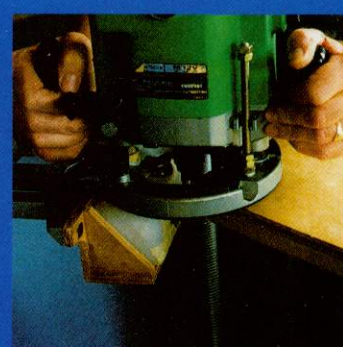
A template profile cutter with shank bearing used to finish off the round
