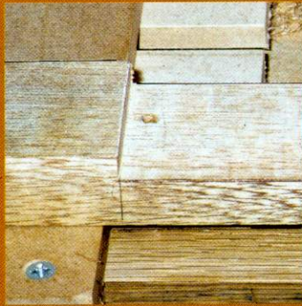
Cross cutting jig - completion of wide groove
