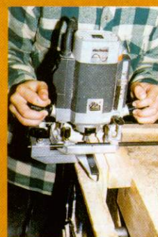
Use guide piece when dovetailing ends
