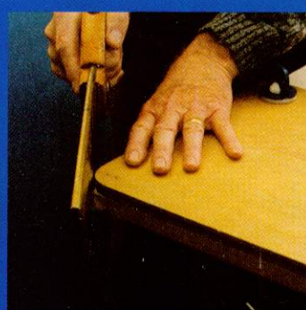
Prior to trimming using the external radius template cut off the waste
