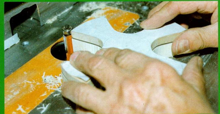
Final trimming using a bearing guided trimmer cutter
