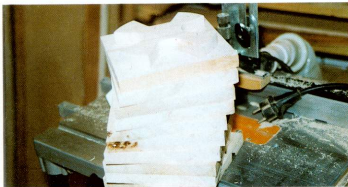
Stack of 6in. square sections cut and ready
