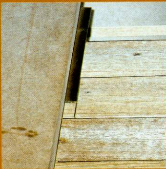
Cross cutting jig - wide groove set up for routing
