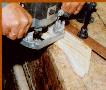
Round over shaped edge of bracket
