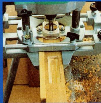
The L/H fence was designated the face side for all mortises
