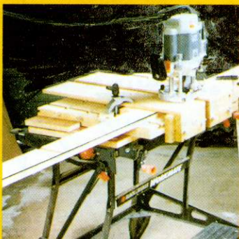
Cross cutting housing in rails J
