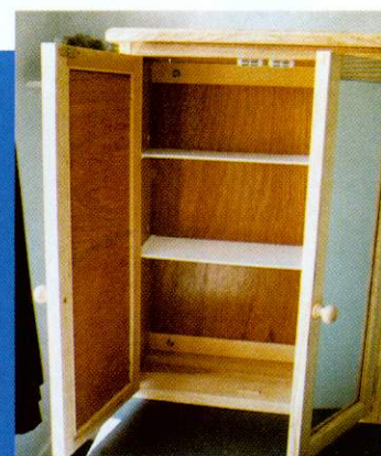
Chest showing shelves, door catches and fixing screws through back rails
