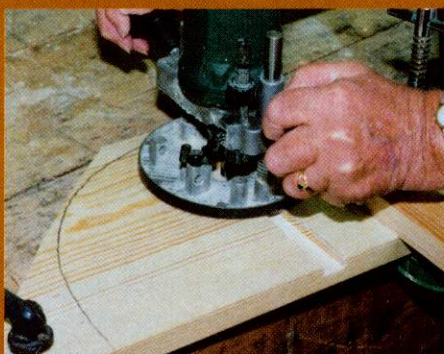
Cut groove with router against guide strip
