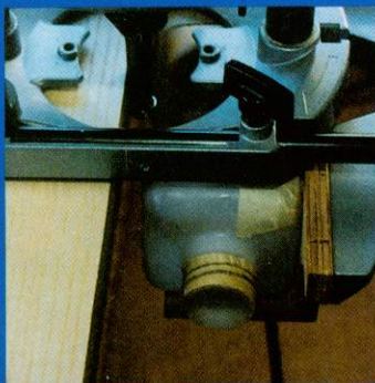
A self-guiding trimming cutter will need effective dust extraction
