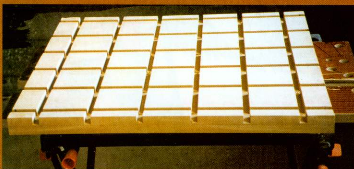
Cross cut jig - first stage of making baseboard
