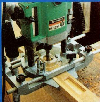
The router is set to position the mortise in the centre of the stock
