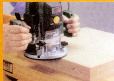
Base and top edges are also rounded with the ovolo. Do this in two operations
