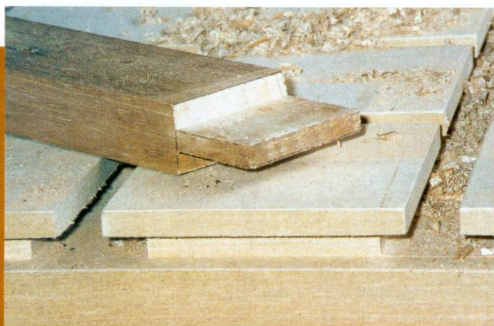
Cross cutting jig - completed tenon
