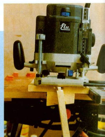
6 & 7 Cutting dovetail on angled leg - note use of scrap to avoid breakout.
