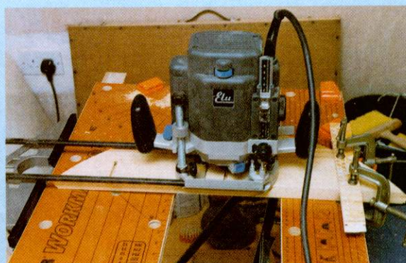
5 Cutting second dovetail housing.
