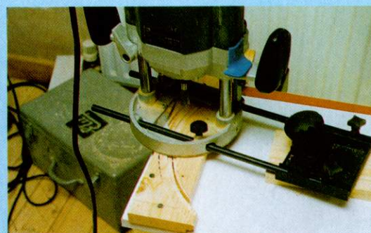
14 Rebate being added to rear of retainer.
