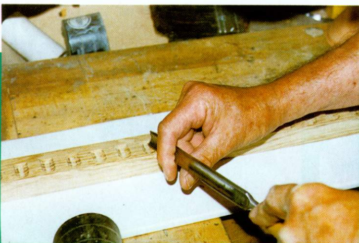
16. A gouge the same width as the tumbnail is best.
