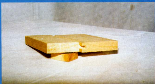
Completed tongue and groove joint.
