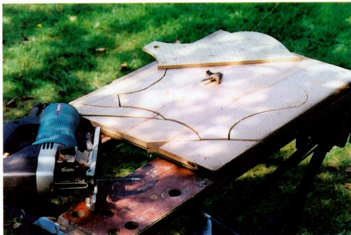
The shield is cut to rough profile.
