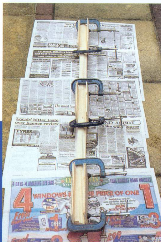
Dado rail is glued to the square edge timber to make a suitable section.
