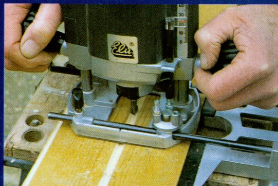
Central Vee joint being routed.
