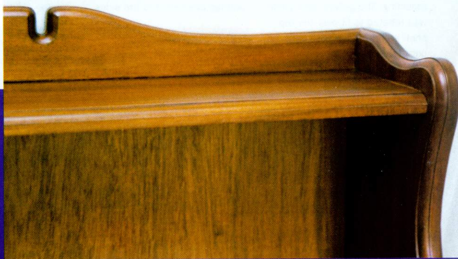
5. Detail of gallery, showing mitred corner..
