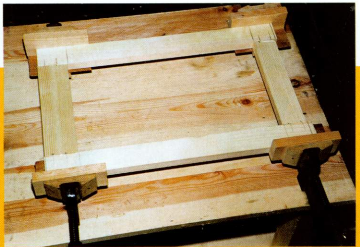
Door frame glued and cramped.
