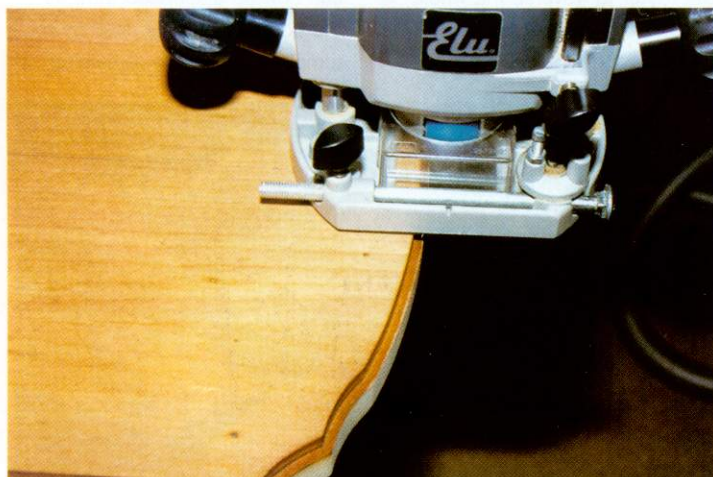
6. The pattern for the glass mirrors was produced by traversing with a rebate cutter set to the required depth.
