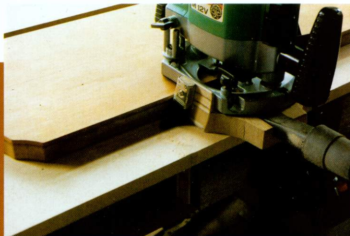
5. Providing concentration can be maintained together with a smooth traverse of the template an excellent finish can easily be produced.
