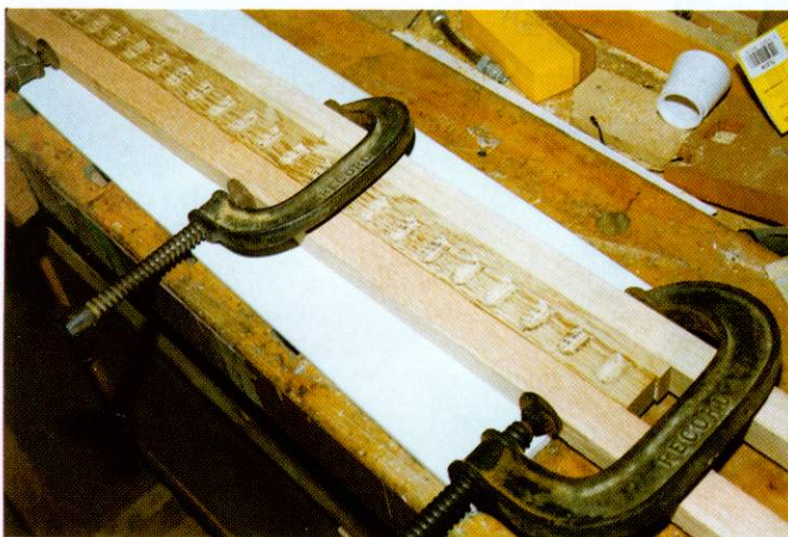
14. The original strip is glued and clamped to the moulded strip.
