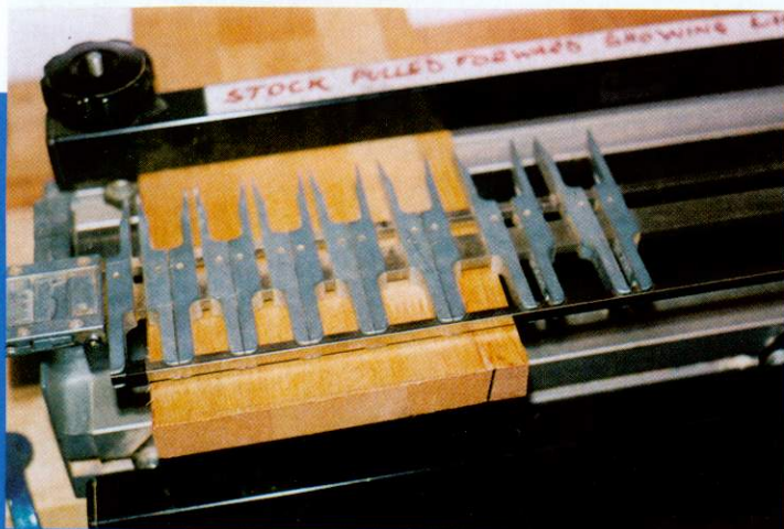
Stock advanced to show line of cut scribed across timber.
