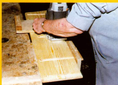
Grooving for shelves. Bench hook as guide.
