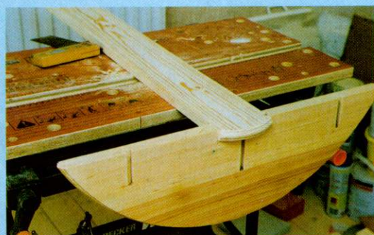
12 Test fit of mirror support to shelf.
