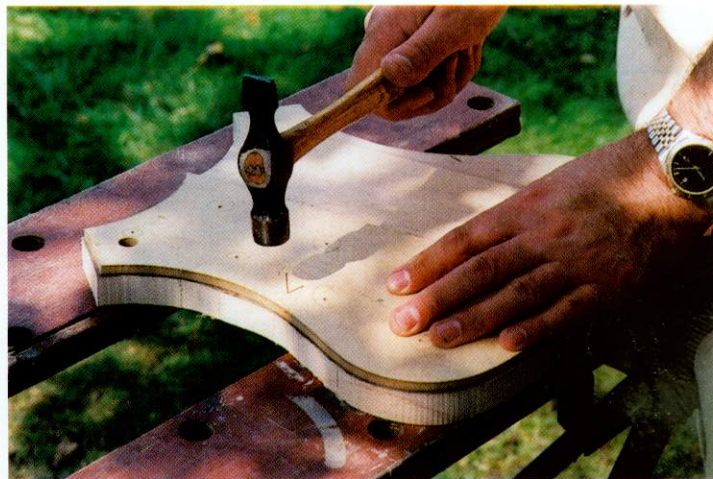
The template is pinned in place.
