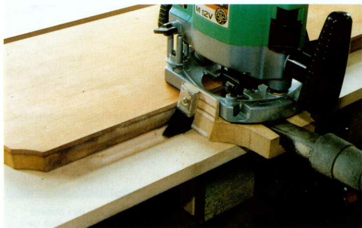
3. Although it doesn't look high tech the end of an old 1in. paint brush effectively sealed the gap left by the moulding.
