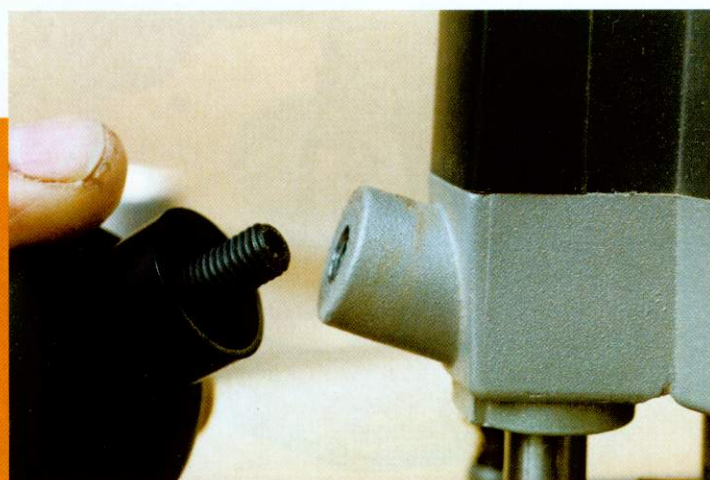
It is possible to remove the non-locking knob completely giving a good deal of extra clearance where required.
