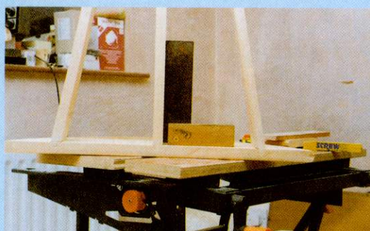
8 & 9 Initial fitting of legs - note breakout on shelf - should have been avoided by use of scrap clamped in place before routing.
