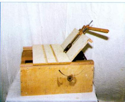
Hinged router bracket set at 45 degrees.
