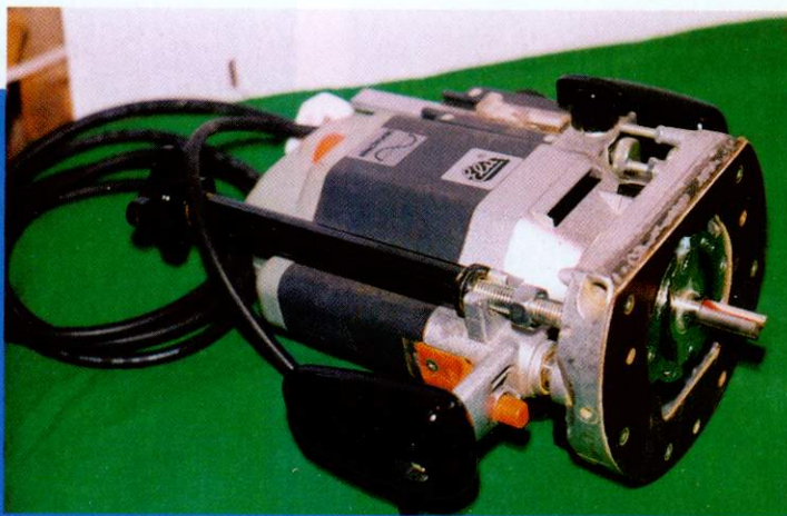
Elu E177E fitted with Leigh guide bush carrier 5/8 inch bush and 1/2 inch diameter cutter.
