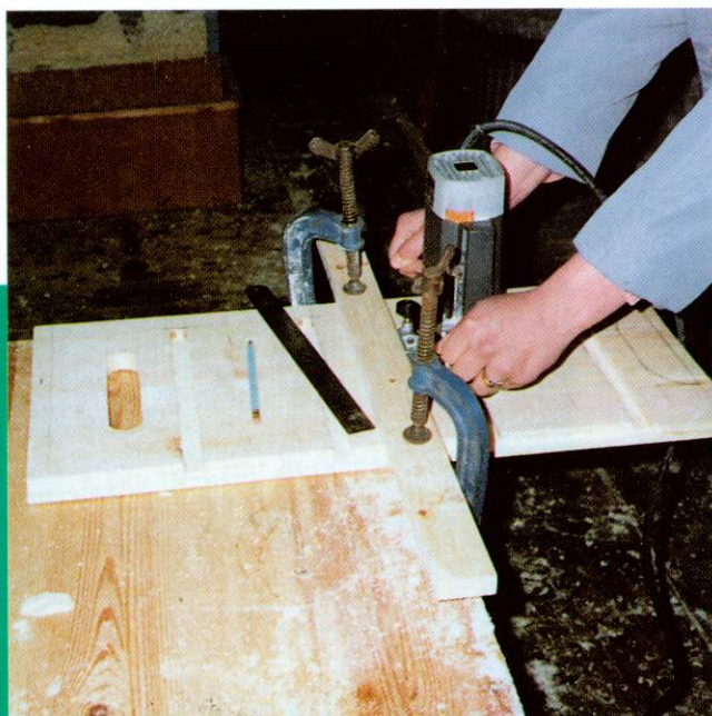
Cutting housing against guide strip.
