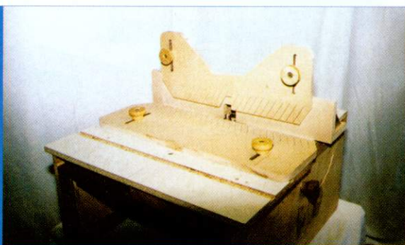
Router table in spindle mode with fence and spring pressure plates in position.
