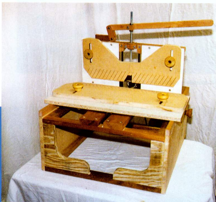
Comb joint jig in place.
