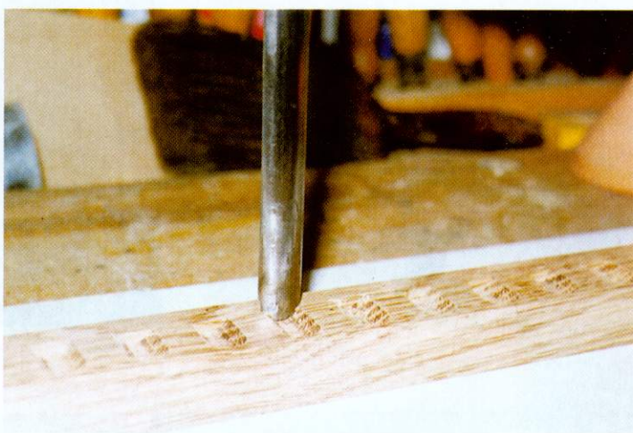
15. As there is little to remove a light tap with a mallet makes an incision.
