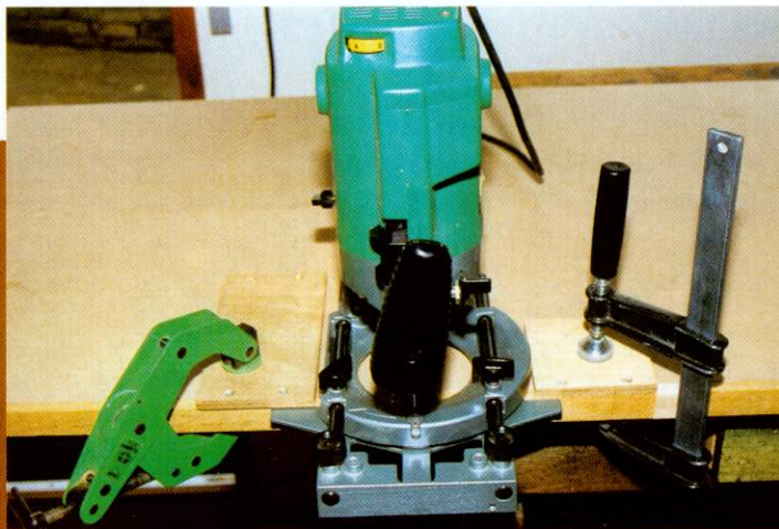
9. With the rod in place the hinge positions can be accurately transferred onto the framing.
