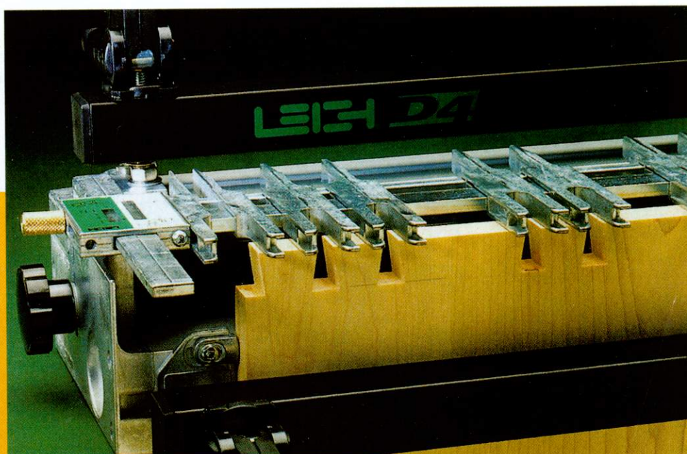
Leigh D4 jig, set up to cut tails.
