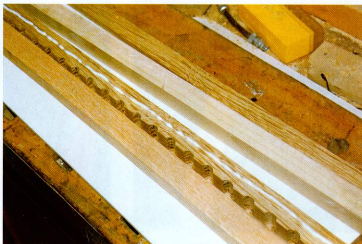
13. A bead of glue is spread along the surface.
