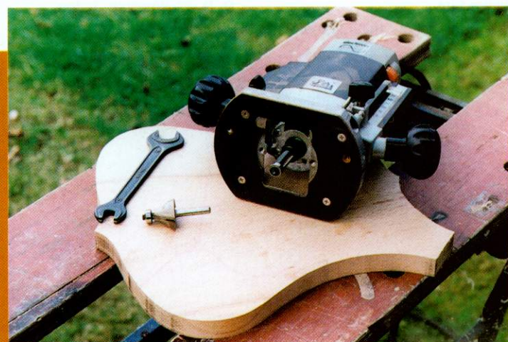
The shield profiled, in the foreground is the moulding cutter.
