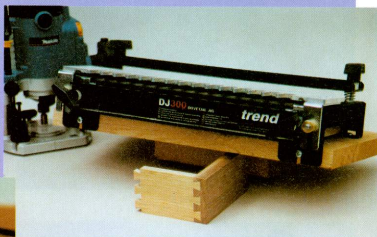
A dovetail jig is used in the drawer construction
