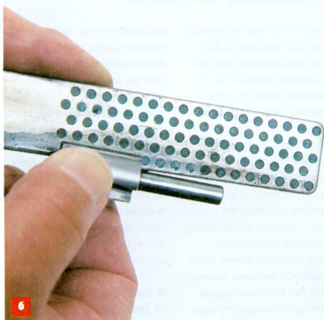
Honing a 5/8in straight cutter. Woodcut extra fine (Green) hone
