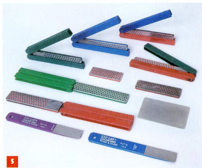
Selection of diamond hones suitable for router cutters
