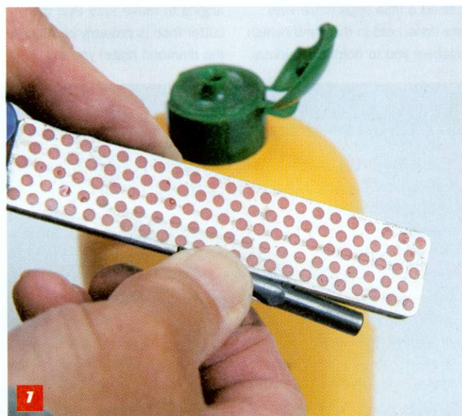
Honing 1/4in straight cutter. DMT Double Diafold hone. The small diameter of the cutter makes this difficult
