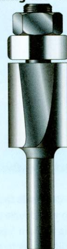
Fig 4 Cutter for trimming the laminate
