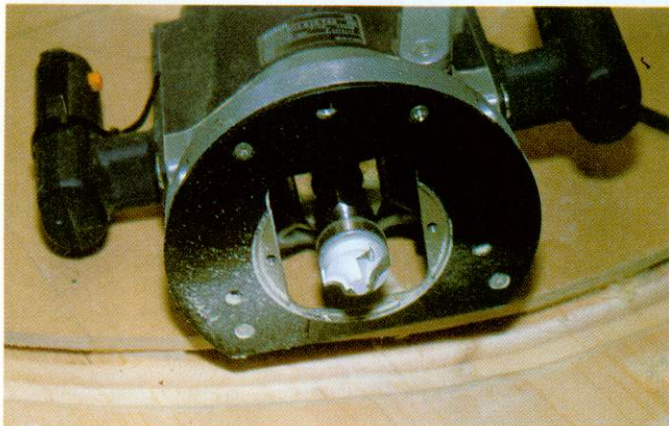
Cutting out the bear's face using the MDF template and guide bush
