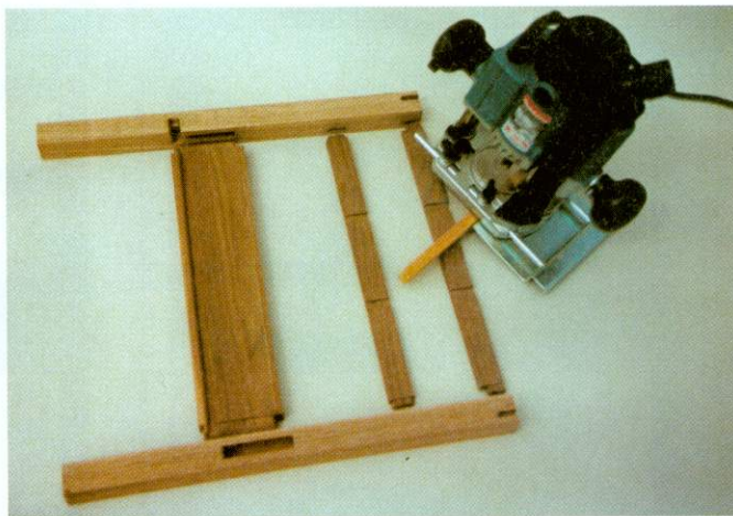
One end panel ready for gluing. Note the groove for the drawer runner
