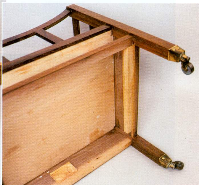
The drawer stop and runner can be seen here
