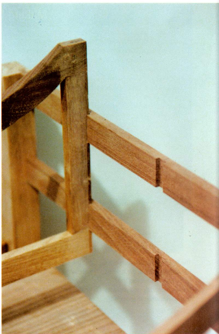
This project is almost all half-lap joints and rebates
