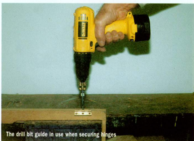
Boring with a twist bit
