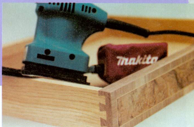
Smooth the burr with a fine finish abrasive paper
