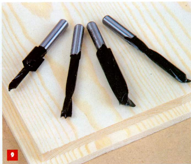
Four drilling bits: from left to right: \frac{3}{16} in drill/countersink/counterbore, \frac{3}{16} in lip-and-spur, 10mm lip-and-spur, 6mm lip-and-spur
