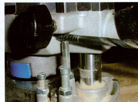
Setting the depth of cut
