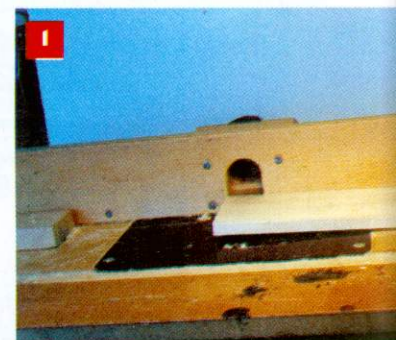
Side of box lowered on to router cutter with stops to control start and stop
