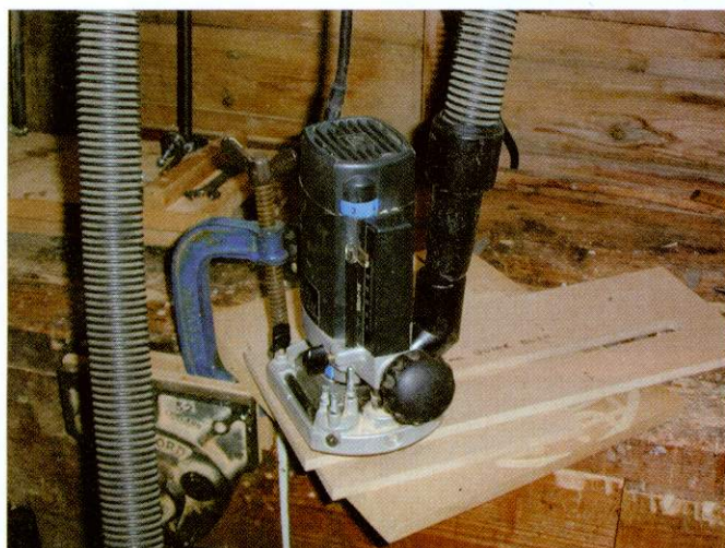
Machining the slots in the floor/back
