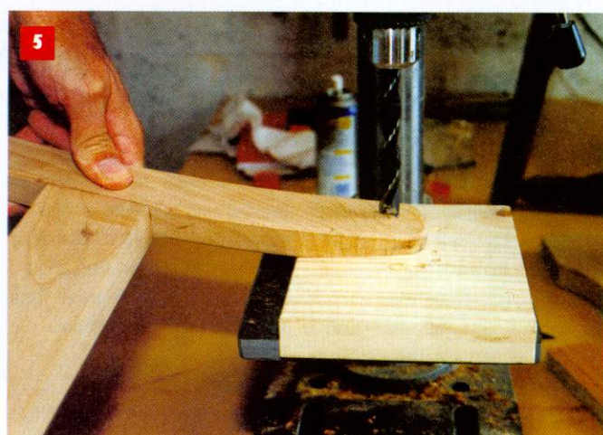
5 A cleanly cut bearing hole is important
