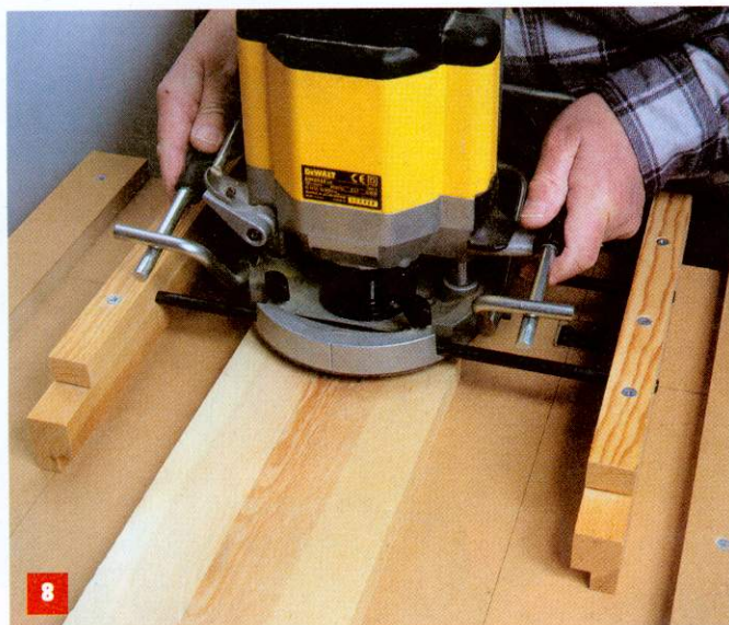
Thickening in progress with the 6-wing cutter in the DW 625 router, on my home-made thickening table with the router mounted on home-made 'skis'
