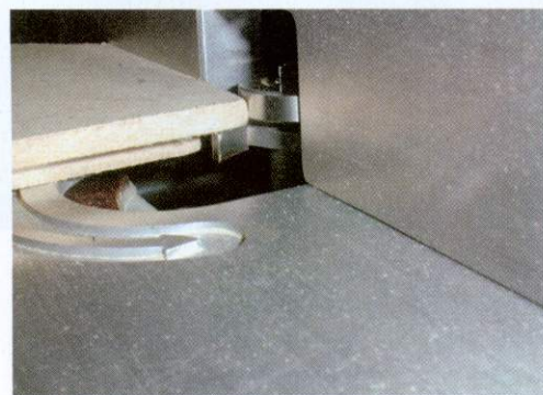
Machining the ends to receive back and floor (guard removed)
