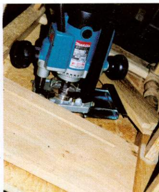
A groove is cut for the drawer rails to fit into the end panels
