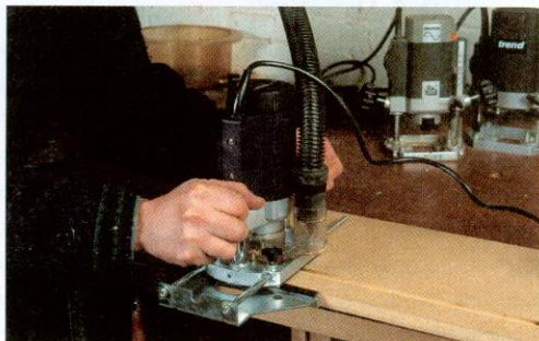
Pressed steel side fence for straight edge work
