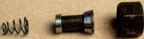
Small spring pushes collet out to ease cutter removal
