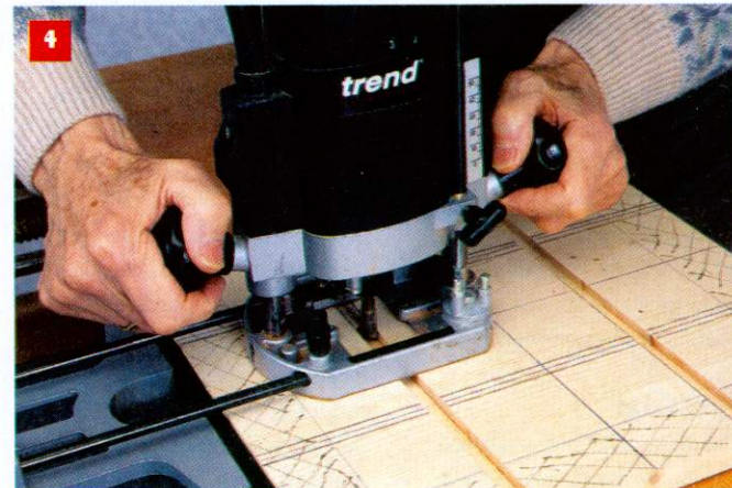
Dovetails being routed with side fence set to cut equidistant slots from each of the four sides of the board
