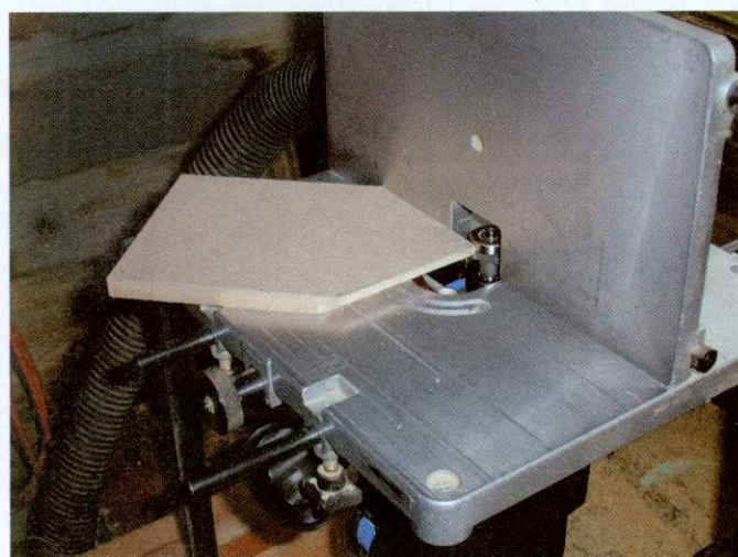
Machining the ends to receive the roof (guard removed for photograph)
