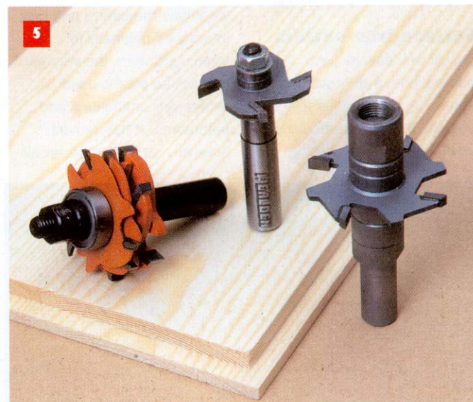
Three heavy-duty slotters: CMT, Wealden, Titman. The CMT slotters can be used singly or in combination
