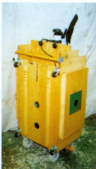
Rear view. Note the cable holes and the notches in the runners to stop the workcentre from slipping when leaning against the van.
