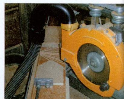
Cutting the slope on the end pieces
