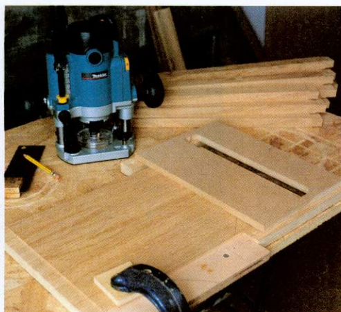
The rails are cut from a wide board after the tenons have been cut on their ends. Note the home-made jig
