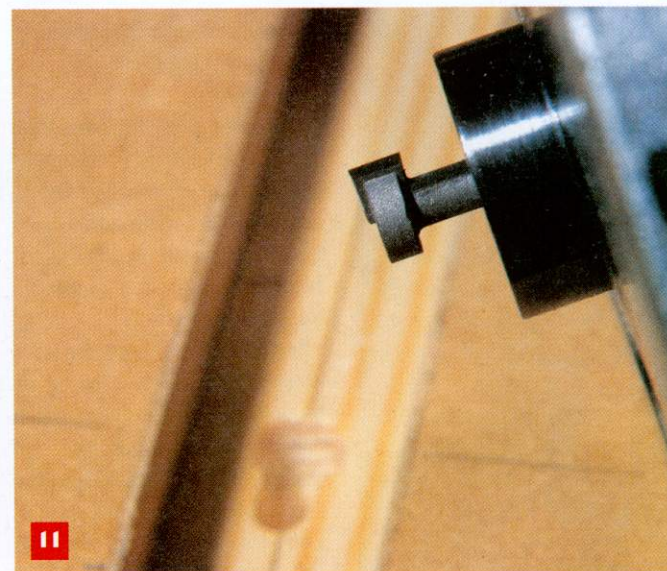
A keyhole cut being made in the back of a plaque for wall mounting. Note the simple home-made jig to guide the guide bush
