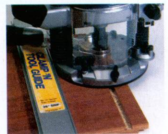
Housings can be made by running the router against a straight edge...
