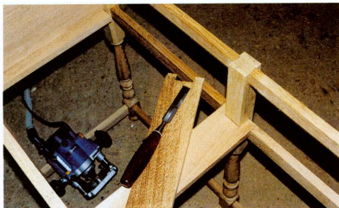
The drawer runners are notched into the rails
