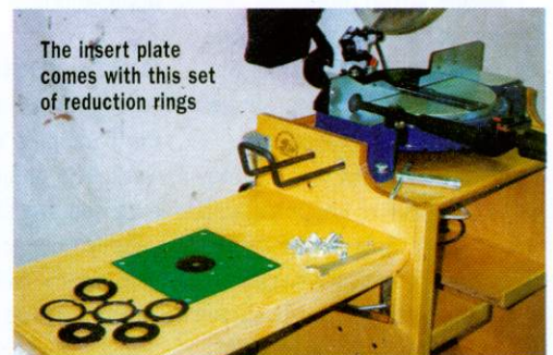
The two holes either side allow you to use the extensions for the chopsaw
