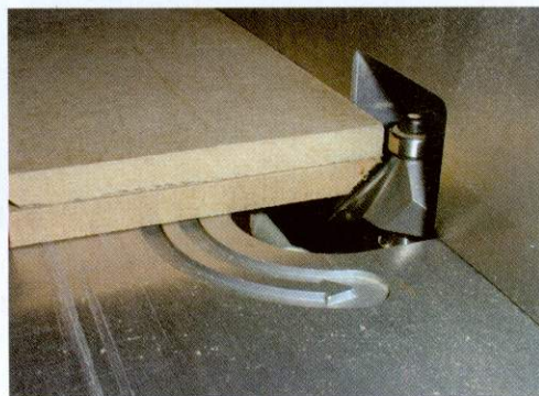
Machining the roof mitre (guard removed)
