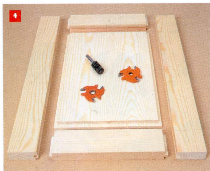
The components of a small panelled door with the only two cutters used to make them - \frac{5}{32} in for biscuit jointing the panel boards, and \frac{1}{4} in for grooving the rails and stiles and tenoning the rails. They were used on a \frac{1}{4} in arbor
