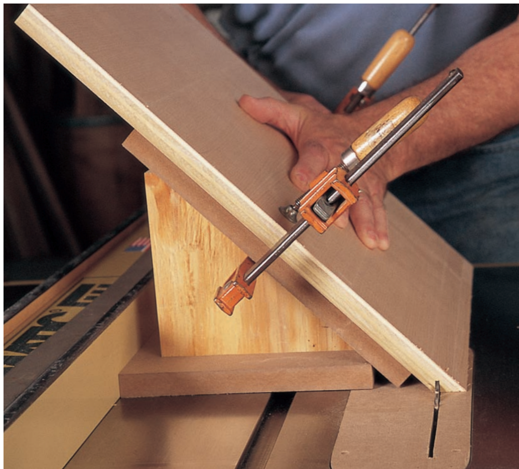
A shop-made angle sled allows you to cut both bevels and spline grooves on the table saw without tilting the blade. Clamp the work to the sled's sloping fence and guide the sled along the saw's rip fence to make the cut.
