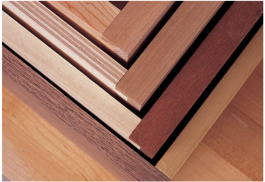
Stock thickness doesn’t affect router-cut half-blind dovetails. You can use one thickness for fronts, a different thickness for sides and even a third for the back.
