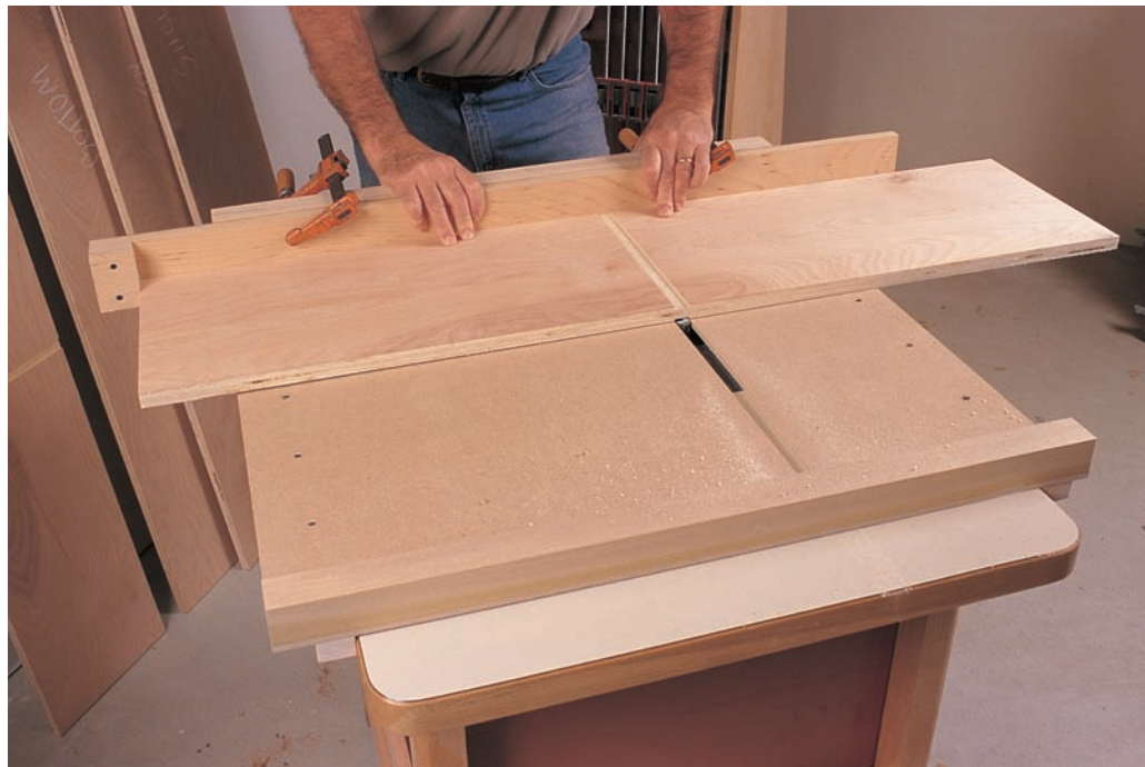
Dado large workpieces on a router table with a sled like a table-saw crosscut sled. A stop clamped to the sled's fence locates the cut and immobilizes the work. Slides on the underside reference the edges of the tabletop to guide the sled.
