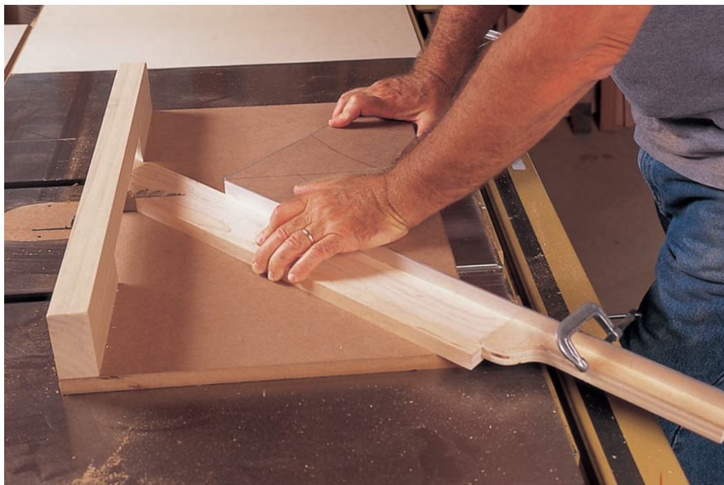
A fixed miter sled for the table saw produces perfect right-angle joints. Stops clamped to the aluminum angle fence extensions ensure parts are properly sized.
