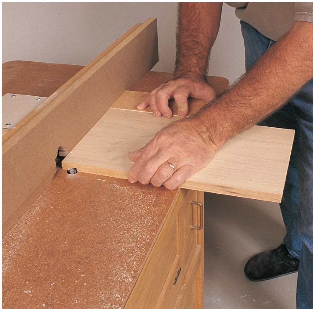
The typical router table setup works for dadoing parts like drawer sides. A push block — just a square scrap — stabilizes the work and backs up the cut, preventing tearout as the bit emerges from the cut.
