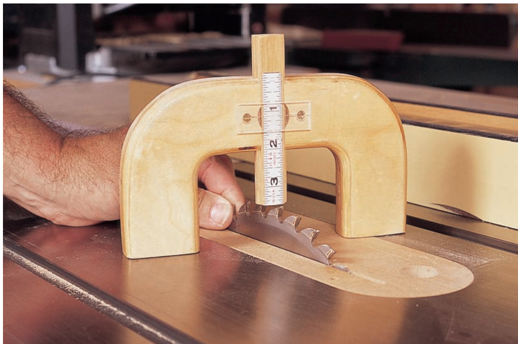
Using a rule or commercial or homemade gauge, set the height of the blade to match the tenon length you want.
