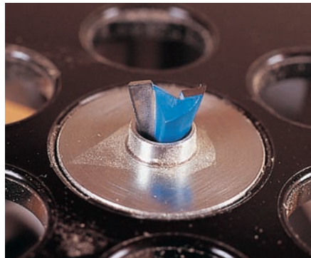
Stock thickness doesn’t affect router-cut half-blind dovetails. You can use one thickness for fronts, a different thickness for sides and even a third for the back.
