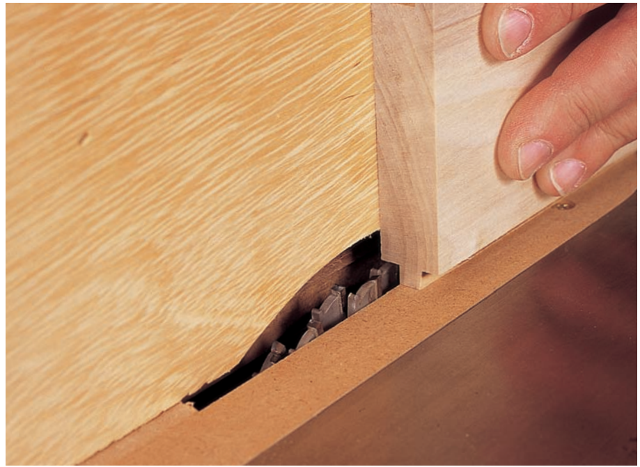
A rabbet cut into each edge of the board forms the tongue. It's a good idea to cut a sample and check its fit before cutting all of the boards.
