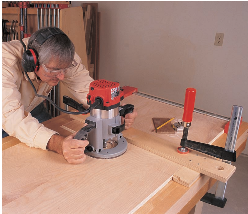
A crossbar attached at right angles to a plywood straightedge makes an easy-to-align T-square guide for dadoing with a router. Clamp it securely to the work and the bench top at each end.
