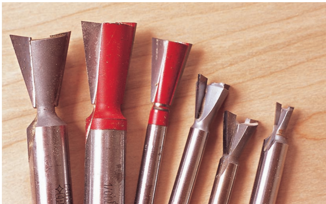
Dovetail bits are made in a wide variety of diameters, roughly from \frac{1}{4} " up to 1". Angles range from 7^\circ to 14^\circ .
