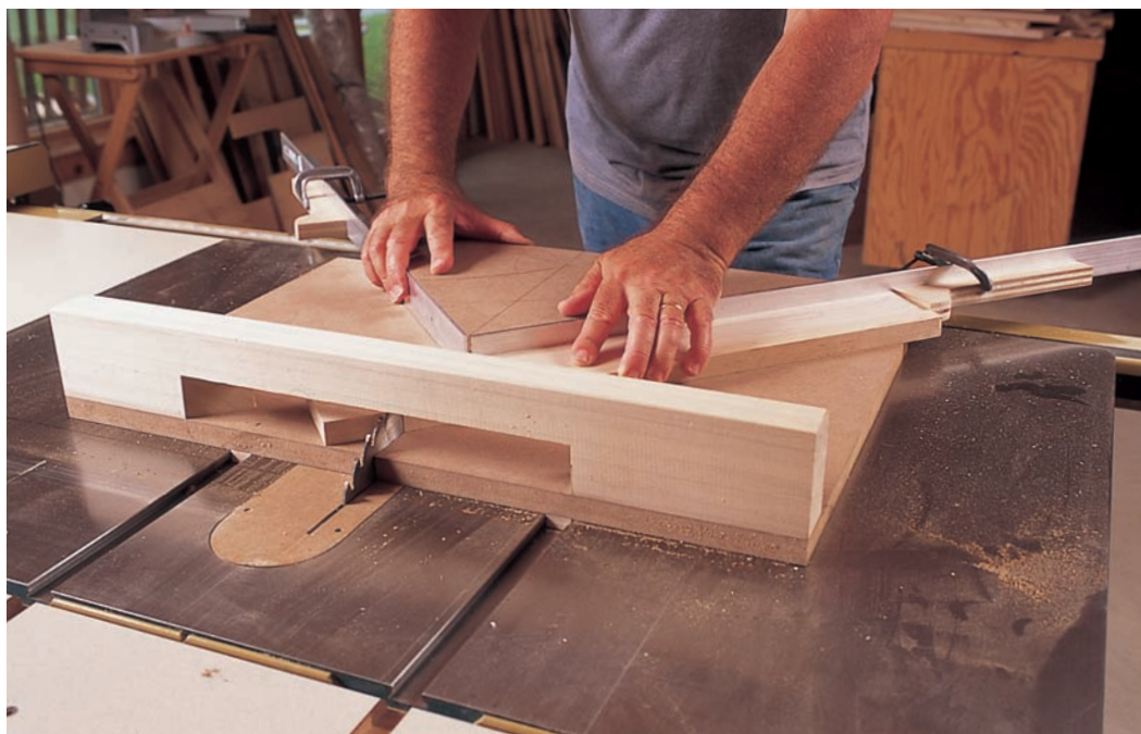
With the sled, cut one-half of the joint on the left side of the blade, the other part on the right side. The miter cuts may not be perfect 45° angles, but as long as the sled's fence block is a perfect right angle, the miters cuts will come together at a perfect right angle.
