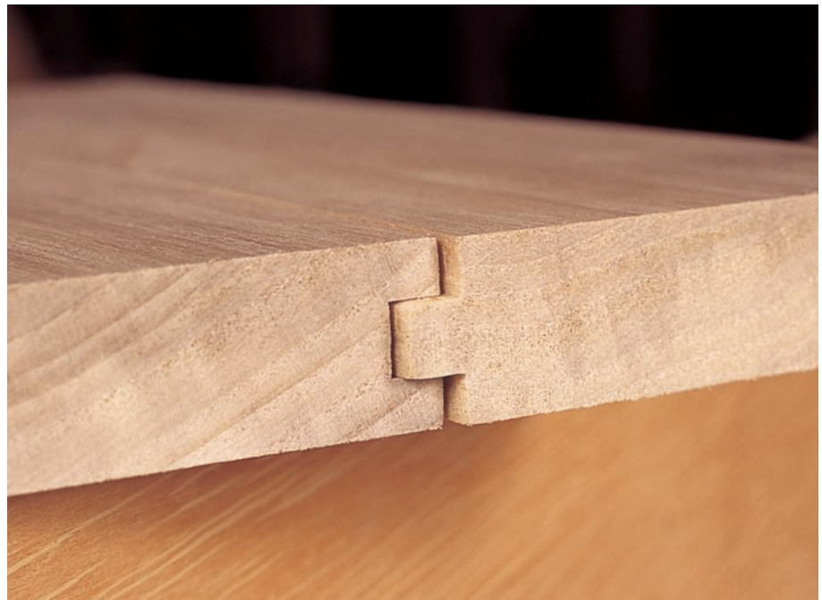
A rabbet cut into each edge of the board forms the tongue. It's a good idea to cut a sample and check its fit before cutting all of the boards.
